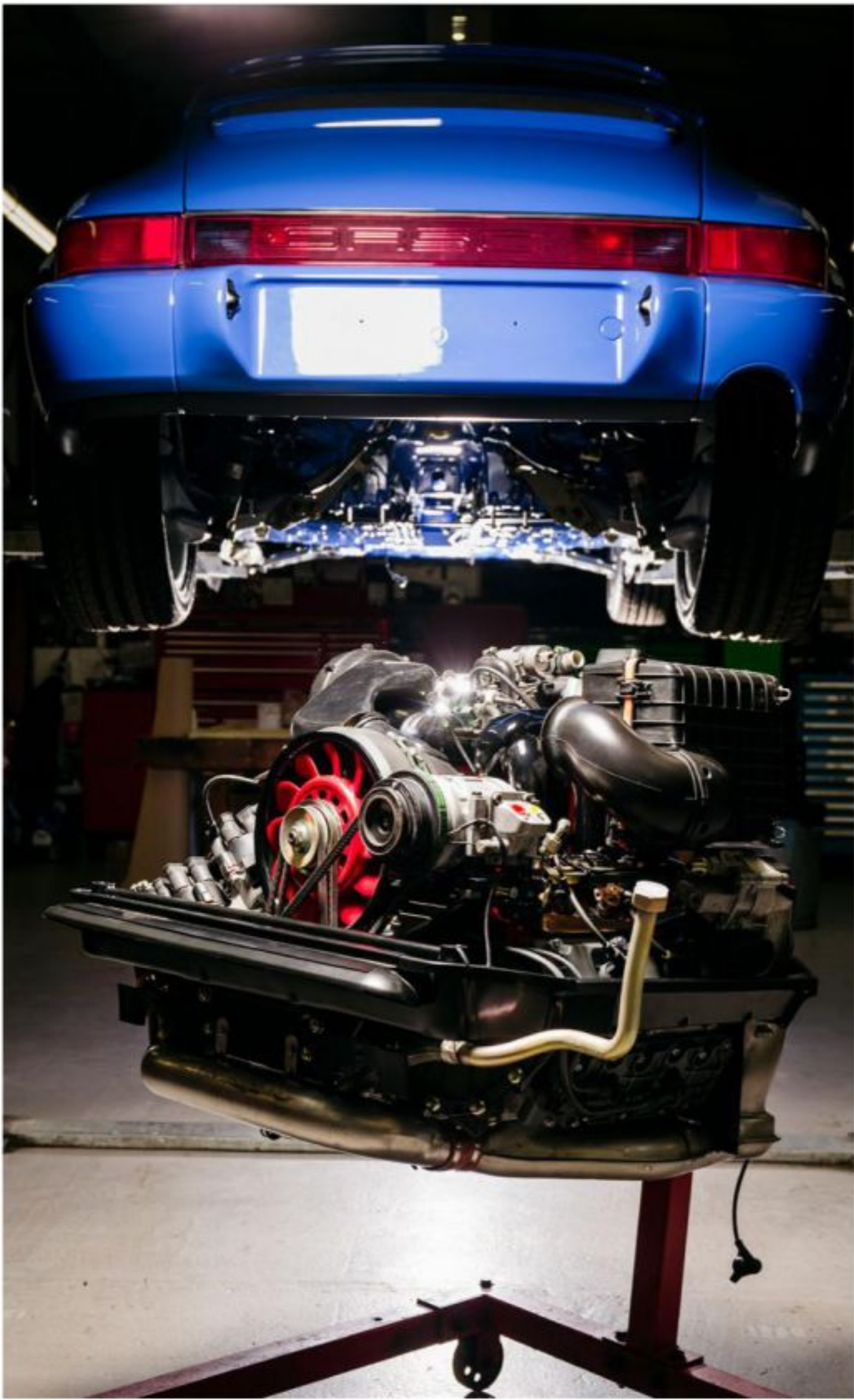
LEFT Flat six is a mixture of 964 C2, 993 RS and custom 9m parts
