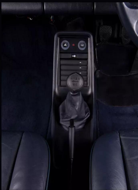
ABOVE G50 gearbox (above) is more desirable than the 915 gearbox, where reverse is down and right
