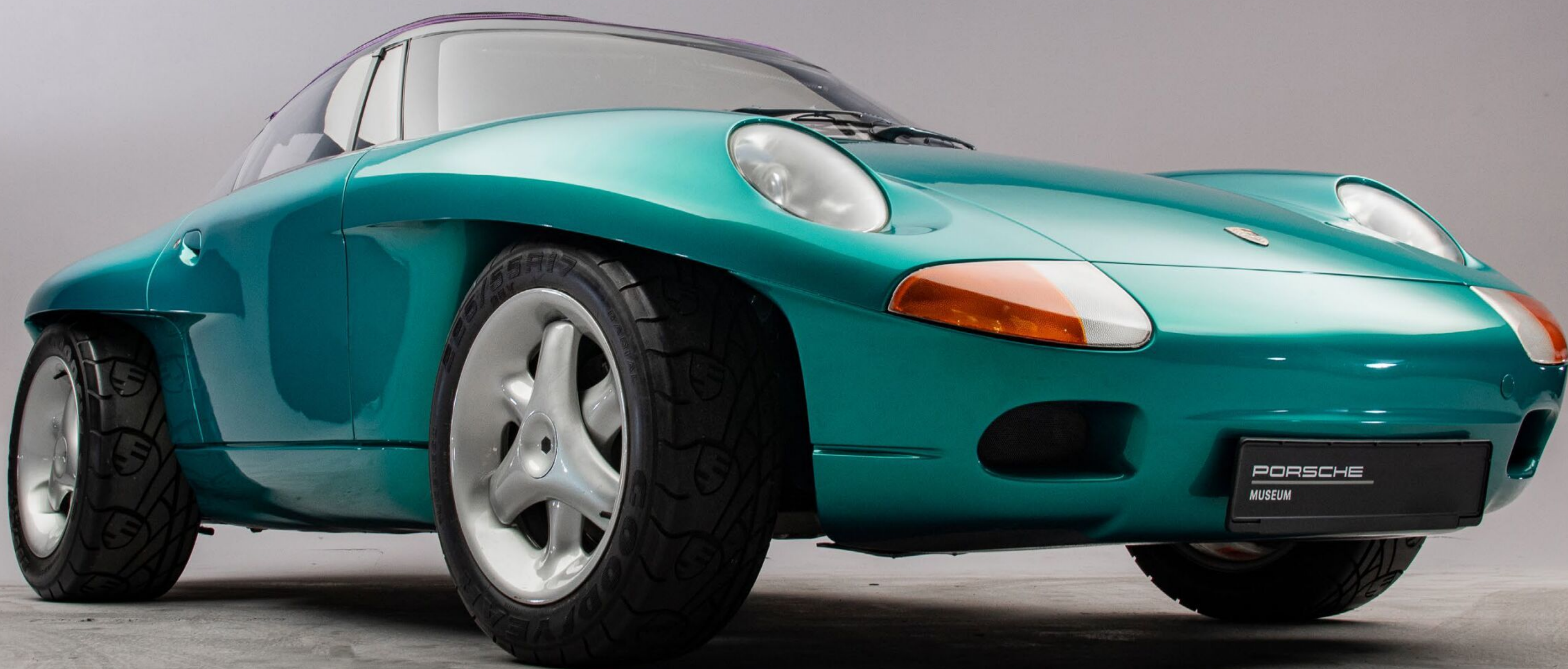
ABOVE Panamericana's body was made from carbon fibre. Cut-away arches allowed for long travel suspension and all terrain tyres
