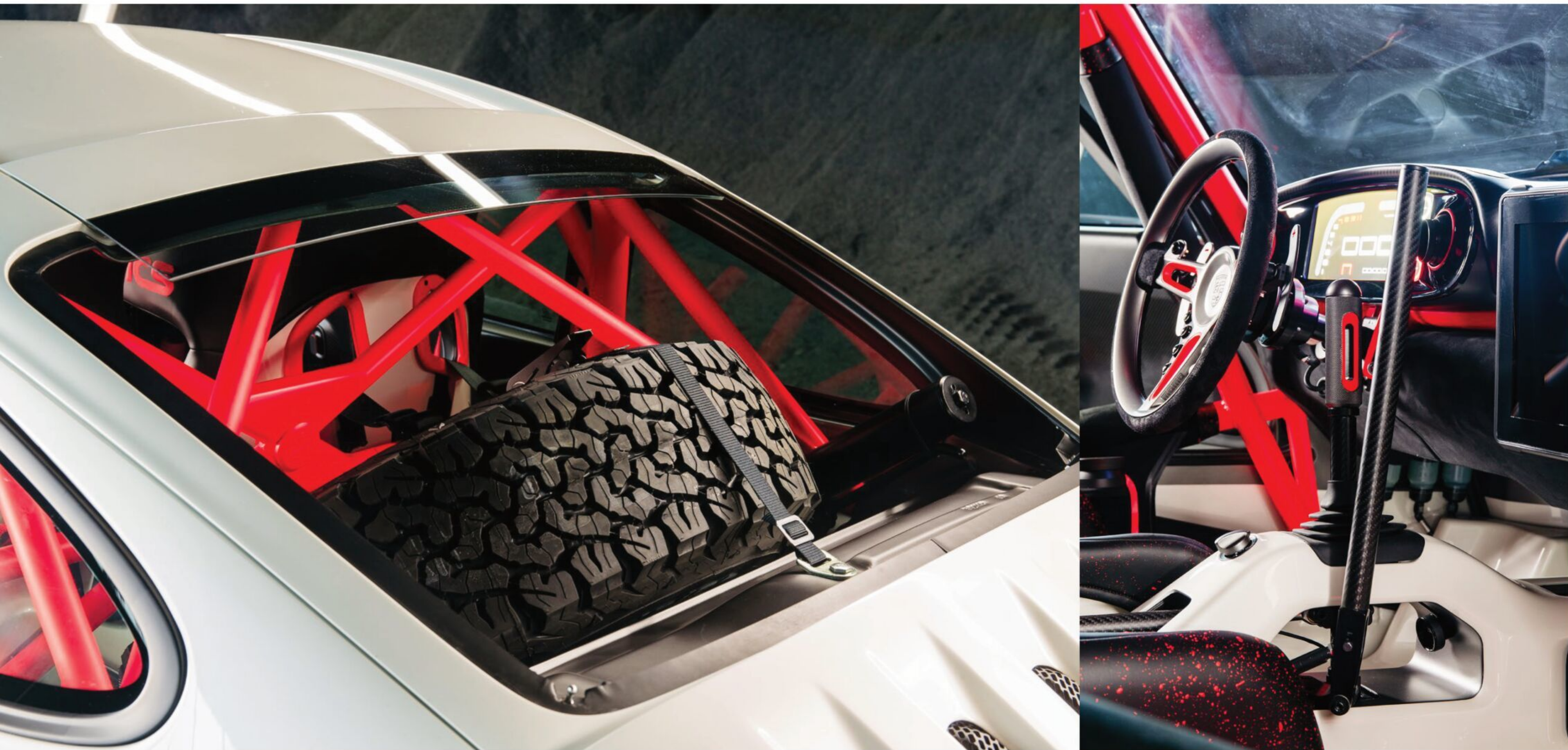
ABOVE Removable rear screen allows quick access to sixth wheel and all-terrain tyre
