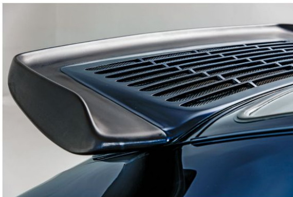
ABOVE Tea tray wing housed a single intercooler. Speedline wheels were the reserve of the 964 Turbo 3.6 and 3.8 RS
