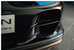
ABOVE The GT2 featured a revised front PU with larger air intakes over the 996 Turbo
