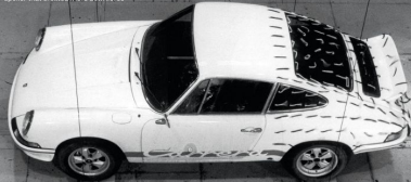
BELOW Three days of testing in a wind tunnel resulted in the ductal spoiler that created more downforce.
