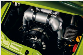
3.8 litre engine developed in-house, producing 385bhp @7500rpm
