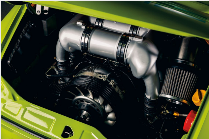
3.8 litre engine developed in-house, producing 385bhp @7500rpm
