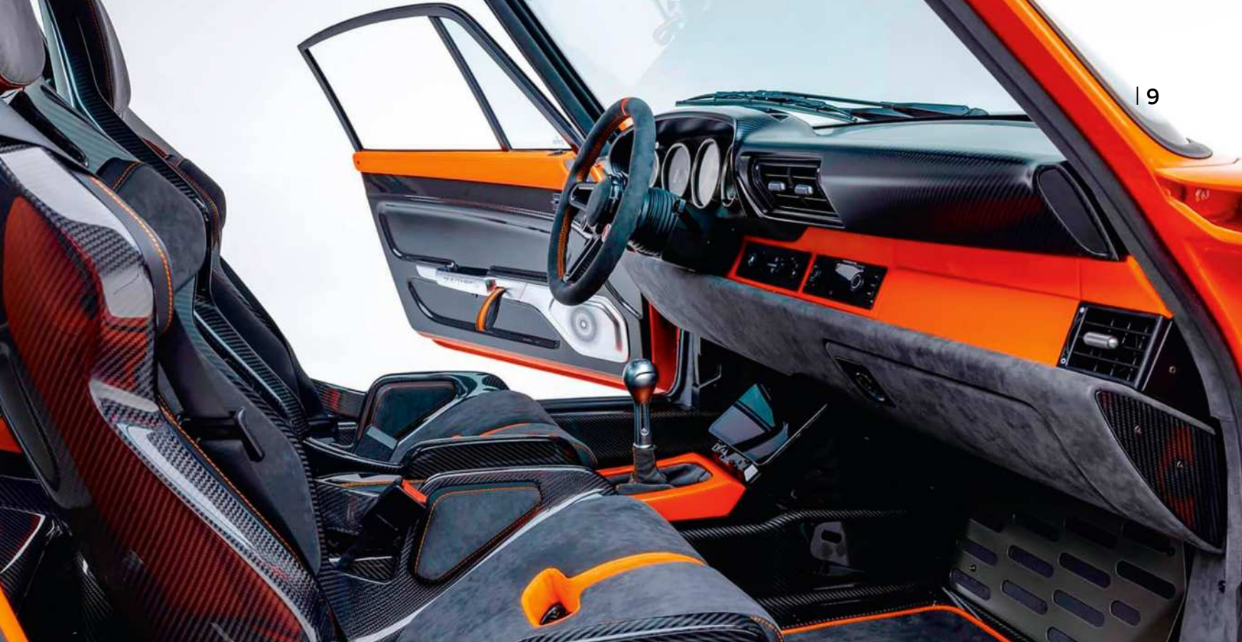
ABOVE The bespoke carbon-fibre steering wheel features controls for track days, while carbon-fibre bucket seats can make use of five-point harness and three-point belts
