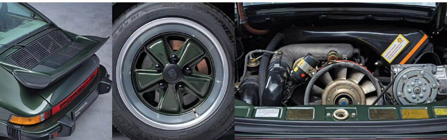
ABOVE The Oak green metallic of Ferry Porsche’s 930 extends to its Fuchs wheels, although the Porsche crest was painted black to help it stand out. The 3.0-litre blown flat six ensured the car could achieve 0-62mph in 5.5s with a top speed of 155mph, but interestingly Ferry chose to remove all external references to the 930’s Turbo nature
