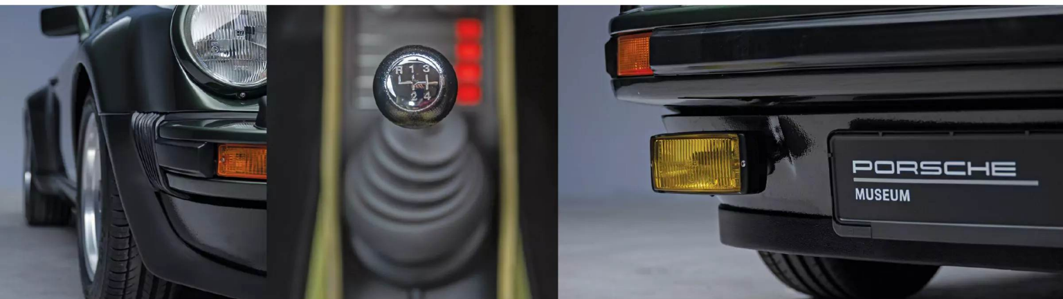
ABOVE Ferry’s 930 featured many production Turbo features including its wide-arched body, to accommodate girthier Fuchs wheels. A four-speed gearbox fed power to the rear wheels only. Yellow fog lights were ordered as standard, alongside air conditioning, a passenger side mirror, a radio with traffic broadcasts, and a sunroof
