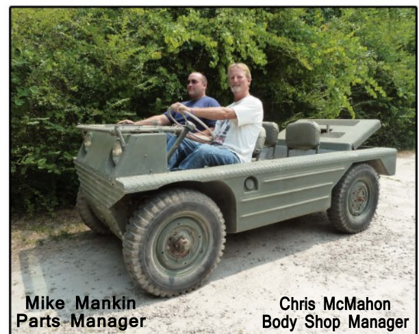
1953 "The Flair #115" - all aluminum amphibious prototype with a Fletcher - Porsche designed engine
