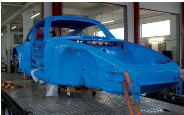
Care was taken to preserve the original chassis number in its original panel (far left), exactly as the factory stamped it back in December 1975. With the the body restoration and the installation of the rollcage complete, Kremer had the bare shell coated with a rust-preventative, which coincidentally is a close match to final colour!
