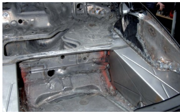
New inner strengthening box-sections were fabricated by Kremer to replicate the original panels which were beyond use. New front end (far right) now complete following lengthy seam-welding session! New weld-in rollcage was necessary to meet current FIA regulations - original bolt-in cage was no longer legal
