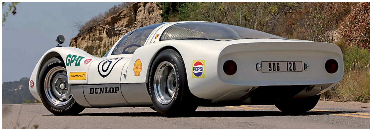
Rear three-quarter view is the most dramatic, showing off the ultra-low profile to perfection. Wheels are two-piece, with aluminium rims riveted to steel centres
