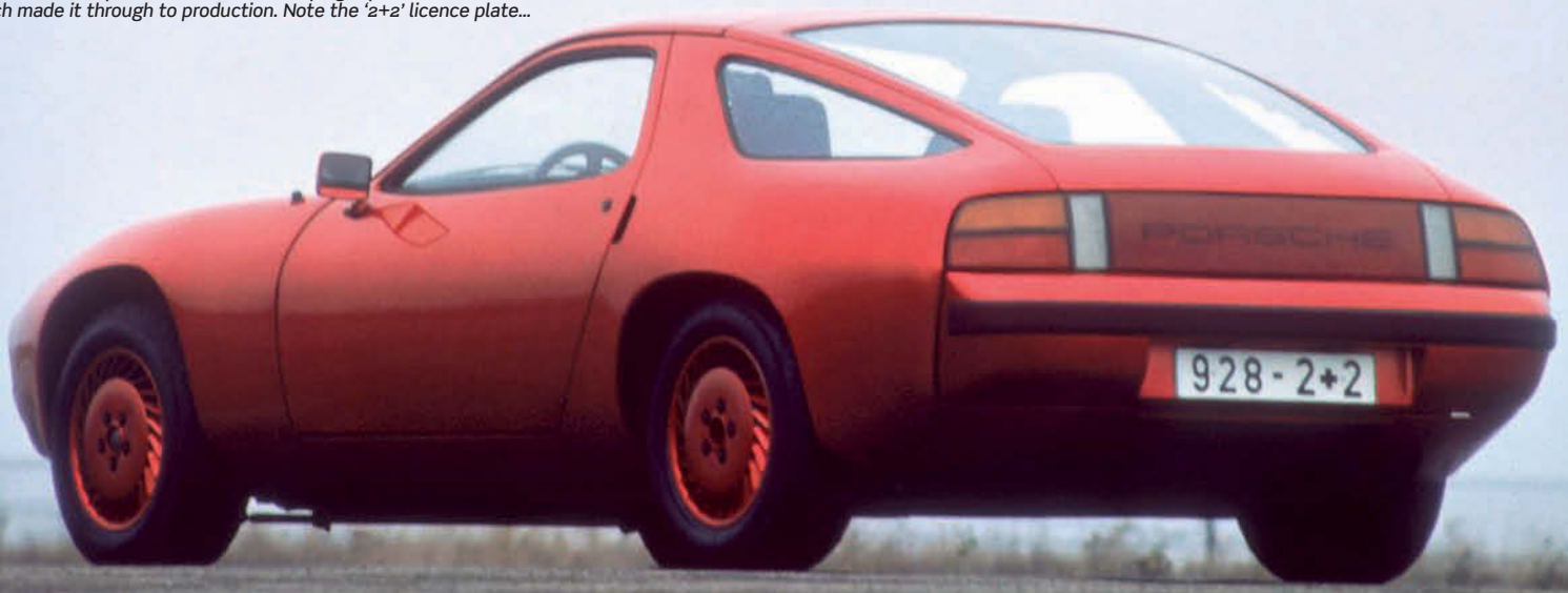
Porsche built a number of mock-ups, this one dating back to 1973. The buttressed rear quarters and forward-sloping B-pillars are two elements which made it through to production. Note the '2+2' licence plate...
