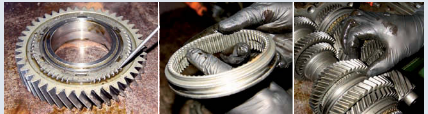
996/986 gearbox internals are beefier than those in, say, the old 915 transmission, but time has shown that second-gear dog teeth - specially angled for a smoother shift - are prone to wear. Rebuilding used not to be possible, but parts are now available - watch out for a how-to soon
