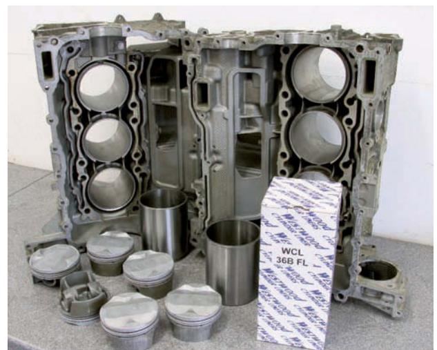
Mg6/Mg7 engine presents a number of failure scenarios, but scored pistons and bores – although often just two of each – are among the most serious (main photo, opposite). There are various explanations for that, but highly localised overheating, due to the water in the conventional coolant mix boiling and temporarily turning to steam, now seems the most likely. So far the most resilient – and elegant – solution appears to be the fitting of steel liners, as in this Redtek block (below), and Northway offers a similar conversion, but inevitably that is both a complex and costly route. Evans Waterless Coolant isn’t cheap, either (see next page), but pre-emptively it’s a lot less expensive than a full rebuild, and obviously far quicker and easier, too. Product has many other benefits, including excellent protection against internal corrosion and sludging of the radiator (above). Hartech-modified cylinder block (below left) shows cut-back coolant passage to improve flow: every little helps, it seems
