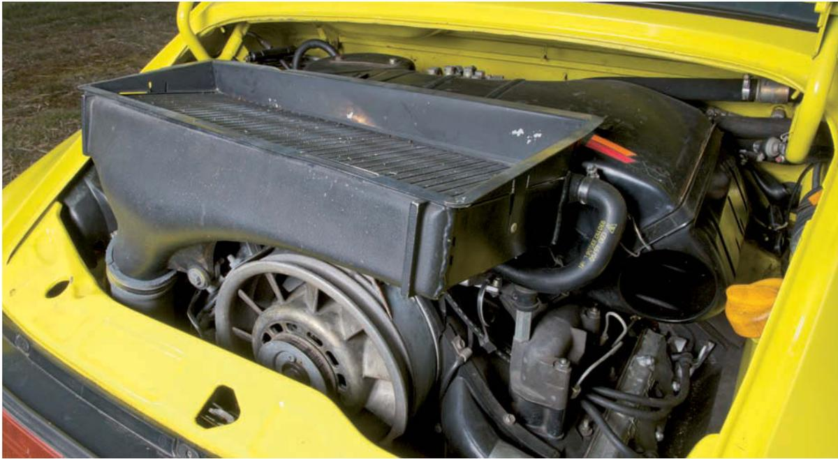
The DP Motorsport 3.3-litre Turbo S engine is dominated by a huge intercooler. Power is a lazy 360bhp, but adjustable boost control means it can be tweaked to over 400bhp
