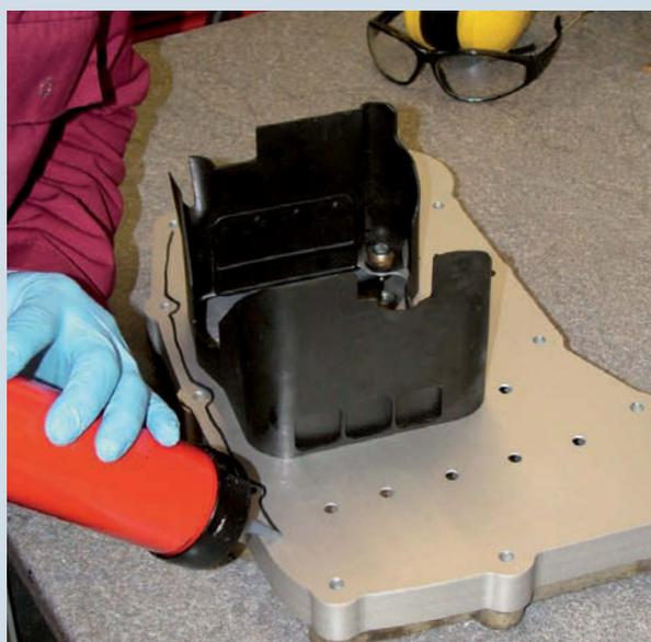
*Oil smoke in an Mg6 engine's exhaust can have a number of unhappy causes, but if it's purely as a result of hard circuit driving may be resolved by fitting a so-called deep-sump kit, which not only allows the engine to carry more oil without the danger of over-filling, but also – and no less importantly – has improved baffling to prevent oil surge. A new air/oil separator will almost certainly help, too*
