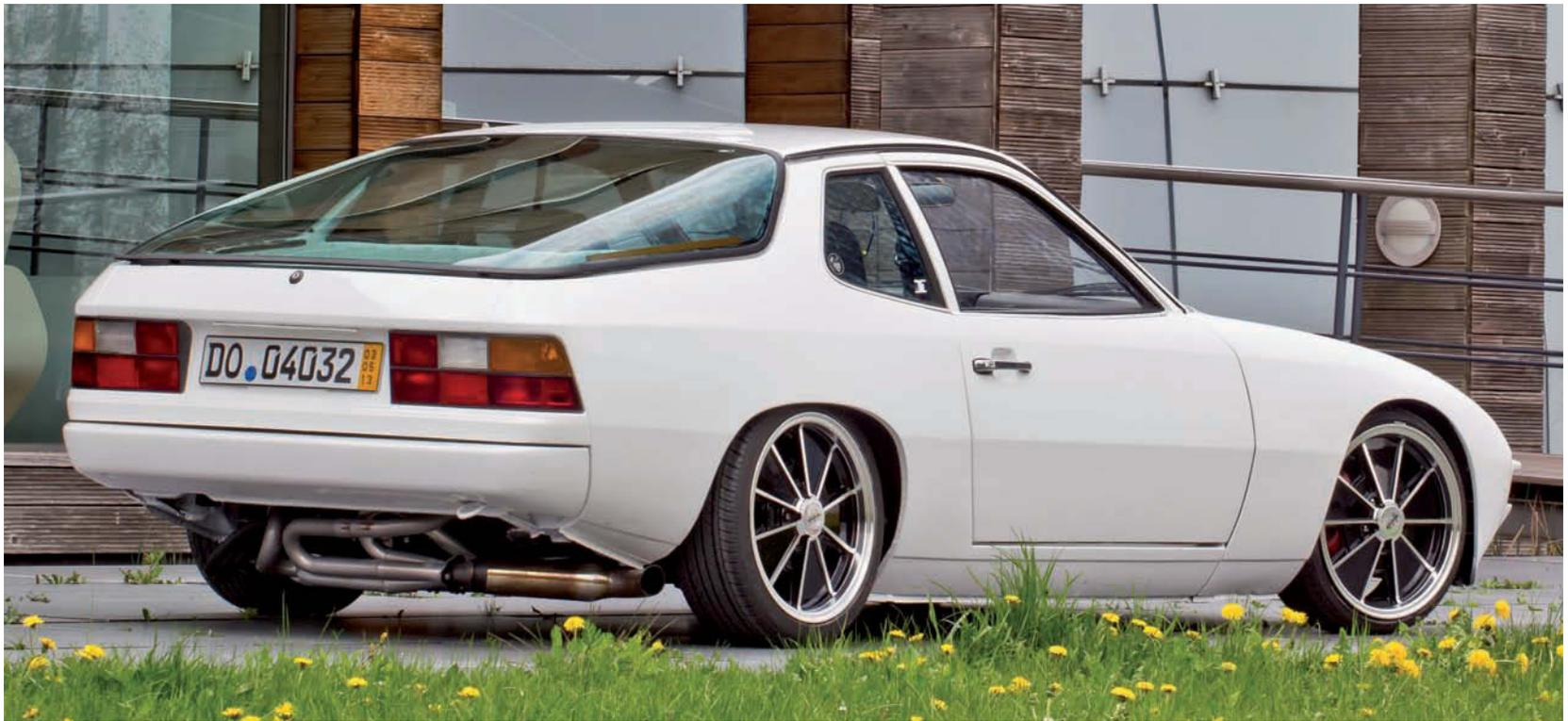
in favour of the MacPherson struts from the front of a Beetle 1303S. This allowed the fitment of Beetle discs and hubs, which in turn opened up a world of possibilities for wheel choices. As it is they've chosen a BRM replica wheel, which looks fantastic on the 924 and have echos of Fuchs about them.
