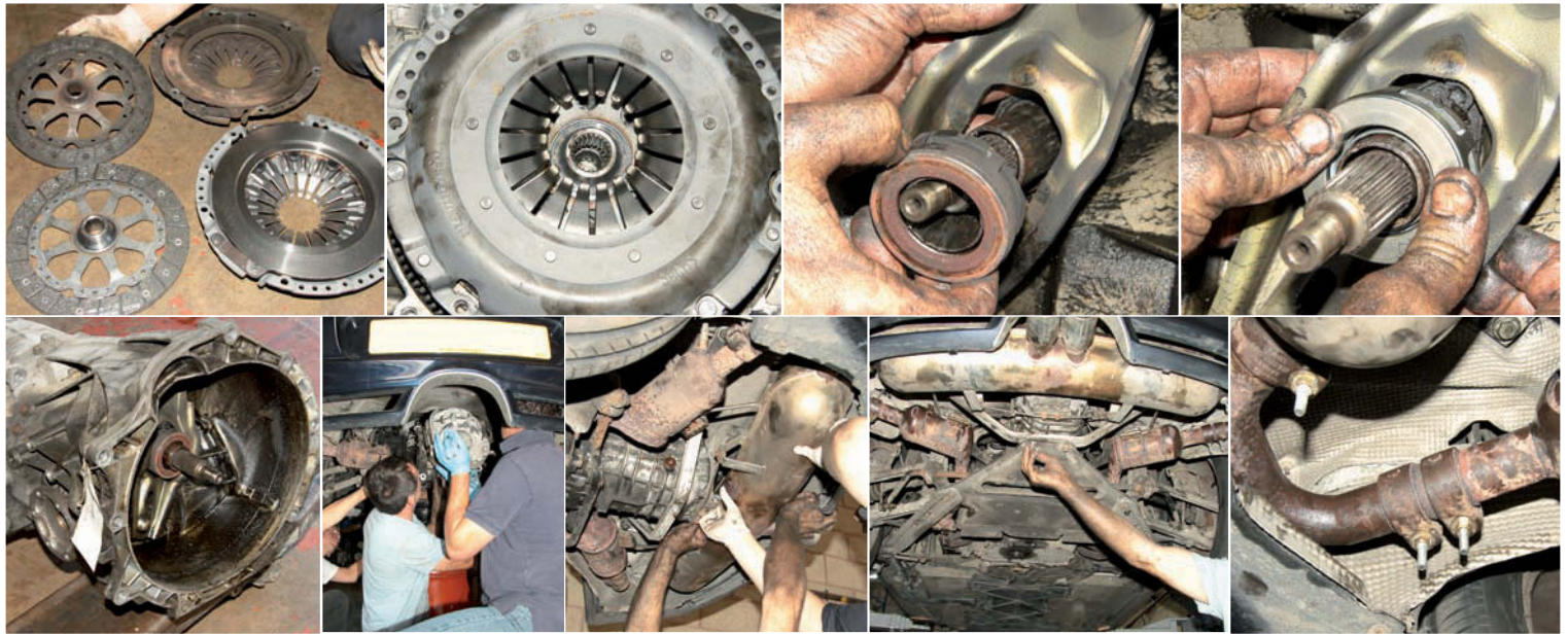
Clutch replacement is a simple enough task - but can you centre friction plate by eye alone (above)? We would guess probably not. Still no obvious sign of why clutch was so heavy. Release mechanism was OK; must have been cover-plate springs. New release bearing was fitted as a matter of course. Replacement transmission (above) shows evidence of leaking crank seal; oil easily rinsed put with brake cleaner. Team gathers again to manhandle transmission back into position; job nearly done
