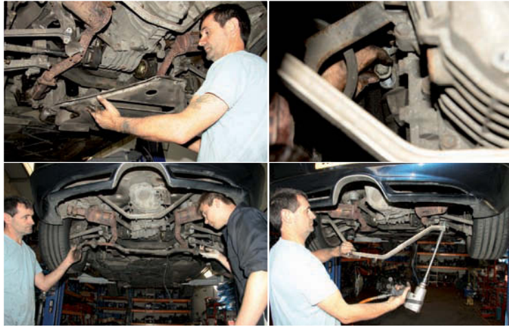
Obvious 'disconnections' to allow transmission removal include undertray(s) and support(s), drive shafts, anti-roll bar, and naturally clutch housing-to-engine bolts - no less naturally leaving a couple until you're ready actually to separate units. Younger of these two, above left, is apprentice Dan
