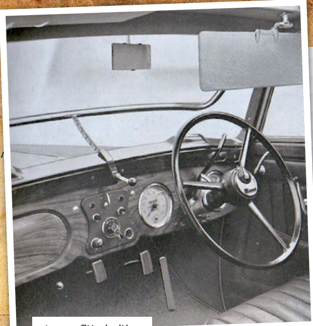
In cars fitted with preselector gearboxes, the left-hand pedal is referred to as the 'gear changing pedal', rather than a clutch pedal. Centrifugal design means no ordinary clutch pedal is needed
