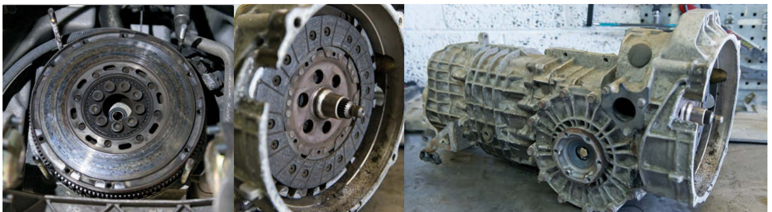
Above: Fraser's GT3 at TTV Racing's premises. Below: Gearbox off, old clutch removed
