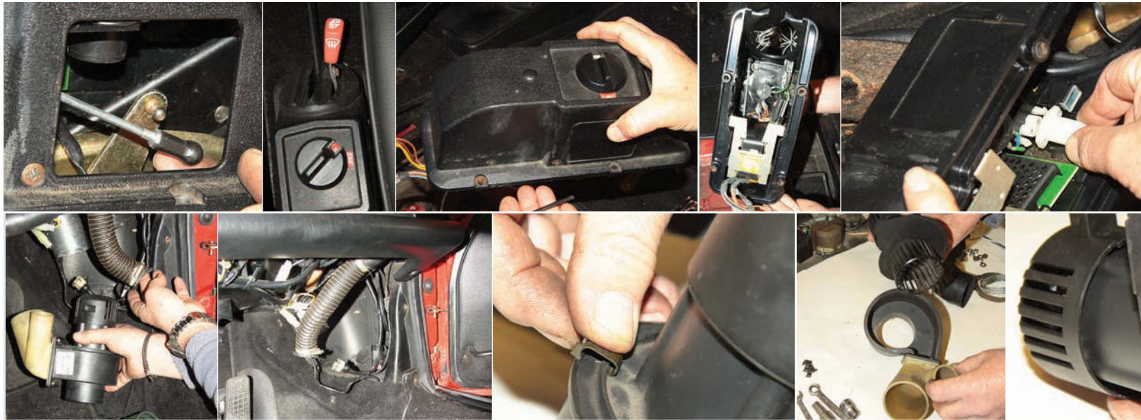
Infamous red heater lever fitted to earlier cars with automatic control unit (top row, second from left) was designed to be used only in 'emergency'; pull it before that arises and you will simply break the auto unit. Size of hole in bulkhead requires mods to new flap-valve sensor wire; larger connector is for cabin-temperature sensor. Multimeter is essential for accurately assessing components
