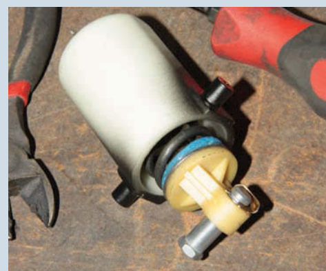
New clutch helper spring comes ready compressed - remove the split-pin (not shown) only after fitting
