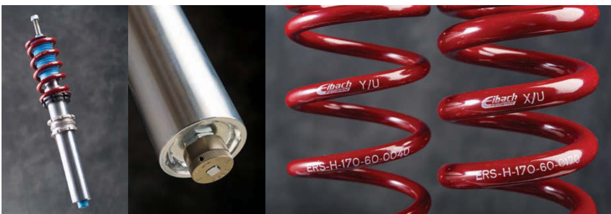
Far left: Complete Bilstein/Eibach spring and damper unit. Dampers are adjustable so we'll have lots of fun arriving at a set up. Not surprisingly the springs are rather thicker for the rear than the front. That will be all that weight from the engine then. Look out for complete fitting and set up feature in a future issue
