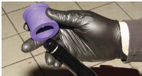
'M030' anti-roll bar for 944S2 used to be 30mm thick, but relevant part number has superseded to this 28.5mm diameter item (above, in Rob Nugent's hands)
