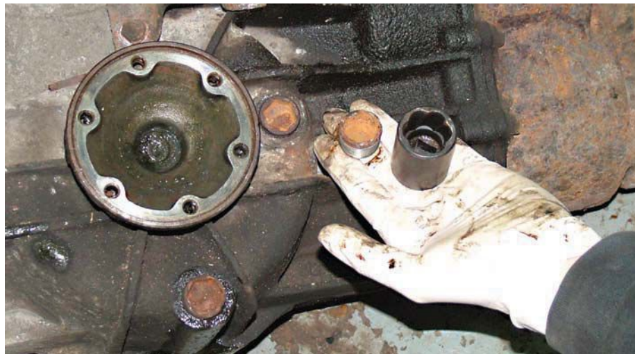
Many transmission drain and filler plugs – shown here on a 924S transaxle removed from the car – require the use of a hefty hexagonal key to locate in their central recess in order to undo them. They often 'round out', though, in which case one of these special reverse-fluted sockets should do the job
