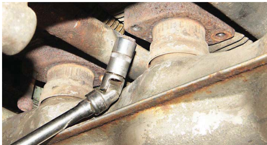
Avoid this scenario, says JZM's Steve McHale – and potentially having to damage the heat-exchanger to fit the socket on the nut in the first place – by first quickly heating the nuts to cherry red
