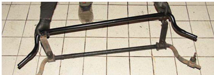
'M030' anti-roll bar for 944S2 used to be 30mm thick, but relevant part number has superseded to this 28.5mm diameter item (above, in Rob Nugent's hands)
