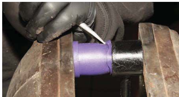
'M030' anti-roll bar for 944S2 used to be 30mm thick, but relevant part number has superseded to this 28.5mm diameter item (above, in Rob Nugent's hands)
