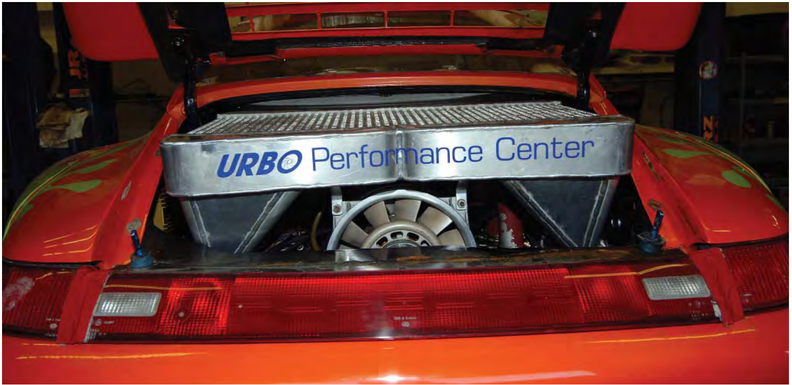
Top: The NACA inspired intercooler is vital in making big power. The design's flow dynamics limit the amount of resistance thus generating more boost. Bottom: The engine/transaxle are moved 1 inch within the wheelbase to improve weight distribution.
