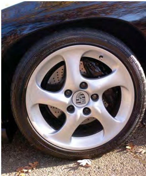
Sporting 996 Turbo wheels, 8x18 with 225/40 ZR 18 tires in front and 11x18 with 295/30 ZR 18 out back, this 928 is all business.
