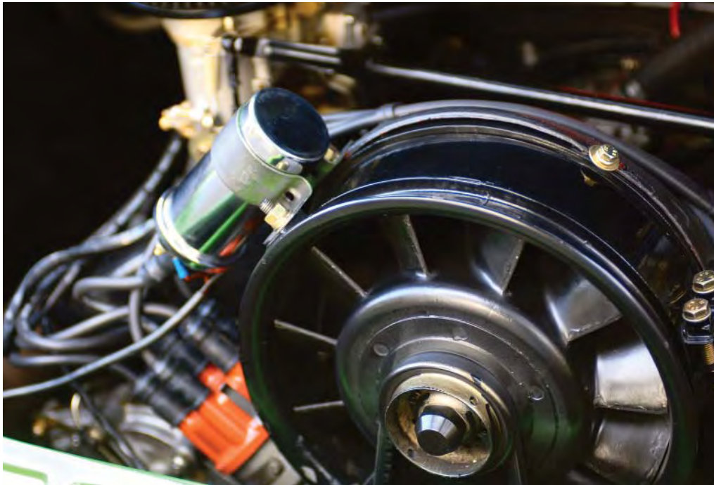
The engine features a high-lift cam to extract the best range of power from its PMO 46 MM carburetors. Compression is 10.5:1 using Mahle high-domed, Nikasil-coated pistons. The 3.2 flat-6 produces nearly 300 hp at the fly.
