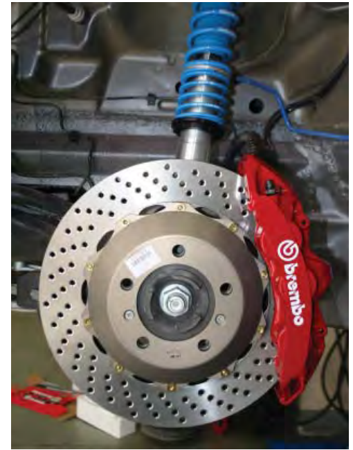
Below: The RK Coupe includes a specially designed Bilstein coil spring/shock system with larger Brembo brakes. Bottom: STU-DIOTORINO modifying the Cayman S body.
