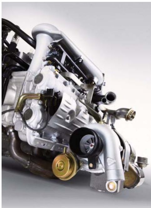
The rear-drive SPR1 was clocked at 240 MPH at Nardo with its Twin-Turbo, 3.6L, dual injector engine.
