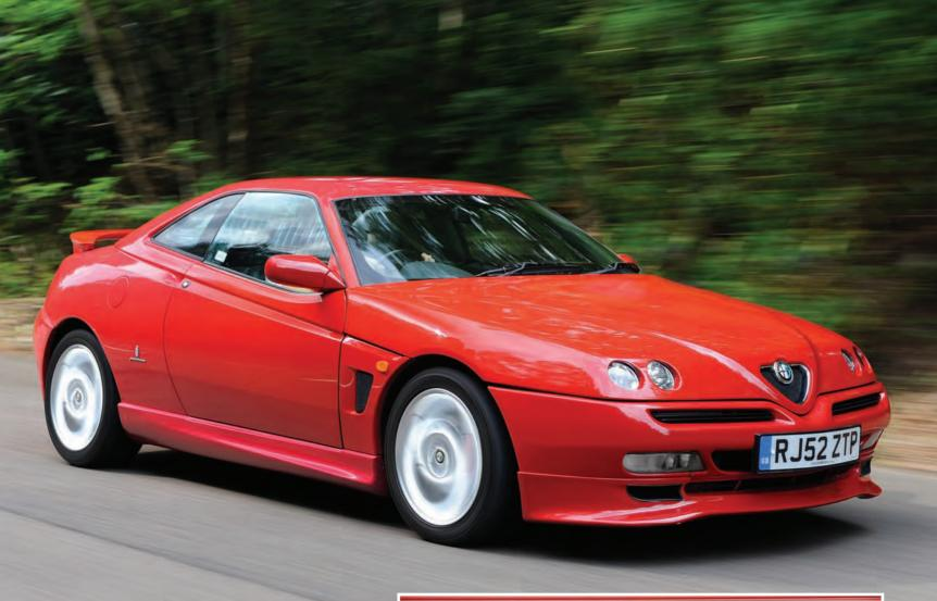
Autolusso), GTA 3.2 single-mass flywheel and clutch (saving around 4.5kg), Koni STR.T OE-spec dampers, Suplex OE-spec springs and custom exhaust with one fewer silencer in it.
