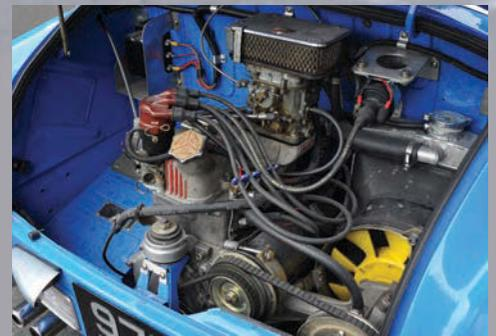
cam engine but nevertheless it enjoyed some notable competition success. Three Double Bubbles finished in the top three places in class at the 1957 Mille Miglia. The winning Double Bubble averaged a staggering 73.26mph over 1000 miles – not bad for a 750cc pushrod engine producing 47hp at 6000rpm.
