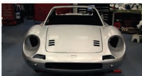
Nut-and-bolt restoration in progress of a Dino 246 GTS to original specifications.
