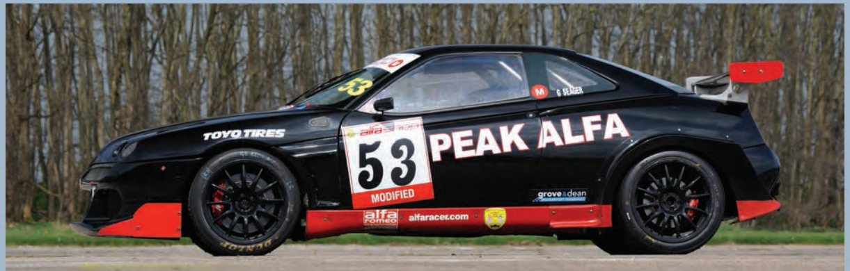
ABOVE: Graham Seager's brutal-looking overbored 3.8-litre GTV pushes out nearly 500bhp thanks to the Rotrex supercharger
