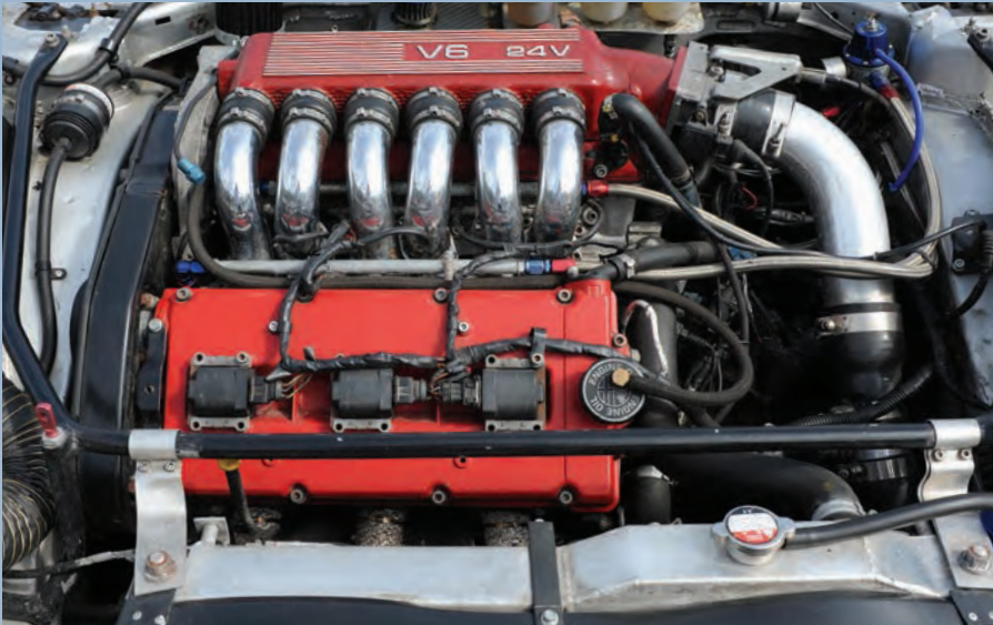
ABOVE: Graham Seager's brutal-looking overbored 3.8-litre GTV pushes out nearly 500bhp thanks to the Rotrex supercharger
