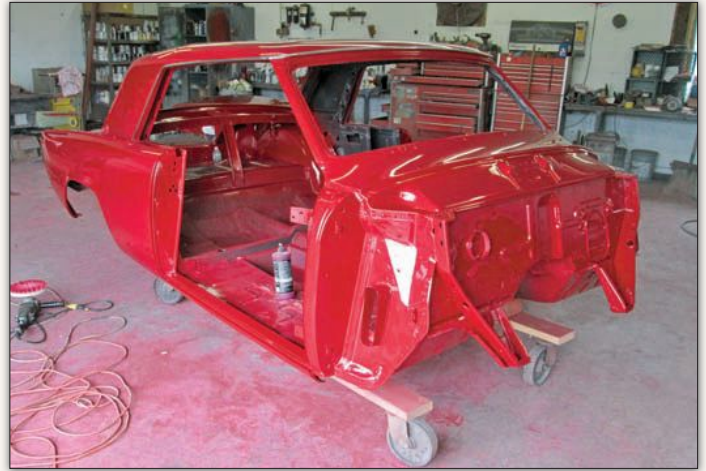
Bordeaux Red, a correct model-year factory color, was chosen versus the original Golden Sand color. The paint was PPG DBC Concept single-stage, matched to sections of original panel that had not been exposed to UV light and other dulling elements.
