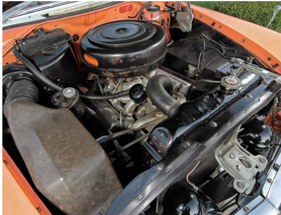
Red Ram Hemi V-8 was a 241-cu.in. little brother to the Chrysler’s FirePower 331 engine. With the dealer-installed Offenhauser intake and four-barrel carburetor, the Red Ram produces 170 horsepower.
