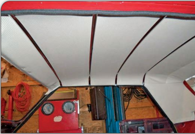
Few interior parts were reproduction material, such as the headliner. Described as unforgiving, the material had to be carefully positioned and secured. The most difficult areas were the complex C-pillars. The chrome ribs are restored originals.
