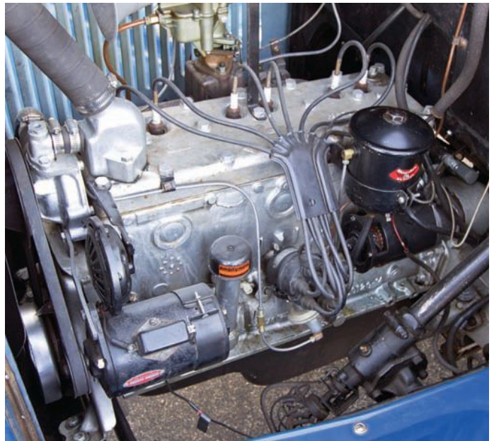
Dodge's cast-iron flathead six displaced 189.8 cubic inches, offered 5.2:1 compression, and developed 61 horsepower in 1930. To make this Phaeton more roadable, the owner swapped in an externally identical 217-cu.in. L-head six (with 6.2:1 compression) from a 1941 Dodge. This bumped power up by a third, to 91 horsepower.
