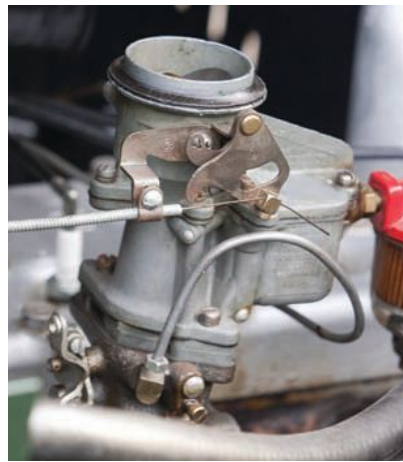
A Carter BB downdraft carburetor trickles fuel to the 228-cu.in. L-head six-cylinder used in this Canada-built truck. U.S.-built light trucks were equipped with a 230-cu.in. straight-six. Heavy duty oil-bath air cleaner was used on Dodge trucks following WWII battlefield torture testing.
