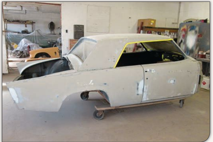
After all of the metal work had finally been completed, the body was partially reassembled and delivered to the body shop. Skim coats of body filler are in the application and sanding phase. Note the fabricated dolly to help move the shell around.
