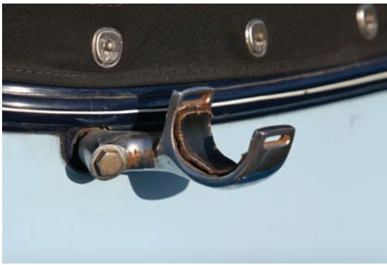
The Phaeton roof is not permanently attached, but it is foldable. It rests on one hook on each rear corner.
