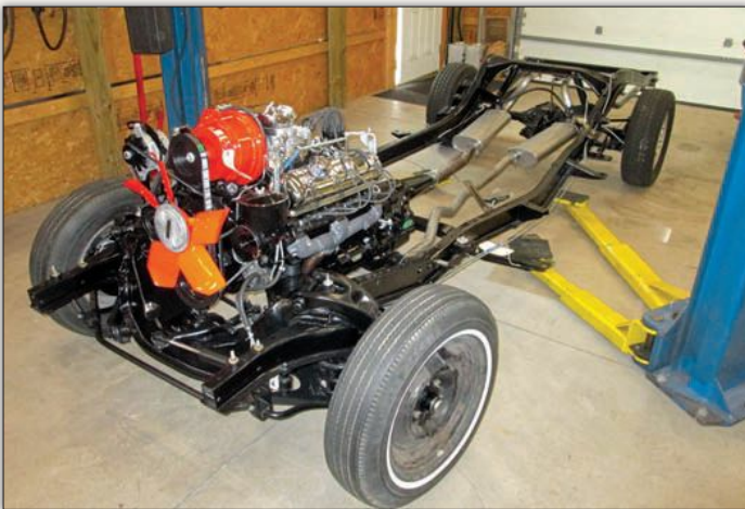
The chassis restoration has been completed. This includes the installation of the rebuilt engine, the Borg-Warner automatic transmission, installation of the dual exhaust system and the freshly rebuilt Paxton supercharger and corresponding parts.
