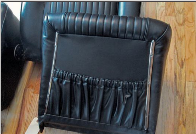
A previous owner had already used NOS vinyl upholstery to change the interior color from brown to black. Its long-term storage ultimately resulted in exceptionally minimal wear, meaning the upholstery was reusable, the exception being the seatbacks.
