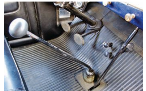
All is as should be inside the Phaeton's interior, save for that overdrive knob. To allow a top speed greater than 40 MPH, the owner installed a mid-1950s Dodge overdrive unit. With a .70 overdrive gear, this knocked the final drive ratio from 4.9:1 down to a reasonable 3.43:1.
