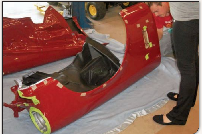
The front fenders, which also received the same paint process, received some of its componentry, such as the headlamp bucket and vent door. Note the application of painter's tape, done to protect the edges of the finish, preventing unwanted chipping.
