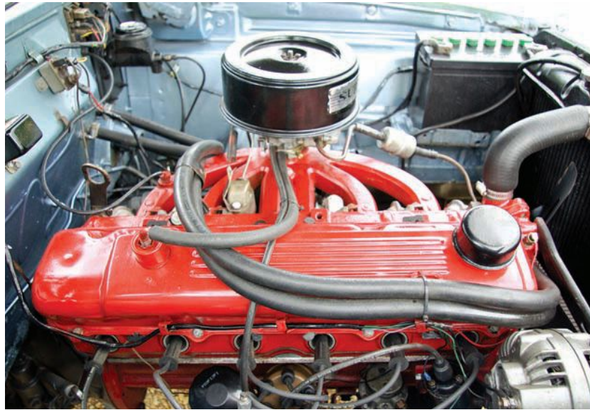
Slant-Six engine was rebuilt in 2003 after providing nearly 300,000 miles of reliable service. Now overbored to 238 cu.in. and fitted with dual exhausts, it has a lot more get-up-and-go.
