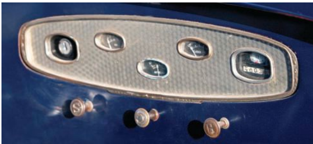
All is as should be inside the Phaeton's interior, save for that overdrive knob. To allow a top speed greater than 40 MPH, the owner installed a mid-1950s Dodge overdrive unit. With a .70 overdrive gear, this knocked the final drive ratio from 4.9:1 down to a reasonable 3.43:1.
