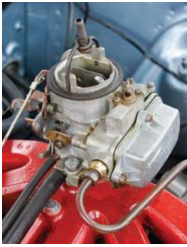
Slant-Six engine was rebuilt in 2003 after providing nearly 300,000 miles of reliable service. Now overbored to 238 cu.in. and fitted with dual exhausts, it has a lot more get-up-and-go.
