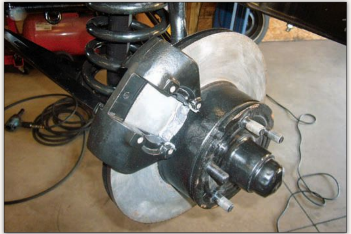
Having been originally equipped with the optional power front disc brake system from the factory, new replacement components were obtained and installed while the chassis was being restored. The system required Matt to hunt for proper wheels as well.
