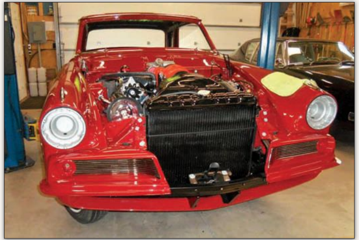
Front end reassembly is well underway, including the installation of the front fenders. New wiring is already in place, as is a refurbished radiator. Chrome trim and the front bumper, already restored, are next on the list to reinstall.
