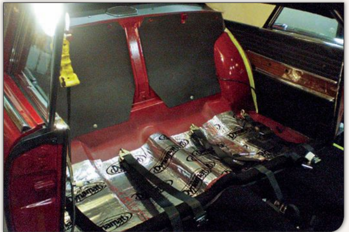
Here, the rear side interior panels have already been installed. Note the one upgrade that will ultimately be hidden by carpet and seating: the Dynamat sound deadening mat on the floorpan. As the product implies, it decreases noise transfer into the cabin.
