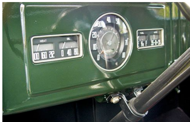
A three-speed transmission was standard, but this long-wheelbase one-ton was equipped with a rugged non-synchromesh four-speed. Spartan dash includes optimistic 80mph speedometer flanked by gauges for engine temperature, oil pressure, fuel level and amps.
