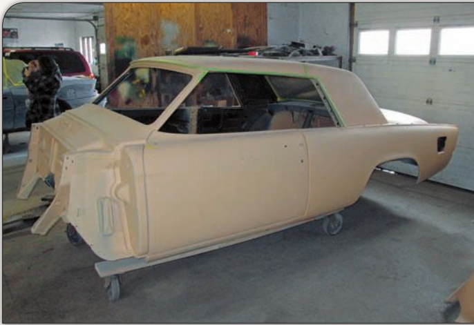
With the filler work completed and sanded smooth, several layers of primer were applied and allowed to cure between coats to help ward off unwanted shrinking. Each coat was also sanded in order to achieve a superiorly smooth surface for paint.
