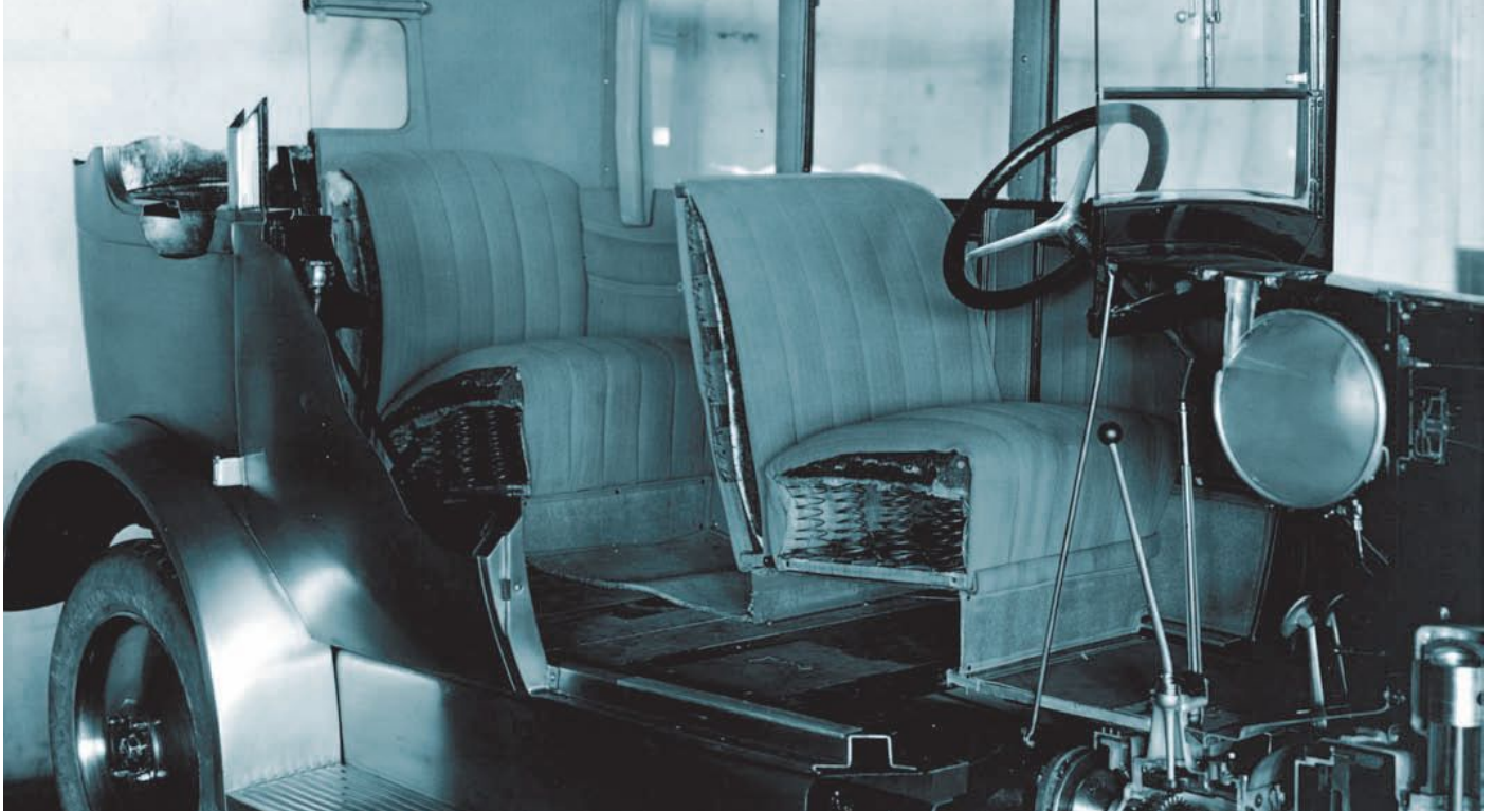
This three-dimensional cutaway clearly illustrated exactly how the well made stamped-steel panels of the body were constructed. Precise welding techniques joined the individually stamped pieces together to form a rigid body, free of rattles.
