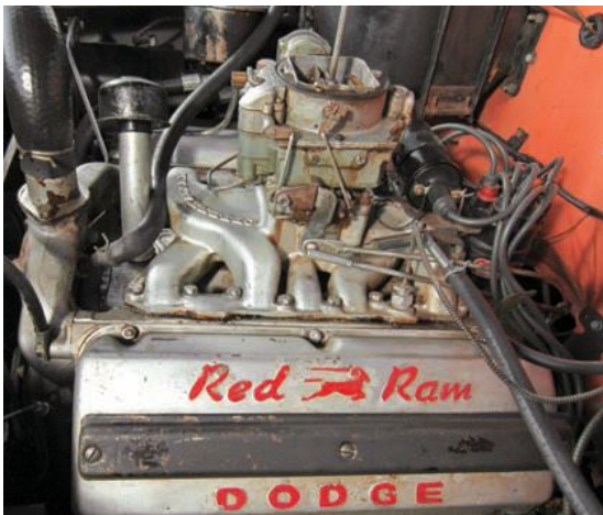
Red Ram Hemi V-8 was a 241-cu.in. little brother to the Chrysler’s FirePower 331 engine. With the dealer-installed Offenhauser intake and four-barrel carburetor, the Red Ram produces 170 horsepower.
