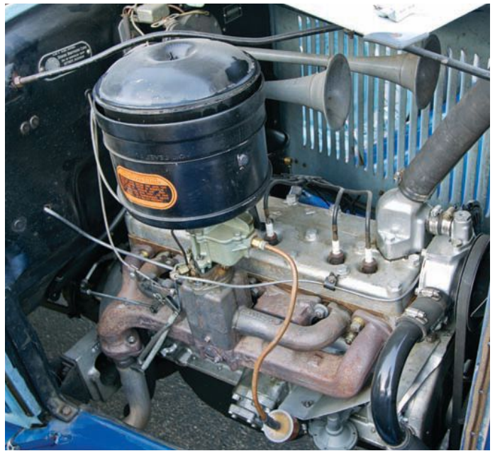
Dodge's cast-iron flathead six displaced 189.8 cubic inches, offered 5.2:1 compression, and developed 61 horsepower in 1930. To make this Phaeton more roadable, the owner swapped in an externally identical 217-cu.in. L-head six (with 6.2:1 compression) from a 1941 Dodge. This bumped power up by a third, to 91 horsepower.
