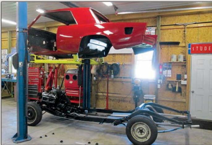
After the paint cured and the body was returned, it was positioned on a two-post lift before it was carefully lowered to the completed chassis. Using new mounting parts, the two were finally reunited after several months.
