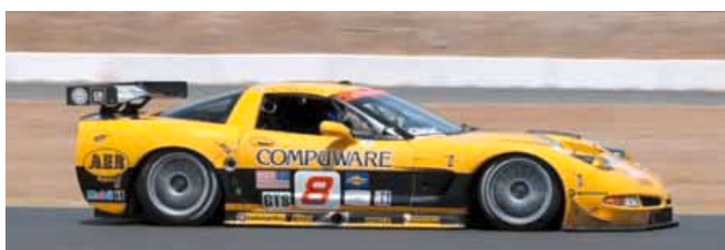
GM's new C6-R sportscar features exterior design changes and a 7-litre small block V8
