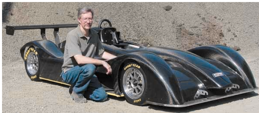
Lee Stohr with his semi-monocoque DSR which uses a part steel, part carbon fibre construction. Here with carbon body
