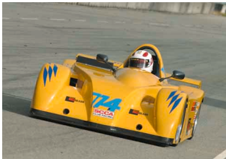
The traxStar DSR carries its motorcycle powerplant beside the driver, offsetting the cockpit to the right side of the car
