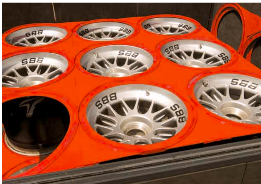
Motorsport wheels have traditionally been manufactured from magnesium to take advantage of its weight saving properties
