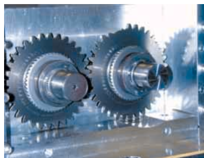
Xtrac tests scale model versions of all its gears to failure on its 'foursquare rig'. This has enabled it to gain valuable information on different materials and heat treatments
