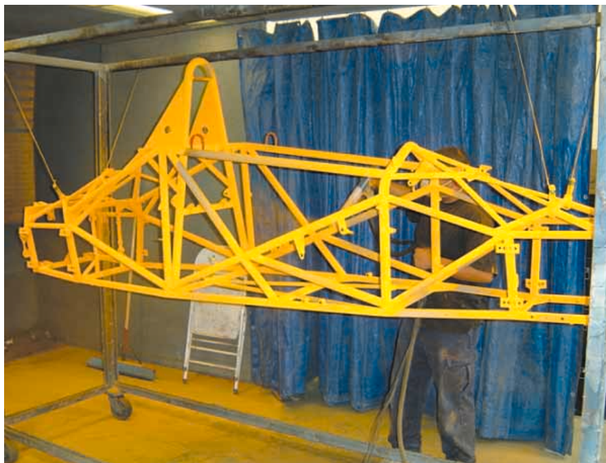
Maloy frames are powder coated in bright yellow to aid crack detection after races and when repairing crash damage
