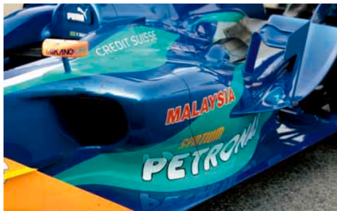
Sauber again utilises its 'folding' radiators, with extreme sidepod undercuts
