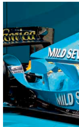
Enlarged chimneys over 2004 car re-direct airflow more effectively from the radiators up over the intermediate and rear wings
