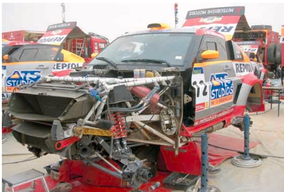
To improve dynamics, this year Mitsubishi mounted its 4.0-litre V6 engine 11cm lower and 5cm further back in the chassis
