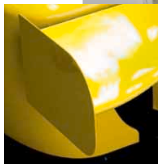
Examples are smaller rear end plates and unusual winglets above the radiator intakes (shown left)
