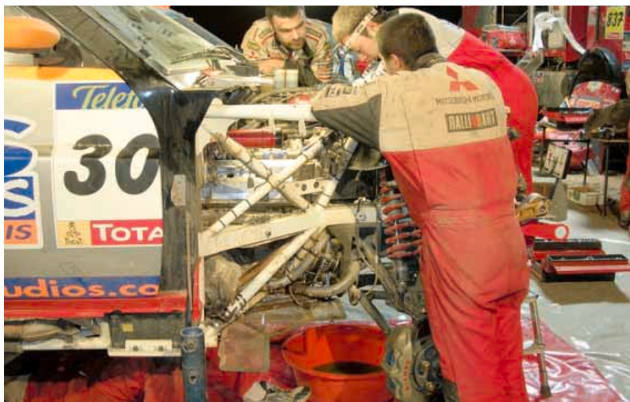
To improve dynamics, this year Mitsubishi mounted its 4.0-litre V6 engine 11cm lower and 5cm further back in the chassis
