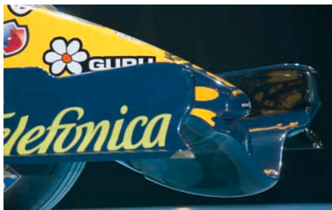
Aside from an innovative 'v-keel' arrangement, car is an evolution of R24
