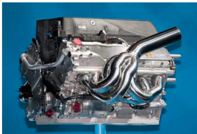
Renault sticks with a 72-degree bank angle but otherwise the RS25 is new
