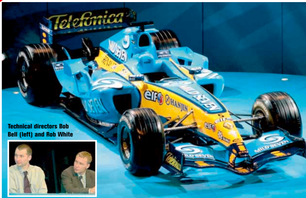
Enlarged chimneys over 2004 car re-direct airflow more effectively from the radiators up over the intermediate and rear wings
