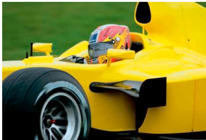
Unusual winglets above the radiator intakes seen at Silverstone in practice
