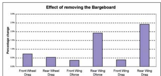
Figure 3: percentage changes to aerodynamic forces on wheels and wings
