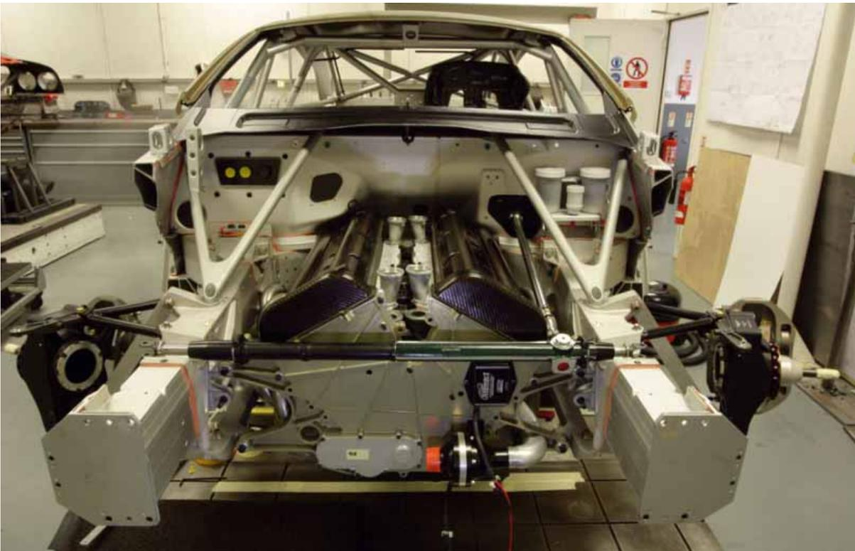
GT regulations forbid moving the bulkhead itself but the DBR9's favourable engine bay layout means engines can be located further back and lower in the chassis than some of its competitors
