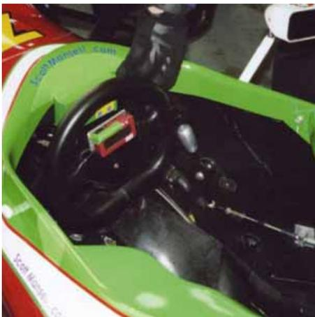
There are no hydraulic and electronic systems on Mansell car, so paddle shift has been replaced with conventional mechanical sequential shift
