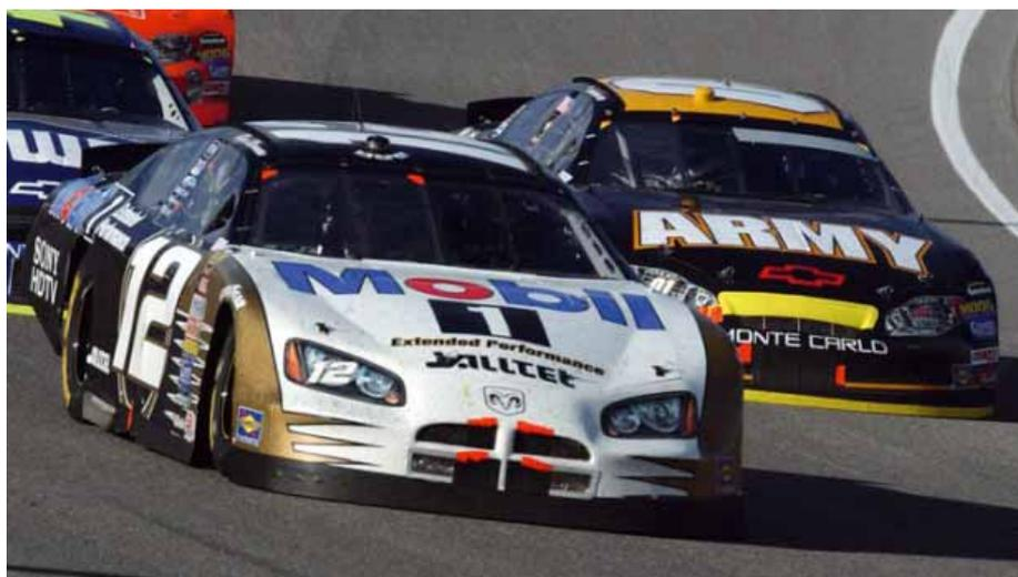
Left: with such tight regulations and so few differences in silhouette shapes, specific aero details such as the front splitter shown on the Dodge (left) are vital to front running teams
