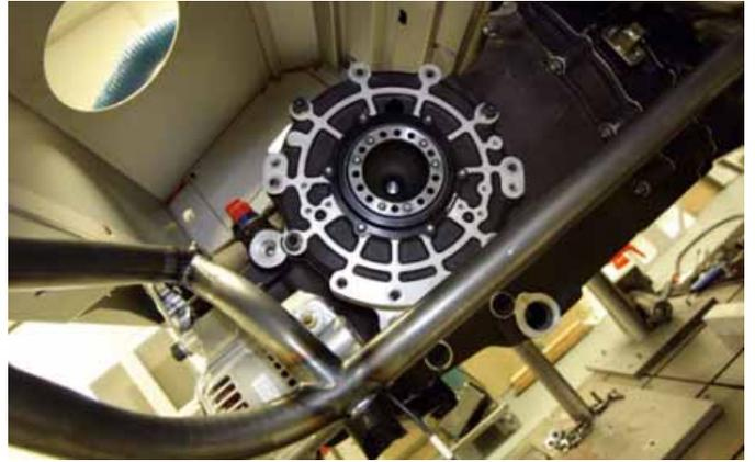
Six-speed, sequential Xtrac gearbox is mounted longitudinally at the rear axle
