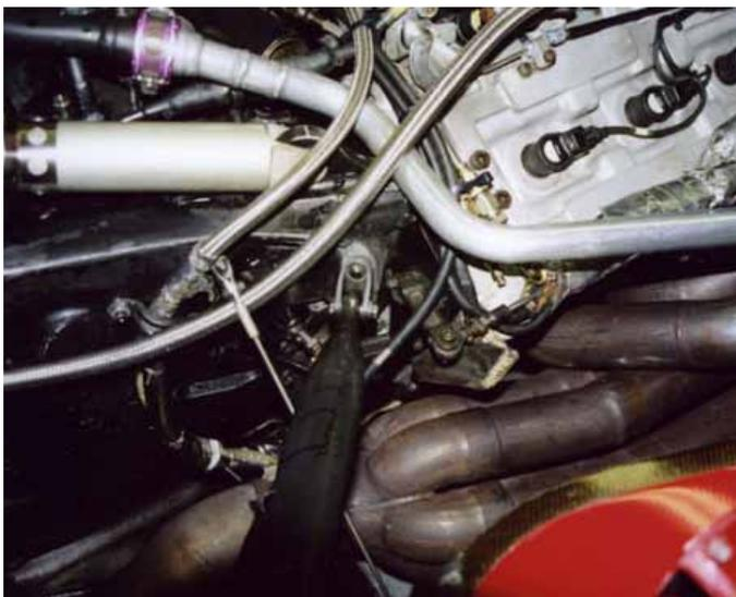
Mounting the Judd engine necessitated the use of a special gearbox adapter, which in turn forced some re-engineering of the rear suspension pick-ups
