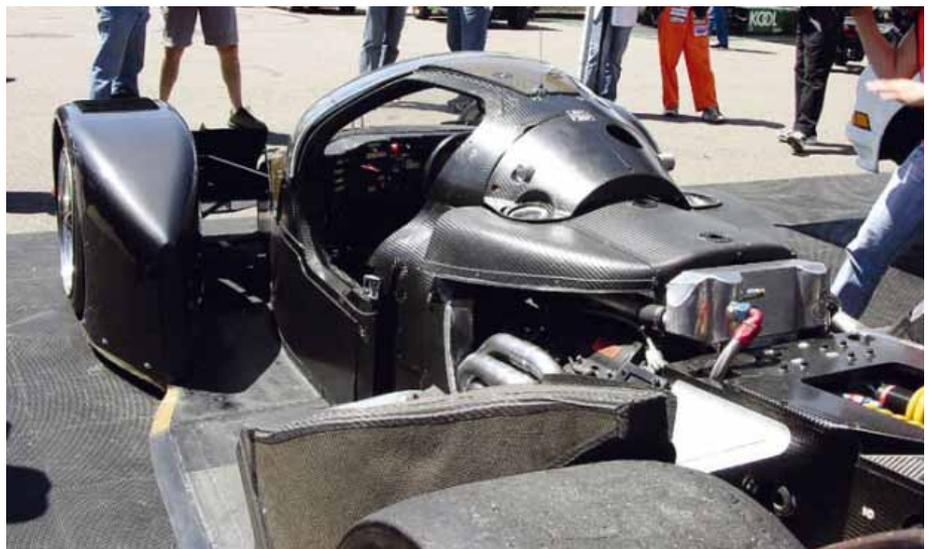
Originally designed to use a small block Chevy, the J2X was built with a Group C compliant Cosworth DFR
