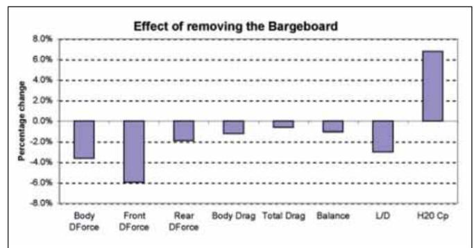
Figure 2: percentage changes to overall aerodynamic forces
