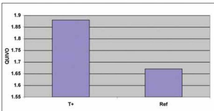
Figure 12: 'QUIVO' indicator showing the gain in front axle behaviour following the front toe-out reduction
