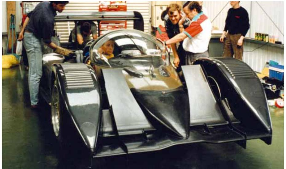
Front wing design, with its secondary flaps between the wings, was way ahead of its time, and worked too
