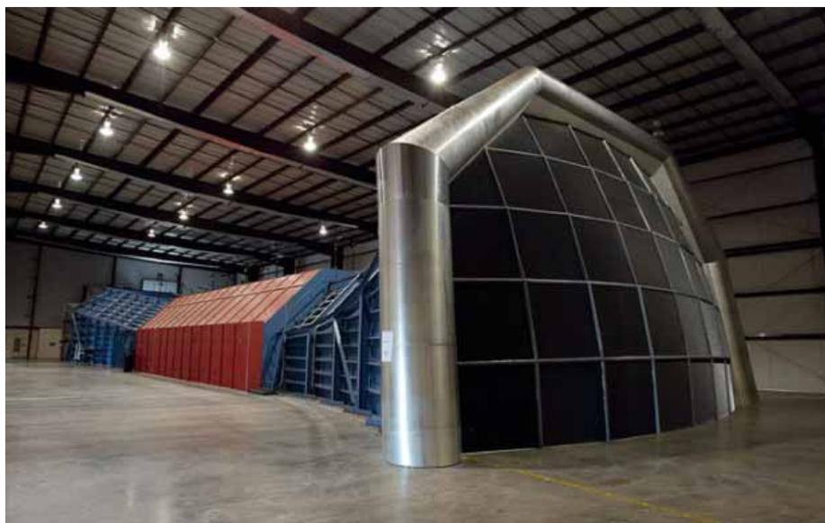
Standing alone in a large warehouse the AeroDyn facility works as an open return system
