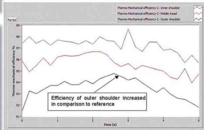
Figure 10: measurements of the thermo-mechanical efficiency of the loaded front tyre after camber reduction
