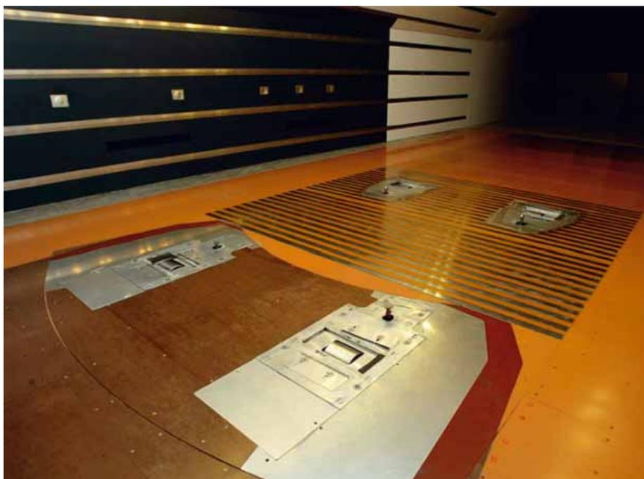
**Boundary layer system uses suction and tangential blowing through precise holes and sprung steel strips**
