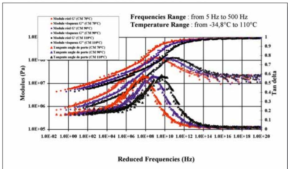
Figure 5: a typical thermo-mechanical analysis plot from a test subject tyre
