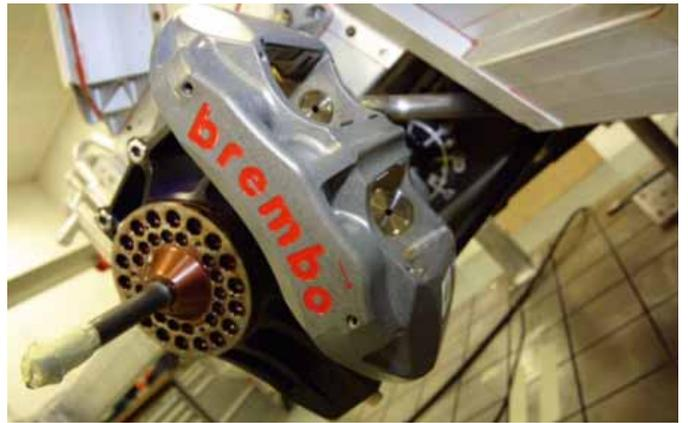
Six pot calipers and carbon discs as standard, though a steel option is offered
