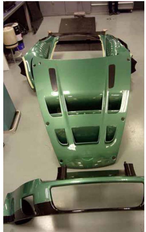
Carbon fibre composite panels laid out ready for use – only the roof of the DBR9 is still made from aluminium
