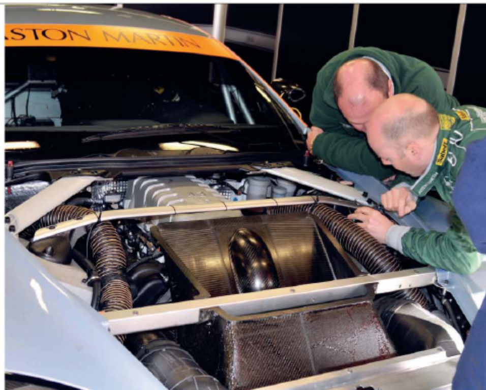
To keep costs down, the engine is a bored-out version of the stock 4.3-litre, aluminium V8, now displacing 4.5-litres
