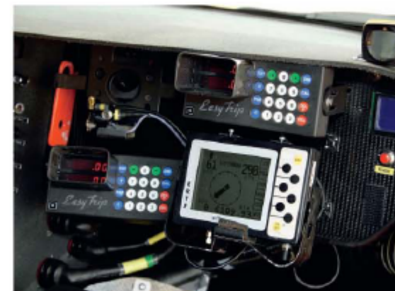
With the Dakar route taking in some of the most remote and inhospitable places on earth, satellite navigation and GPS technology is de rigueur. A brace of rally trip meters ensure accurate measurement of stage times and distances
