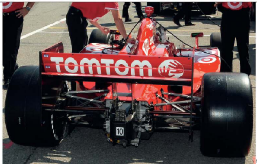
Dario Franchitti's Ganassi Racing Dallara Indy Car finished third at Mid-Ohio fitted with Penske's regressive dampers
