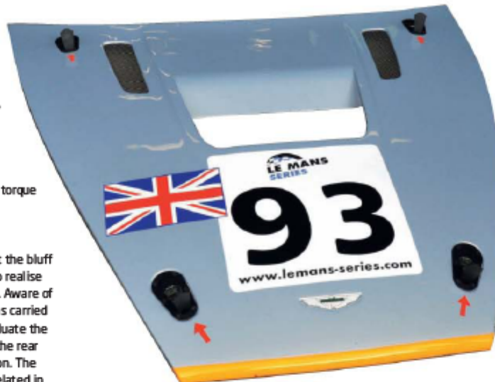
Due to its smaller overall size and overhangs, a special cooling package was allowed that exits through the carbon fibre bonnet
