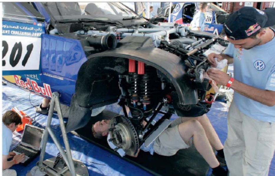
Front suspension uses twin damper / spring units for safety and to share the immense forces encountered across a wider area. A revised damper hydraulic system was developed in conjunction with technology partner ZF Sachs
