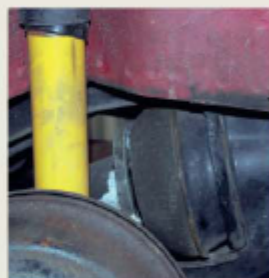
The original Mini's rubber cone suspension - no wonder the driving experience has often been likened to driving a trailer!
