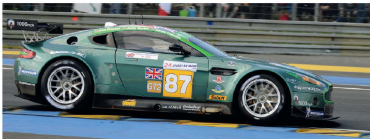
The Vantage GT2 bodyshell is almost entirely carbon fibre, with a CFD-designed GT1 rear wing, flat floor and a simplified version of the DBR9 GT1 rollcage
