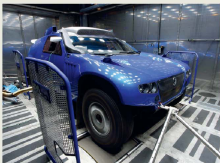
VW's environmental chamber was vital in ensuring RT2's performance didn't suffer at high altitude
