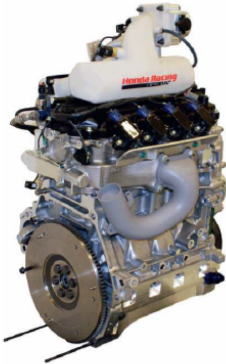
Honda's alternative to the Kent Formula Ford engine is this 1500cc unit, developed by HPD and Quicksilver RacEngines
