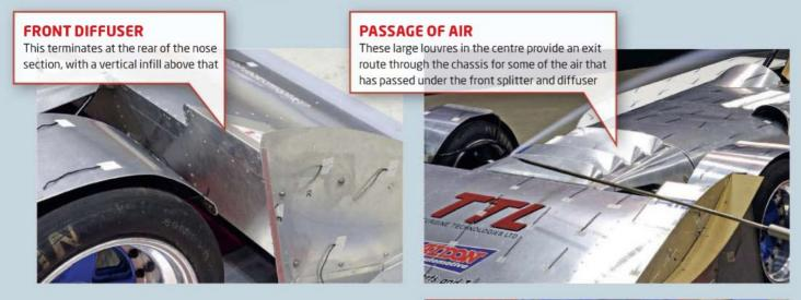
the centre section, attached to the chassis is a secondary splitter with a radiused leading edge and a faired cowling channelling air sideways and upwards. Small trim tabs on the upper trailing edge of the nose are also present, offering three adjustments: high, low and absent.
