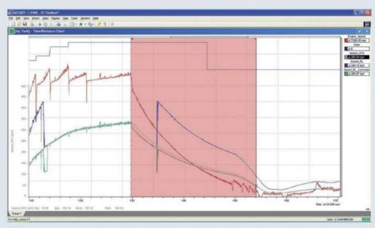
Image 3: overlaying the two traces we can see the speed trace from the hub drops off the moment the power is released and then gradually trends toward the same value as the GPS signal over the course of the deceleration
