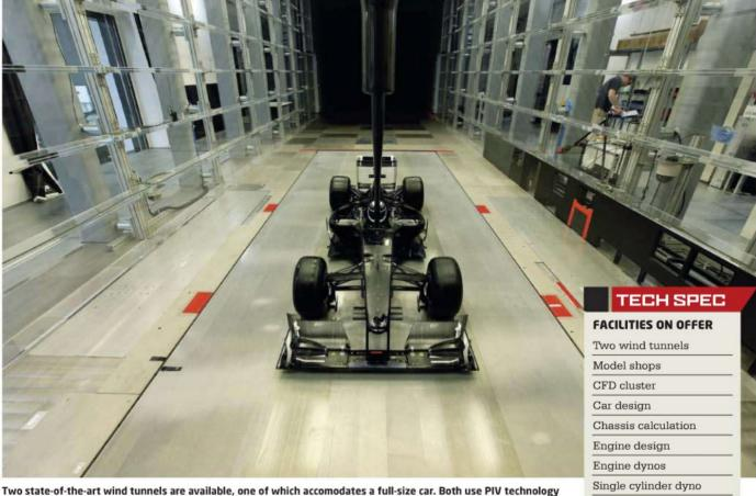
ith more than 30 km2 of floor space, two wind tunnels and a mind-boggling array of research and development equipment the Toyota Motorsport facility in Cologne-Marsdorf, Germany could be considered a motorsport engineer's dream. Only a dream because it was off limits to anyone outside of the Toyota works World Rally, Le Mans and Formula 1 programmes, but the facility is now available to customers.
