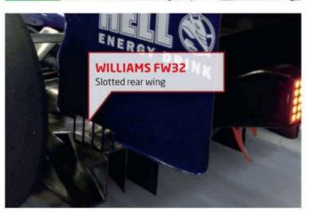
of its blown rear wing assembly. This wing takes the 15cm slot inlet in the front of the main plan and diverges to span the full width of the wing. The team even went so far as to conduct tests with flow visualisation paint applied, to show the complex surface flow under the wing.
