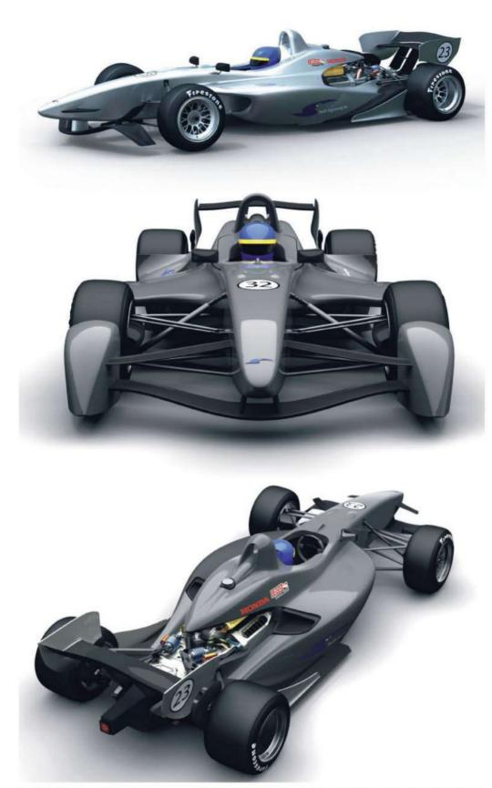
Swift's designs are all based on the proven 017.N Formula Nippon monocoque and feature a number of popular design elements such as an exposed engine and information lights, which let fans know car position and fuel load. One thing that may go against Swift is its intention to build the cars in California instead of Indianapolis
