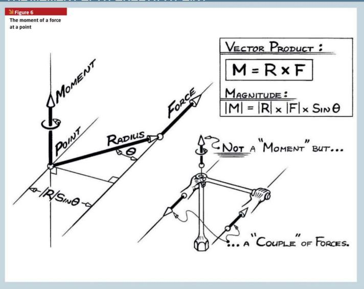
6 we see that wherever we slide force F along its line of action, it always gives the same moment M at the arbitrary point P. The vector product and its moment can replace the second axiom of statics given earlier. Modern vector theory is used in many different fields besides mechanics, such as structural engineering, aerodynamics, electrodynamics, quantum theory and more. So moments are at the core of much of modern engineering and science.
