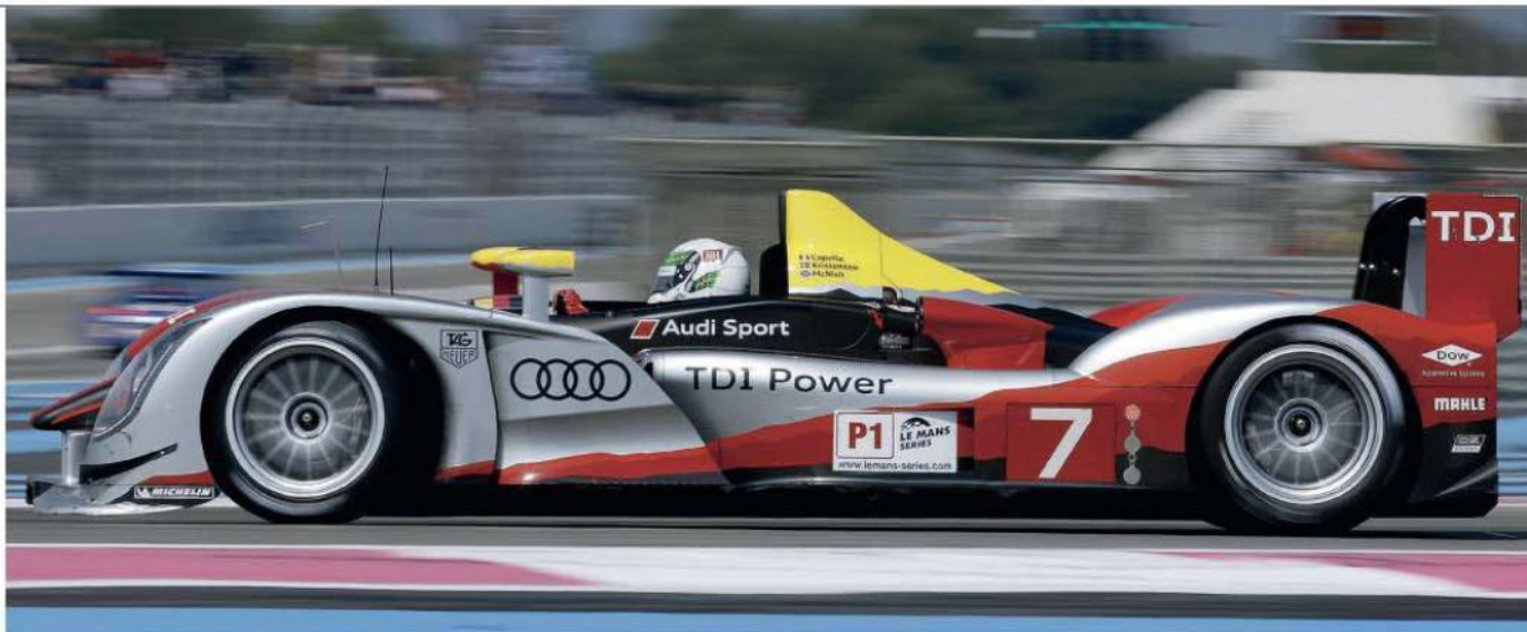
The 2010 Audi ( above ) has far more conventional bodywork compared to the 2009 version ( below ). Gone are the dramatic louvres on the side pods and the rear wing sits further back
