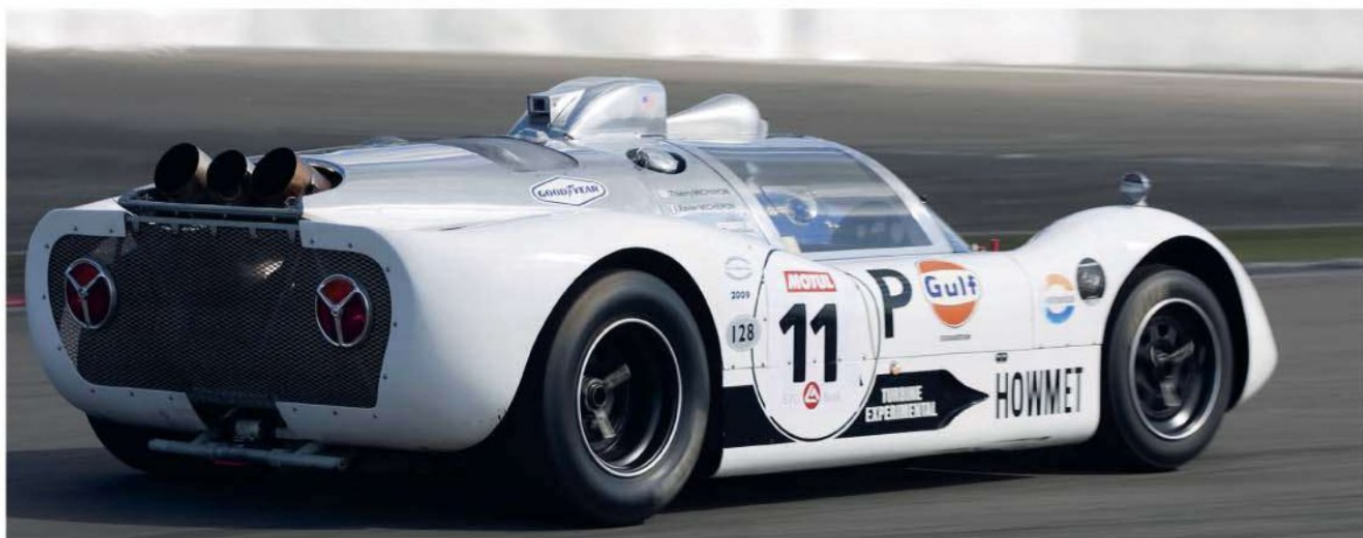
Body was made from a combination of glass fibre and aluminium, the aluminium parts left bare to showcase the products manufactured by Howmet Corp
