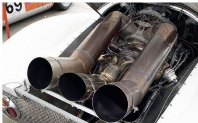
...as the throttle pedal is depressed further, air is fed to the second turbine
