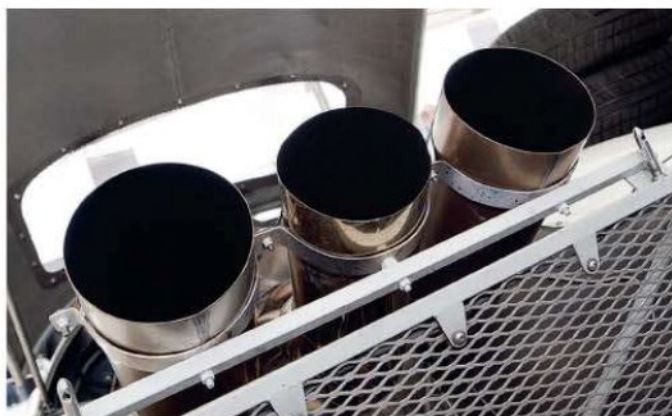
At idle, all of the compressed air is fired out of the central exhaust then...
