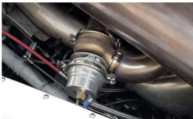
Key to the car's driveability is the wastegates that control the gas flowing between the gas-generating turbine and the power-generating turbine
