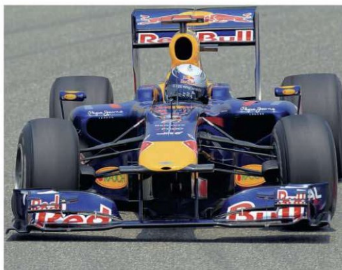
Red Bull's simplified front end aero, used in conjunction with a new floor
