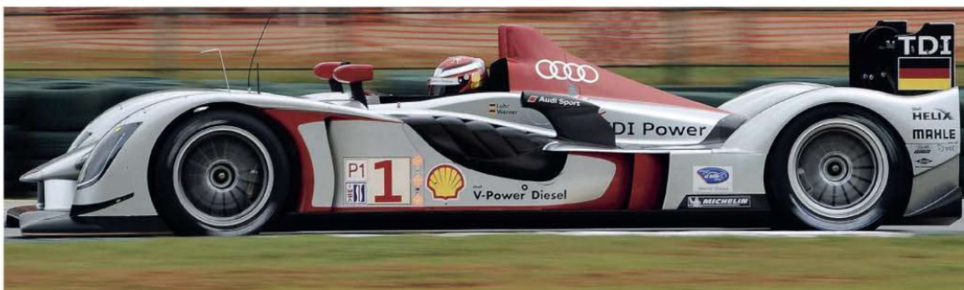
The 2010 Audi ( above ) has far more conventional bodywork compared to the 2009 version ( below ). Gone are the dramatic louvres on the side pods and the rear wing sits further back
