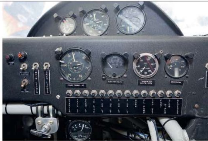
The car's control panel came directly from a turbine-engined helicopter
