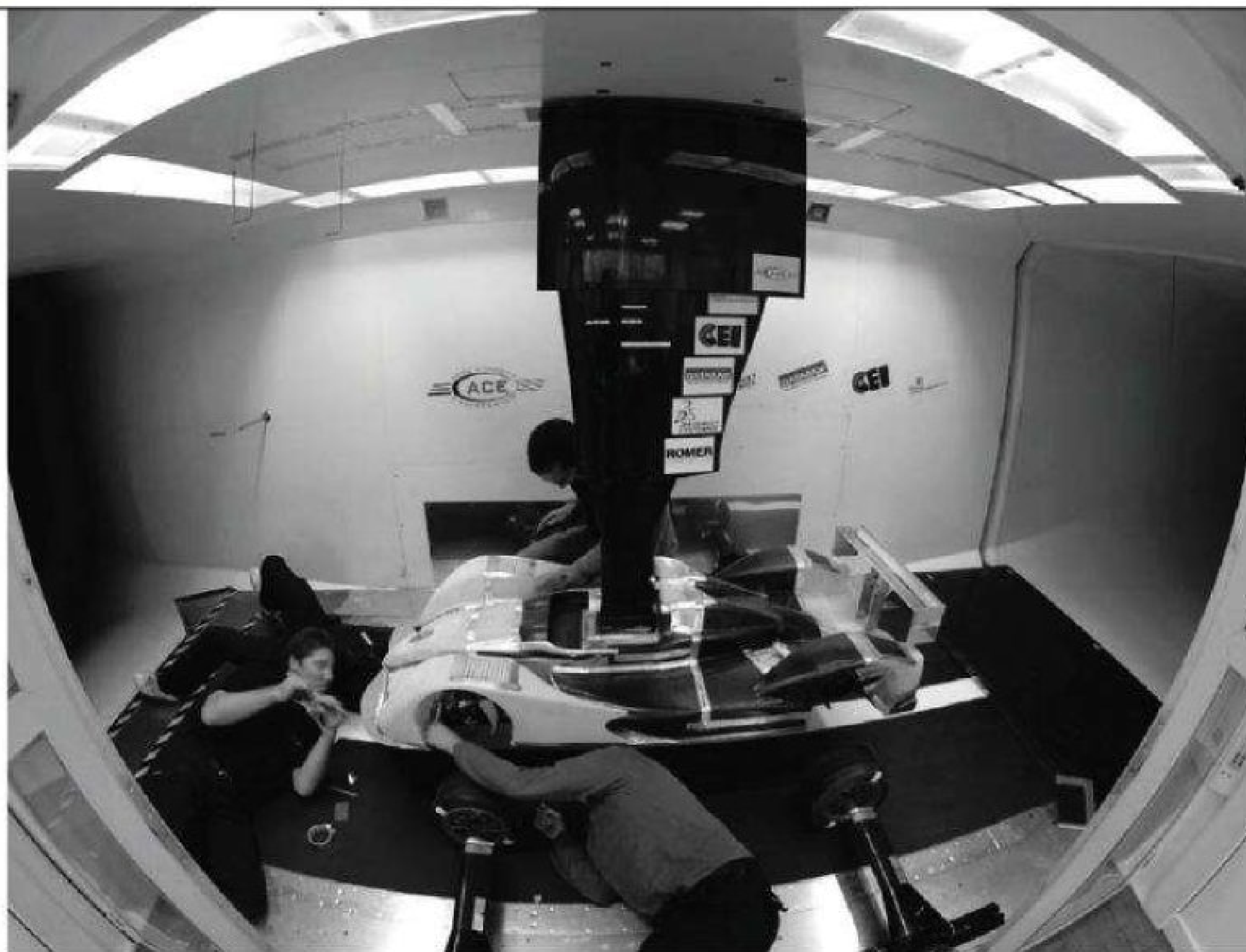
The revised bodywork was developed in the Aero Concept Engineering scale wind tunnel at Magny Cours, France
