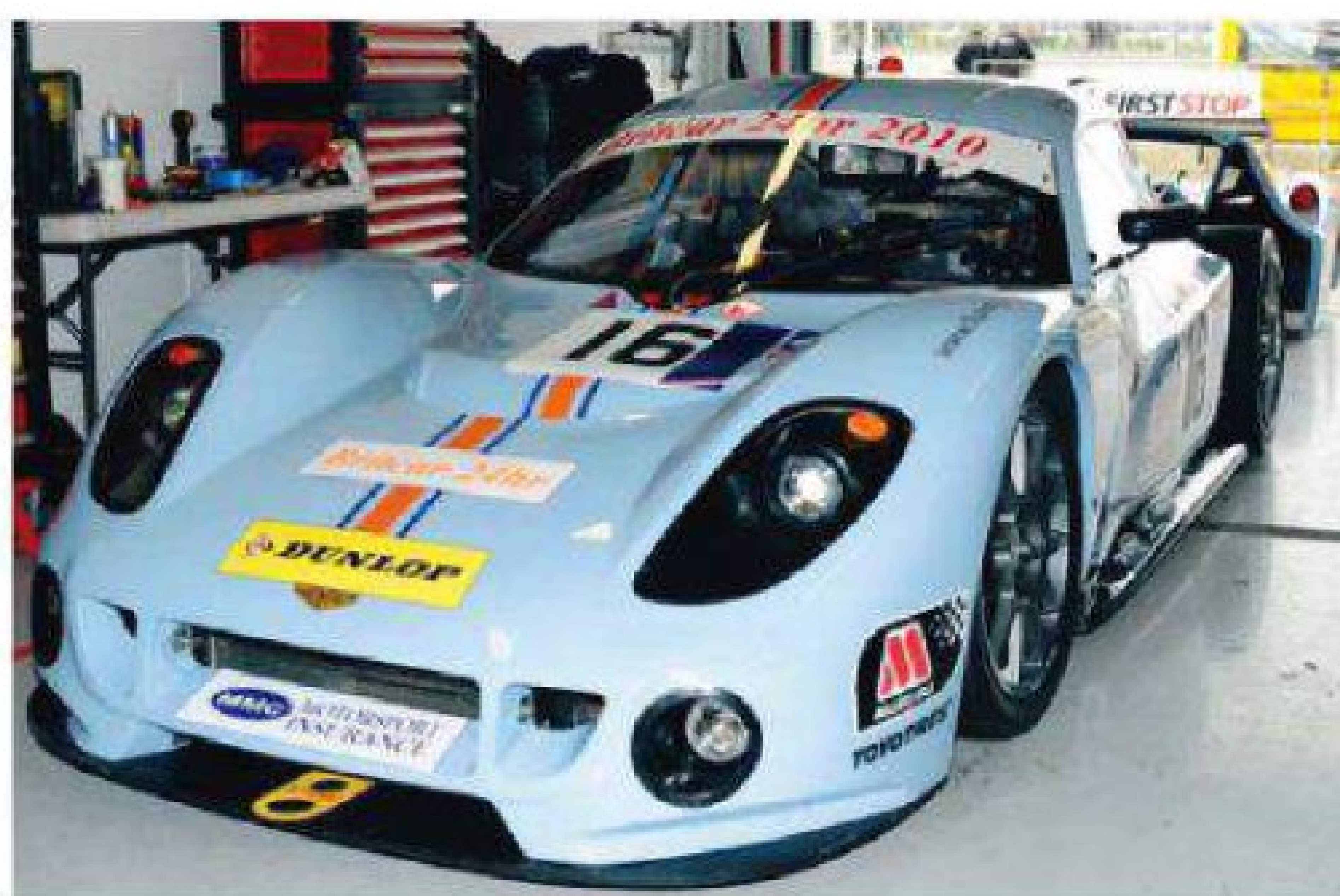
Bodywork was styled by Lester Allan and made from a foam buck cut by Bakers Patterns. The GT-spec car was down to aerodynamicist Frank Doyen
