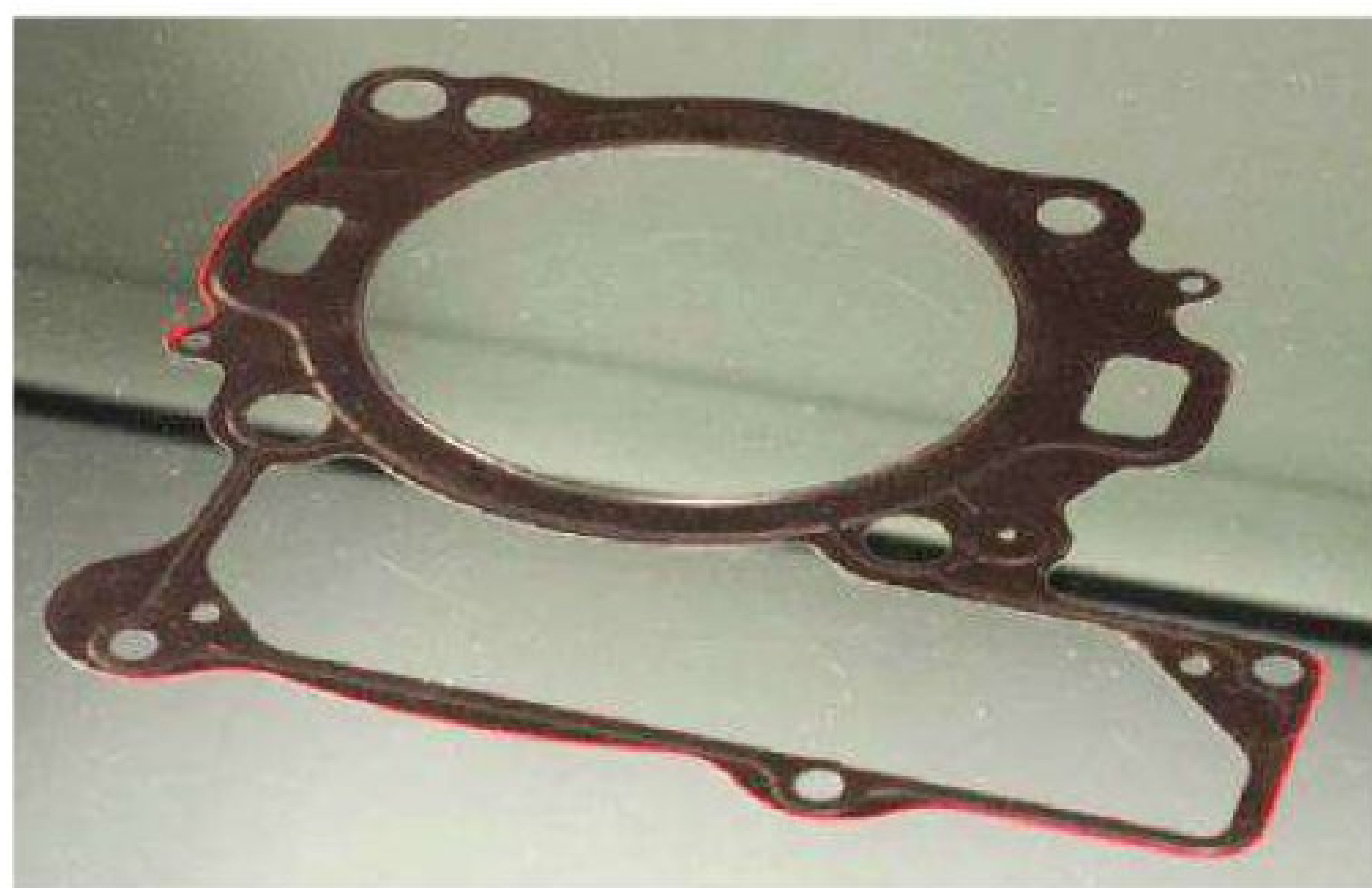
Less layers means less interaction and less friction, plus better repeatability
