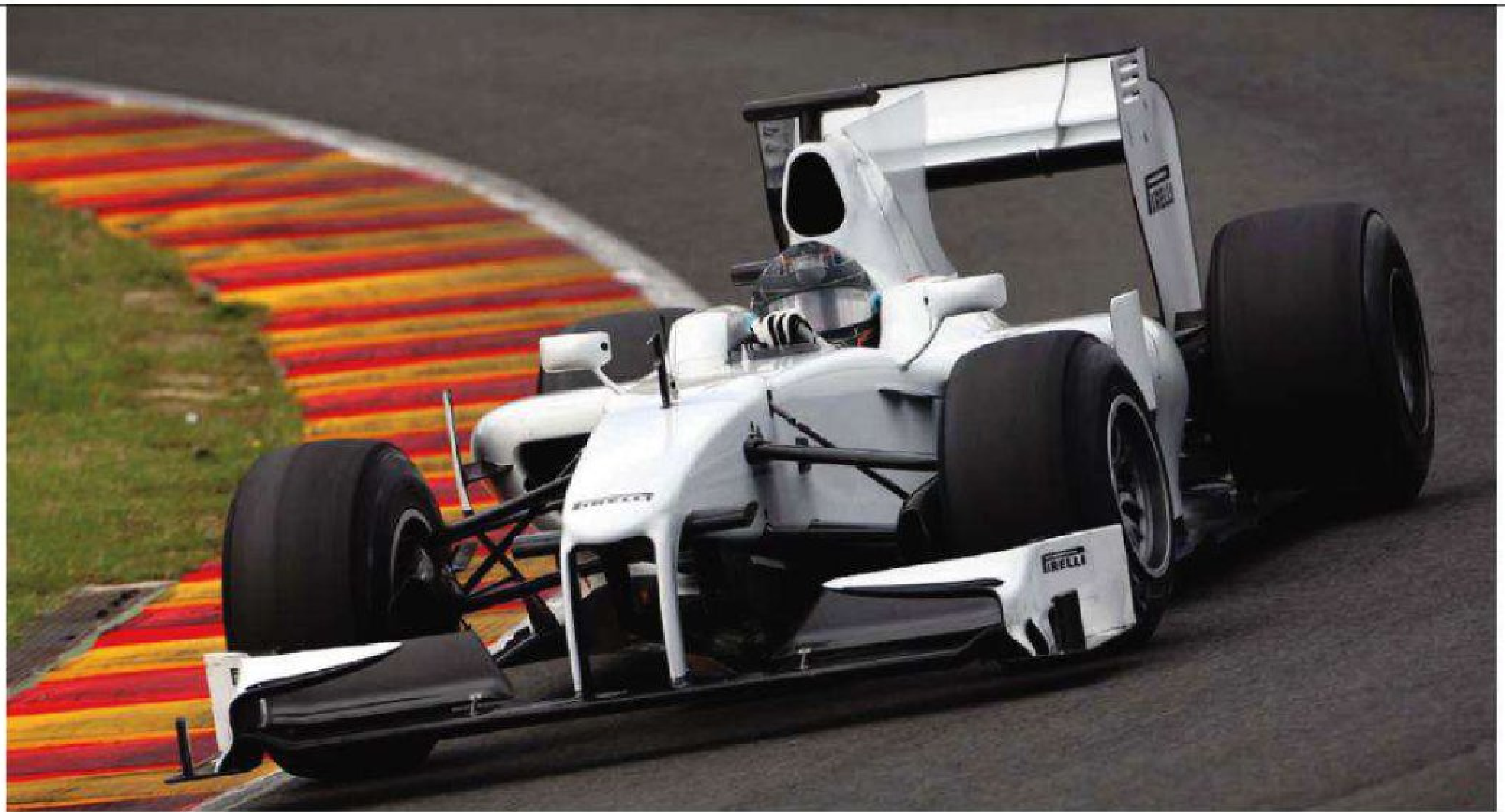
The proven Toyota TF109 was chosen as the test car to develop the tyres. It was modified by Toyota engineers to replicate the dynamics of the 2010 models
