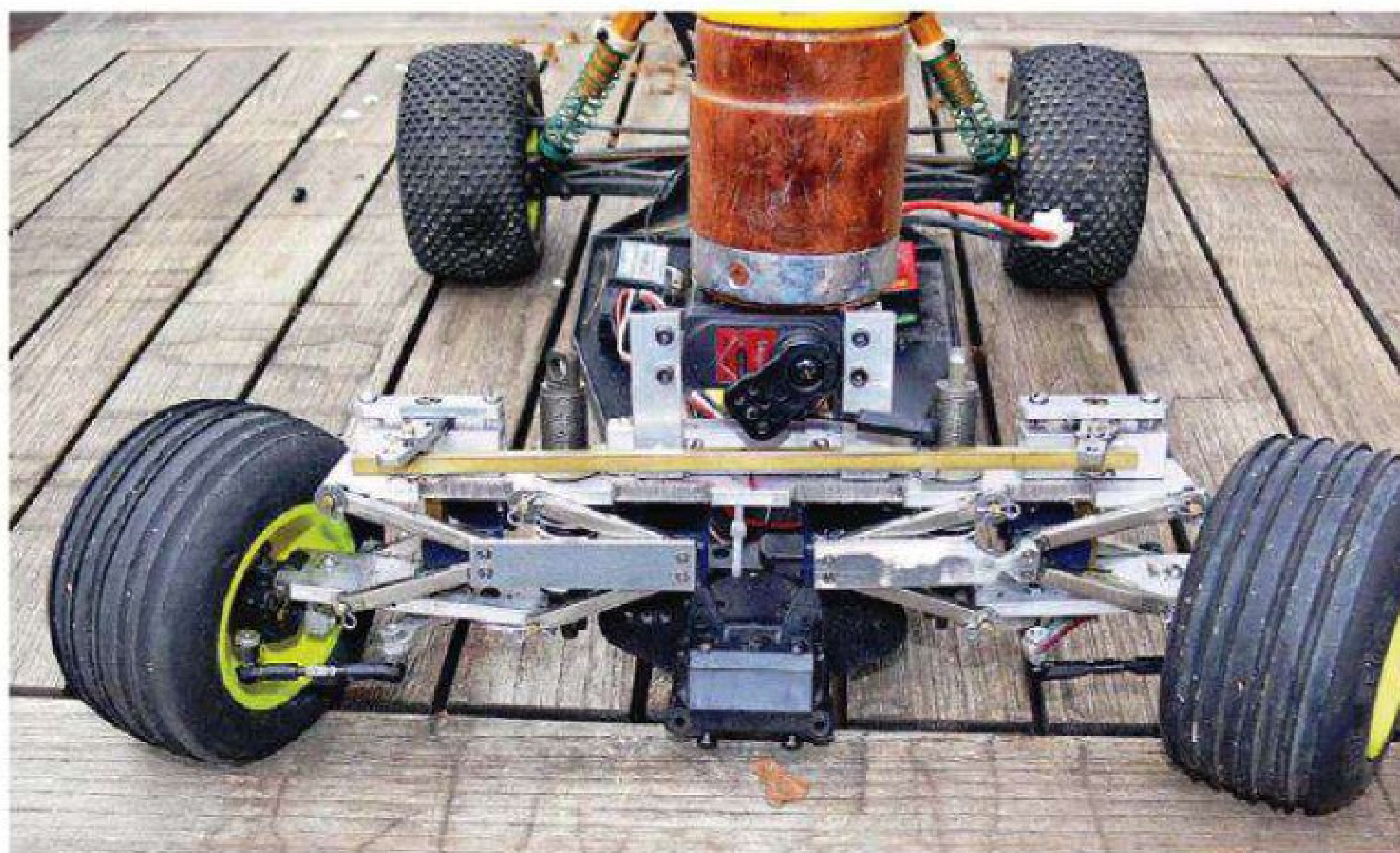
Prototype no 1 with load applied centrally, and steering lock applied
