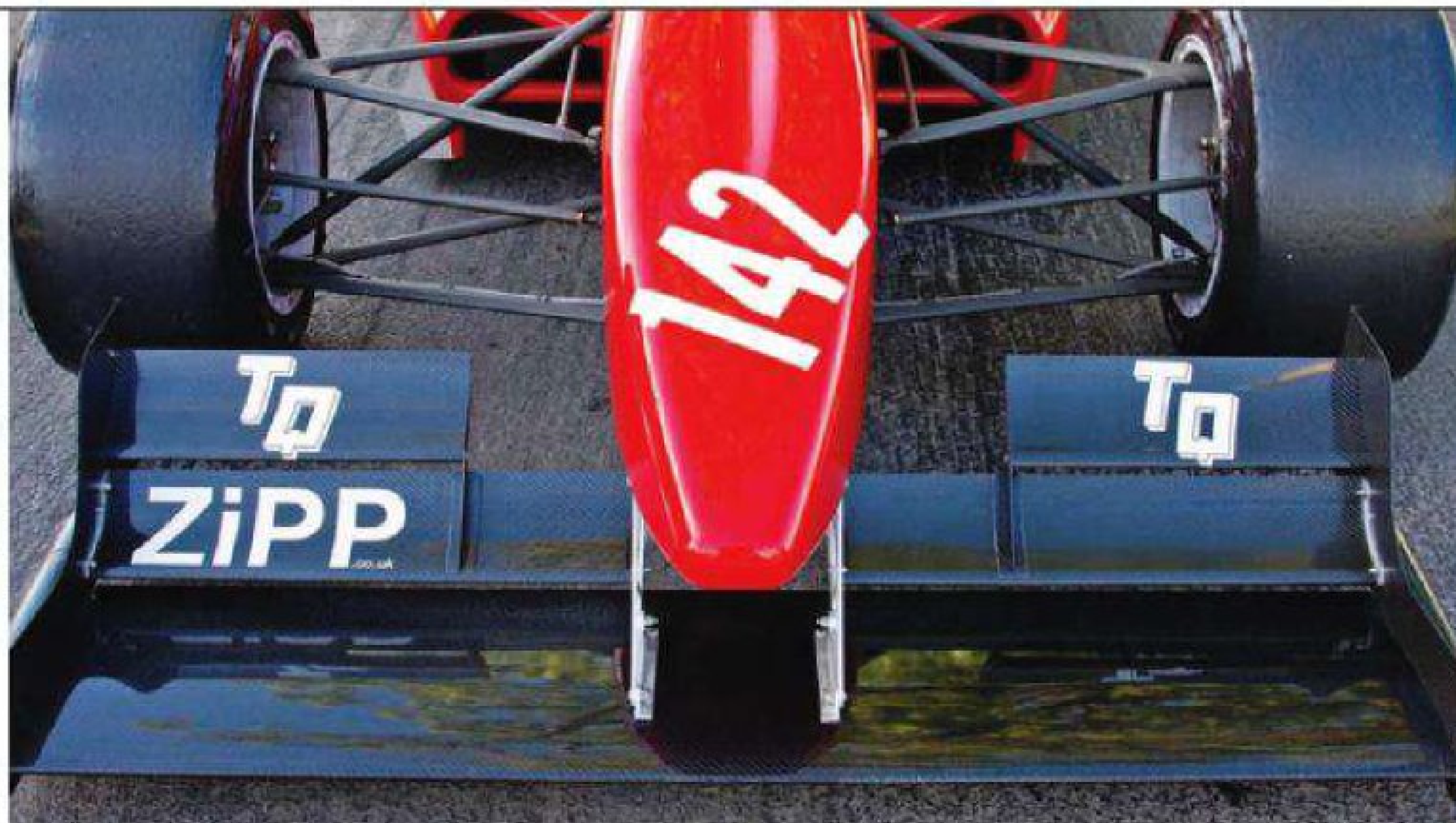
The Firestorm's aero package has been gradually developed throughout 2010. The potent triple element front wing (above) was balanced with a more potent upper tier on the double tier, dual element rear wing. Gills and louvres (bottom) aid heat rejection at the rear
