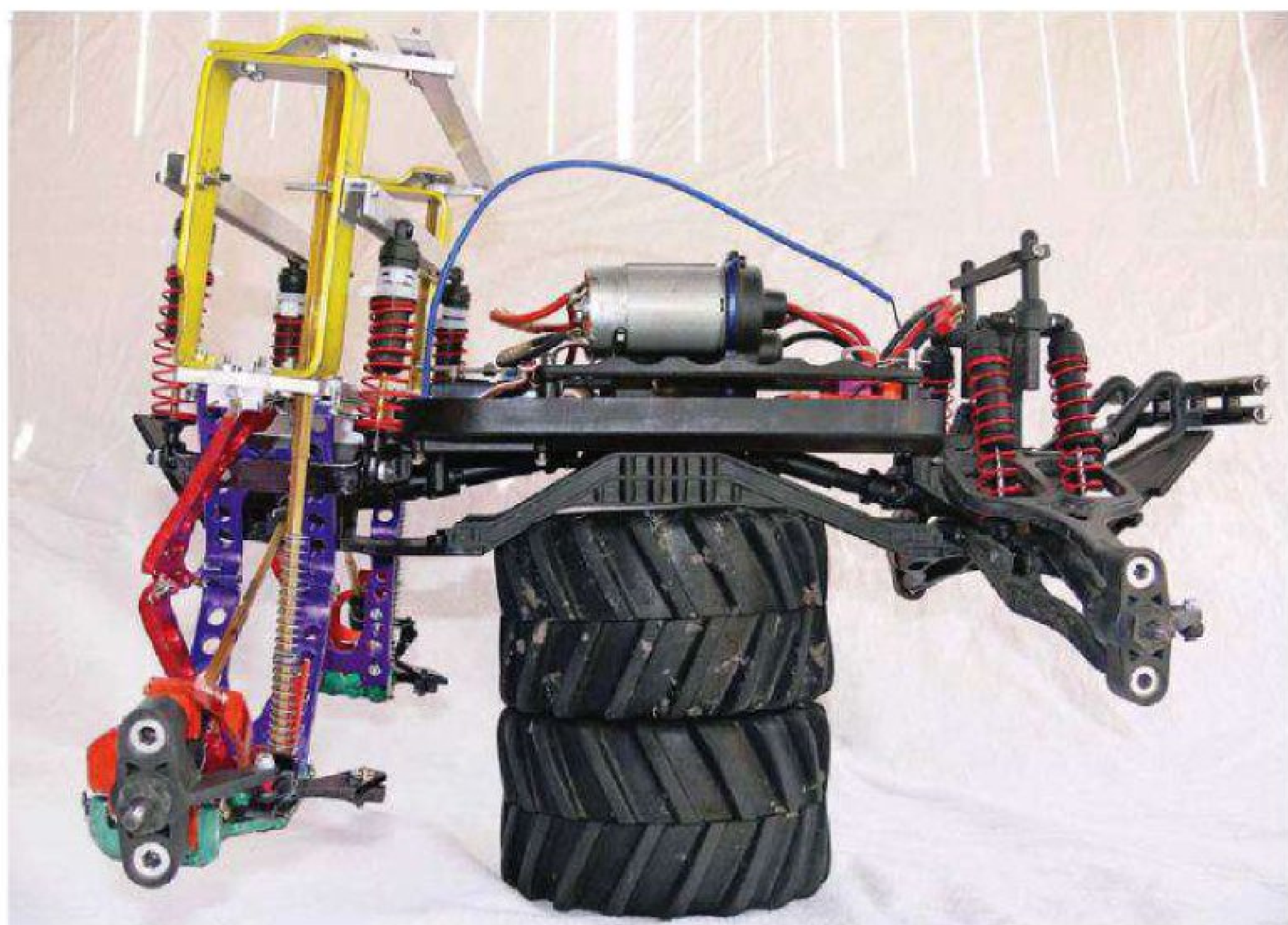
From the side, it is possible to see just how much suspension travel the VXI system has allowed on prototype no 2. Compare the travel of the front VXI set up with the standard SLA double wishbone suspension at the rear
