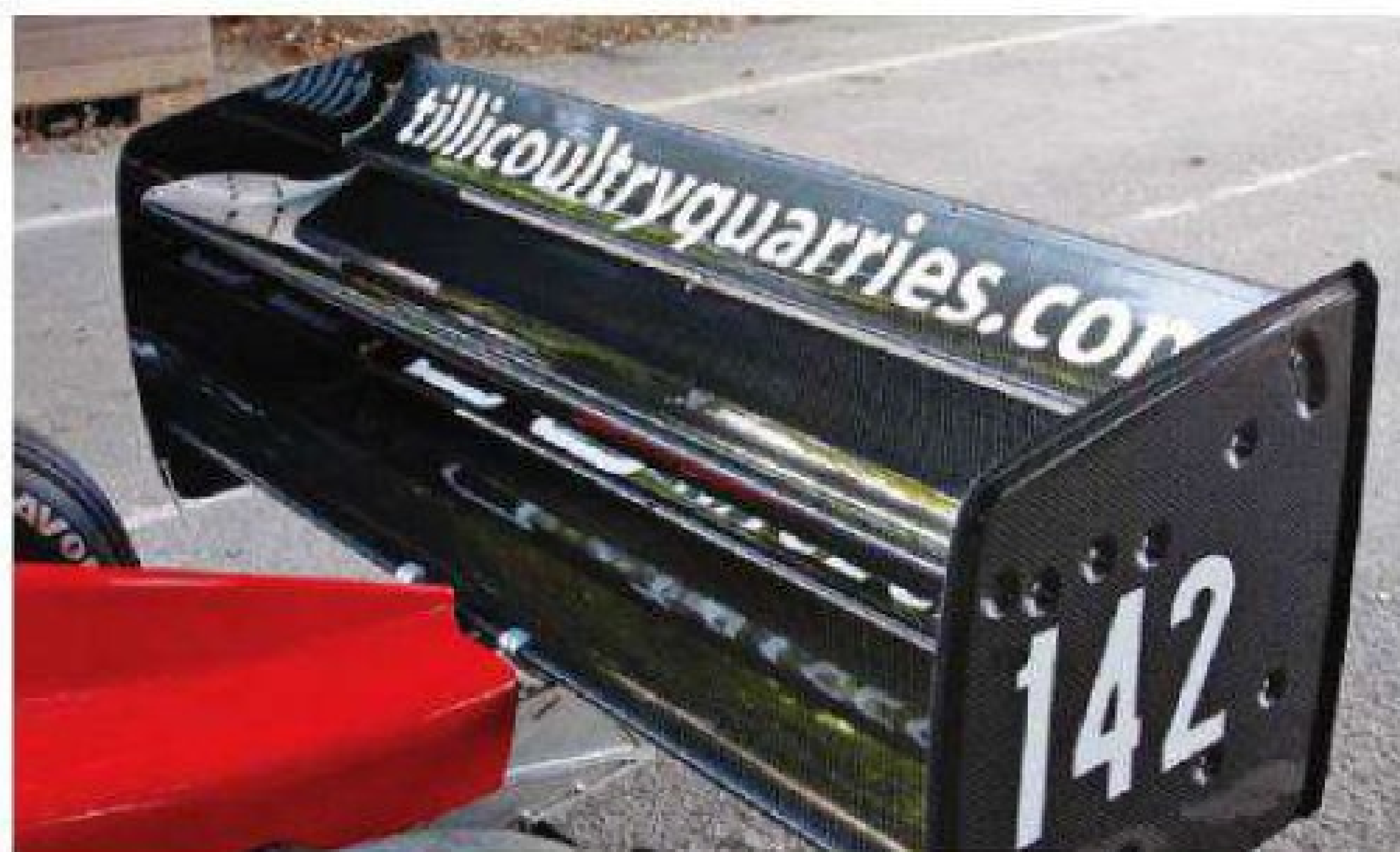
The Firestorm's aero package has been gradually developed throughout 2010. The potent triple element front wing (above) was balanced with a more potent upper tier on the double tier, dual element rear wing. Gills and louvres (bottom) aid heat rejection at the rear
