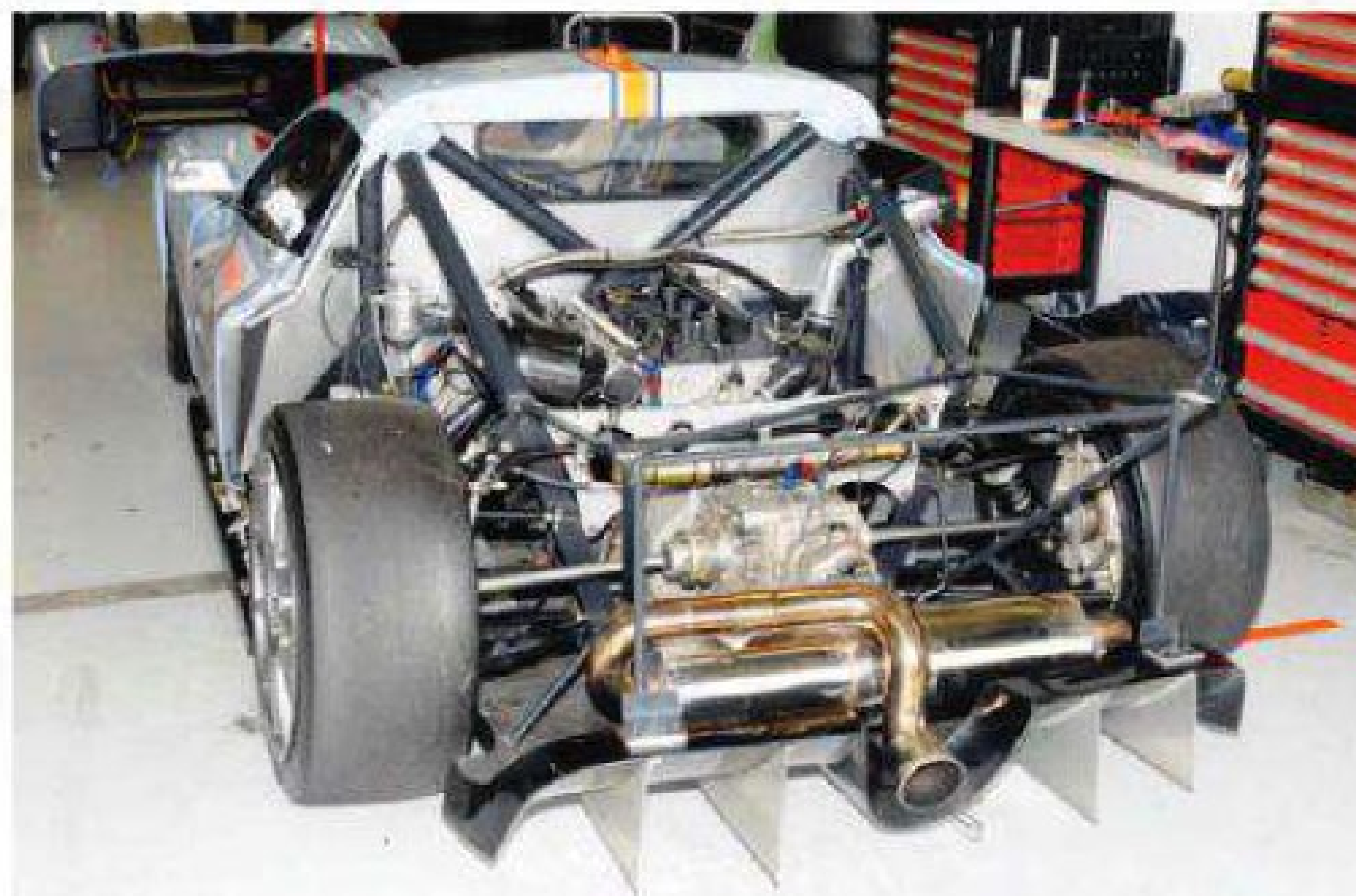
A mid-mounted, 2.0-litre, four cylinder Cosworth YD engine provides the power, hooked up to a Hewland JFR five-speed sequential transmission
