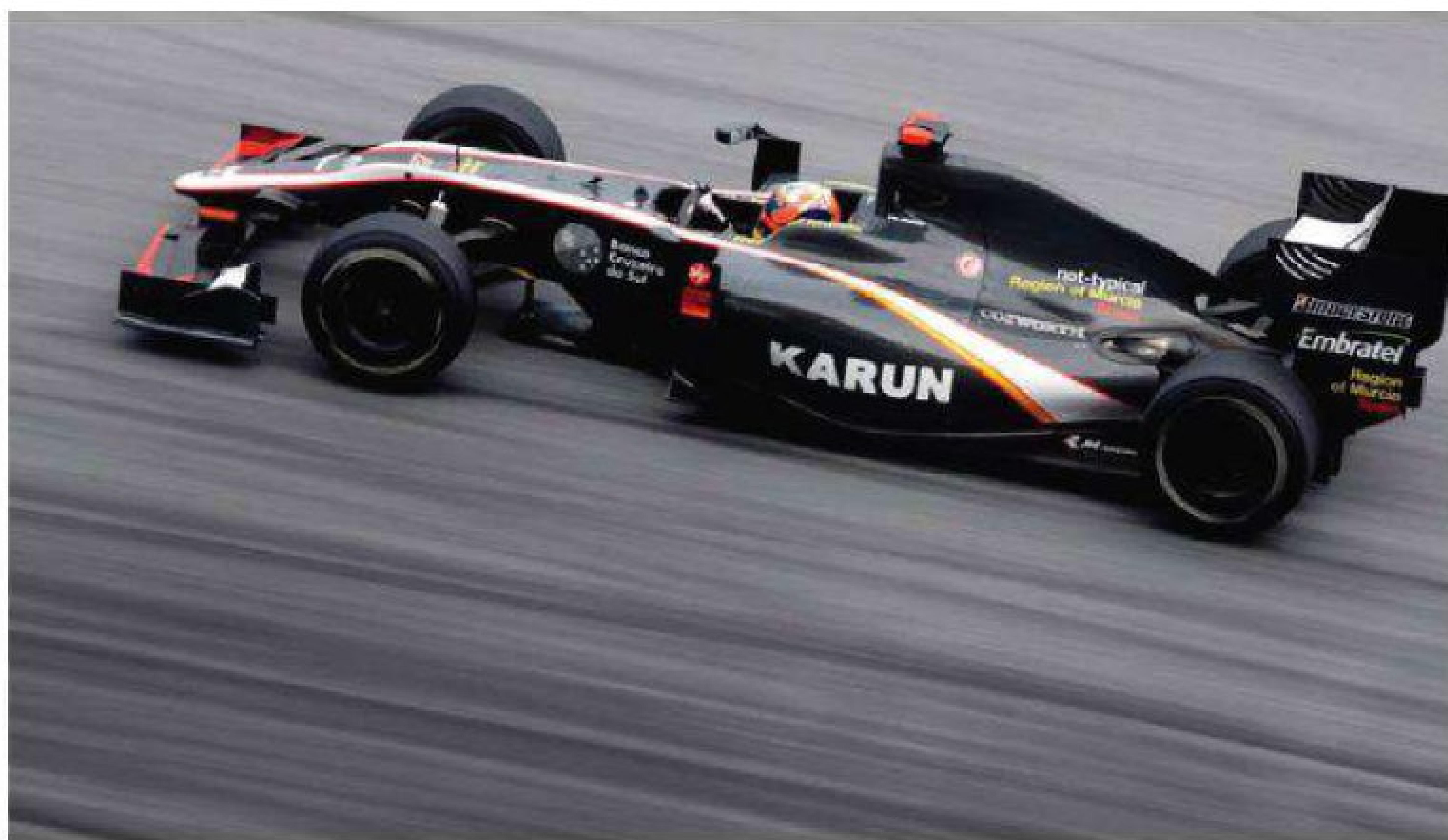
The F110 ran for the whole season in the Mk0 aerodynamic configuration, frozen by Dallara in November 2009. No further work was conducted (other than the wing mirrors - see right), and the Mk1 parts were never made
