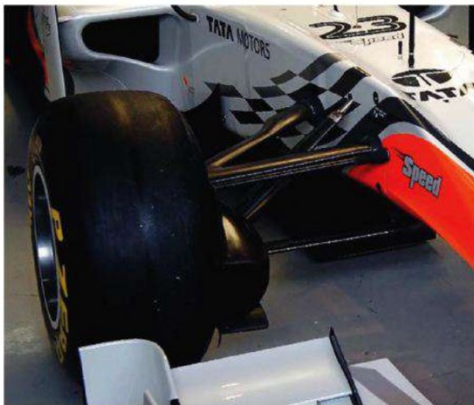
The front suspension of the F111 (above) is carried over in its entirety, and displays no changes compared with the F110 (right).
