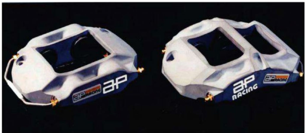
The quest for greater speed and efficiency, together with improvements in simulation and materials technology, has driven down the size of calipers, as evidenced by comparing these 1996 calipers with the one below
