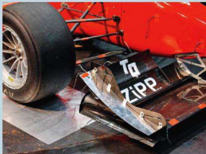
These front end plate flip ups operated similarly to some dive planes on closed-wheel cars, and showed a modest drag benefit
