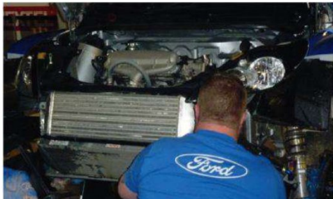
The Fiesta's powerplant is based on Ford's production I4 block and head, as used for the EcoBoost engines in the manufacturer's current road car range
