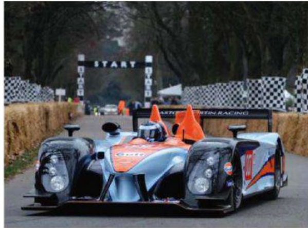
Aston Martin Racing has gone with an open-top design and turbocharged straight-six power for its AMR-One LMP1 contender
