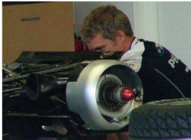
...looking from this angle, it's not hard to see why calipers easily overheat when a car comes to a stop out on circuit, as the shroud acts like an oven
