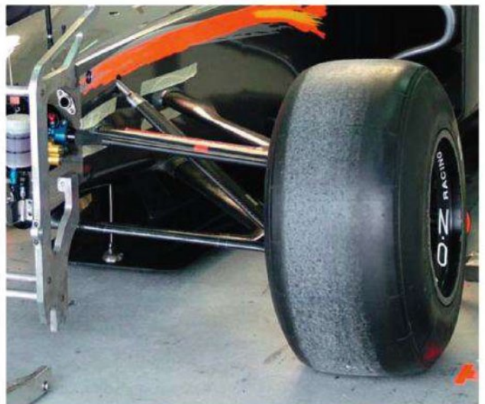
The front suspension of the F111 (above) is carried over in its entirety, and displays no changes compared with the F110 (right).
