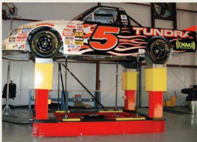
Adding roll resistance at the front increases front but not total load transfer
