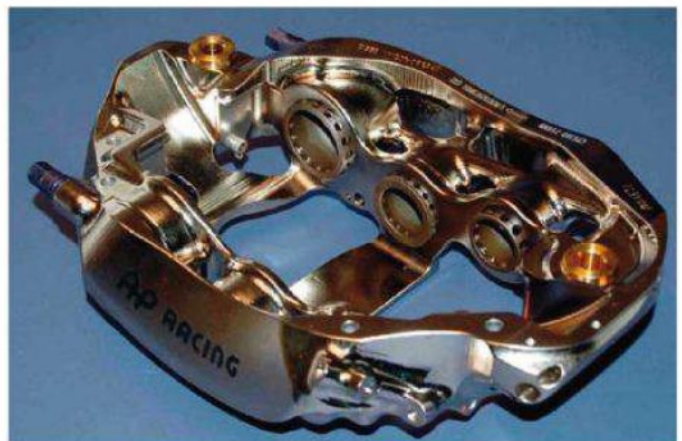
F1 calipers are limited to three pistons either side of the disc, generally of varying sizes to ensure even pressure is exerted along the pads' length
