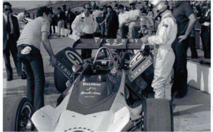
Following a test at Indianapolis with both dihedral and conventional wings, the rearward dihedrals were removed. Mario Andretti recalled, 'When the dihedral wings were taken off, the VPJ1 began to feel like a proper racecar'
