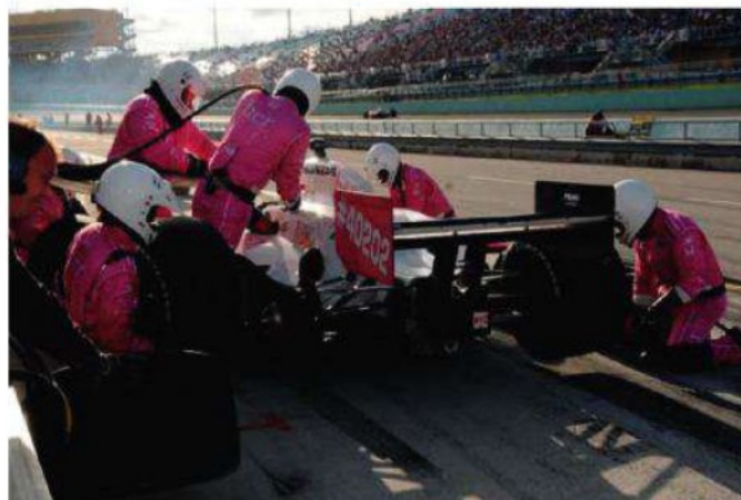
Tyre management in the Indy 500 dictates most of the strategy calls. The Speedway now has a highly abrasive surface, which is hard on race rubber
