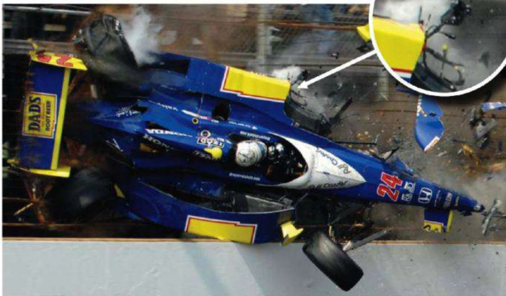
McLaren is understandably proud of how tough and reliable its ECUs are, having withstood Mike Conway's horrific 200mph crash during last year's Indy 500. That's the detached ECU circled, which still functioned afterwards!
