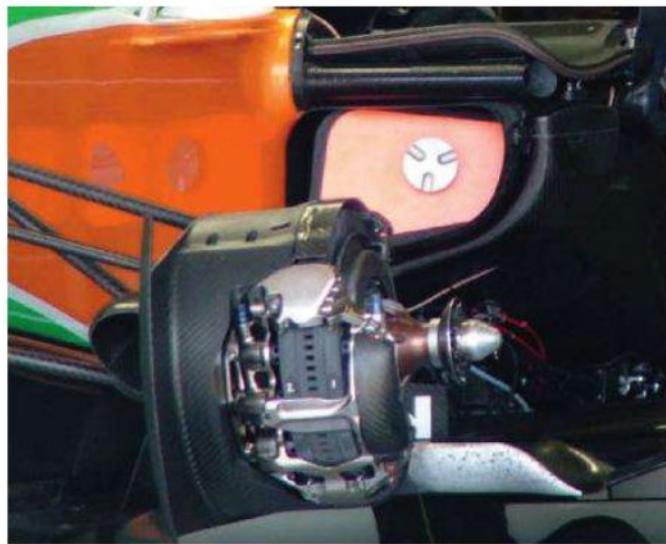
The service life of an F1 brake caliper has more to do with the thermal cycling that the caliper sees than the mileage over which it is used
