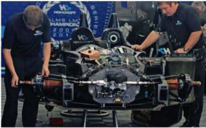
Packaging the wider P1 tyres and wheels, and the associated cooling ducts, presented some issues, but lessons learnt from the P2 project paid off
