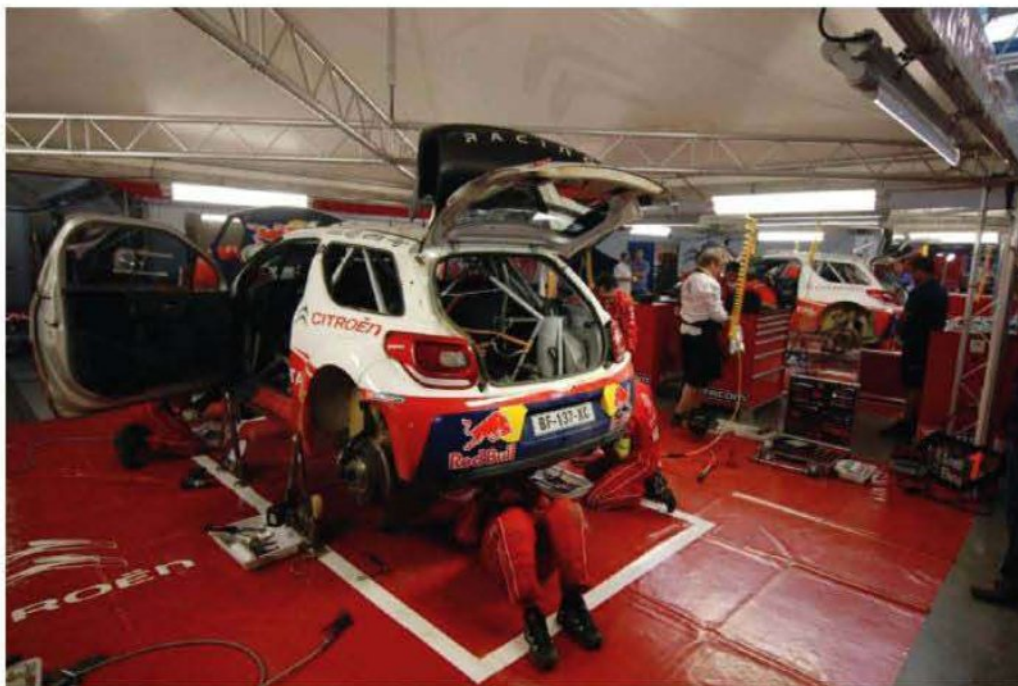
Outwardly similar to that of the outgoing C4, the DS3's suspension and brakes comprises Citroën Racing's re-engineered components, while the gearbox with its rear drive disengage unit, is a joint venture with Sadev
