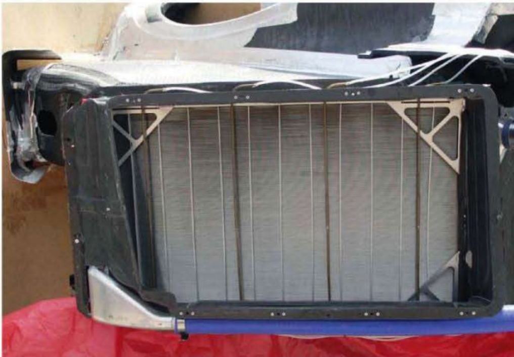
Young's open section tunnel with a Mezzo Technologies IndyCar cooler installed in a complete Dallara side pod. The open section tunnel allows for rapid testing of multiple design iterations
