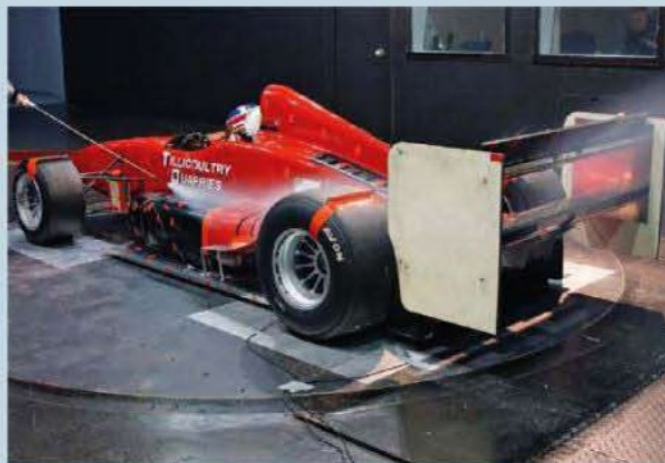
The airflow passing over the rear of the sidepods and flip ups quite clearly encountered the rear wing further downstream
