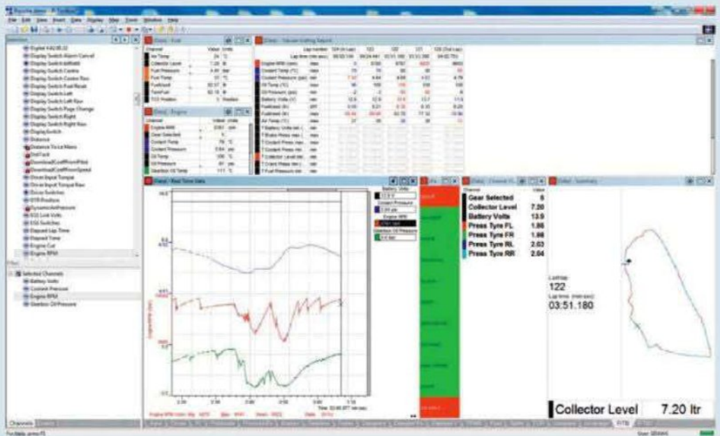
Figure 1: typical view of a live telemetry window. Tyre data is shown as raw numbers and bitfields indicate if there is a problem. Trends are then monitored using live graphs and summary tables
