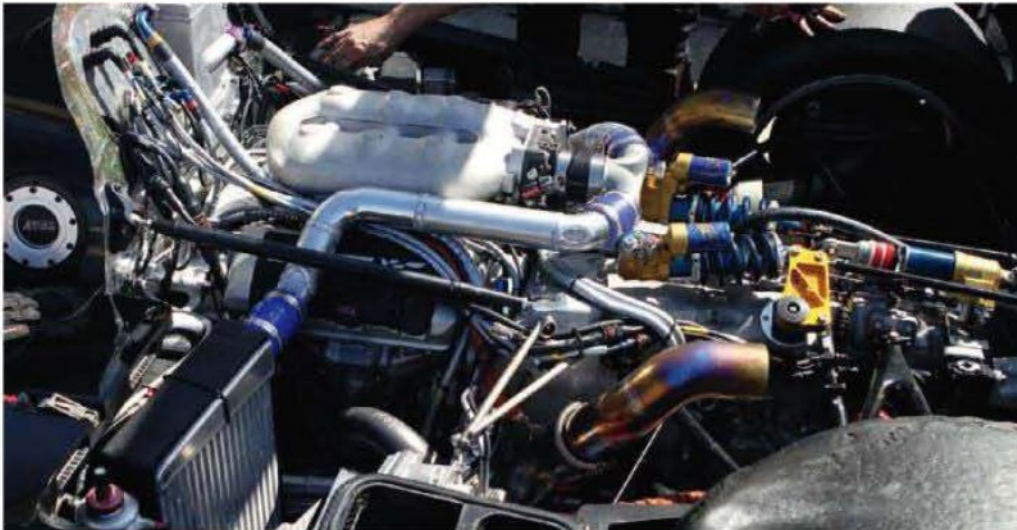
The Honda engine was never intended to serve as a fully stressed member, so to solve the problem an external structure was built, which encases the engine and offers the amount of rigidity needed
