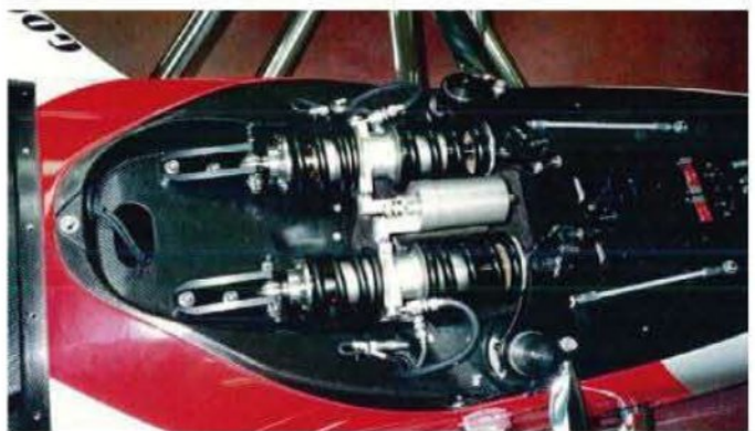
Another front installation showing the banjo fittings feeding the actuator. The damper portion is at the bottom (right), towards the Moog valves
