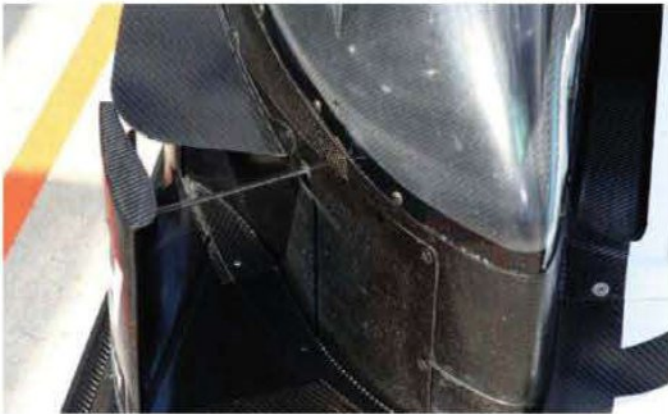
Elements of the 02a-to-01d aero kit have been carried over to the 01e, including the flow conditioners used at the outer edges of the front wings
