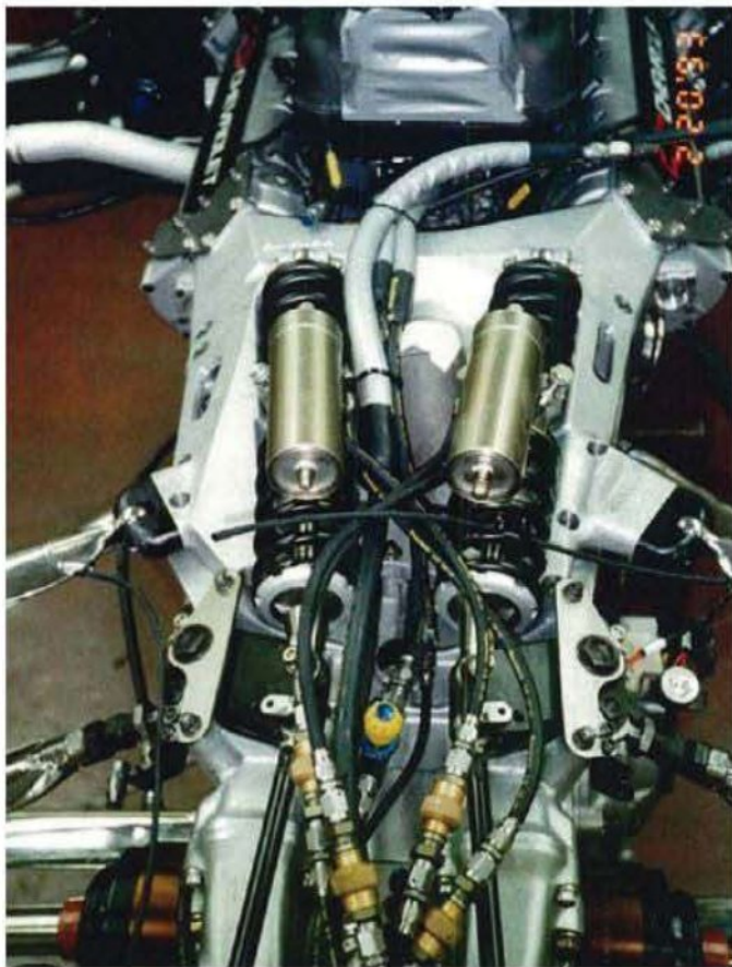
In this pre-installation view, the actuators are at the top, towards the engine
