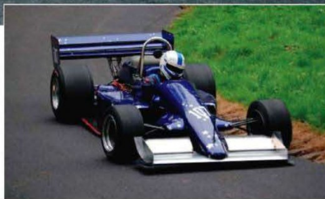
Pilbeam's most recent chassis, the MP97, again uses a carbon monocoque and is a development of the MP87. It's a regular in the Top 12 Run Offs
