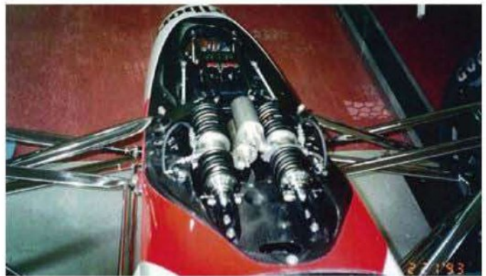
The front installation showing the upper actuators with the redundancy springs pre-loaded and installed. The two mechanical Moog valves can be seen at the front of the nose box in front of the ARB blades
