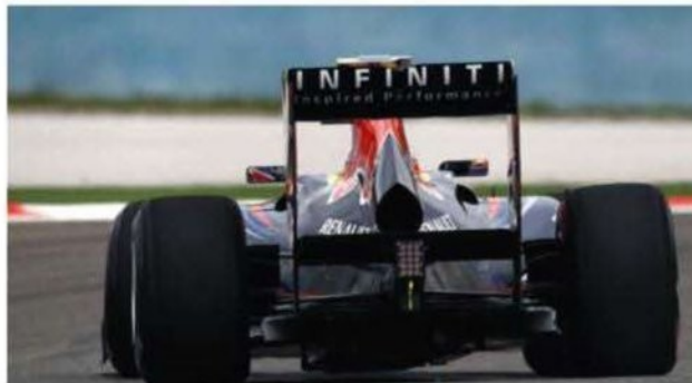
The FIA says blowing exhaust gasses through the diffuser when off throttle is tantamount to a moveable aerodynamic device
