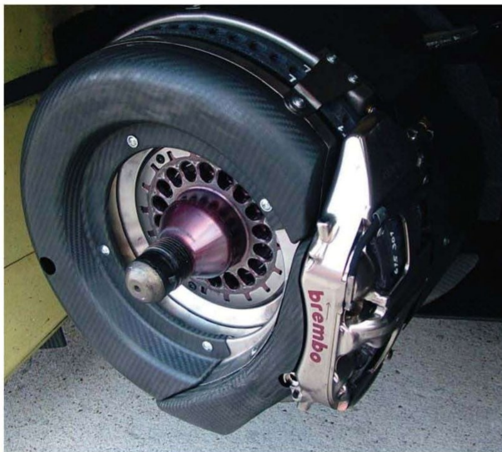
Everywhere on the new car the emphasis has been on improving efficiency and reducing weight. The brakes are lightweight alloy monobloc calipers from Brembo with ventilated carbon fibre discs all round
