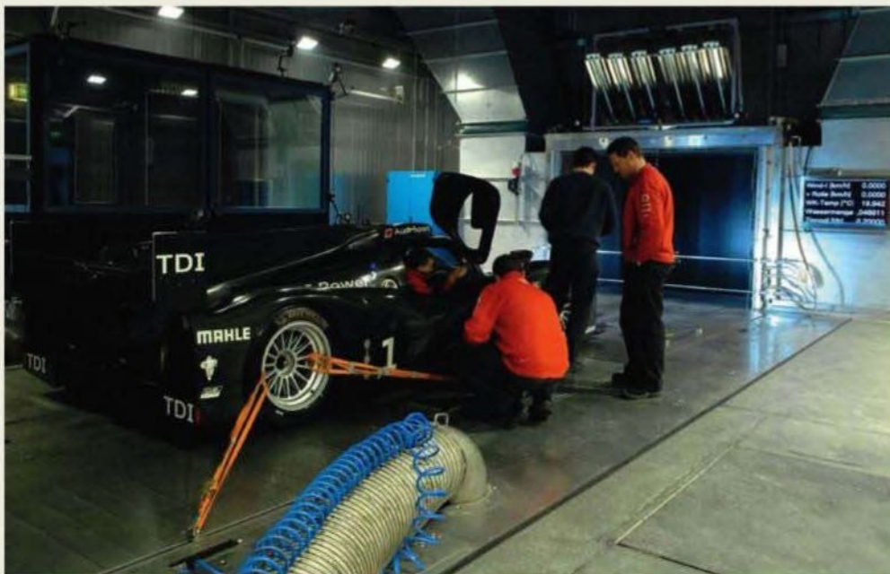
The climatic tunnel is normally reserved for production car test programmes, but proved invaluable for testing cockpit temperature rises in high ambient temperatures and for developing the car's anti-fog windscreen system
