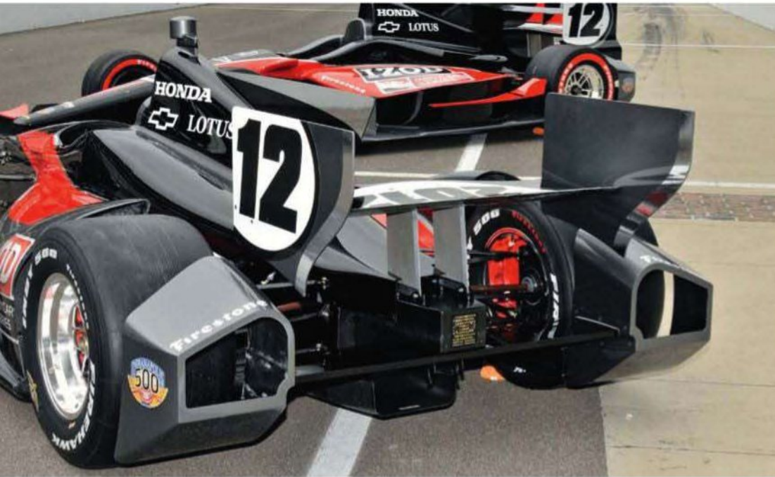
Pods behind the rear wheels are intended to improve straight-line speed, but give the cars an air of Group C Sportscars
