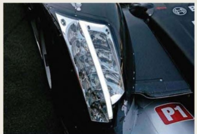
Light fantastic. The R18's headlights use the most powerful LEDs currently available, with the main beam using three extra LEDs to create the effect of a high beam by illuminating the track additionally through reflectors
