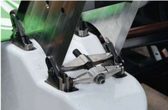
Rear wing location devices vary significantly from car to car, though the key is ease and speed of adjustability at the track
