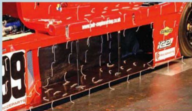
Modified sidepods provided an unrestricted exit for air passing under the splitter and front diffusers
