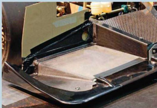
Connecting the diffusers to the trailing edge of the splitter produced a substantial increment in frontal downforce
