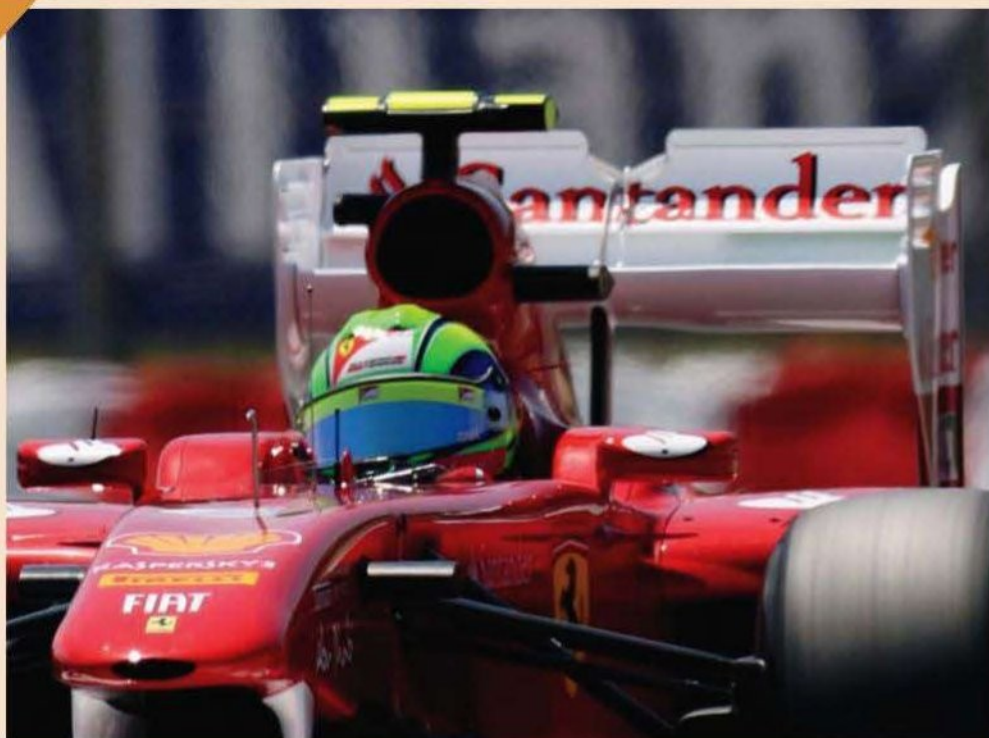
Ferrari arrived at the Spanish Grand Prix with extended Gurney flaps on the rear wing. They were promptly banned and the car had to race in its original configuration (below)
