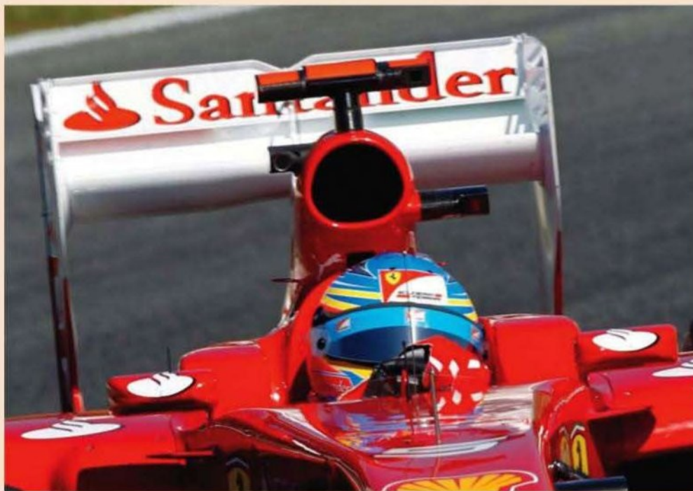
Ferrari arrived at the Spanish Grand Prix with extended Gurney flaps on the rear wing. They were promptly banned and the car had to race in its original configuration (below)
