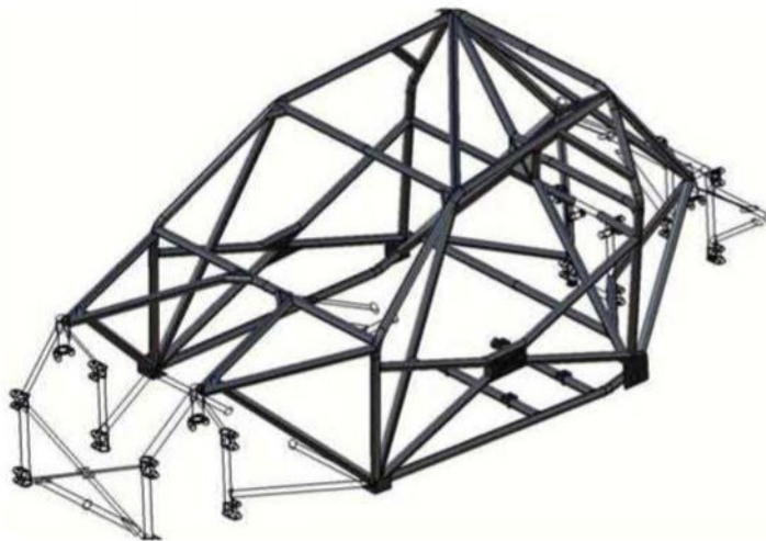
Fabrication specialist Locklid built the 'cage, which was modelled using FEA and features CAD design work by engineering student Eva-Verena Ziegahn
