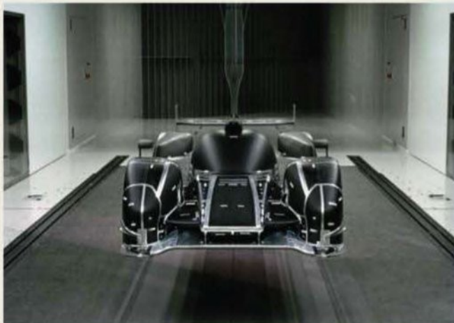
The climatic tunnel is normally reserved for production car test programmes, but proved invaluable for testing cockpit temperature rises in high ambient temperatures and for developing the car's anti-fog windscreen system
