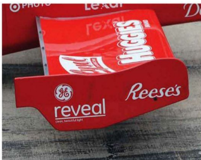
Front wing end plates are open to development by individual teams and generally match the wing angle range a team expects to run
