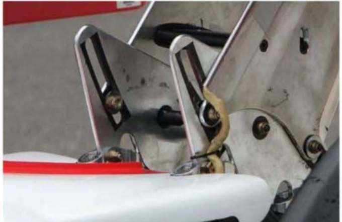
Rear wing location devices vary significantly from car to car, though the key is ease and speed of adjustability at the track
