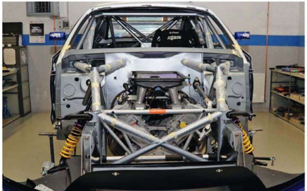
The ex-ALMS LMP2 3.4-litre Judd KV V8 was chosen for its compact dimensions as F3000 engines were not for sale
