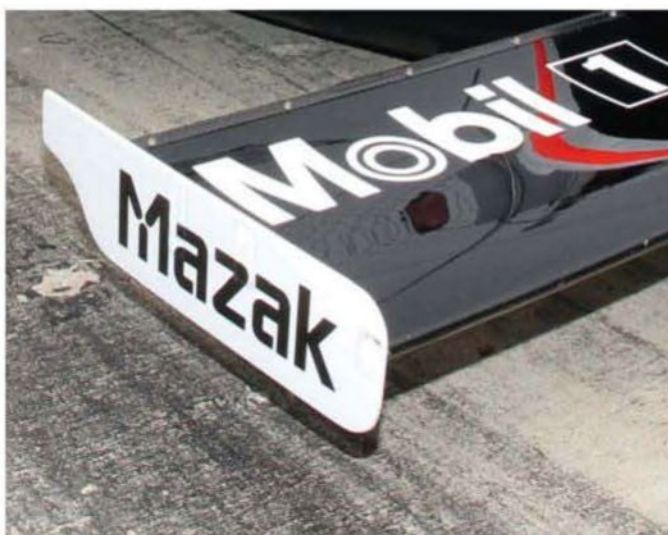
Front wing end plates are open to development by individual teams and generally match the wing angle range a team expects to run
