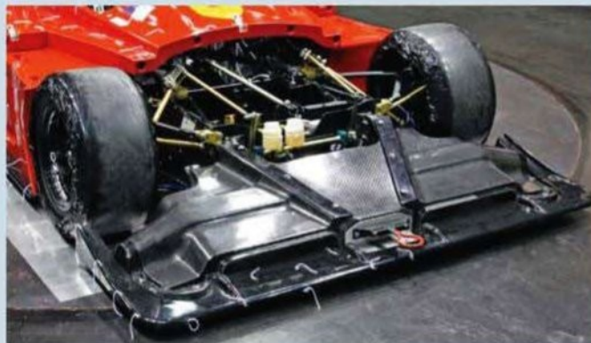
The front end featured a two-tier splitter / diffuser arrangement
