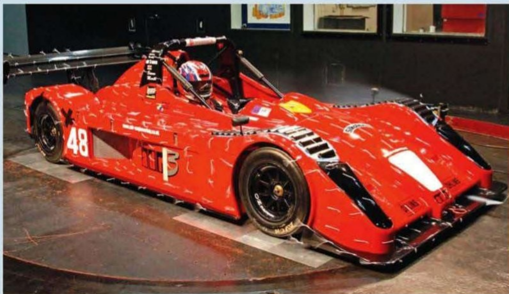
Here we can see the smoke plume entering through the left front aperture and exiting via the wheelarch louvres
