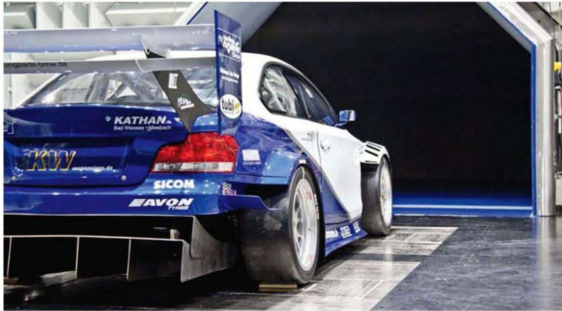
Having used BMW's own wind tunnel to develop the previous car's aerodynamics, this information was used as a baseline for the new car. Carbon composite exterior body panels were manufactured by Flossman Auto Design
