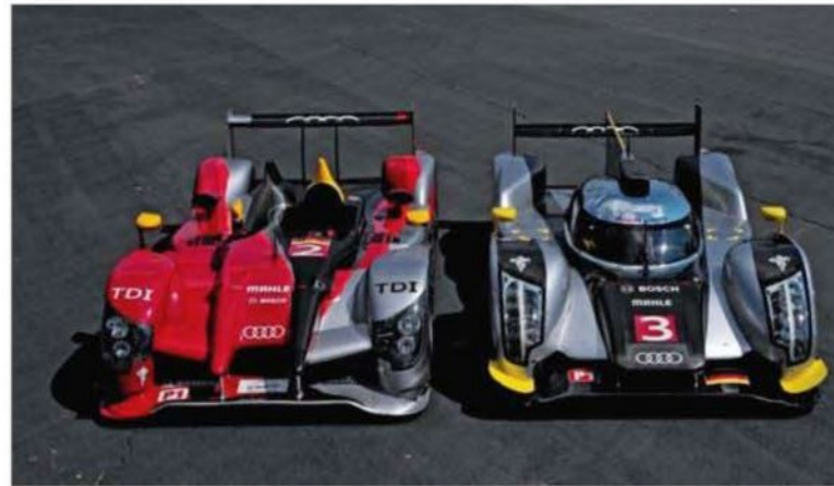
Audi's V10 R15 TDI (left) went through a redesign before the company bowed to the inevitable and introduced a closed Prototype - the V6 R18 TDI
