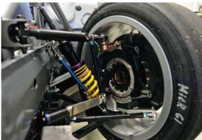
Win Geo and Catia were both used to design the all round double wishbone suspension, which uses modified E36 magnesium front uprights and fabricated rear uprights. Adjustable coilover dampers are by KW Automotive
