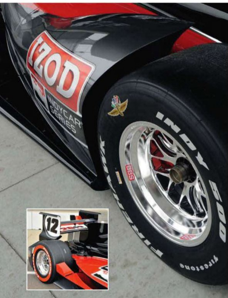
A great deal of thought has gone into the design of the sides of the car to try and prevent cars rolling or taking off when they slide sideways
