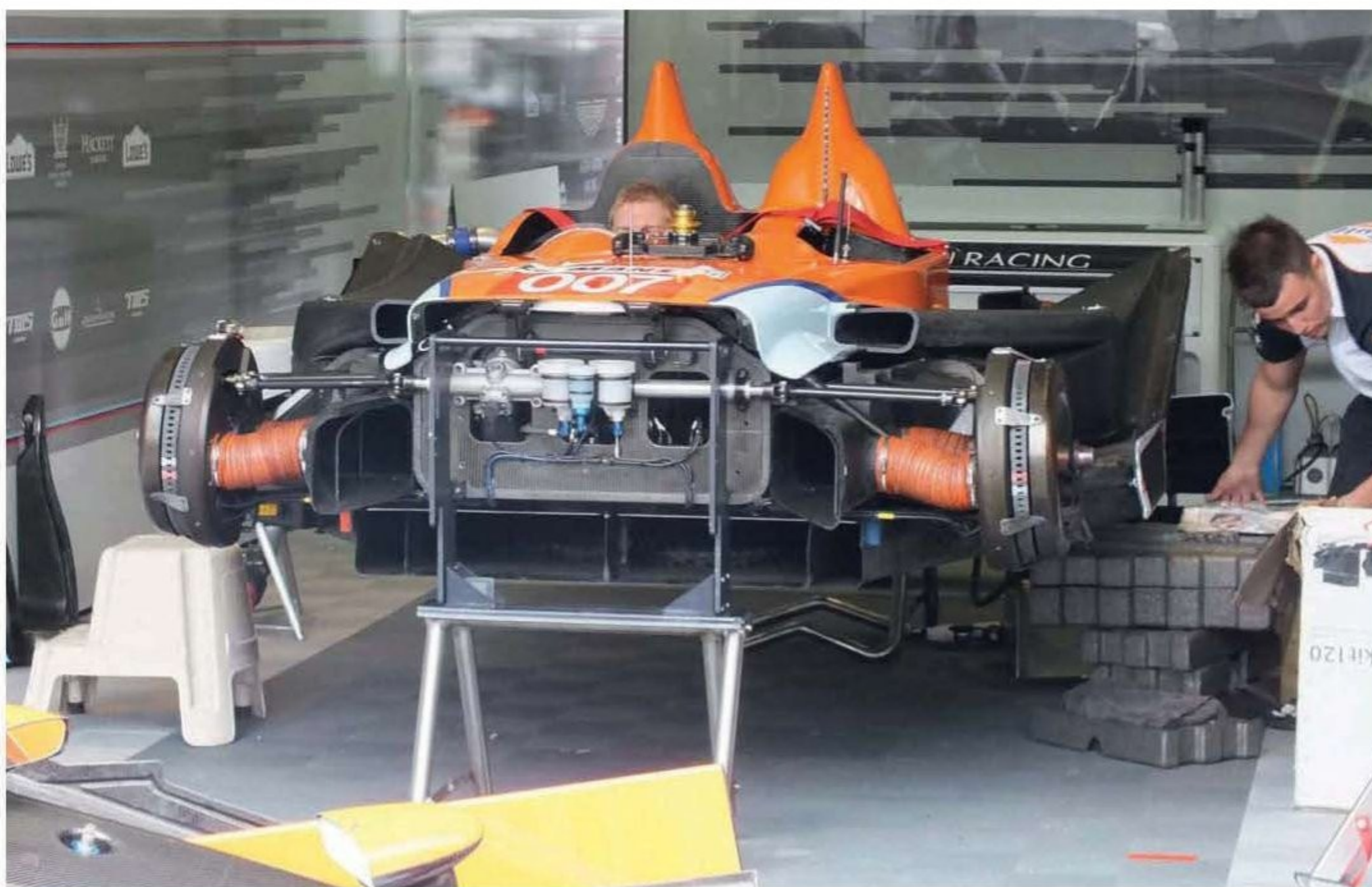
Double wishbone suspension layout is conventional, but there's a complex ducting arrangement that controls airflow through and around the rear of the car
