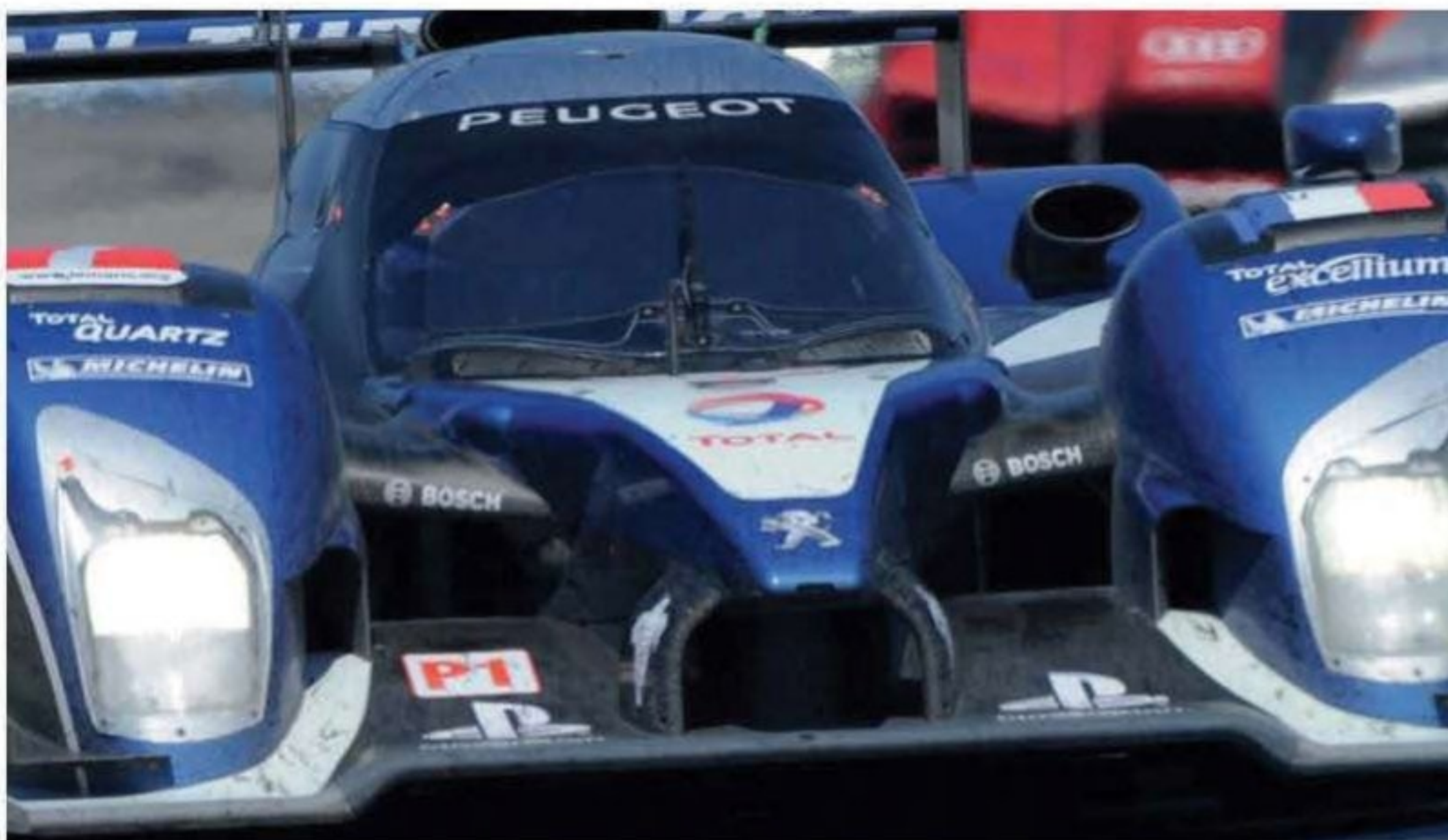
The low drag nose used by Peugeot at Le Mans and Spa has less cooling compared with the original. The brake ducts have been relocated to NACA ducts in the centre of the front panel. The high downforce nose used at Sebring (above) has much larger radiator ducts and large brake ducts.
