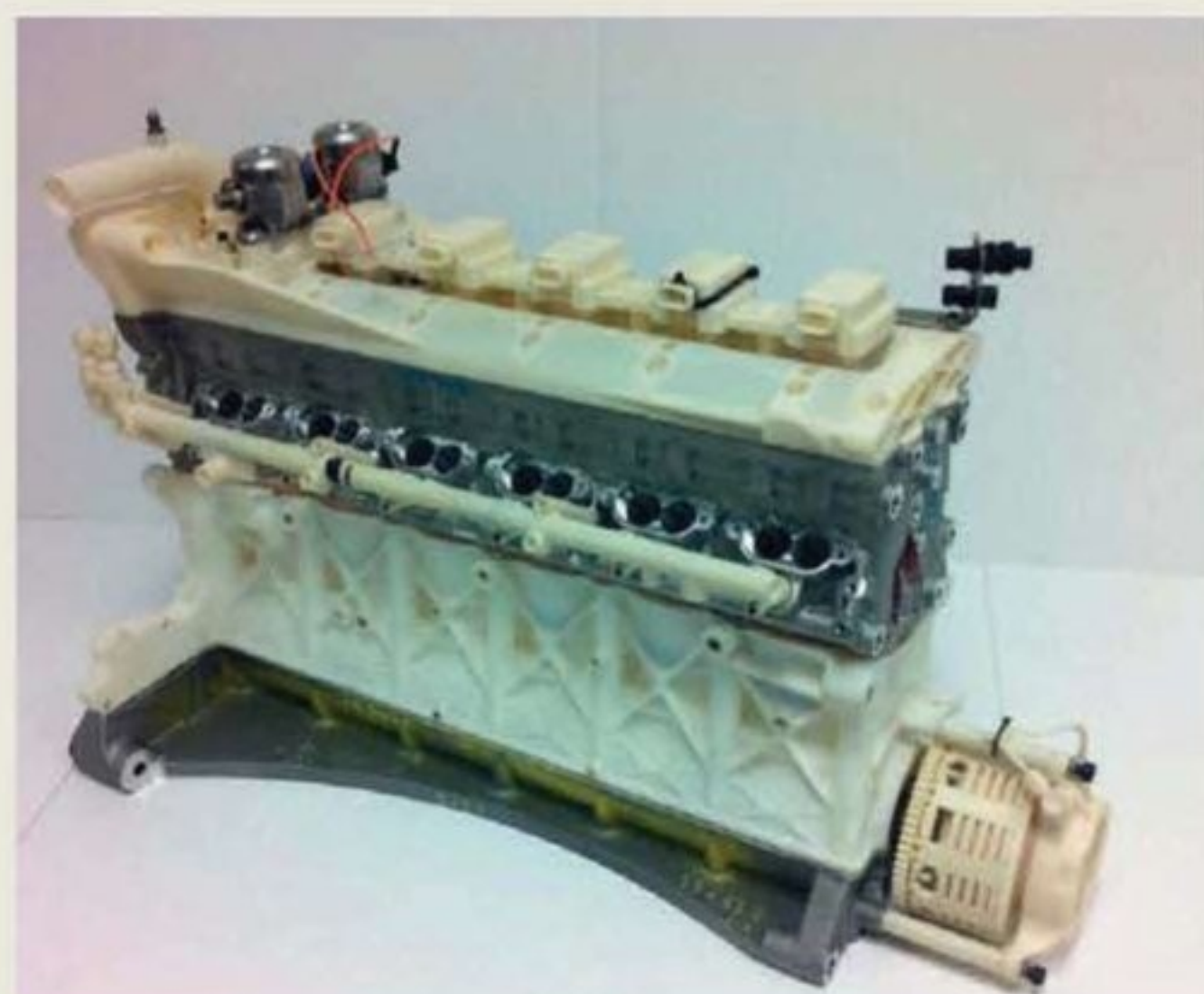
Most of the straight-six engine was rapid prototyped using the Dimension machine, which saved a vast amount of time in the development process
