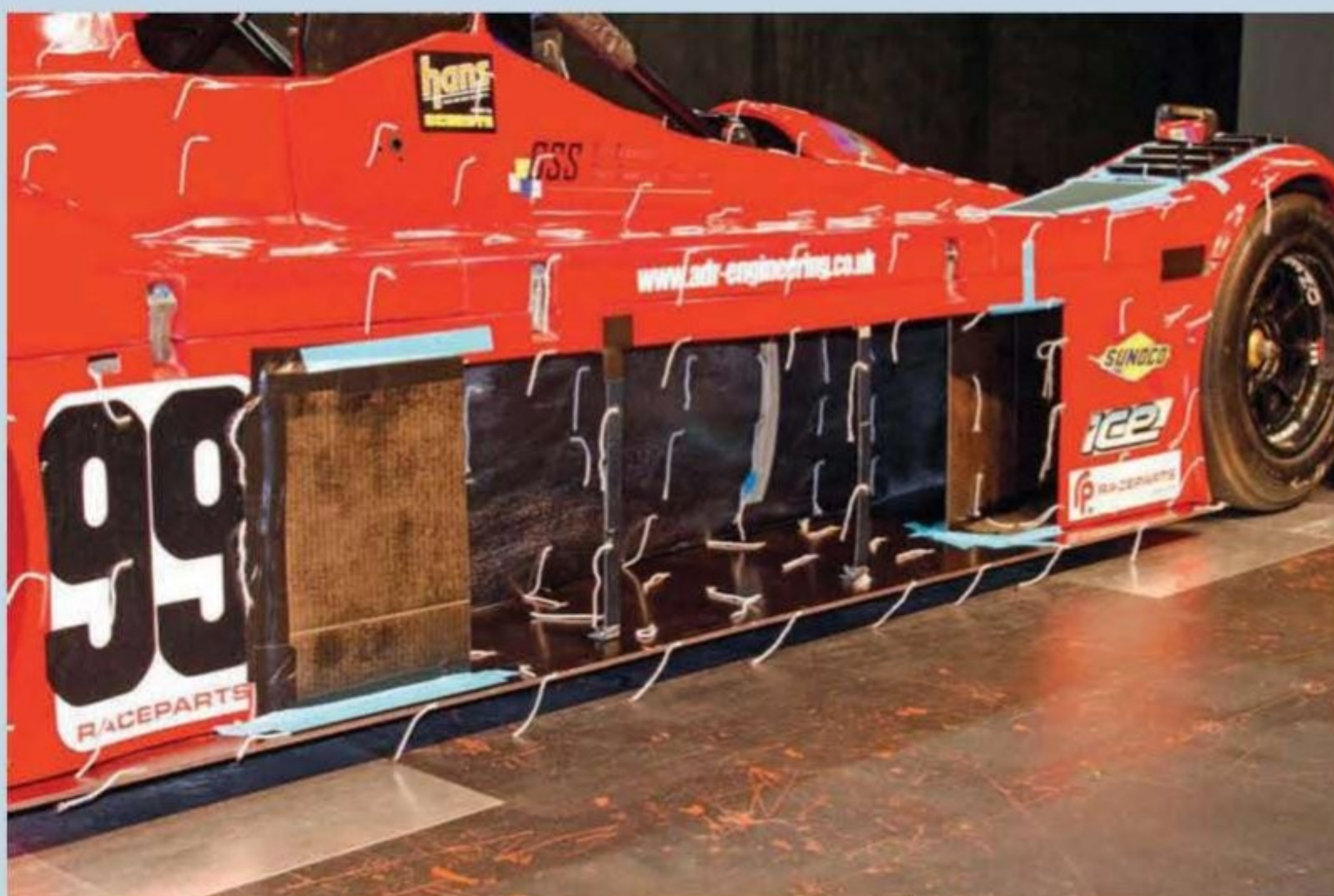
This configuration of sidepod produced the best through-radiator velocity, but reduced front downforce somewhat
