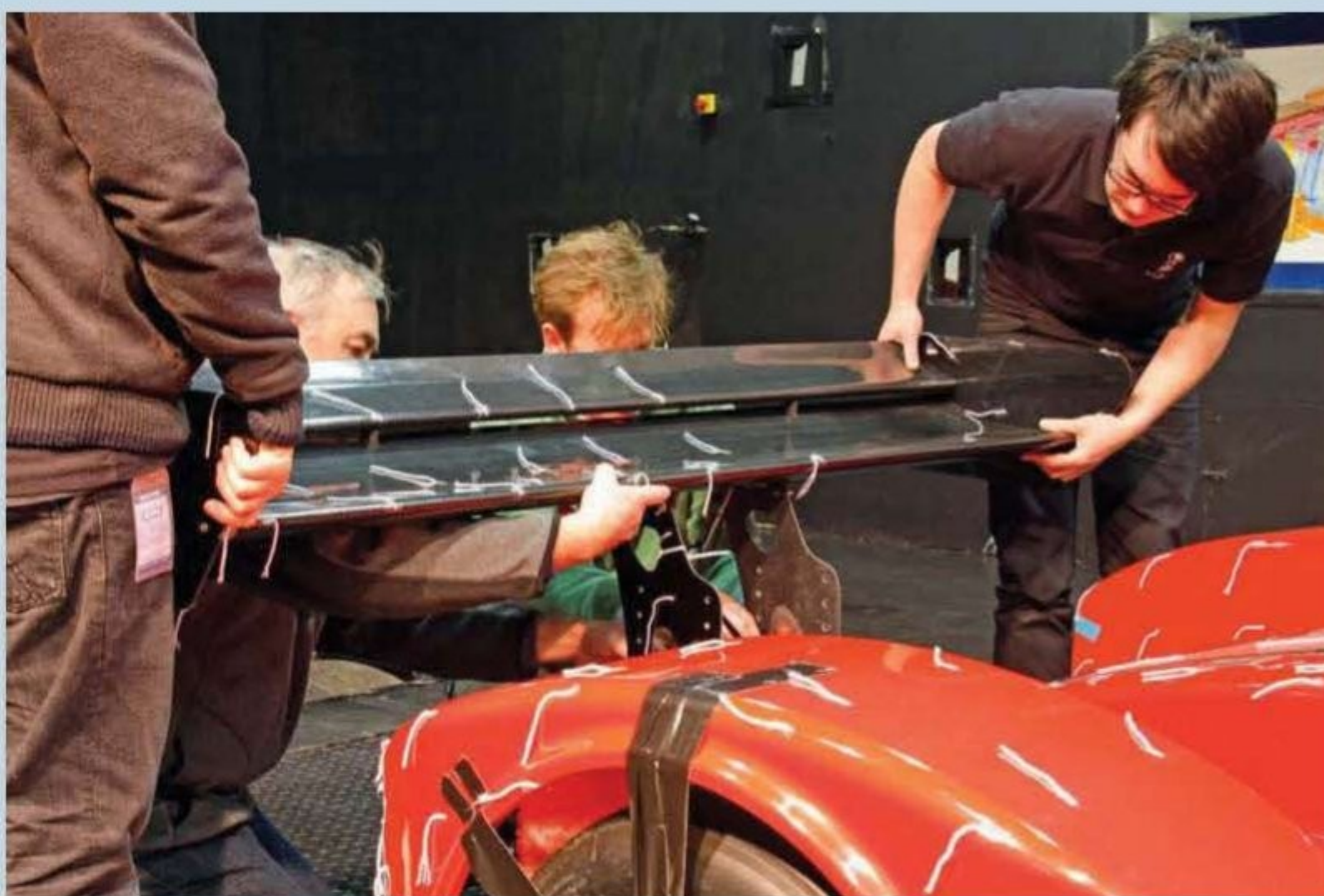
The stock rear wing position was at the maximum permitted height, often best for maximum downforce
