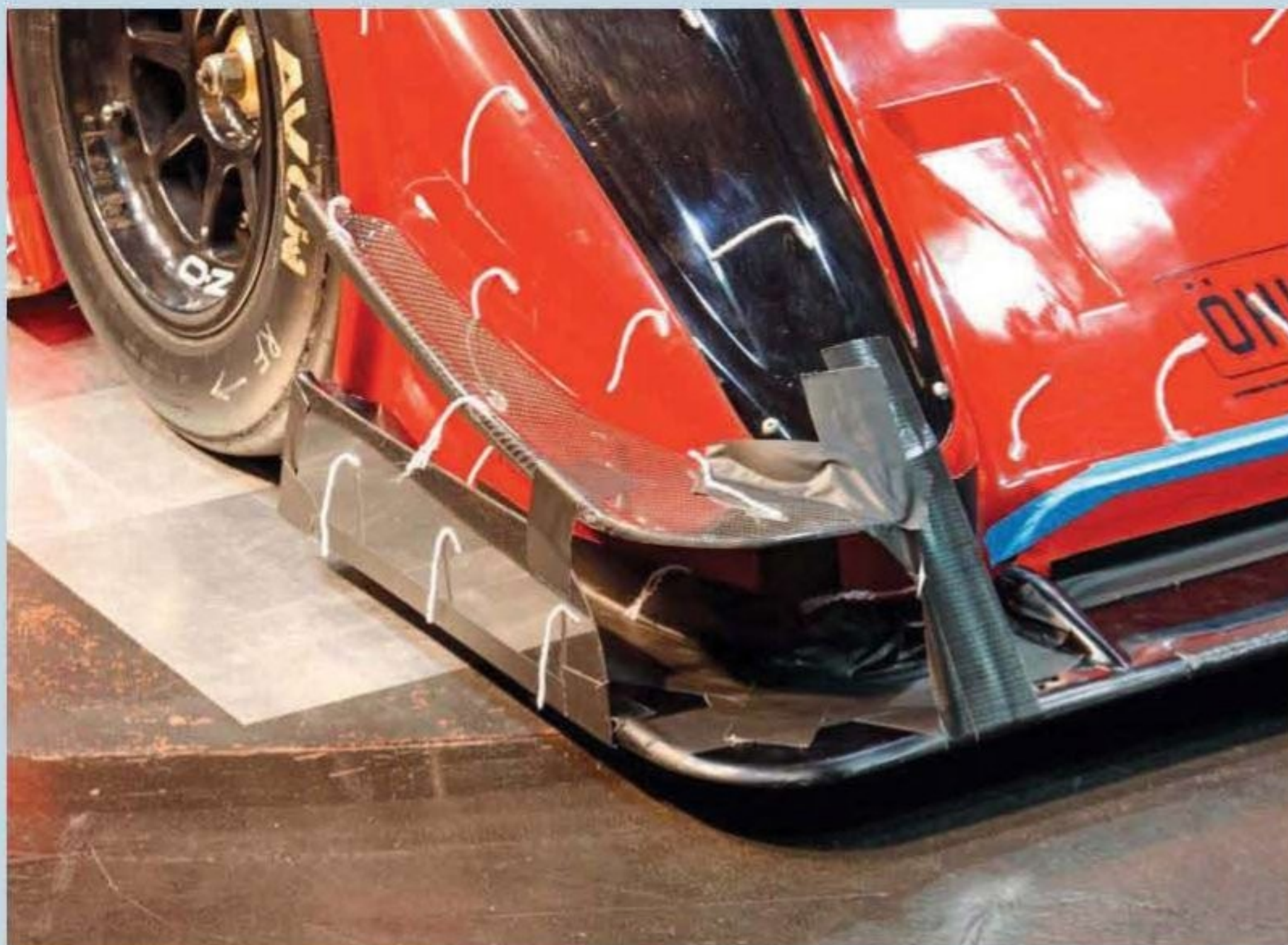
These front end plates also shifted the balance forwards, but knocked more counts of downforce off the rear than they added to the front. Drag did reduce a little though
