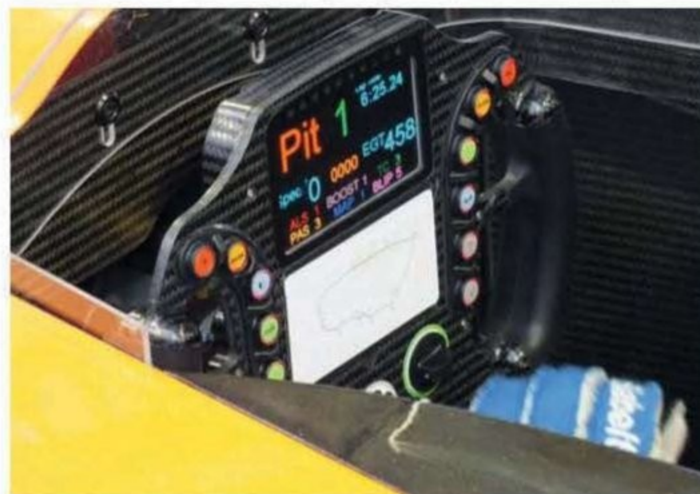
Driver controls were mocked up in the early development stages using the Stratasys Dimension 3D printing machine, then manufactured in house
