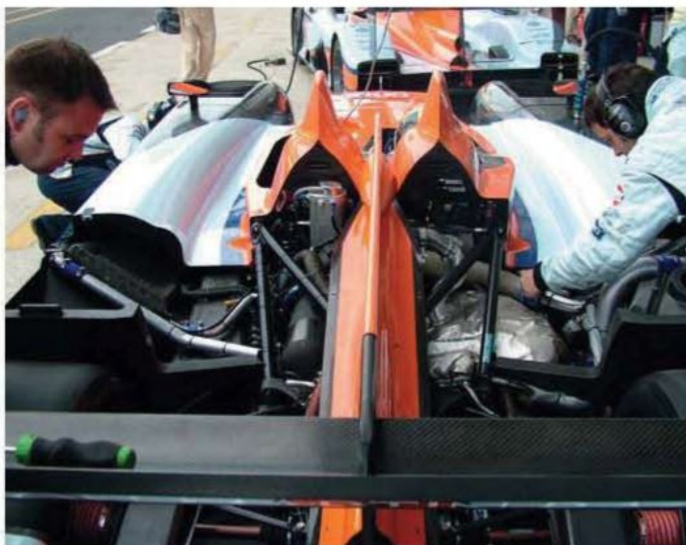
Being an in-line configuration rather than a V, engine layout is asymmetrical, with the plenum on the right-hand side and exhaust on the left
