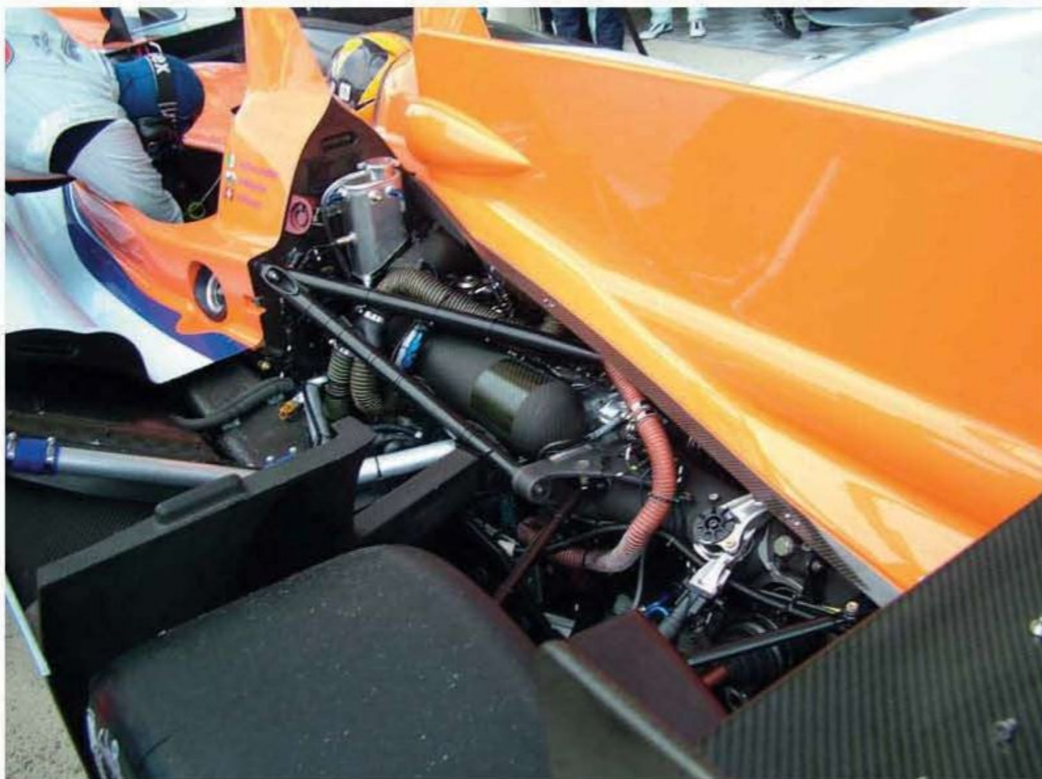
Engine location is not stressed, but is supported by a triangulated structure that picks up on the bellhousing
