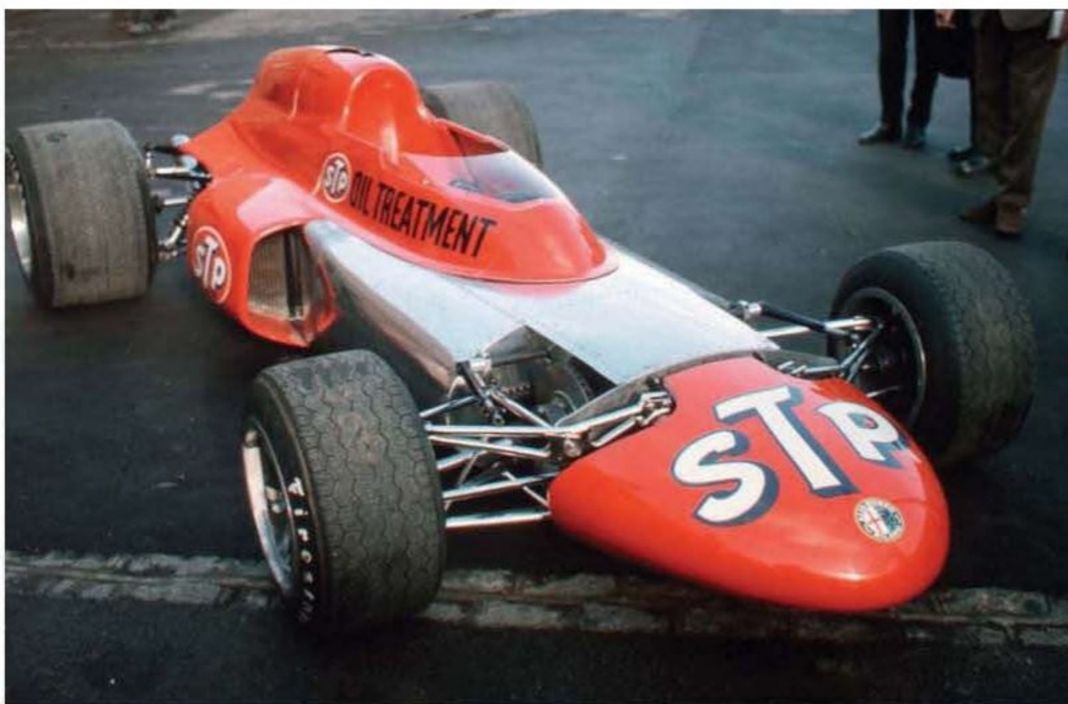
Much of the 711s rear bodywork was discarded when engine cooling problems arose during initial track testing.
