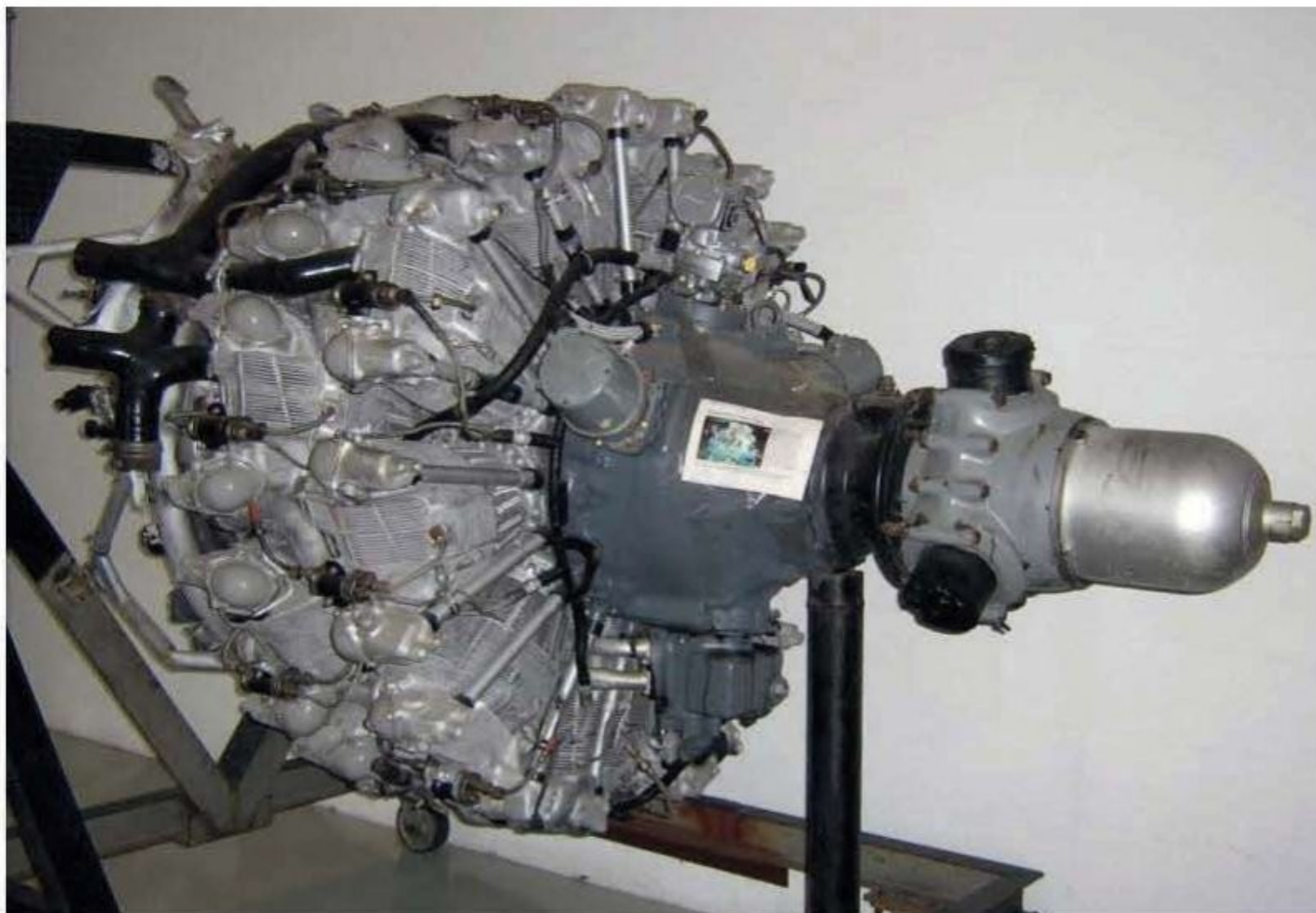
Radial aircraft engines were the first application for turbocompounding
