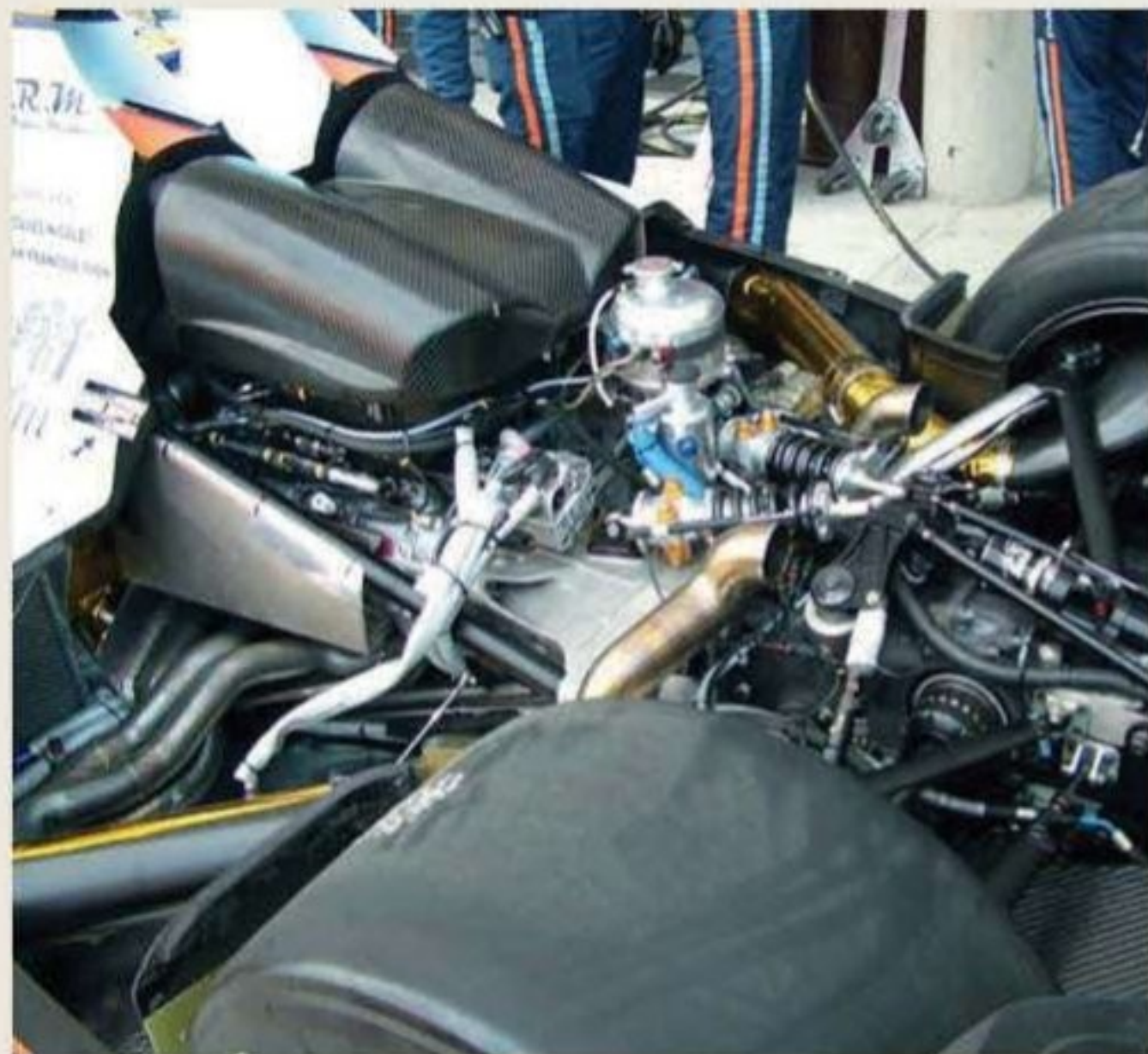
Engine specialists have been forced to use production-based blocks. Judd opted to use the BMW V8, 4.0 litre in road going form.
