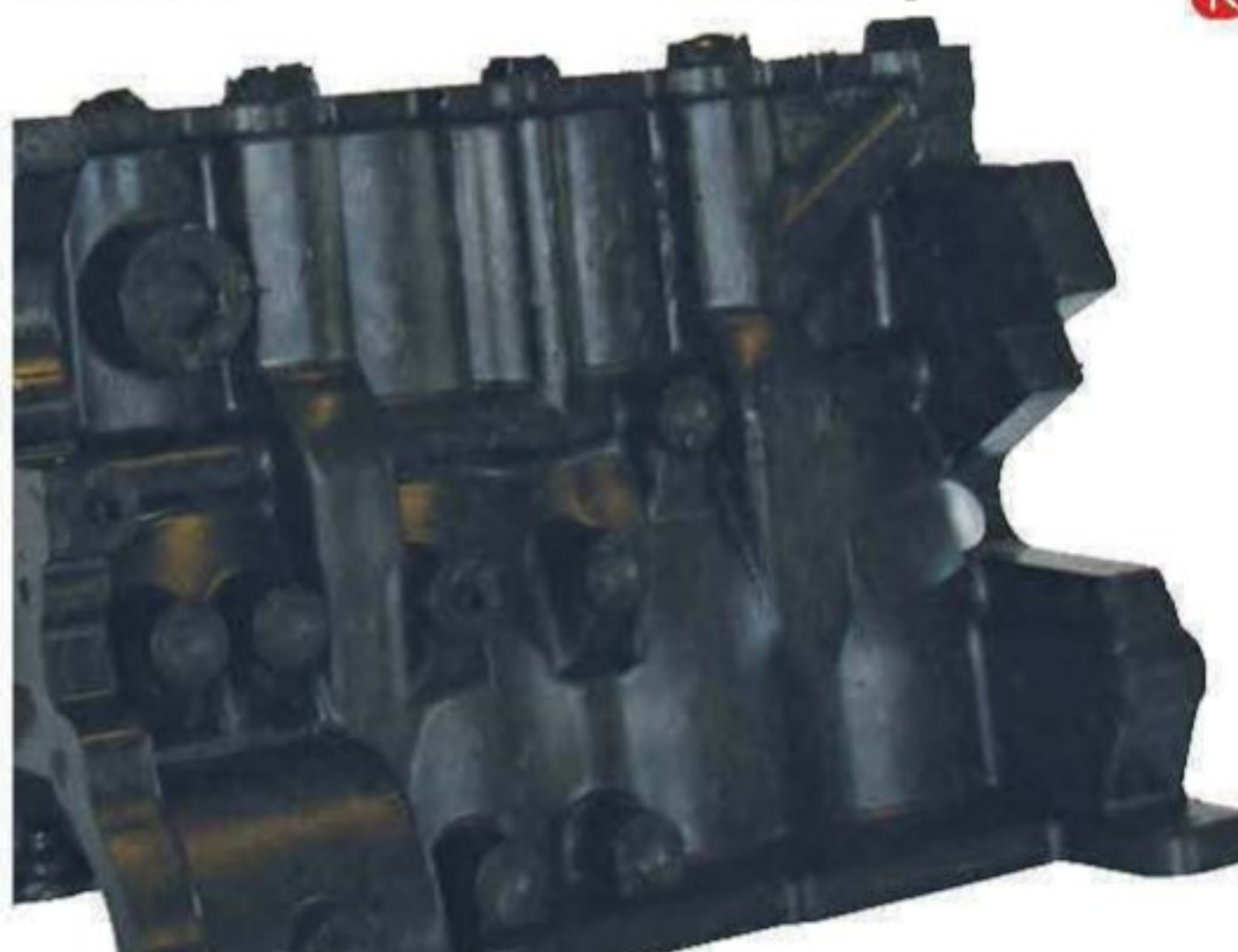
Matti Holtzberg pioneered the use of composite materials in structural engine parts
