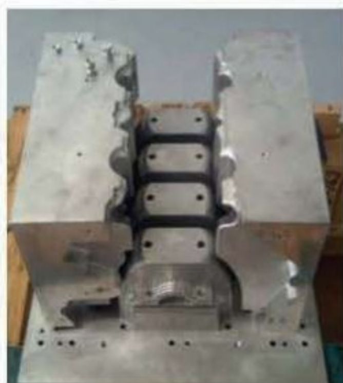
A typical die-casting die will cost $1million, and it will be shot after 100,000 parts. With composites, up to a million parts can be made, with a lower priced die
