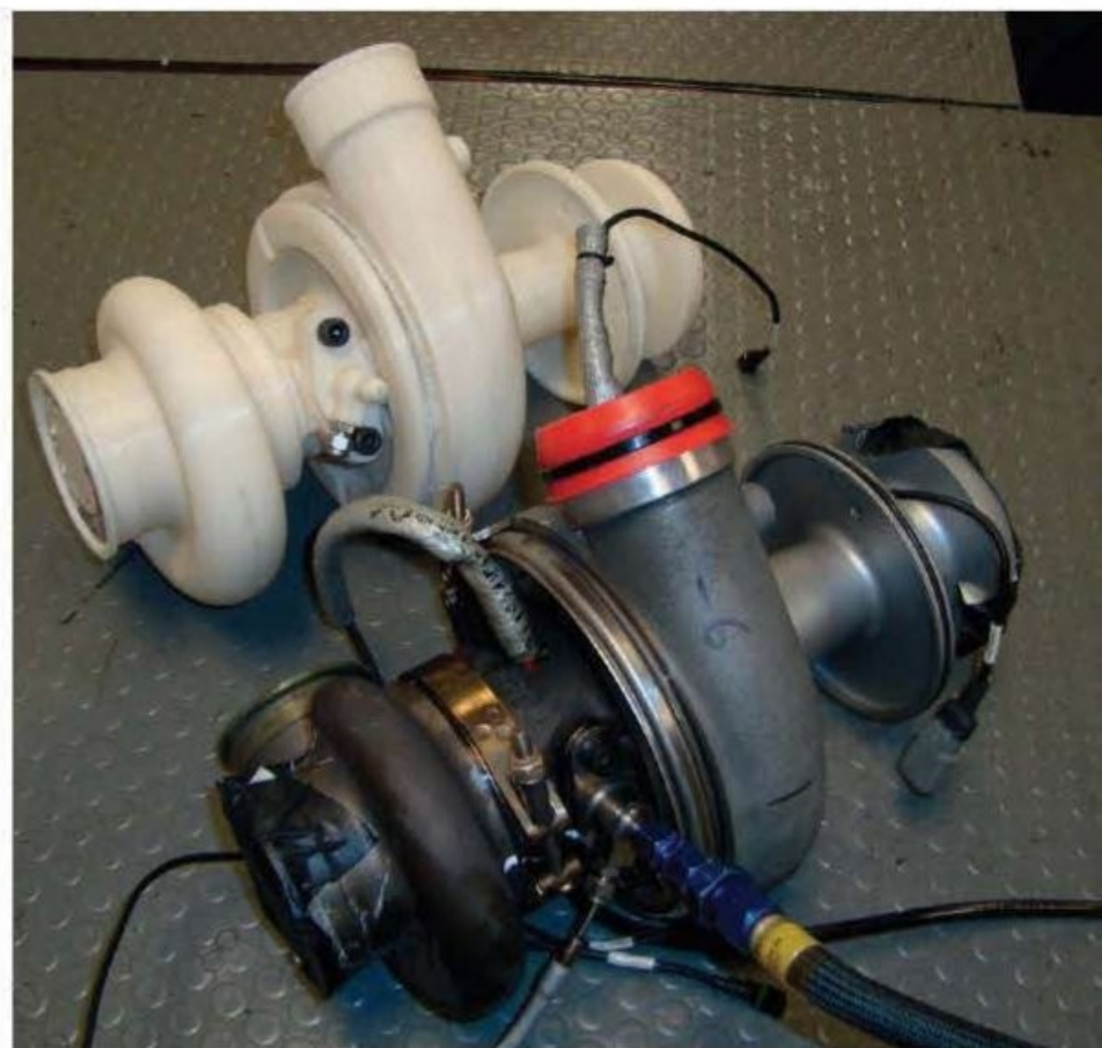
A single turbocharger configuration was chosen, but early tests with an inboard location caused problems with heat management and power potential, so an outboard location was run at Le Mans. The team are currently working on a new iteration of the system
