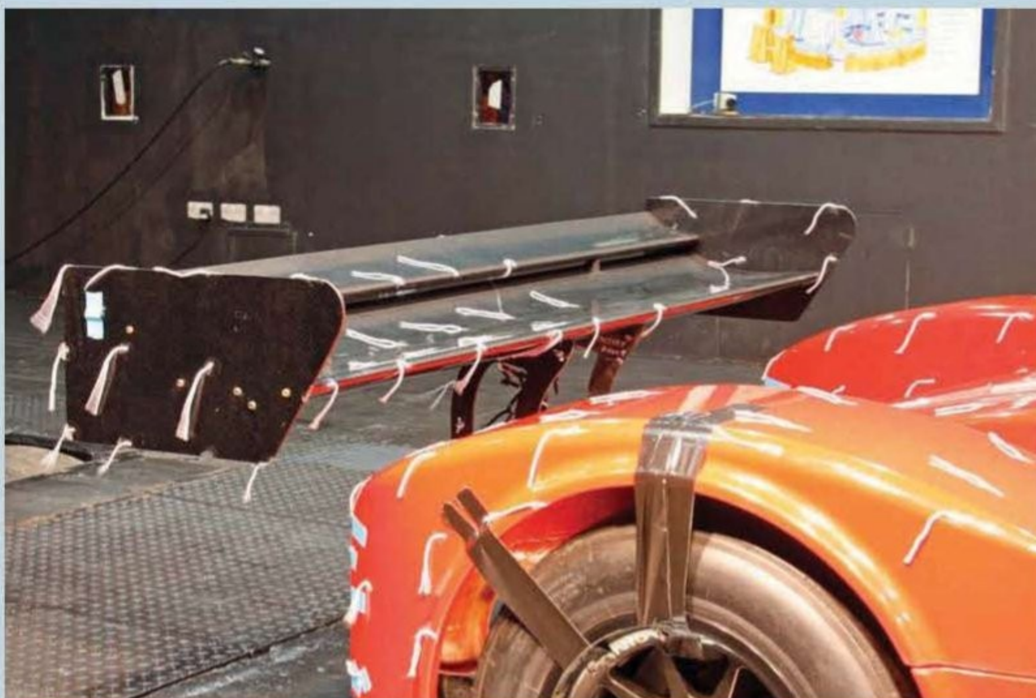
Lowering the wing and moving it forwards by 135mm produced almost as much total downforce but improved both balance and efficiency, leading to the conclusion that its interaction with the underbody had been improved, too
