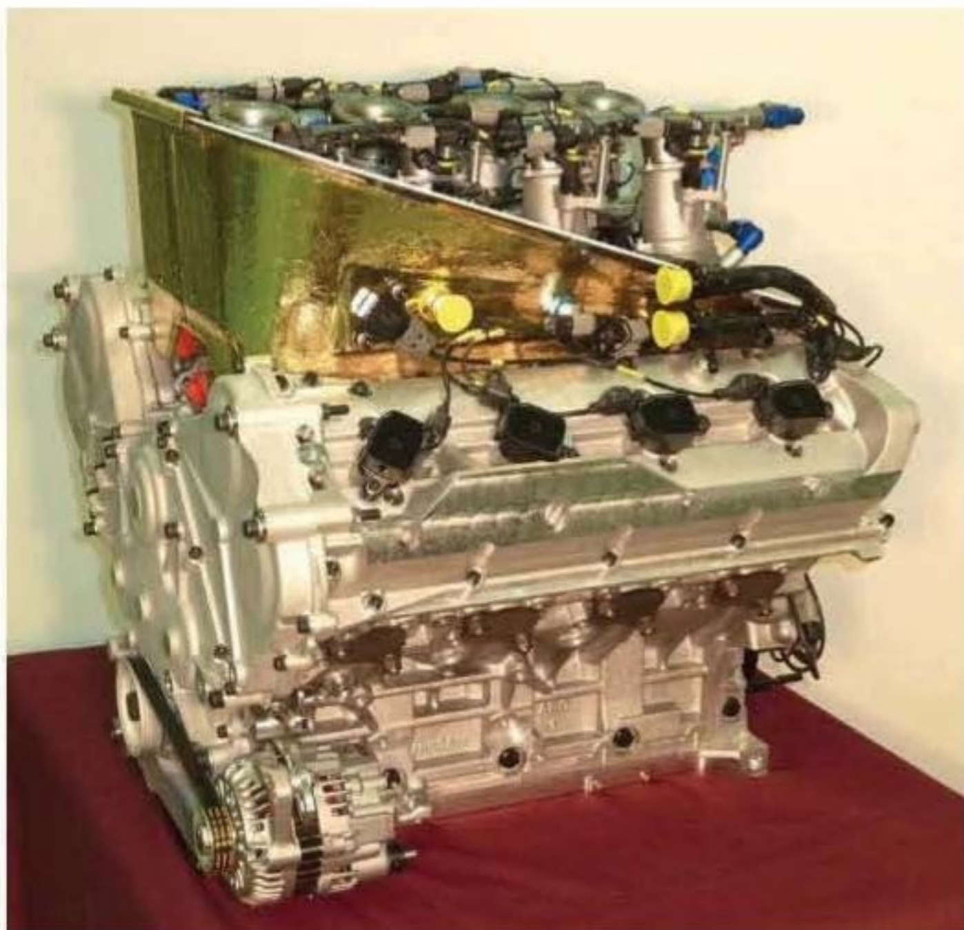
Based on a standard Nissan road car block and heads, the LMP2 engine uses bespoke crank, rods, pistons and intake for maximum efficiency
