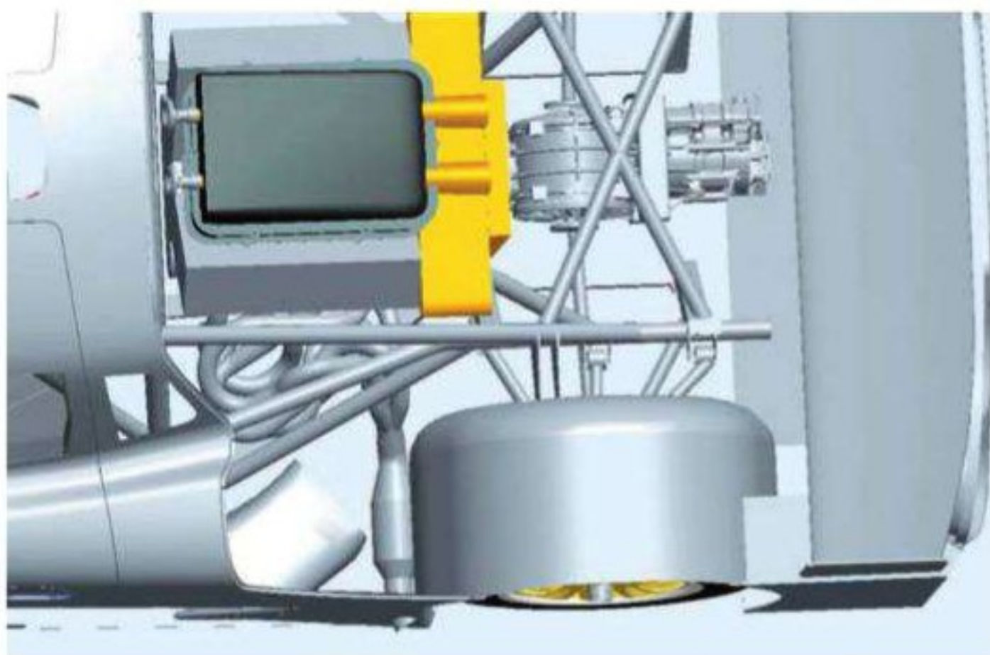
The position of the airbox required a bespoke design, which was modelled in CAD and laid up by carbon composite experts Reverie
