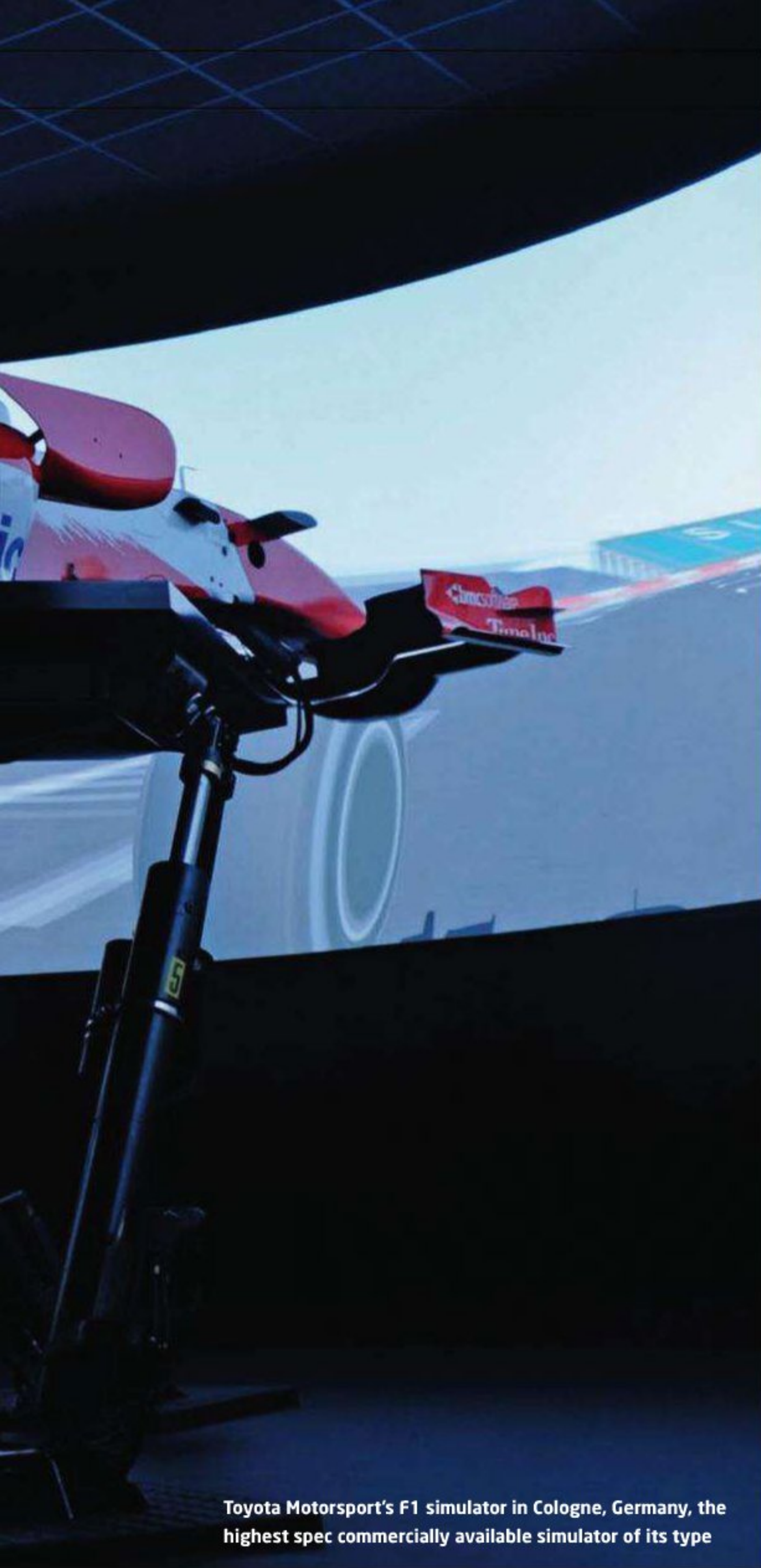
Cruden's Hexatech motion platform offers six degrees of freedom and forms the basis of more advanced simulators
