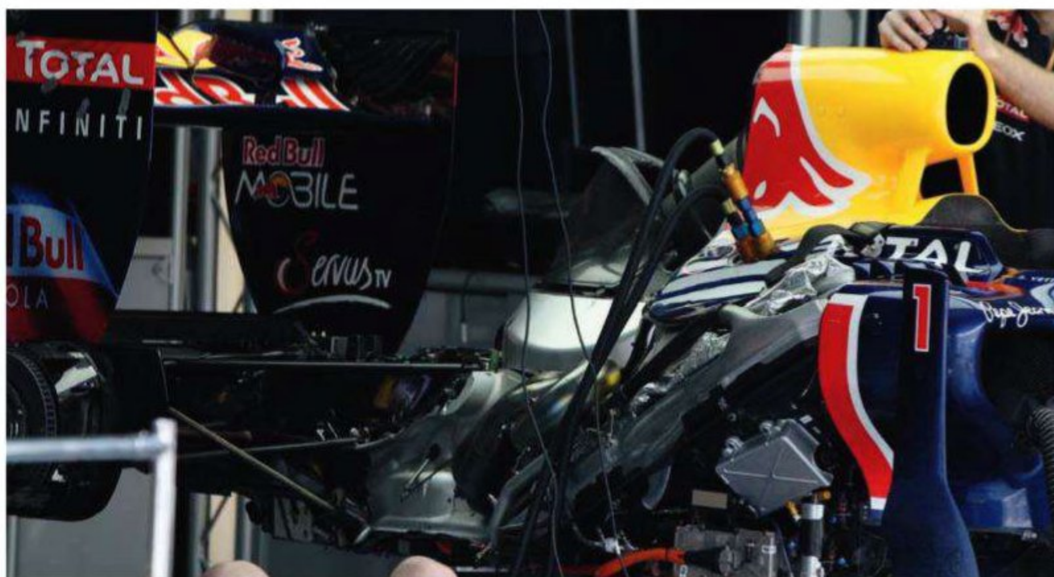
The RB7 has its KERS hardware mounted alongside the gearbox housing at the rear of the car, something that plays a significant factor in the car’s weight distribution. Such layouts are banned under the new-for-2014 rules
