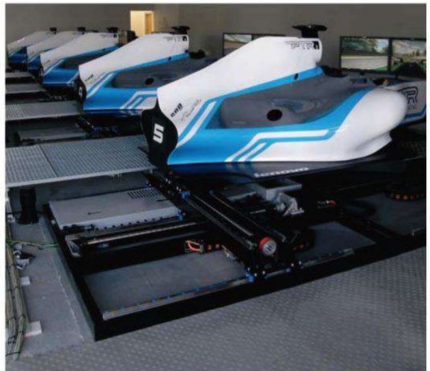
Ball Racing Developments' (BRD) Pure Tech Racing centre in the UK offers a multi-driver simulator experience, with minor yaw and vertical movement
