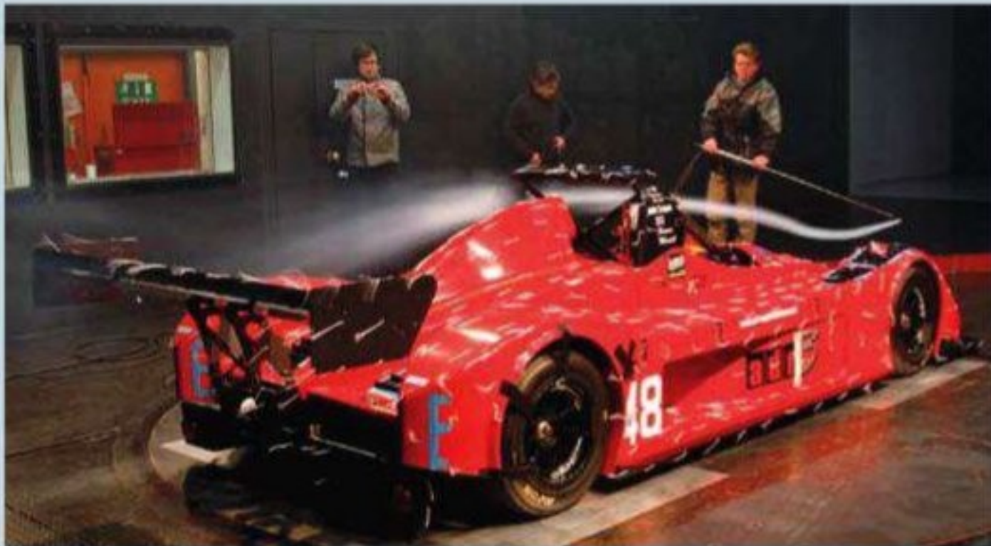
The wool tufts in the centre of the wing's trailing edge show how the engine inlet snorkel affected the airflow downstream
