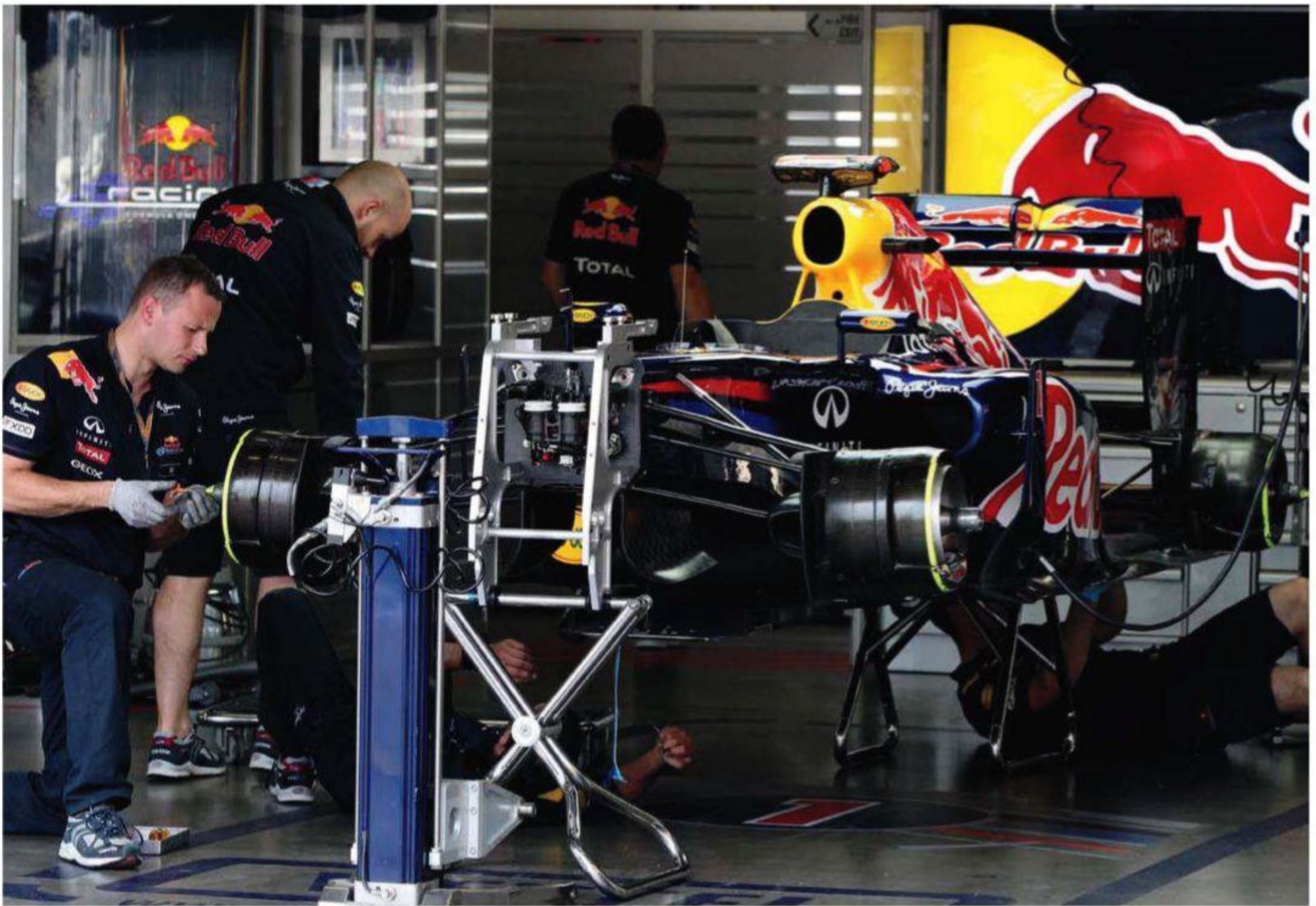
Red Bull use Brembo brakes on the RB7. The RB5 suffered with brake wear issues in 2009 but Newey says the technology has moved on since then: 'I think what you've seen along the grid is much more sophisticated disc drilling patterns than in 2009. In our own case, we supply our own spec to Brembo, but equally, Brembo has developed its own baseline spec in the intervening years, so their baseline spec is also to a high standard'
