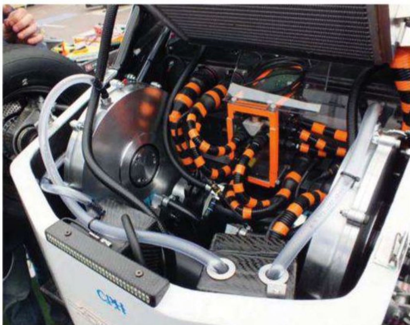
The TU Delft car was powered by twin AMK DT5 electric motors and lithium ion polymer batteries. It was also very light, weighing in at just 178kg
