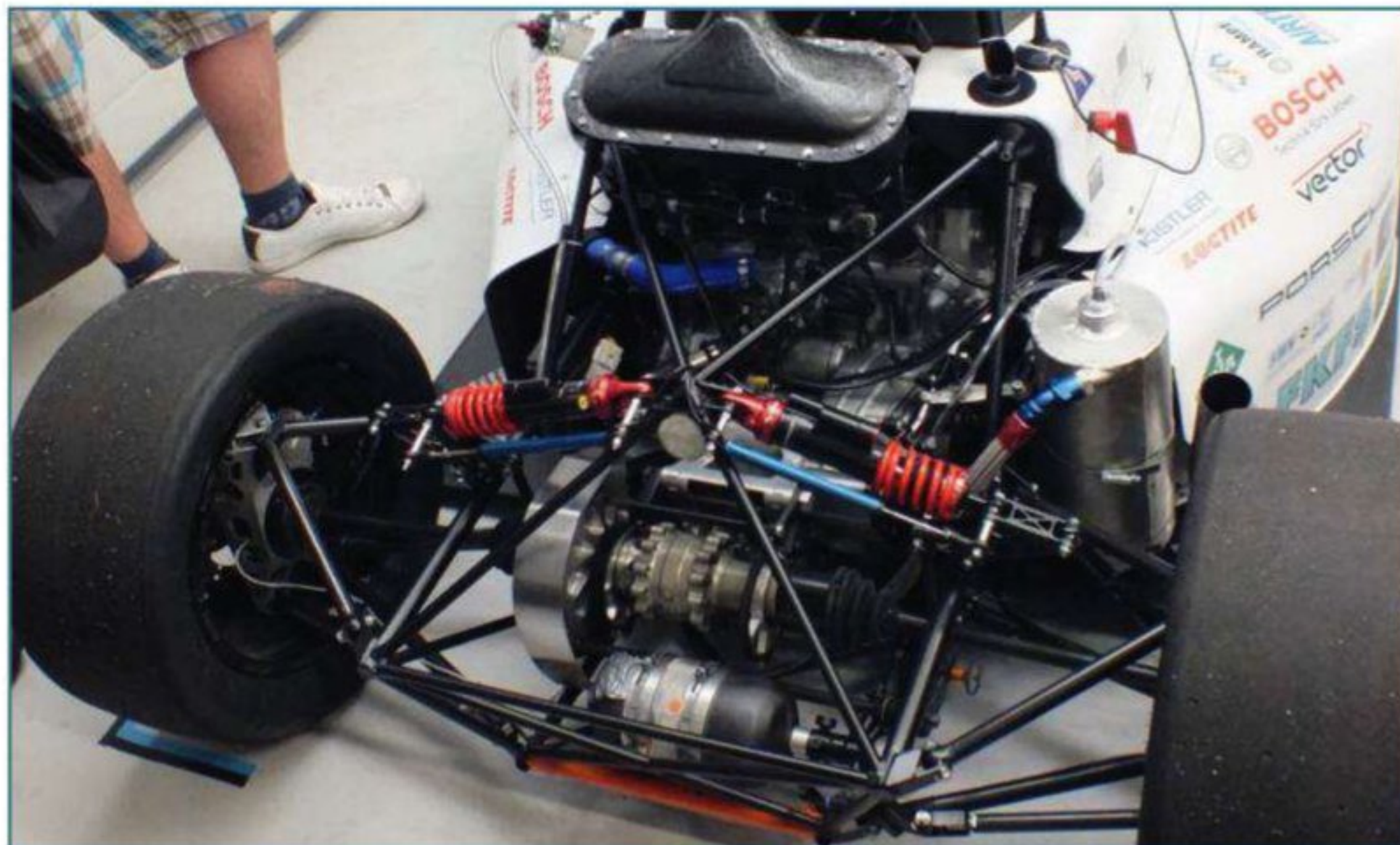
The neat, tidy design of the Stuttgart entry used a tubular rear frame and a composite monocoque front, with the emphasis on ease of maintenance
