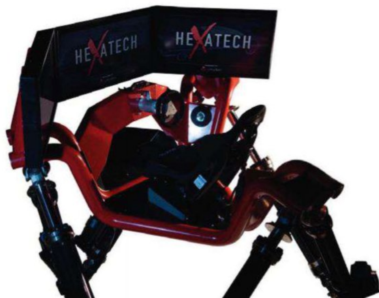
Cruden's Hexatech motion platform offers six degrees of freedom and forms the basis of more advanced simulators
