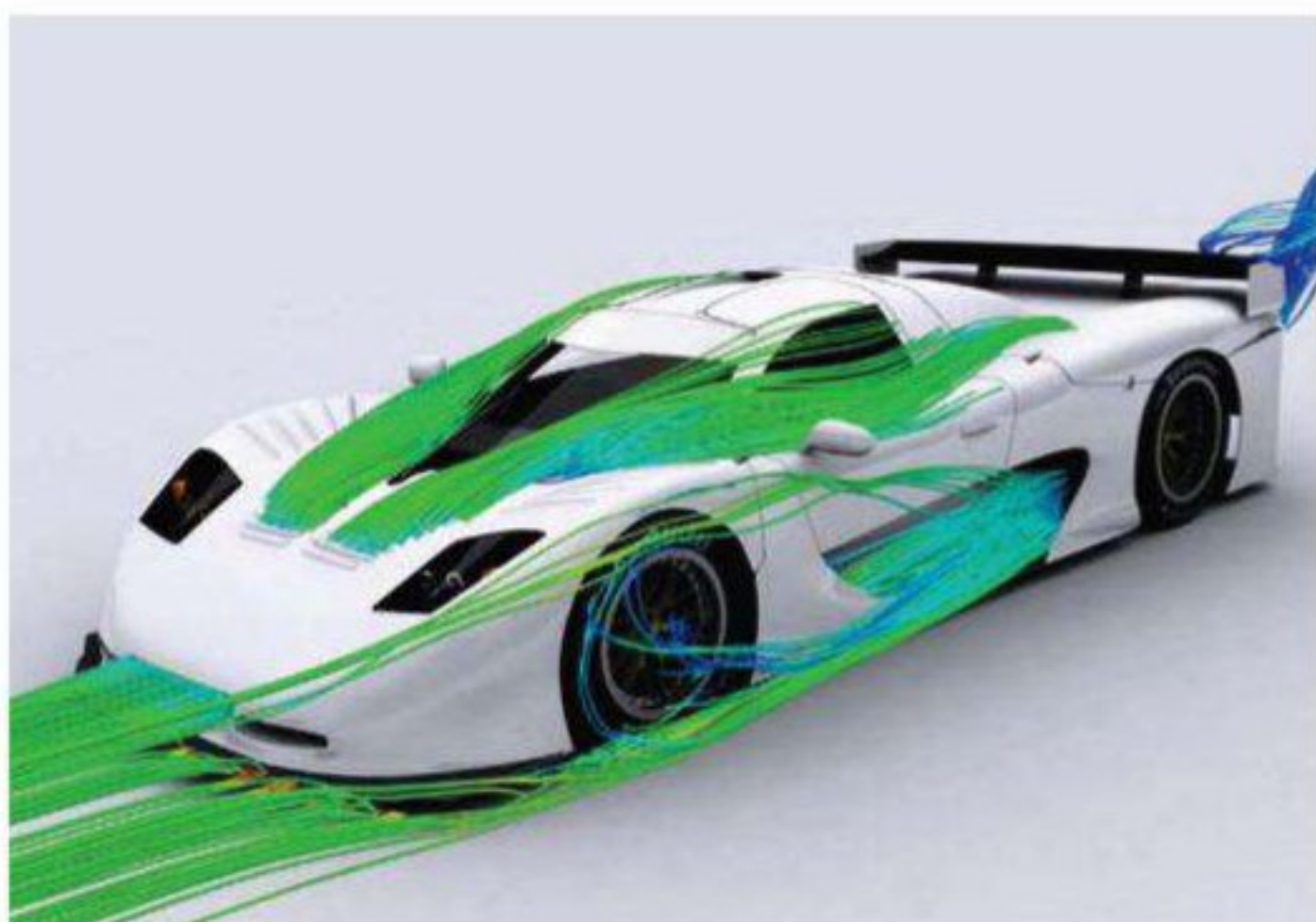
CFD project undertaken with TotalSim yielded benefits. Here we see streamlines viewed from the front of the car
