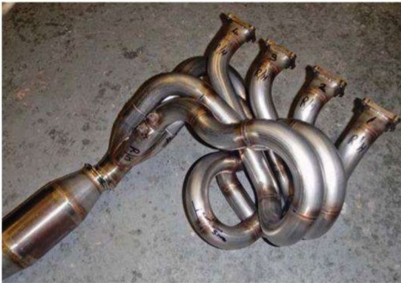
Each four-into-one exhaust system had to feed through a JAF-specified catalytic converter, but no silencer
