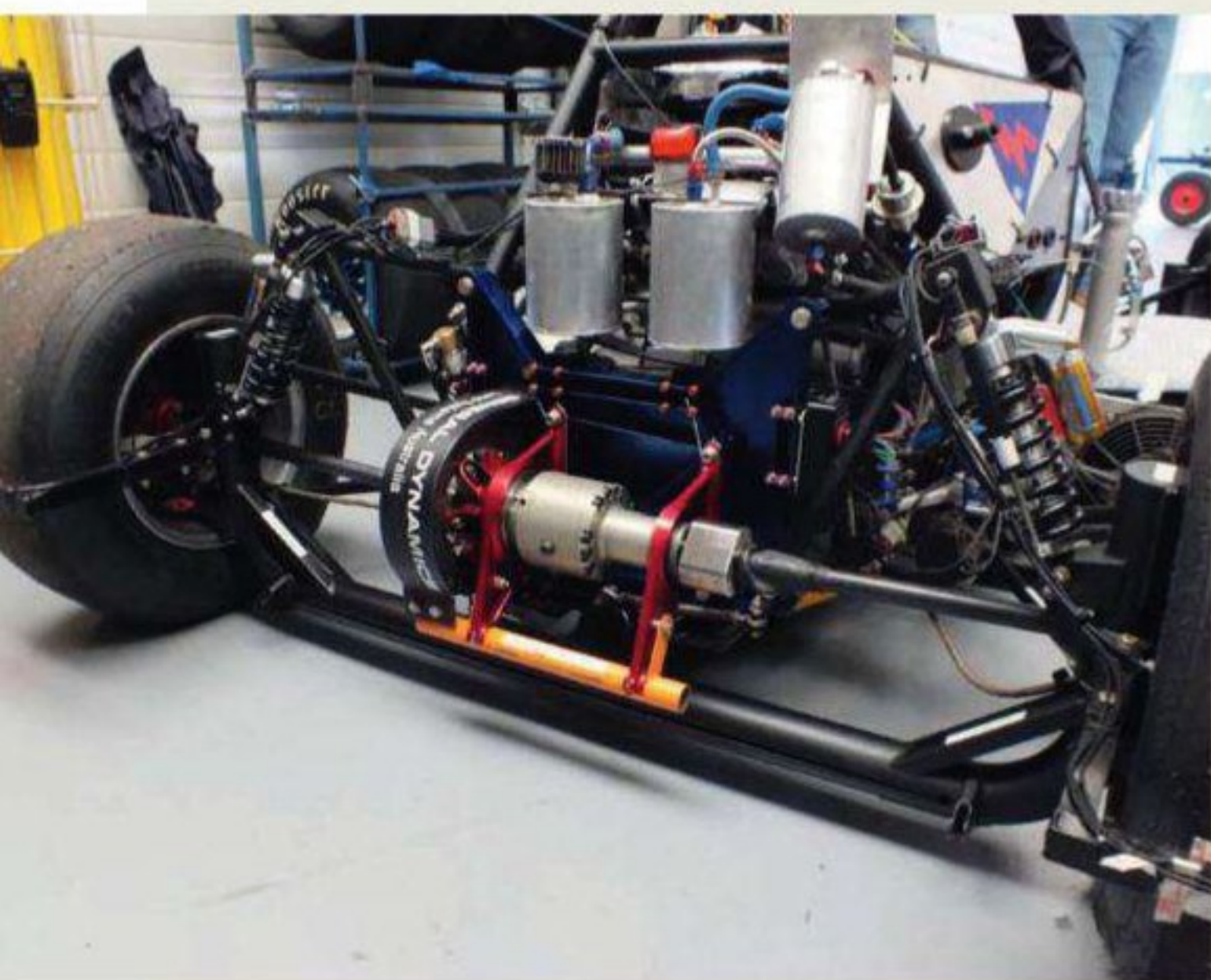
A radical re-think of the use of resources led to the inclusion of a De Dion beam rear axle, greatly simplifying the rear suspension assembly and making manufacture quicker, easier and cheaper. It worked, too
