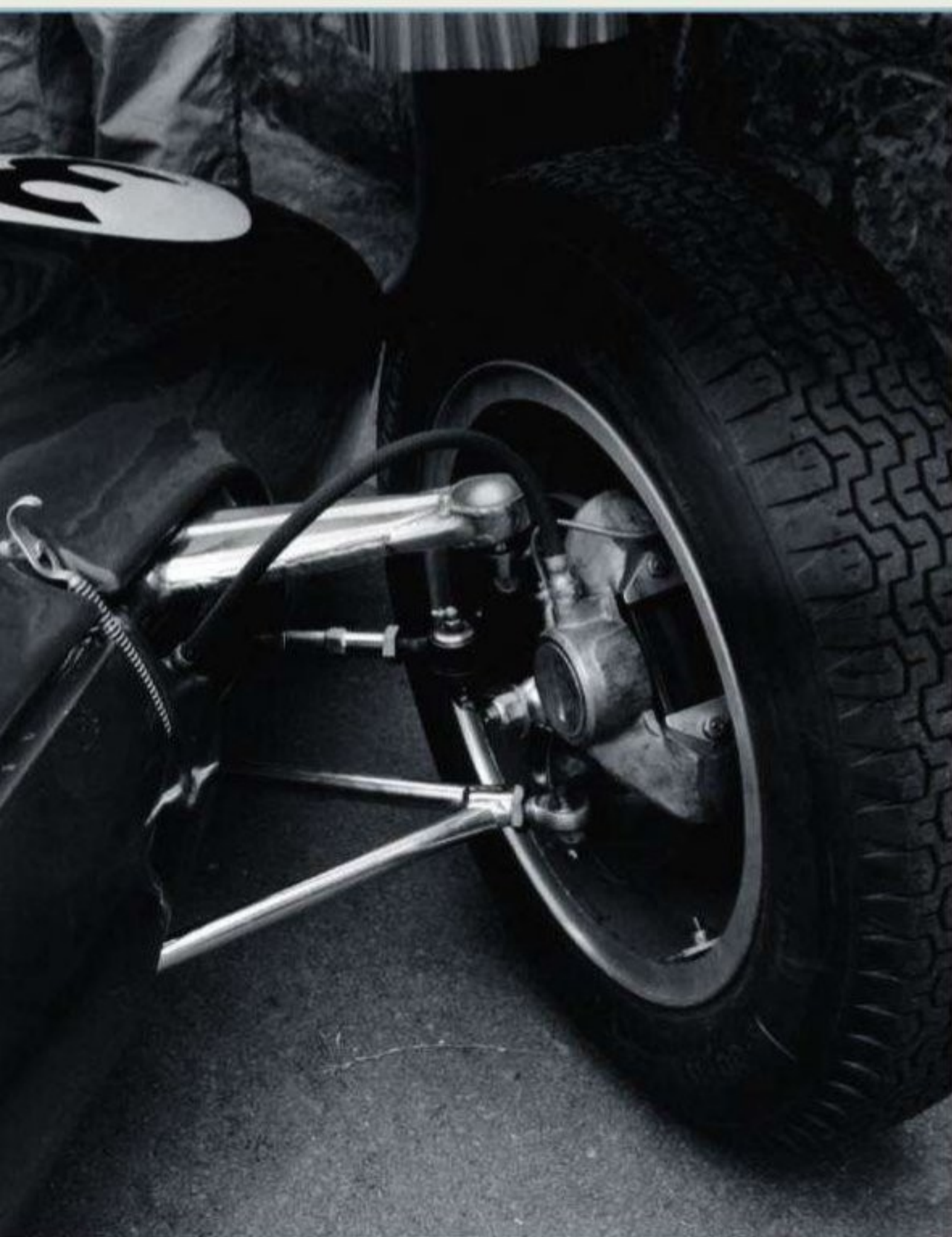
The basic rule of thumb that says the upper wishbone should be 2/3 of the length of the lower one still holds true
