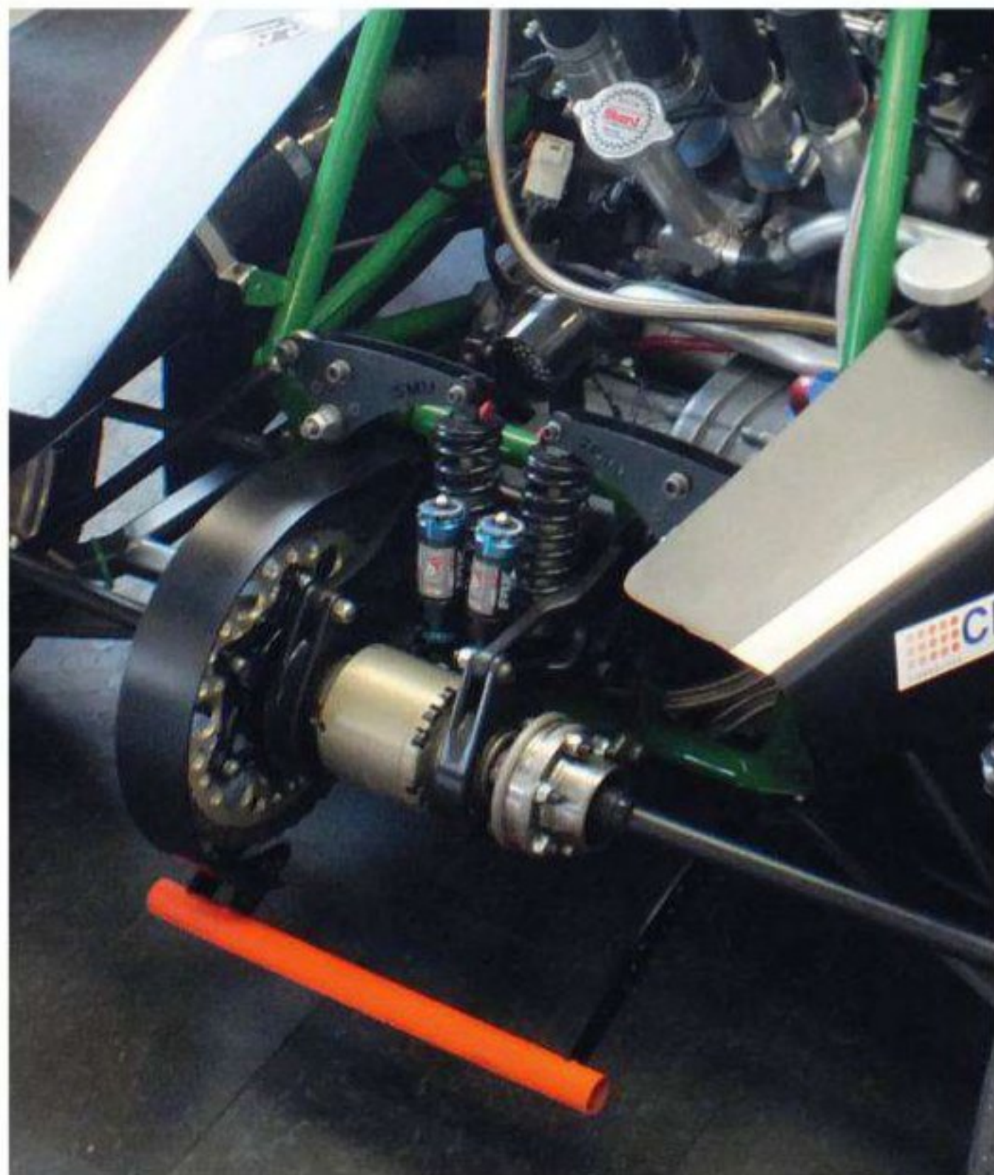
The Drexler diff has been a favourite for a long time. This is the previous generation Drexler diff that is still in use with some teams today
