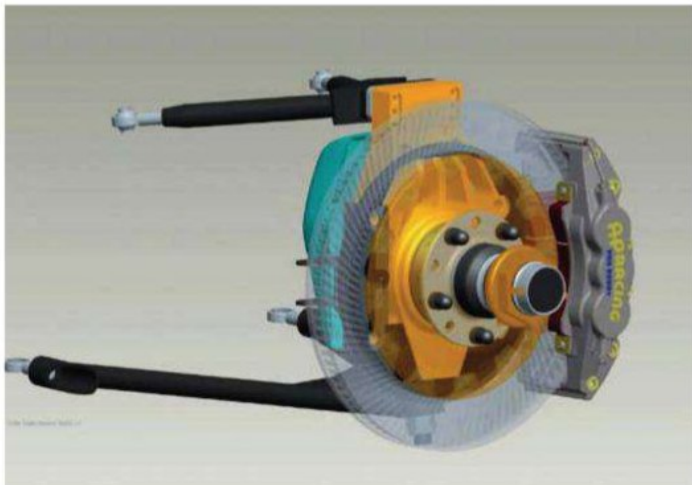
Double wishbones front and rear are used with outboard spring dampers
