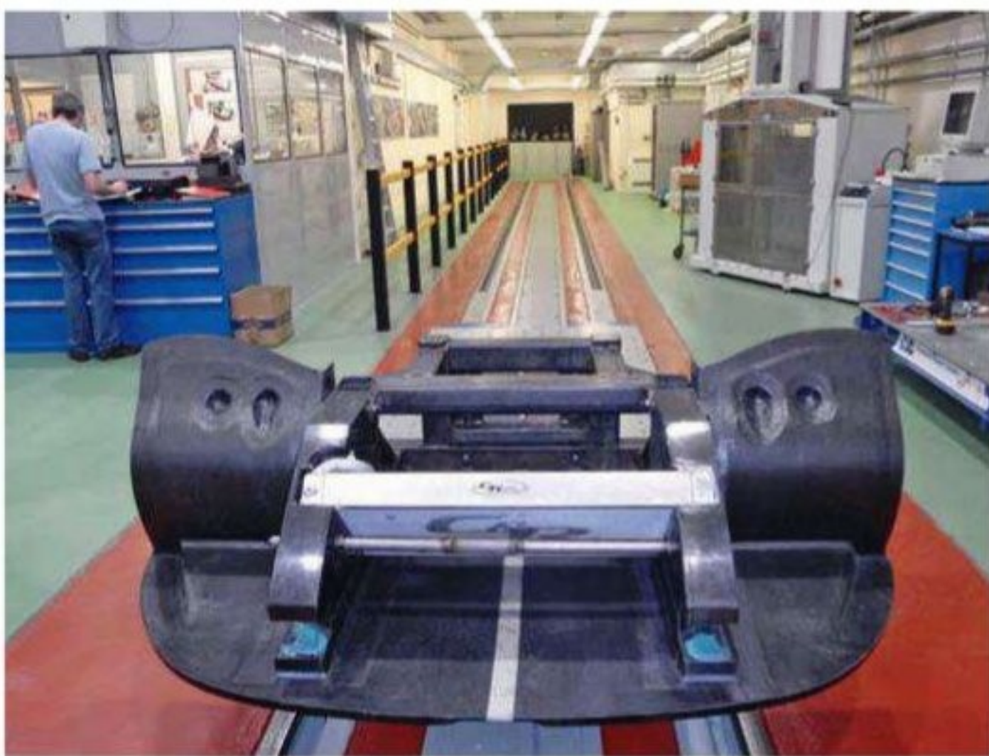
Such was the severity of the frontal impact requirements that the test had to be done at Cranfield Impact Centre in two stages
