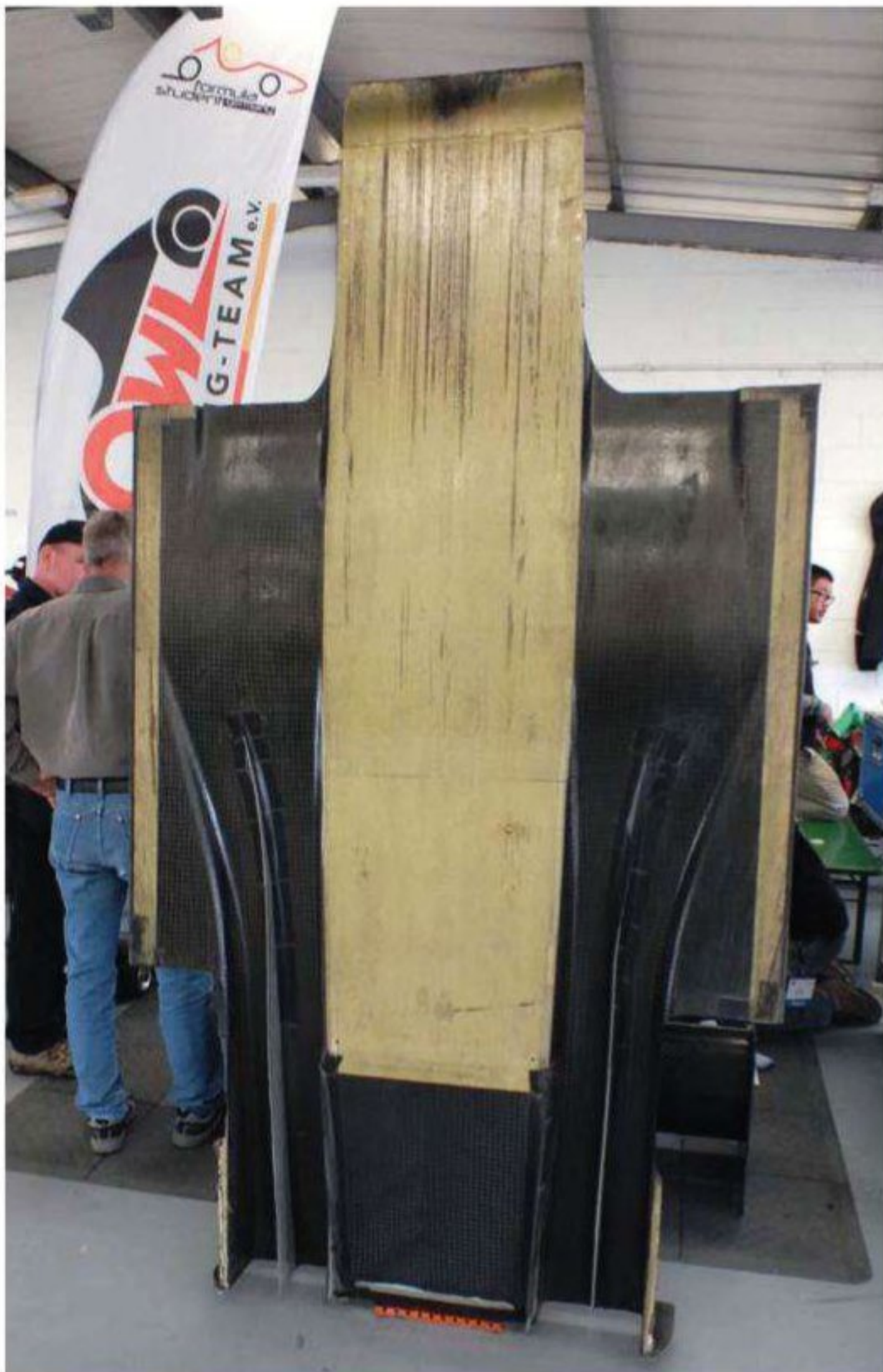
Convinced by CFD and lap time simulation work of its benefits, the GFR entry also had this downforce-generating underbody
