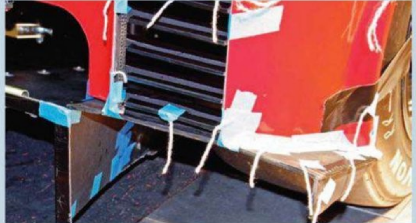
It was hoped that opening the rear of the rear wheelarches and adding ramps at the back would collectively reduce drag and add rear downforce
