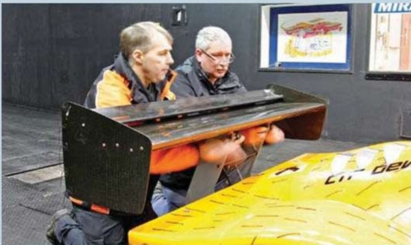
Reducing the rear wing angle overall shifted the balance
