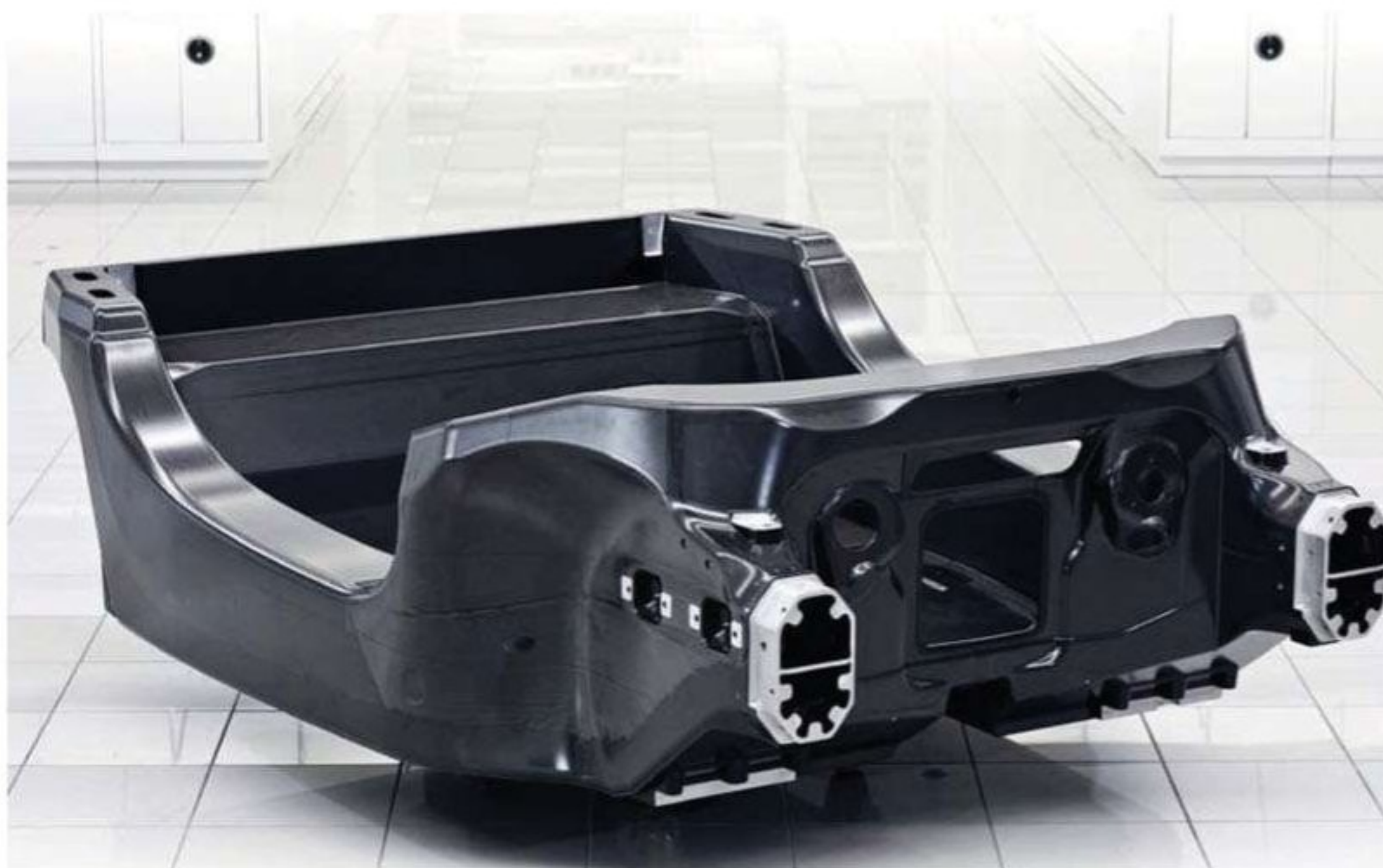
MonoCell, as developed by Carbo Tech and, unusually, for a carbon fibre product, manufactured by robots
