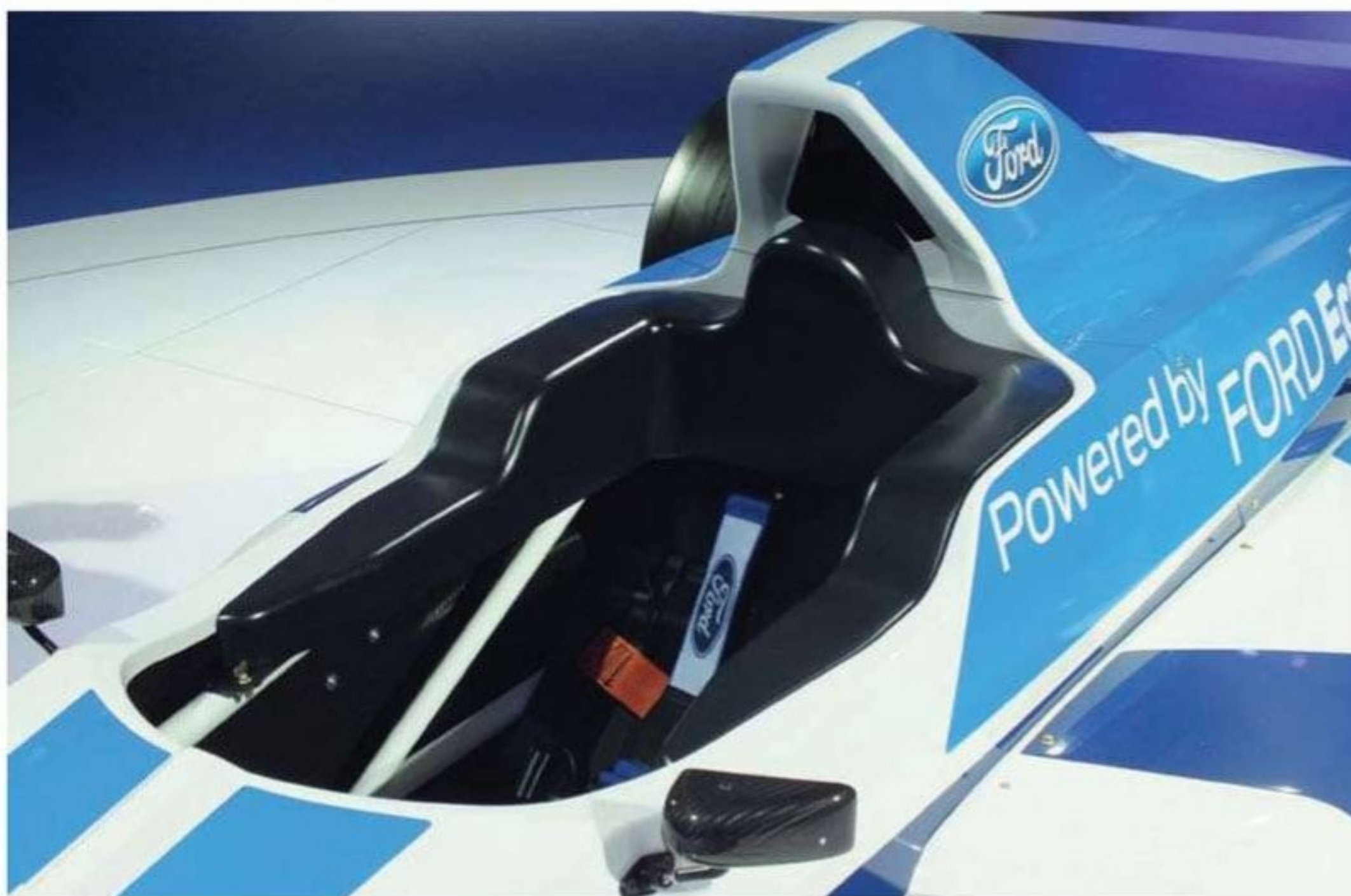
The cockpit aperture is a spec part and includes an F1-style head restraint, removable seat and anti-intrusion bars
