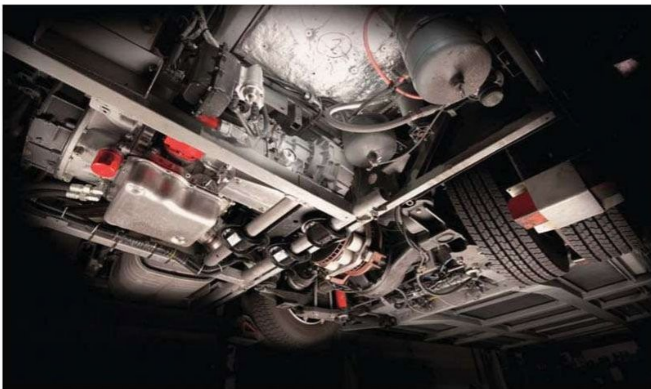
The Ricardo-Torotrak system is being tested in UK-built Optare Solo buses. The system has been designed for incorporation into new builds or retro-fitting into existing ones and offers significant efficiency gains in both
