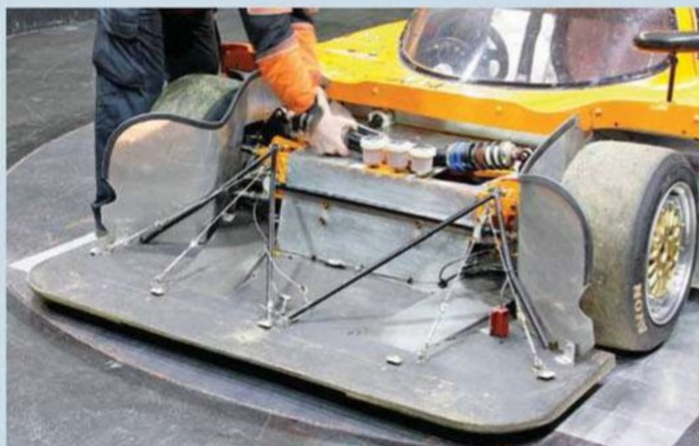
Lowering front ride height shifted the aerodynamic balance significantly
