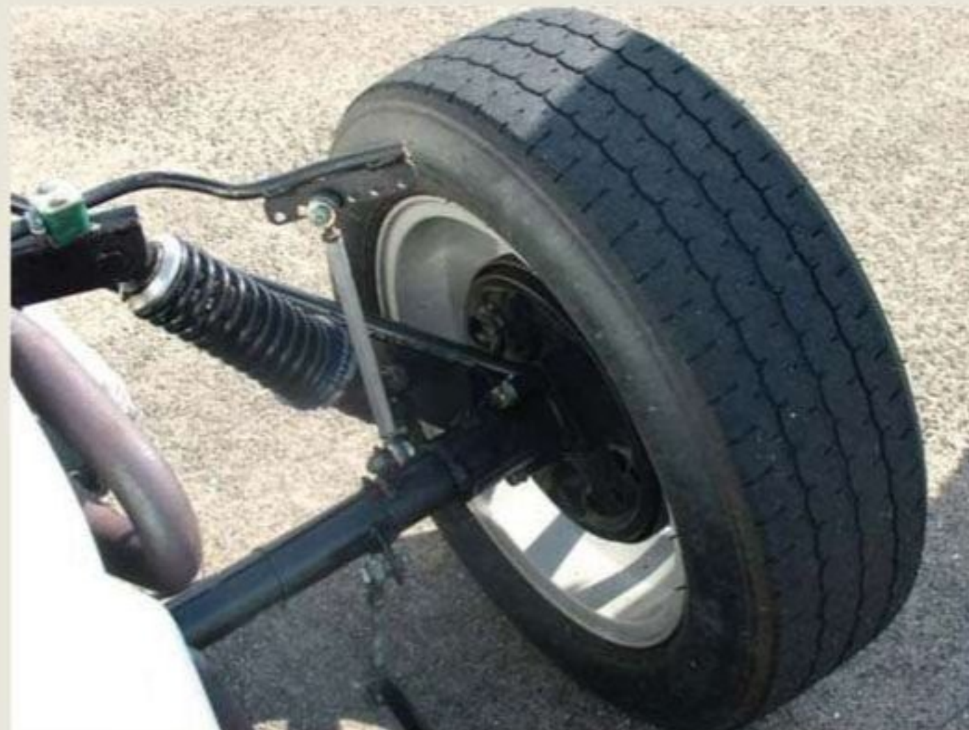
Rear anti-roll bars on European Formula Vees are soft, and adjustable, so are used as a fine tuning device, in combination with the fixed front bar
