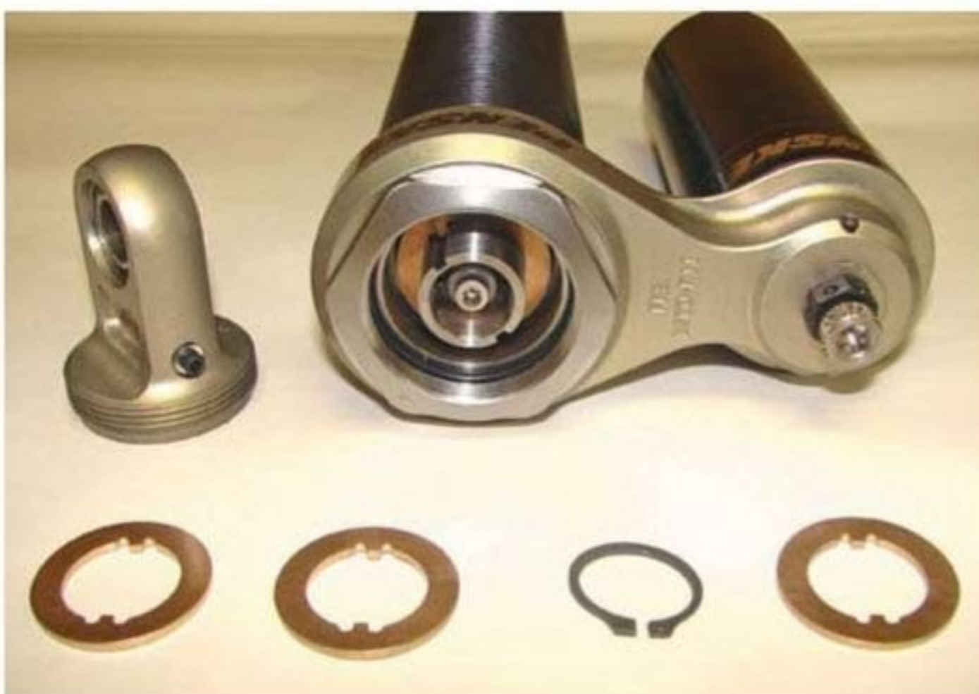
Removing the inerter weight to change for another is a simple matter of unscrewing the top eye and cap
