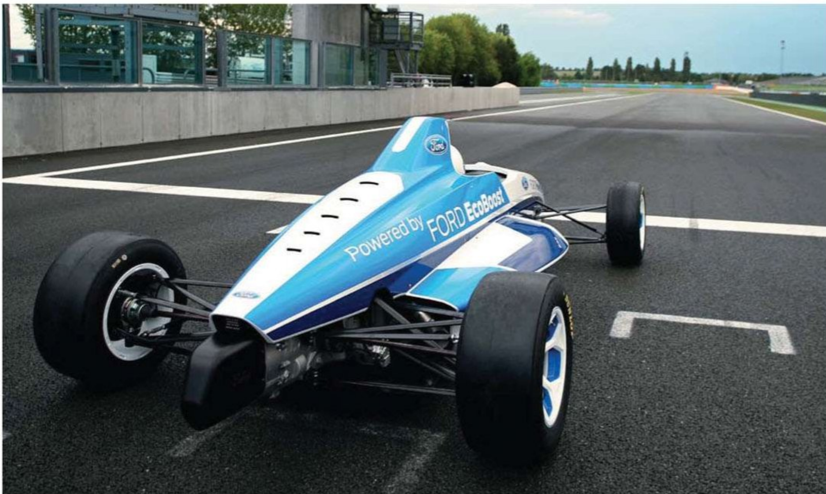
The launch car is Ford's own interpretation of how the new car will look and is based on the Mygale tubular steel chassis that will remain in use. Body design and manufacture will be free but with certain fixed parameters such as the sidepod inlets, front and rear impact structures and a flat floor
