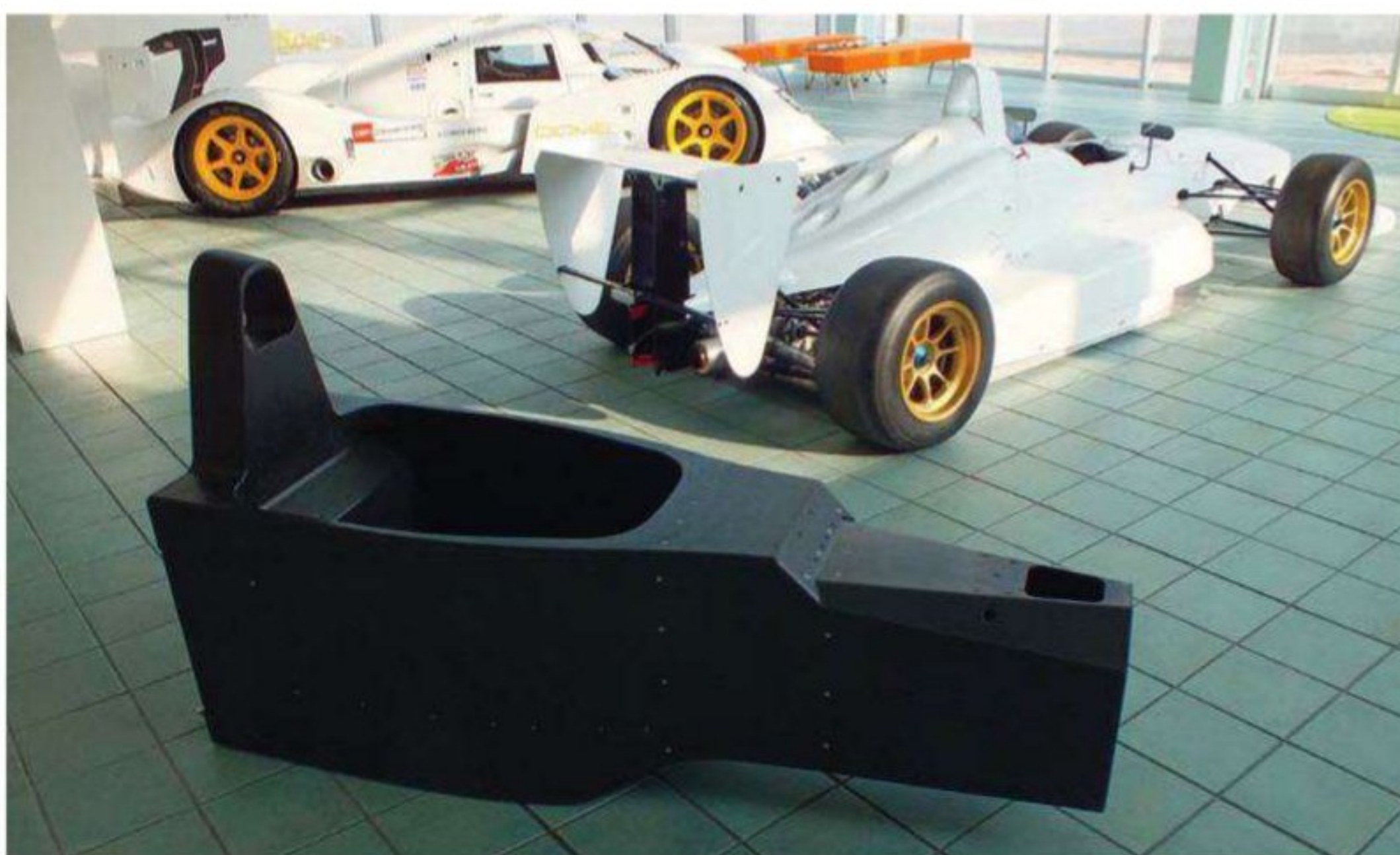
The Uova 4 carbon tub was designed all along to be versatile, enabling it to be used in series outside of Formula 4. Advanced aviation technology was used in its construction so it is as smooth on the inside as it is on the outside
