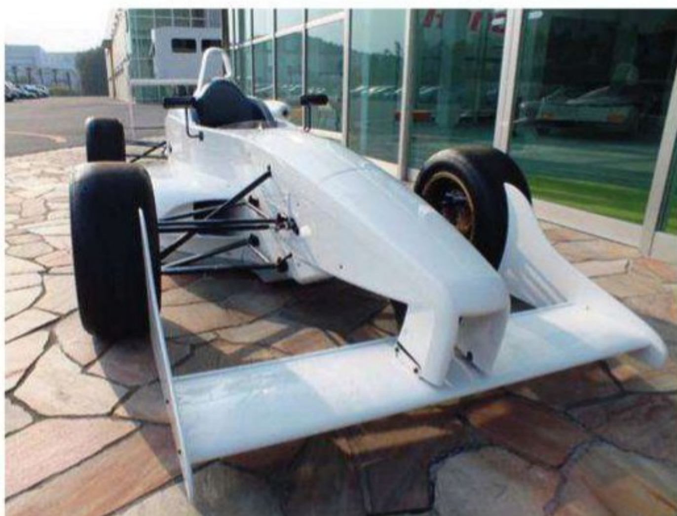
The Zap F108, designed as a styling exercise by Dome founder, Minoru Hayashi. Dome produces the monocoque but the car is built by Zapspeed
