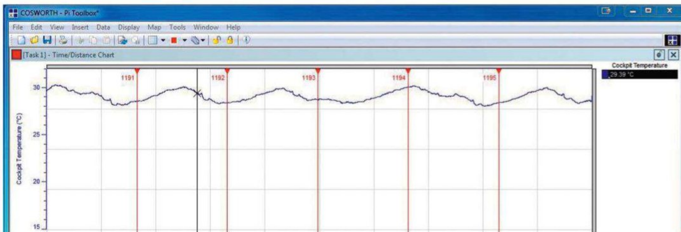
Figure 2: temperature control in a closed-cockpit coupé. The air con is switched on at 30degC and off at 28degC to create a stable environment for the driver
