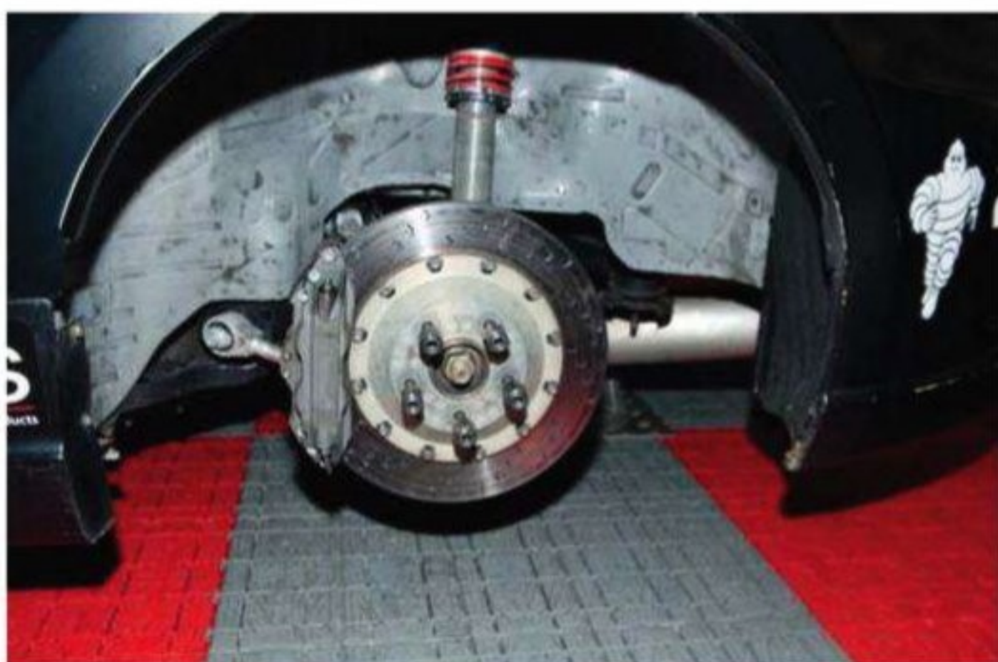
Building adjustability into the rear suspension, and equipping the cars with Bilstein dampers and Alcon brakes is part of the RJN Motorsport upgrade
