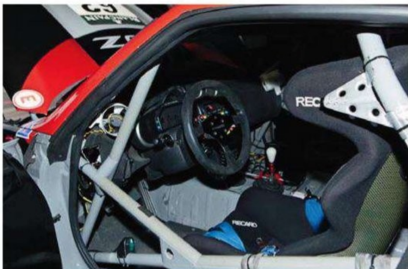
Lightweight body has minimal exterior modifications, but ‘shell is seam welded and a substantial rollcage added
