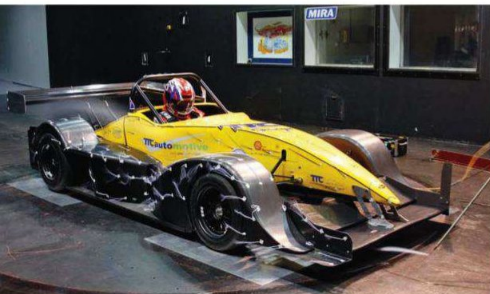
Unusually among sports racers, the Force LM offered adjustable front and rear wings. Notice the flow from the front wing encountering the rear wing
