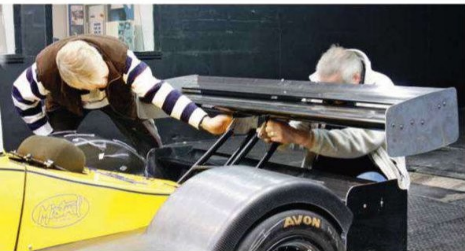
The rear wing angle was increased overall, shifting balance significantly
