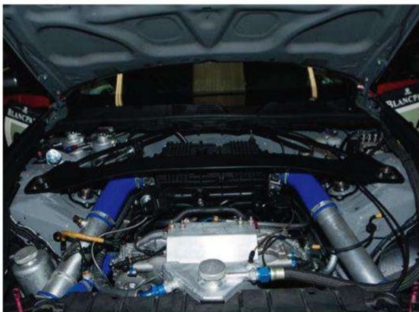
3.8-litre V6 (4.0-litre for the longer Endurance races) comes direct from NISMO in Japan as a complete package. Power output is said to be 440bhp
