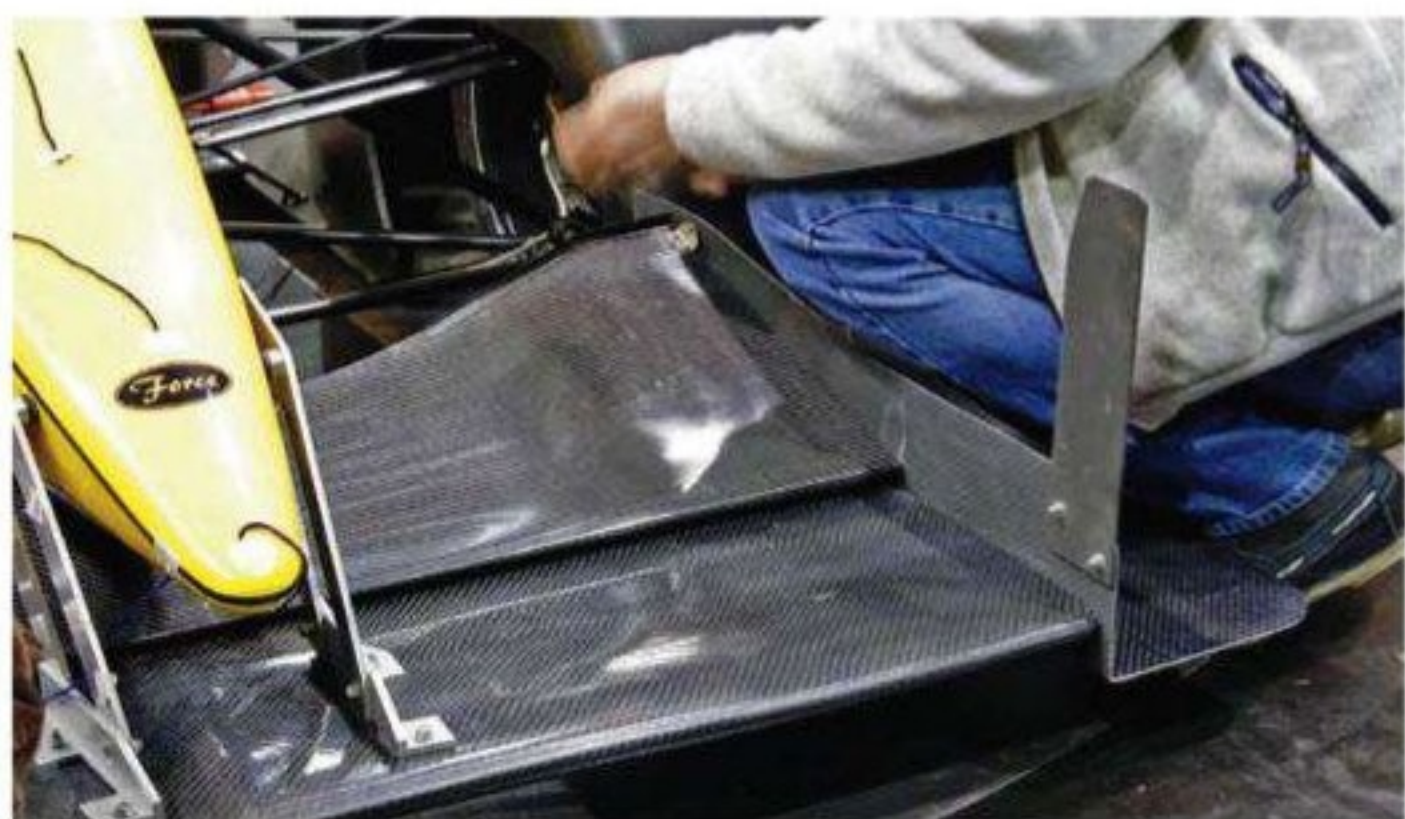
Reducing front wing flap angle had a significant effect, not just at the front
