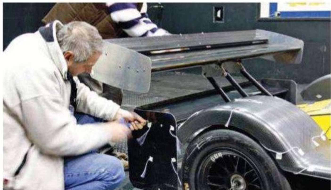
Increasing the lower rear wing angle made a minor difference
