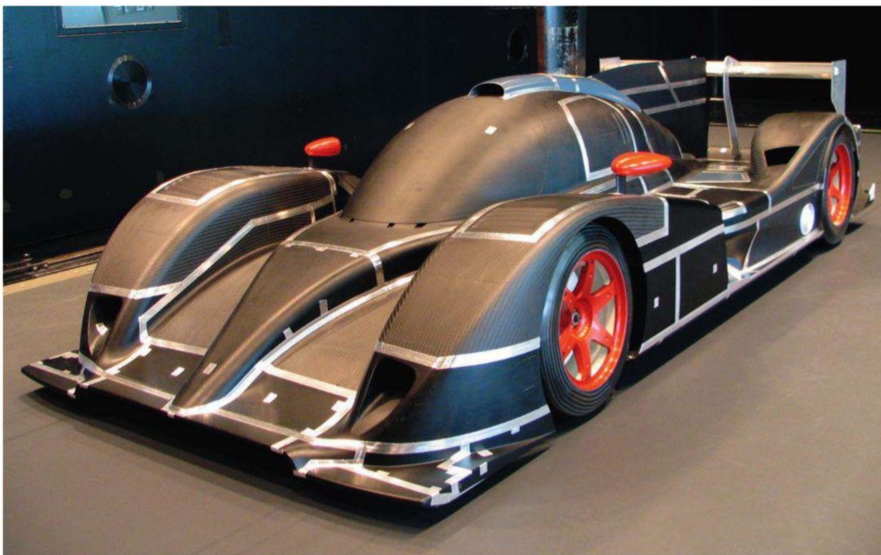
The Dome S102 scale wind tunnel model, updated to 2011 spec, with mandatory fin and narrow rear wing package
