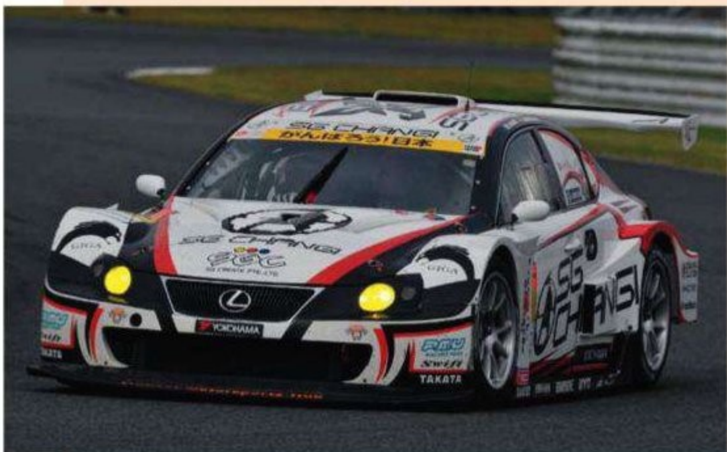
From Toyota's Lexus stable comes this radically re-worked IS350, which uses the GT500 engine, breathing through a smaller restrictor
