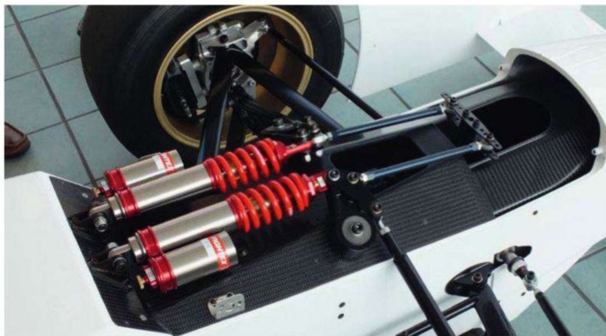
Suspension mounting points on a chassis that has no honeycomb core require metal load bearing plates to be added on the inside of the tub. Note the pushrod-actuated Toda Racing dampers. Upright design is also free
