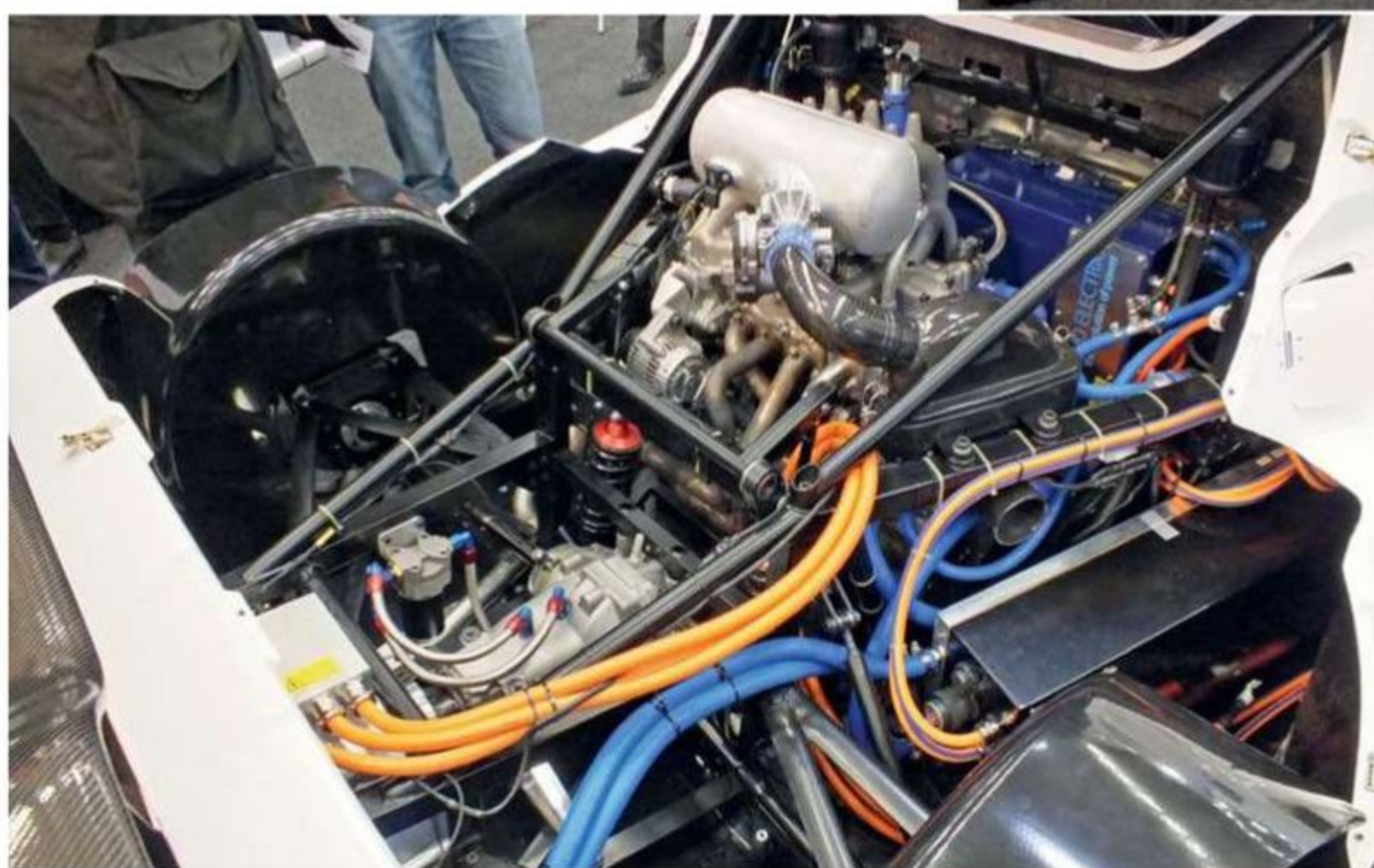
One of the few parts to come from outside the Magny Cours area was the EV powertrain from TMG in Cologne. The bespoke 1.0-litre engine is by ORECA
