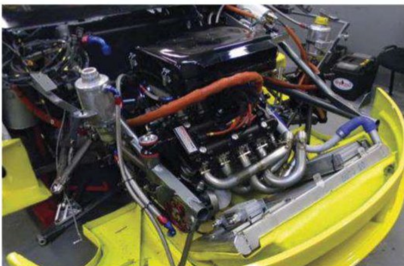
TC2000 series cars use a bolt-on front subframe, which previously housed a highly tuned Duratec V6. The Radical V8 is therefore a significant departure
