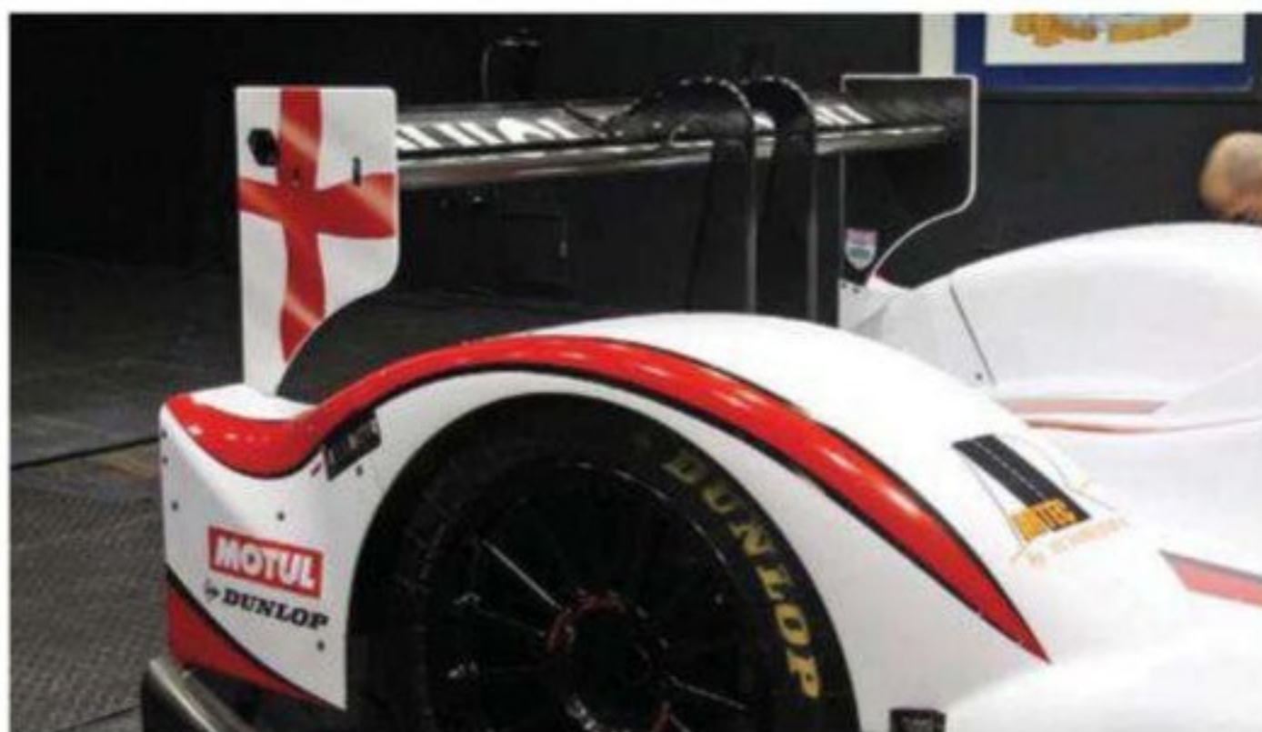
The swan neck-supported rear wing was well cambered and obviously fairly potent
