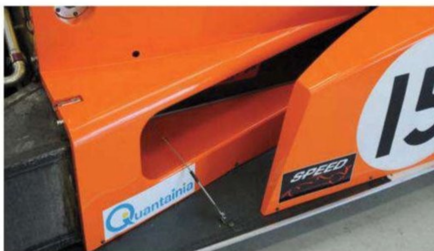
Changes made to the original Peter Elleray-designed aerodynamics led to problems with airflow to the sidepod-housed radiators
