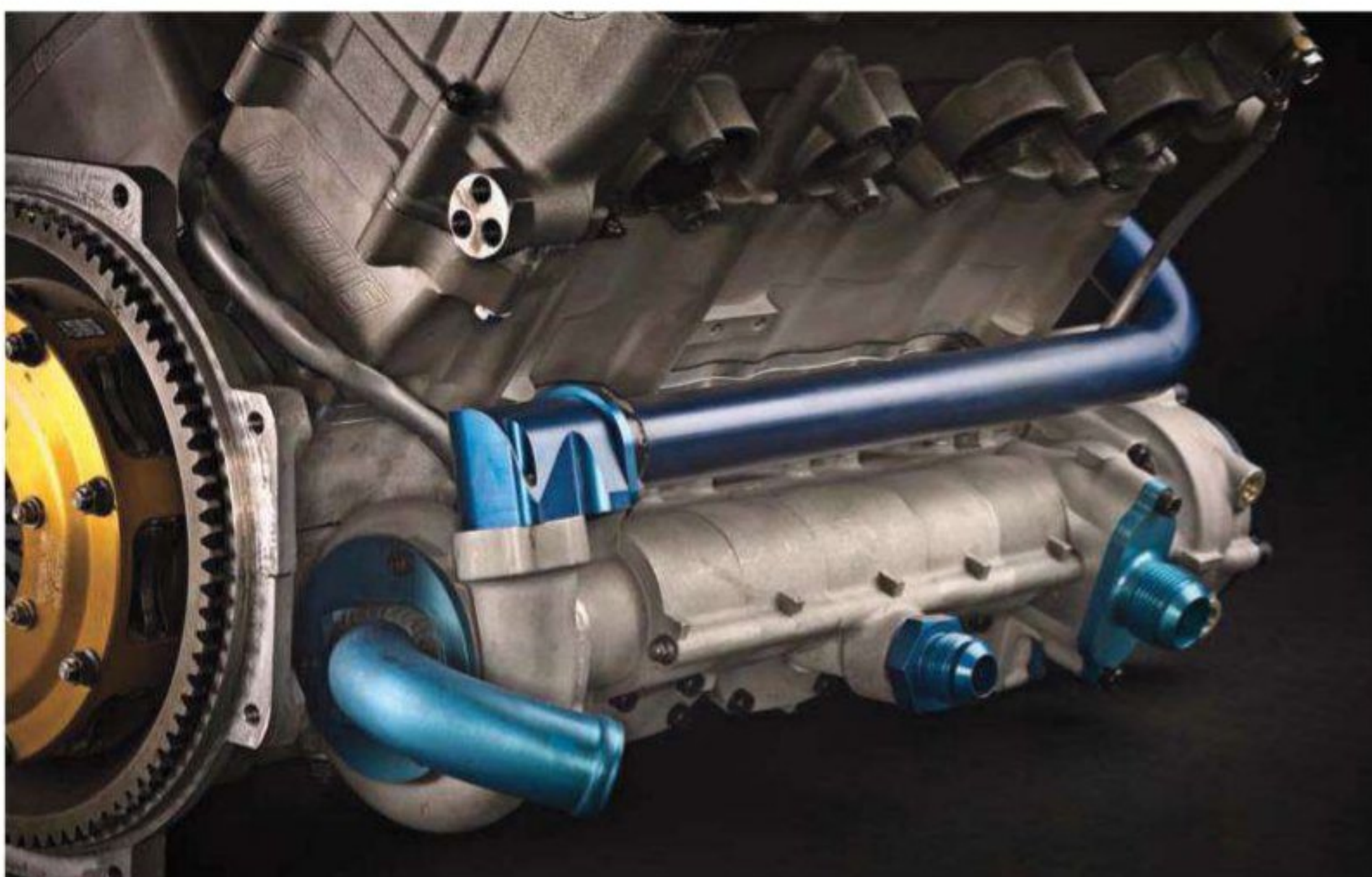
Lubrication is taken care of by twin pumps and a four scavenge pump dry sump system
