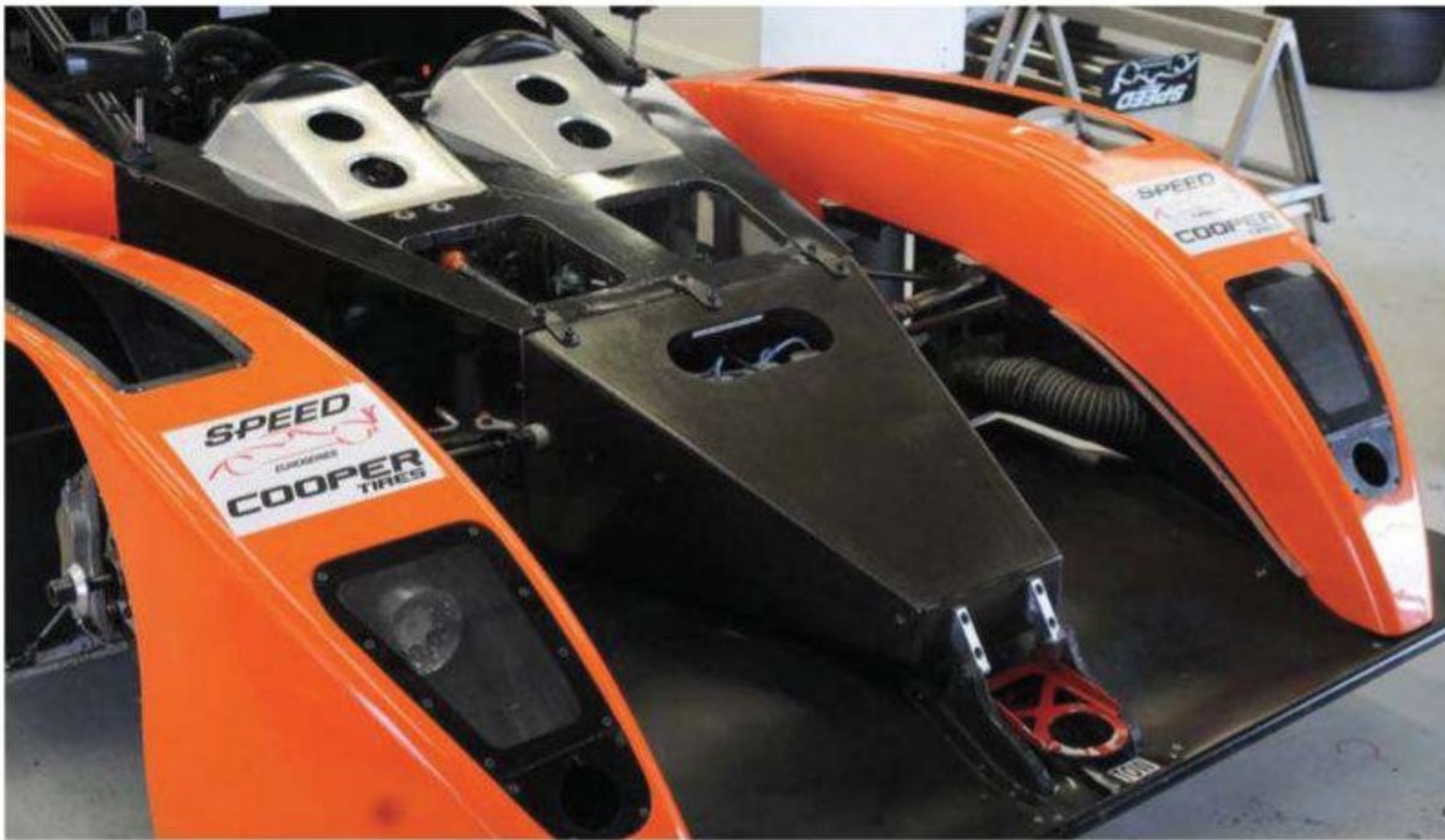
FIA-regulated CN formula crash box structure is a bolt-on carbon piece, sitting above a very large front diffuser
