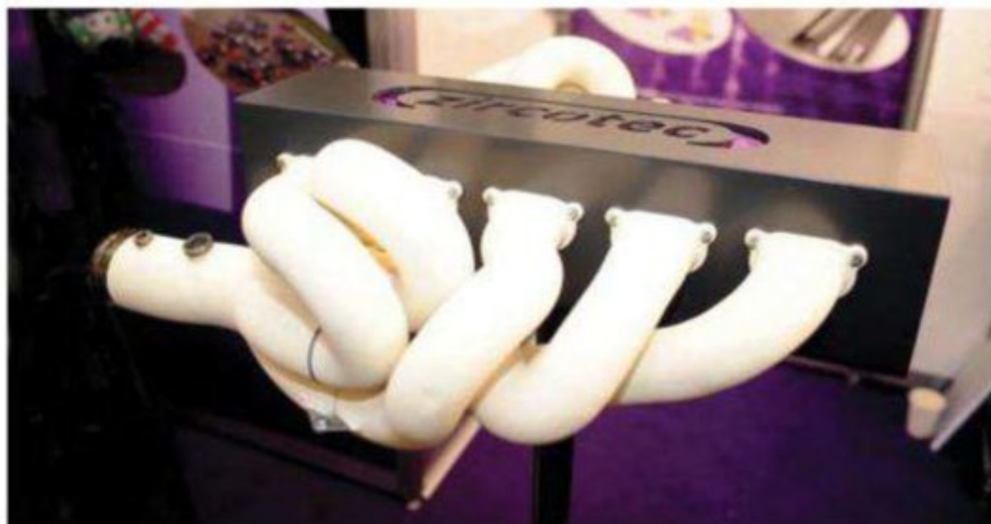
Zircotec's performance exhaust coatings remain an industry standard
