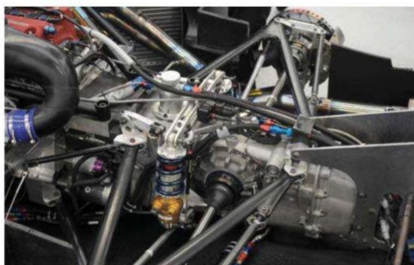
One of the problems encountered was using non-specific parts. The WF03 has pull-rod suspension but used a Hewland FTR gearbox designed for push-rod applications, meaning a conversion bracket had to be made. It broke
