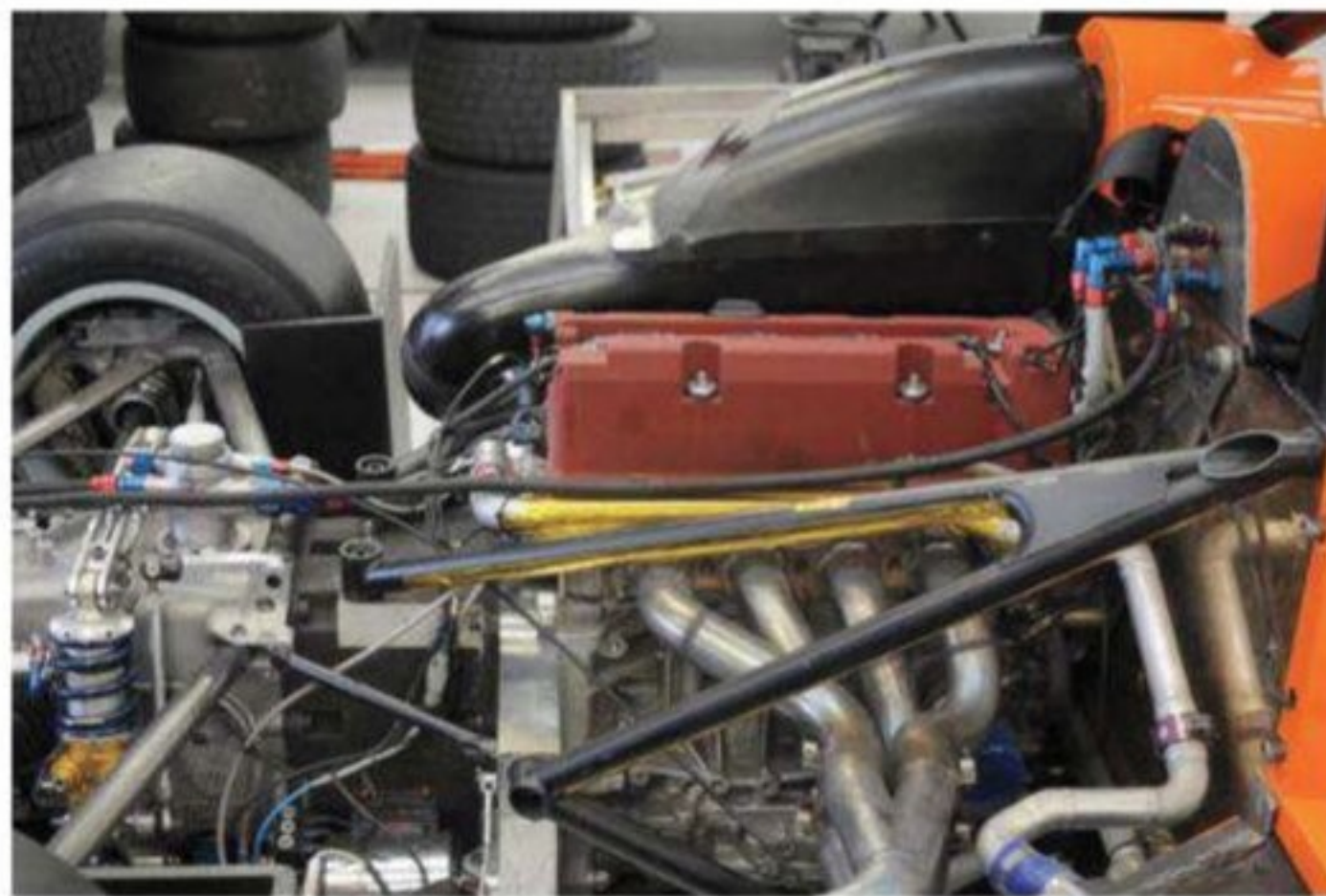
Engine is a spec, Mugen-built, 2.0-litre four producing around 238bhp
