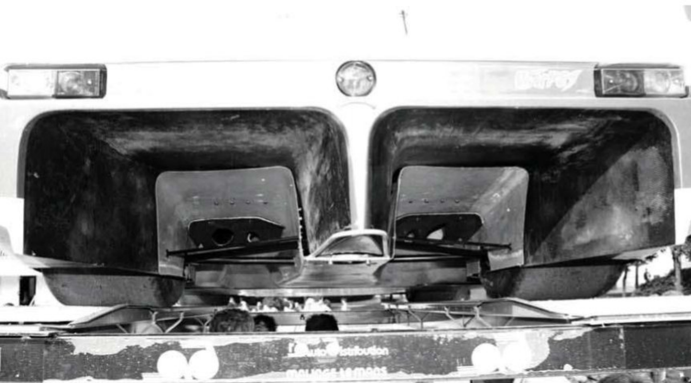
The Le Mans scrutineering hoist reveals the WM's exhaust blown, low drag, low downforce underwing
