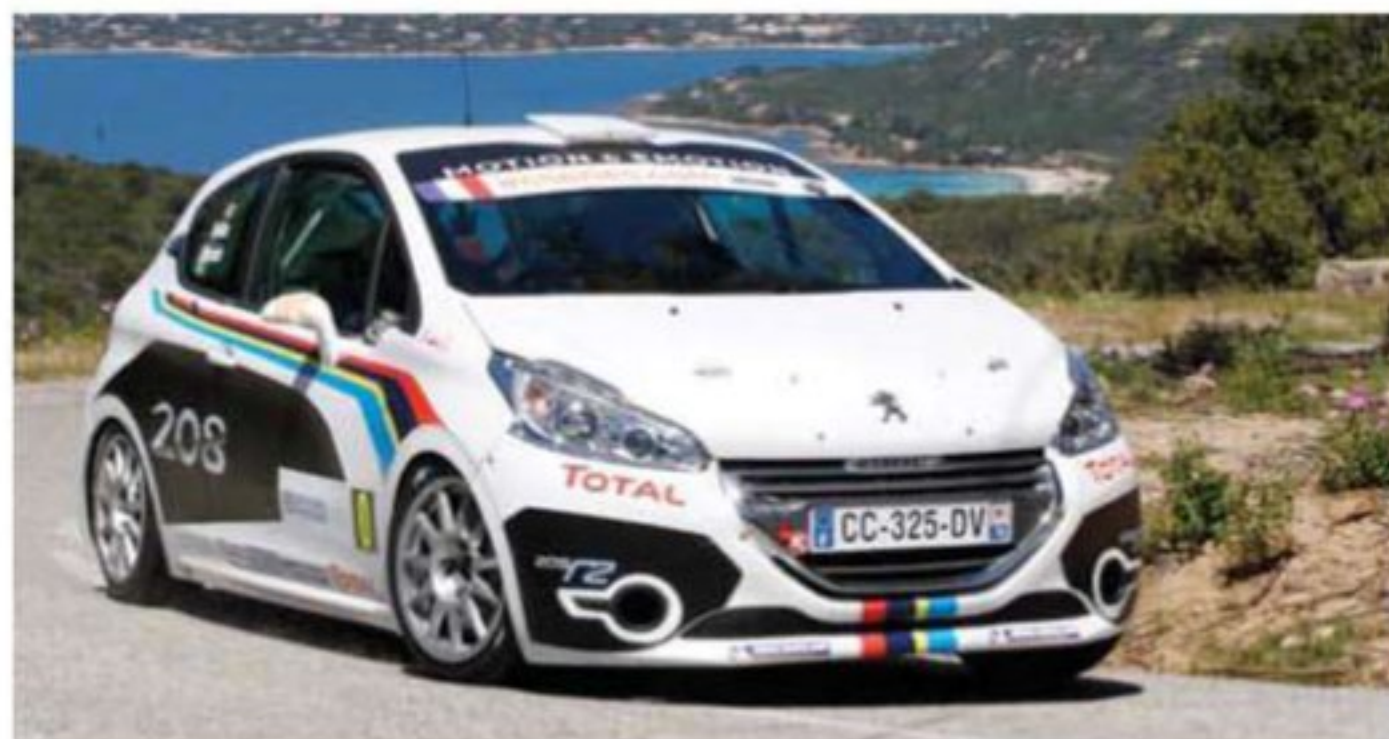
208 R2 will use a 185bhp, naturally-aspirated, 1.6-litre, VVT engine
