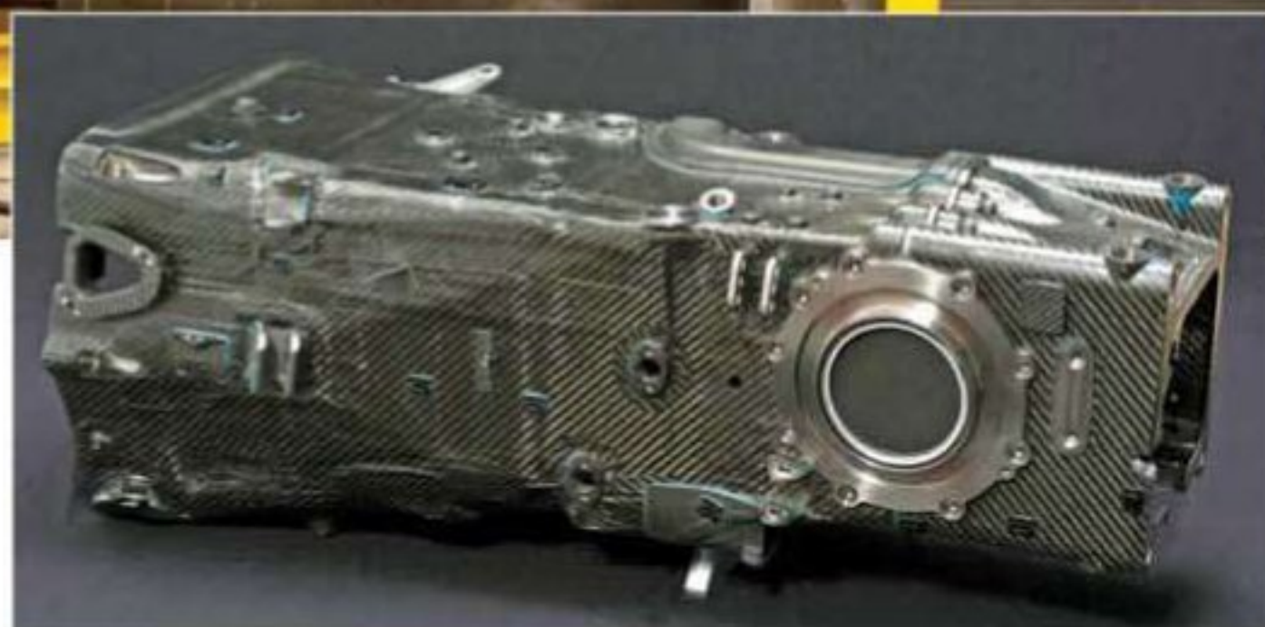
Carbon fibre gearbox casing is another crucial weight saving
