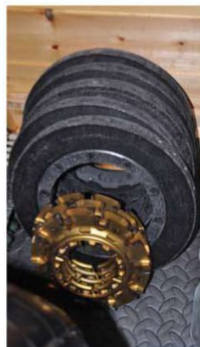
Though a full set of carbon /carbon brakes have been sourced, driver ability dictates the use of steel
