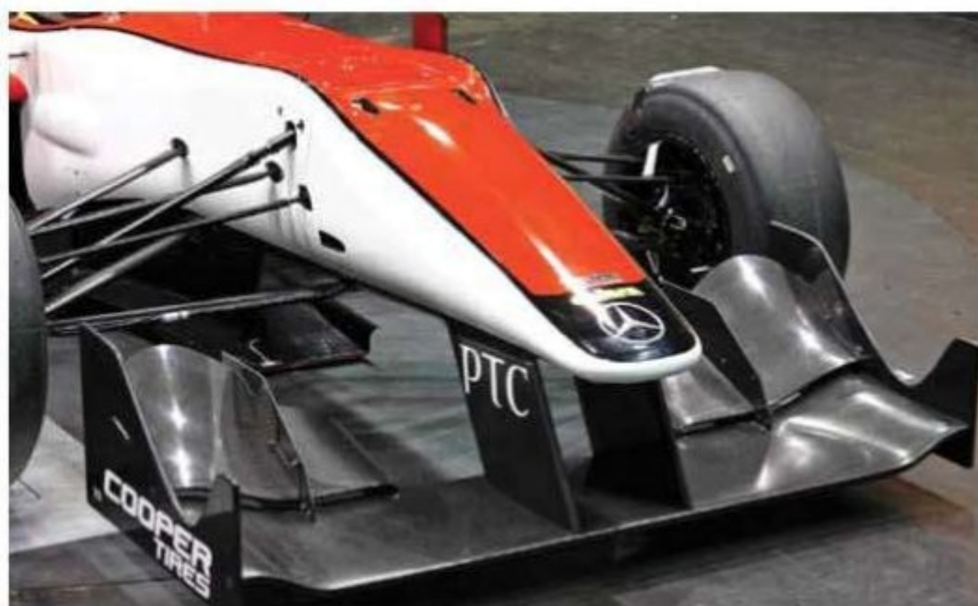
The F312's front wing features a larger main element chord and larger flap area than the previous car's
