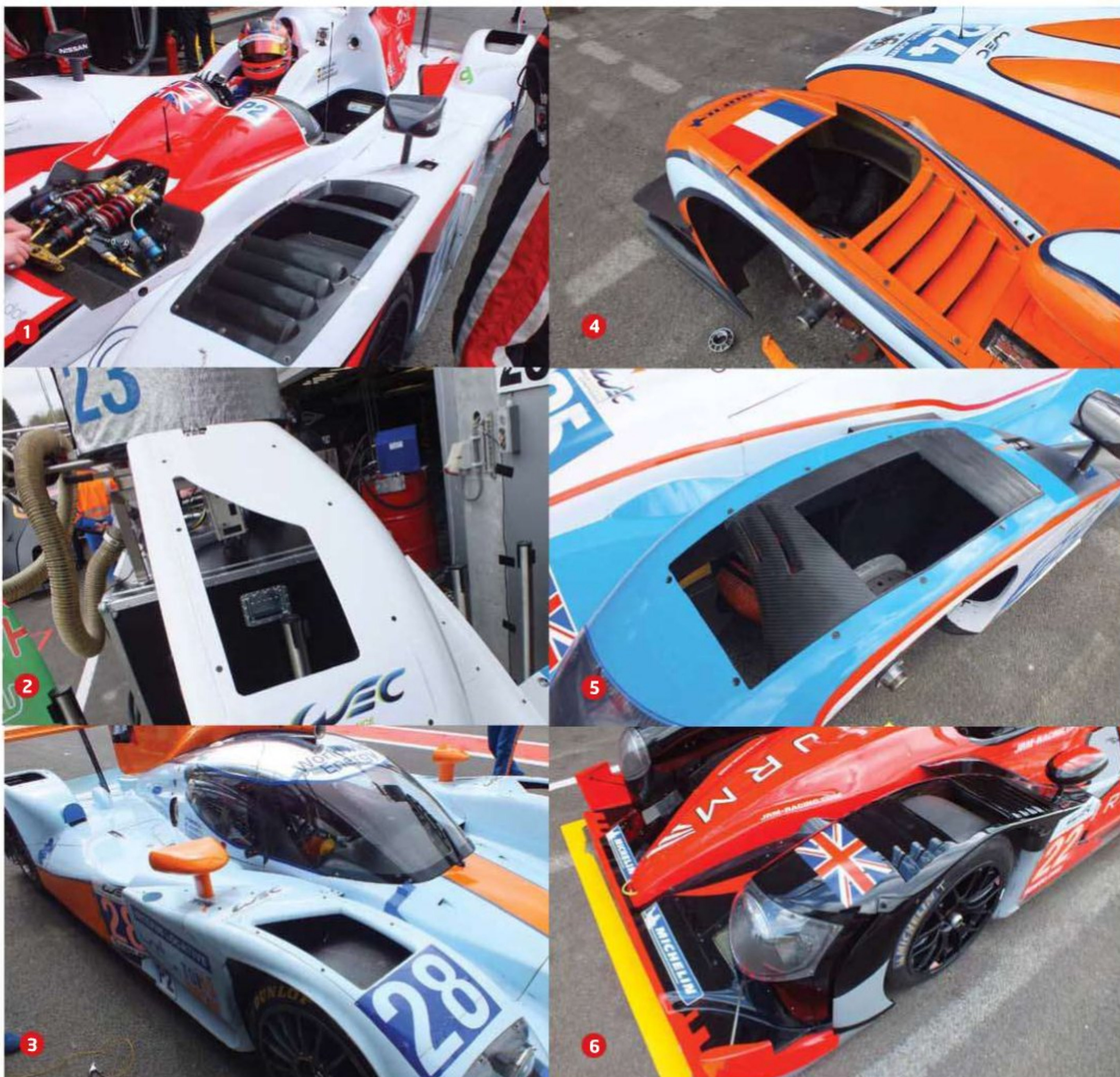
1. Zytek retained some louvres on its air extractors, and added a split exit to smooth the flow 2. Dome ran with an interim solution at Spa similar to the Lola solution 3. The curved tail of the hole is likely to encourage
