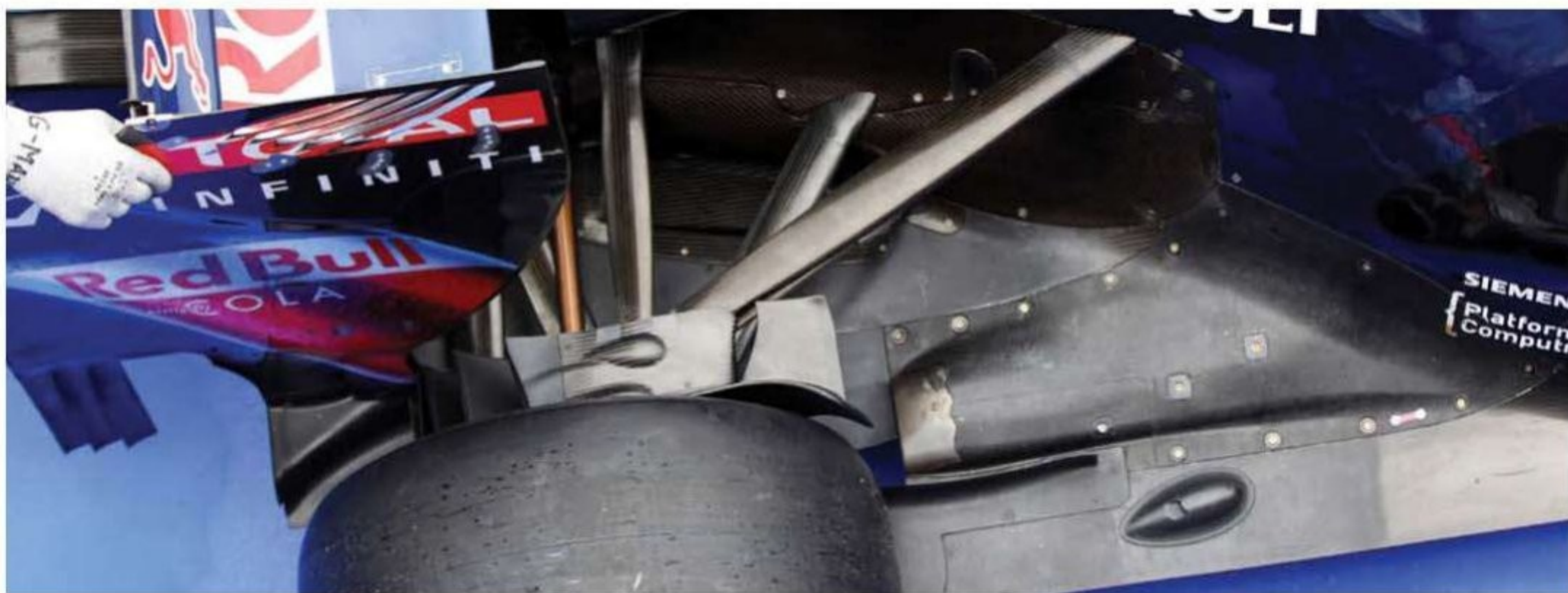
This close-up of the Red Bull exhaust outlet shows how the floor is being blown directly ahead of the rear wheel with the exhaust pointing to the inside edge of the rear tyre to stop the vortex interfering with the flow through the diffuser. Note the cut out just ahead of the wheel where the flow will go down
