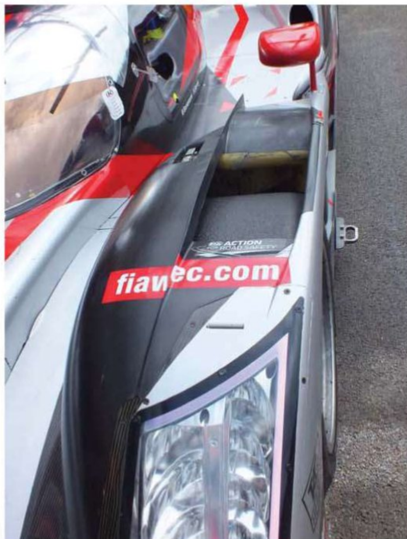
Audi utilises lips both upstream and downstream of the holes to prevent the dirty air from impacting other flow structures across the car
