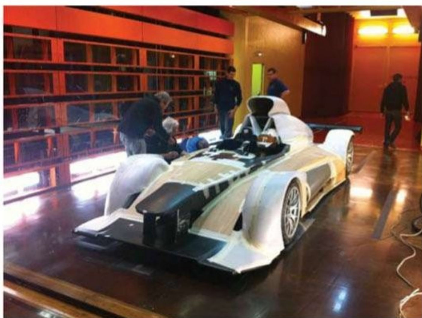
Wind tunnel testing took place at the adaptive wall tunnel at the St-Cyr Aerotechnical Institute in Brittany, France
