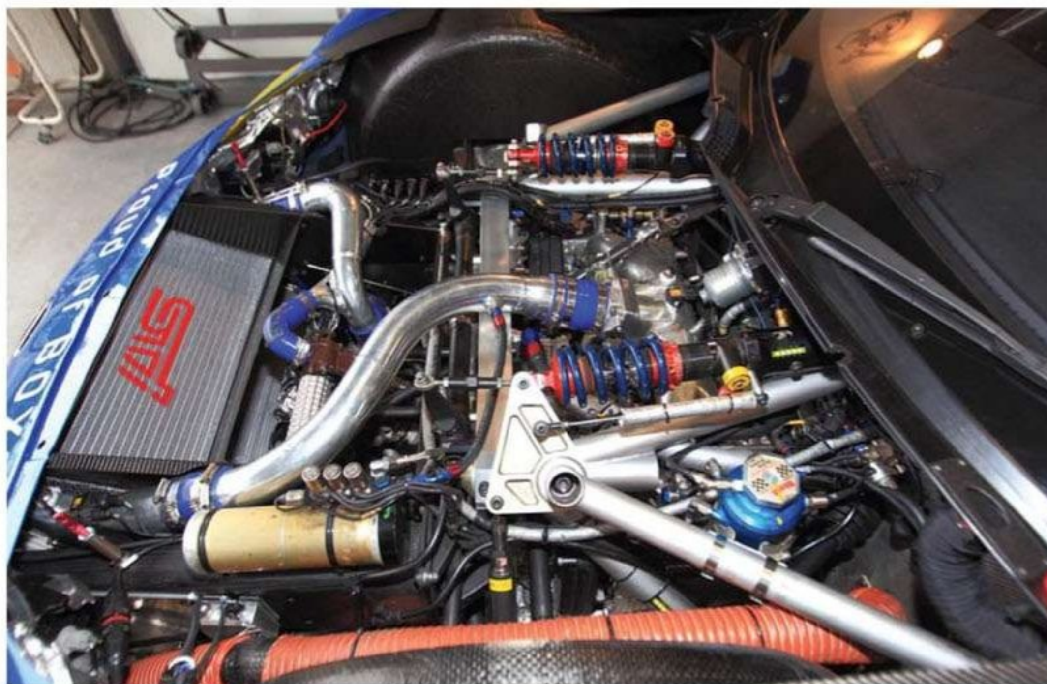
2.0-litre, turbocharged, EJ20 boxer engine is producing upwards of 350bhp. Dampers sit right above the engine
