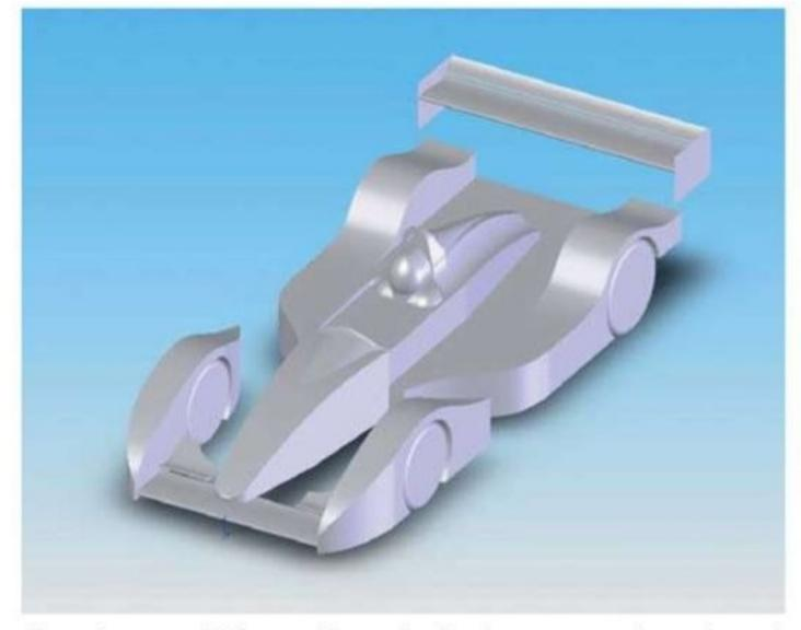
Figure 4: concept #2 featured front wheel pods, a narrower front wing and sidepods enveloping the rear wheels
