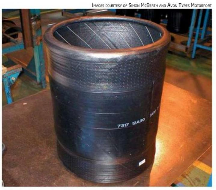
Following the creation of the compound and of the various constituent parts, this is an assembled 'green' crossply tyre awaiting curing
