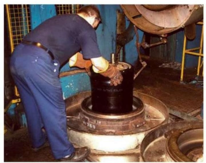
A green crossply tyre being positioned in a two-piece mould at the curing stage
