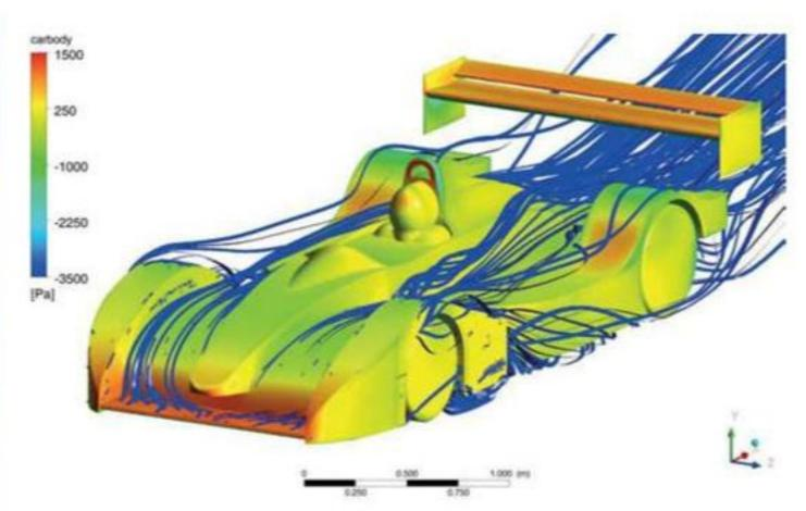
Figure 8: in concept #4 the front upper body integrated with the sidepods, but the splitter and front diffuser were the same as concept #3
