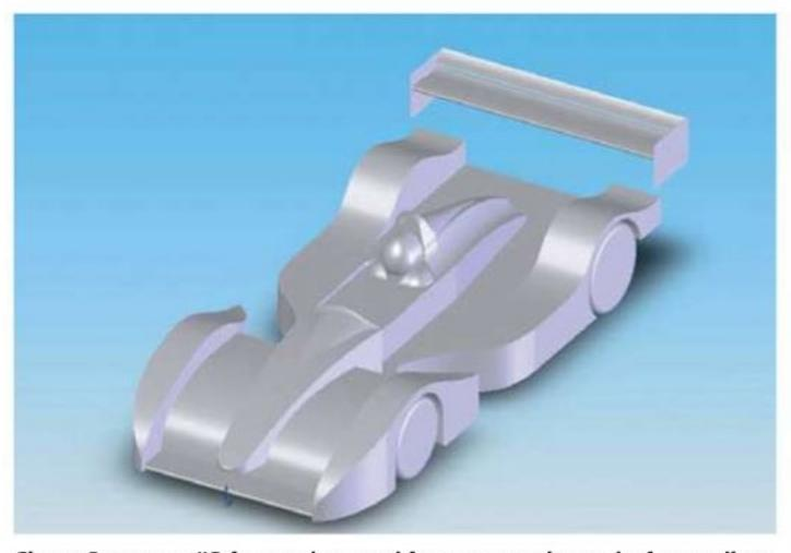
Figure 6: concept #3 featured covered front suspension and a front splitter and diffuser instead of a front wing
