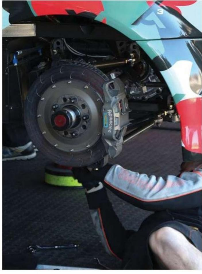
Bigger wheels and tyres will put pressure on the new brake package from AP Racing, but temperatures will be easier to control
