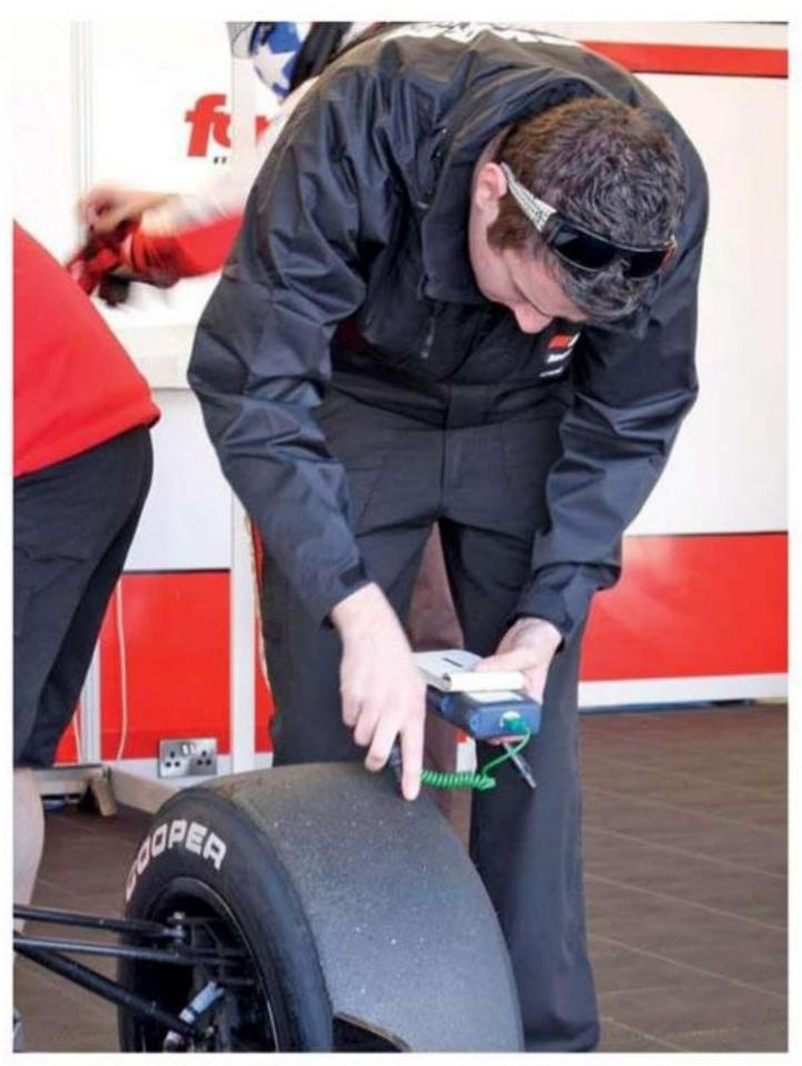
Temperature monitoring. The probe is pushed deep into the rubber 'gauge' for a representative reading
