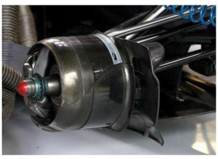
Mark Gillan: 'Brake duct improvement has been significant... We have very good aero data and correlation in this area. Sometimes brake cooling can be a problem, but not for us!'
