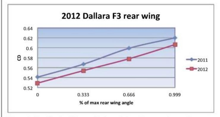
Figure 1: the effect on CD, overall drag, of changing rear wing angle
