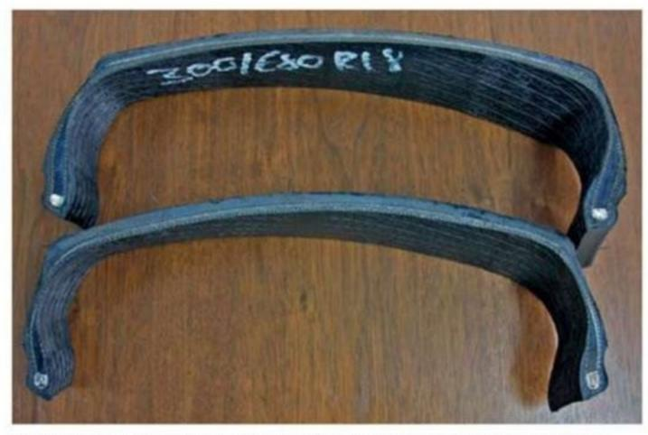
Two GT tyres, a race tyre (top) and a hillclimb tyre (bottom). Note the thicker tread 'gauge' (depth) on the hillclimb tyre
