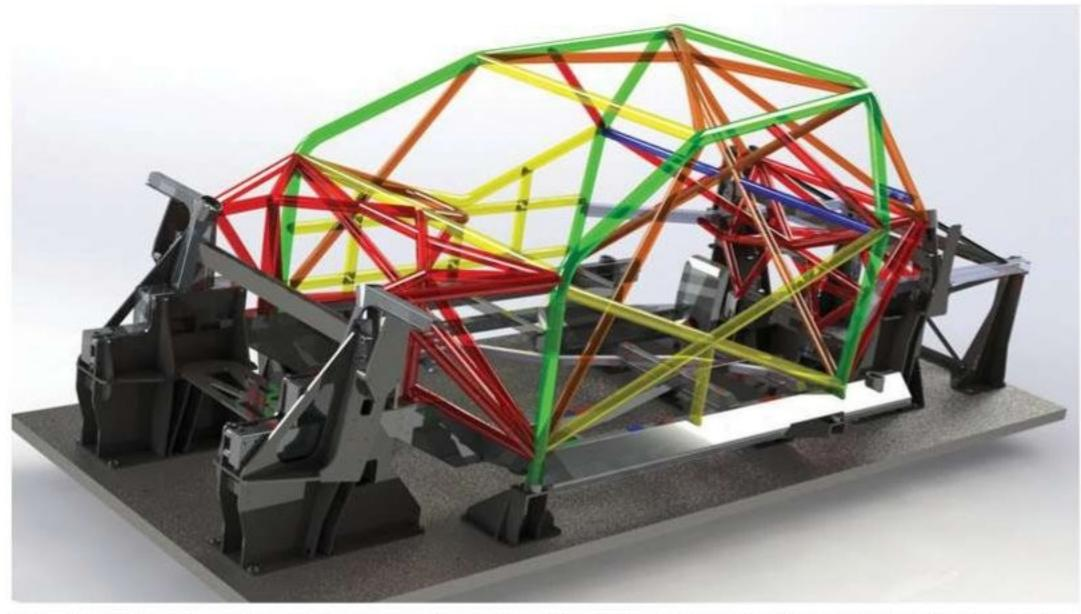
Surprisingly, the new chassis / rollcage assembly is thought to be some 20 per cent less stiff than the current one
