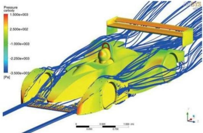
Figure 5: much improved aerodynamics with concept #2
