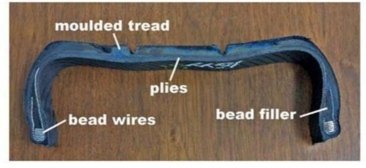
Figure 1: section through a Rallycross crossply tyre
