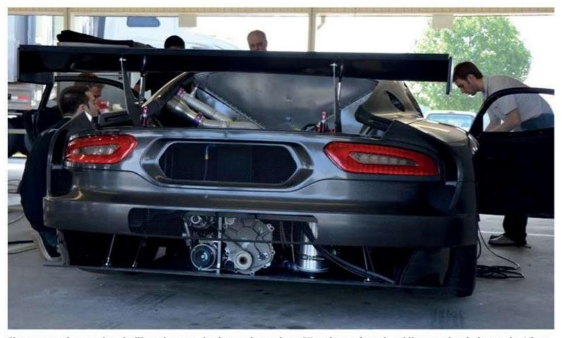
Changes to the gearbox bellhousing are de rigueur in modern GT racing, a fact that Riley used to balance the Viper
