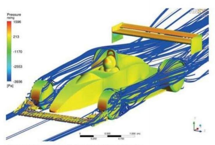
Figure 3: mudguards affected downforce and drag
