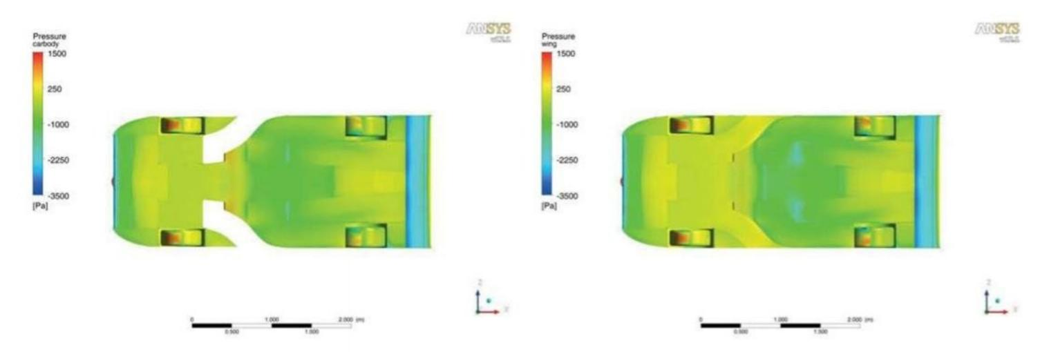
Figure 10 and 11: the static pressure plots on the lower surfaces of concepts #3 and #4 show more low pressure (green / blue) in the front underbody of #4
