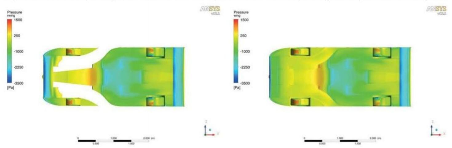
Figure 12: the static pressure plot on concept #2's underside shows more widespread low pressure in the underbody, as well as under the front wing
