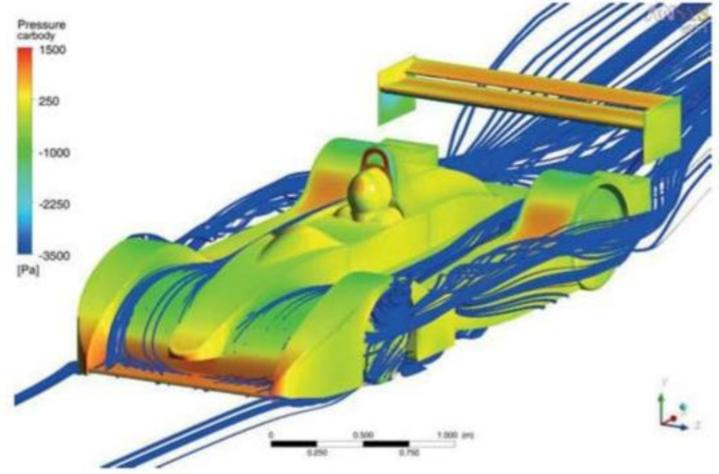
Figure 9: concept #4 saw a downforce improvement, but a shift in balance
