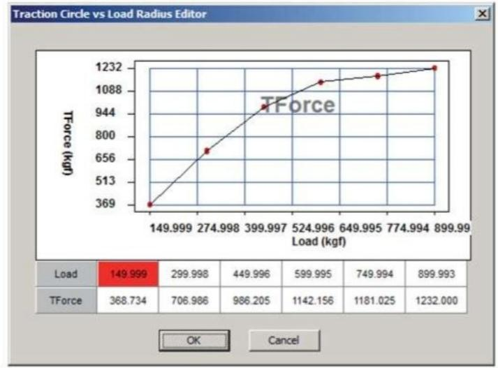
Figure 3: TC radius vs load characteristics
