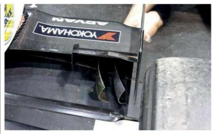
The twin turning vanes under the front wing were also effective
