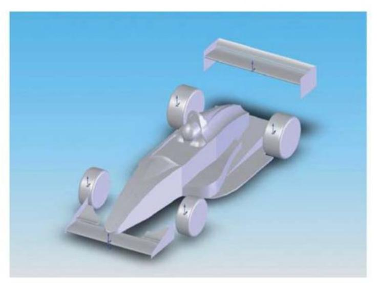
Figure 1: original single-seater Vortex concept in phase 1b guise, with raised nose, sidepods and ground effect underbody
