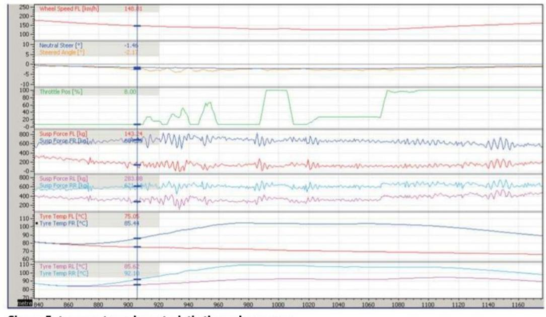
Figure 5: temperature characteristic through a corner
