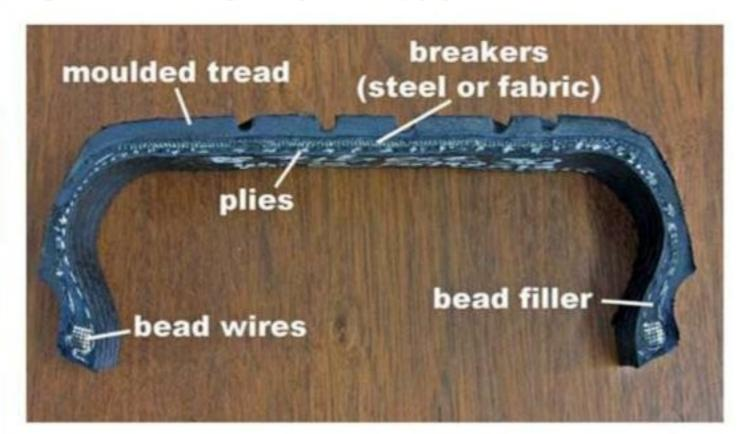
Section through a CR500 radial tyre. Note the addition of the 'breakers' between the plies and the tread, and also the different ply orientation visible on the inside surfaces compared to the crossply Rallycross tyre
