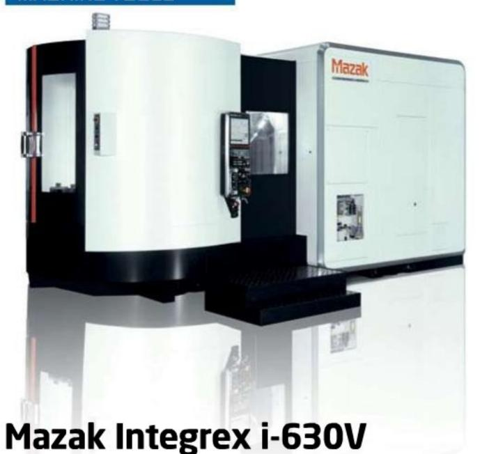
Yamazaki Mazak has extended its range of multi-tasking products with a new, space saving machine specifically designed for the machining of heavy duty applications. The new Integrex i-630V is a vertically configured machine capable of machining large work pieces, with dimensions up to 1050 x 1000mm and up to 1750kg.
