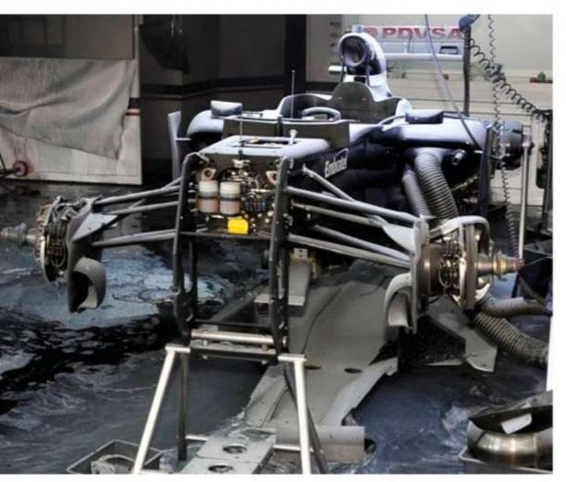
Following the Spanish GP, the Williams garage was destroyed by a freak fire, though this did enable us to see the front suspension and bulkhead
