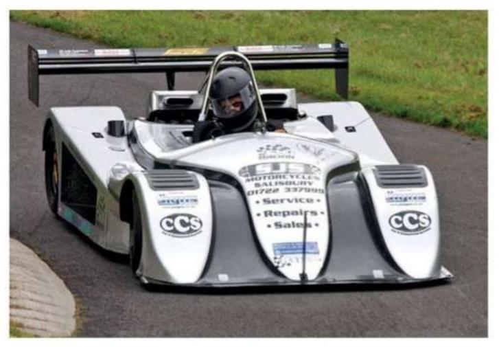
Twin Hayabusa-engined Force SR8 and single-engined SR4 sibling featured a central driving position, but fairly conventional front aero treatment
