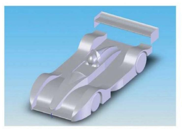
Figure 7: despite bluff appearance, the drag of concept #3 was very similar to concept #2, but downforce was disappointing
