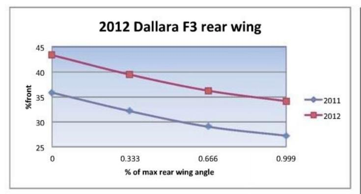
The effect on '%front', or aerodynamic balance, of changing rear wing angle
