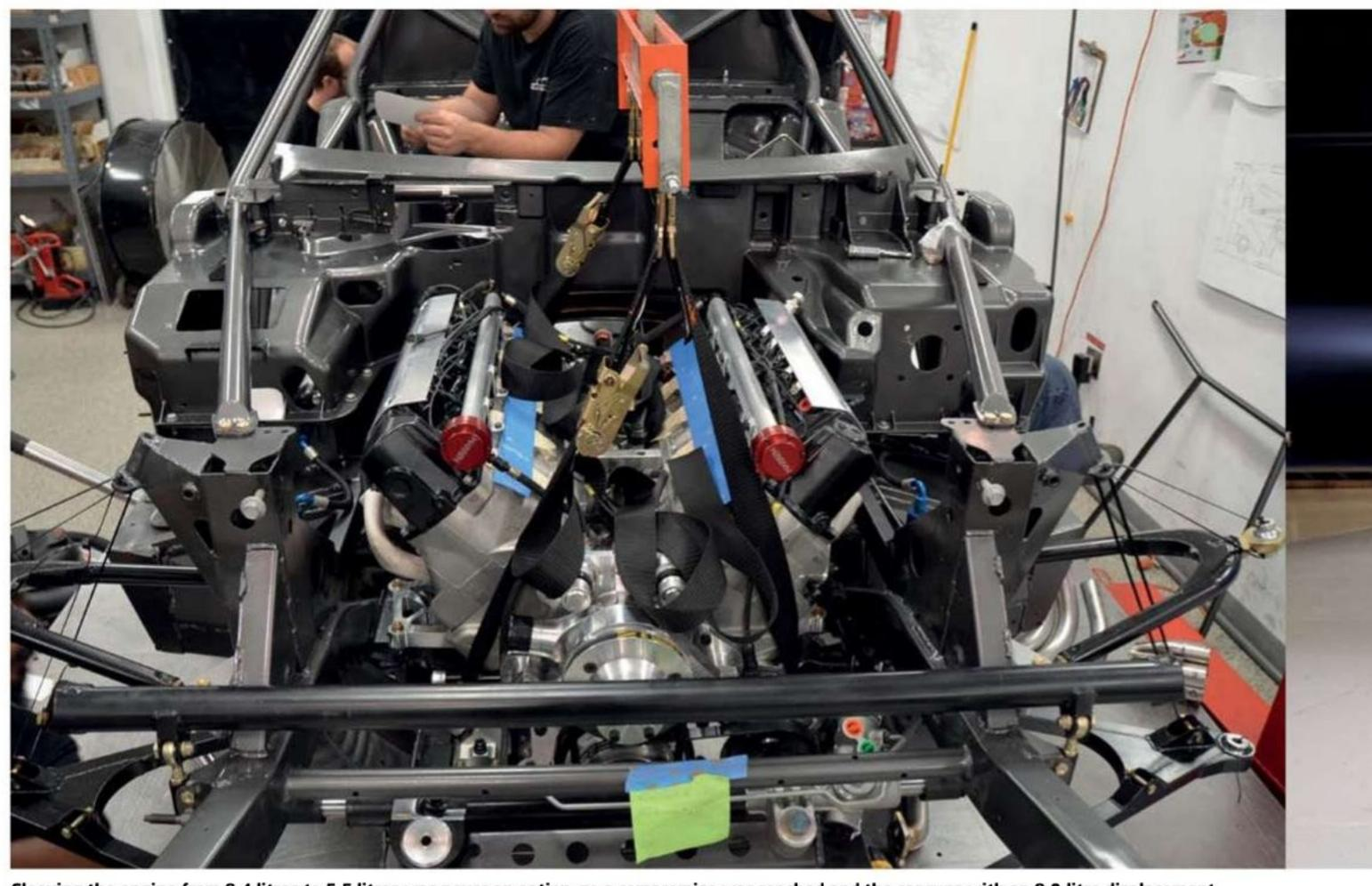
Sleeving the engine from 8.4 litres to 5.5 litres was never an option, so a compromise was reached and the car runs with an 8.0-litre displacement
