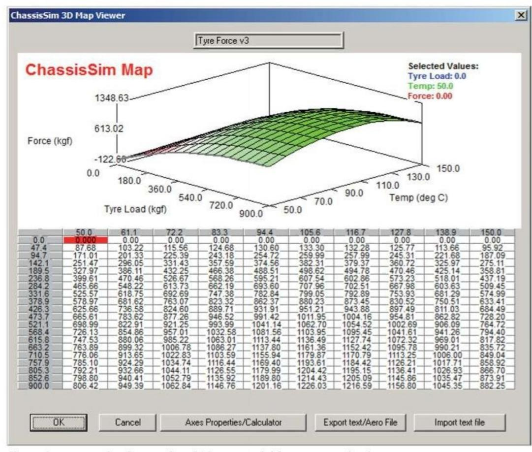
Figure 6: an example of a completed 3D tyre model for an open wheeler
