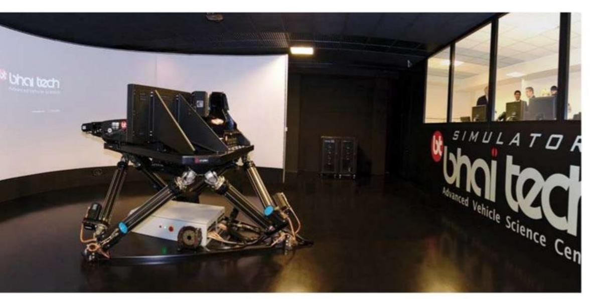
The full-motion race simulator with 210-degree, 8m screen at Bhai Tech Advanced Vehicle Science Centre in Italy
