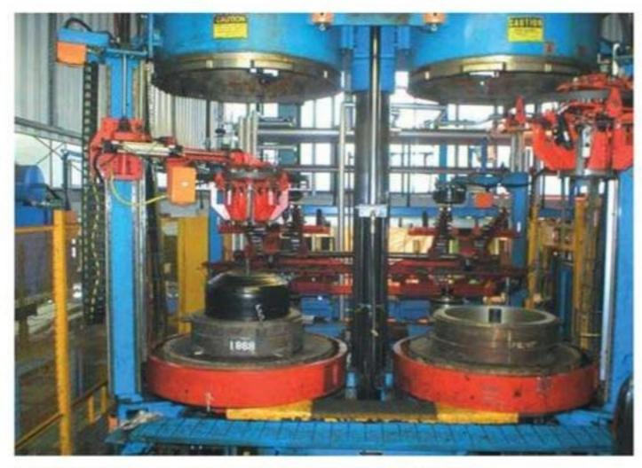
Radial greenstock positioned in a mould at the start of curing
