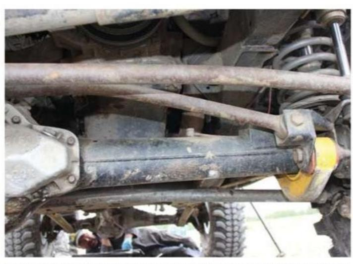
Suspensions are often largely standard in design, but with uprated components and dislocation cones on the springs to allow for increased axle articulation
