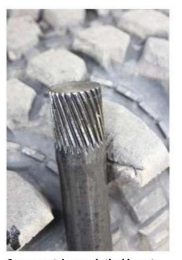
Component damage is the biggest hurdle the racers face. The twisted splines on this driveshaft say it all
