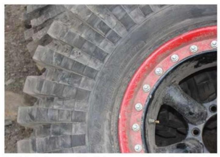
Bead lock wheels are essential, with tyre pressures as low as 10psi used on the rocky sections, which makes for 'interesting' handling on the fast gravel sections
