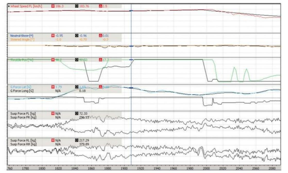
Figure 4: a plot of simulated speeds and tyre loads
