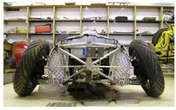
The Camber Car, built by Milliken in 1960 to test his theories on lateral stability
