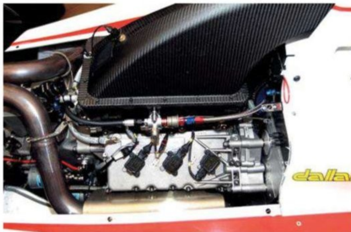
The AER V6 engine had bespoke heads and a major overhaul for GP3
