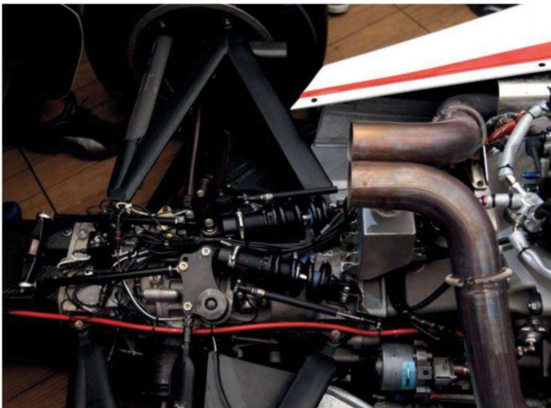
Due a heavier car with higher aero loadings the wishbones of the GP3/13 have been beefed up
