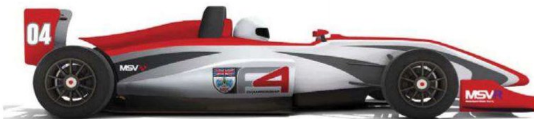
With a 2-litre Duratec engine and 6-speed Sadev transmission, the MSV F4-013 is a 'very controlled car'
