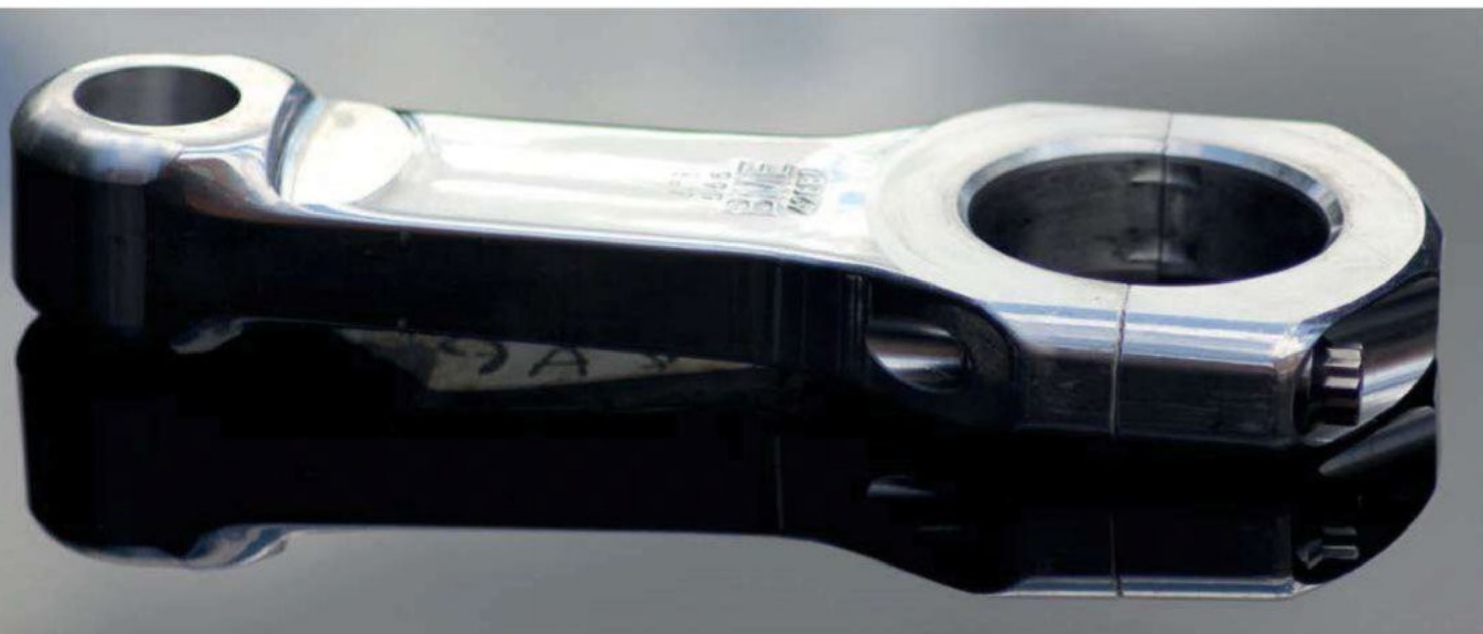
Connecting rods are a huge challenge for materials specialists, in a Formula 1 engine they can stretch and compress 3mm between BDC and TDC
