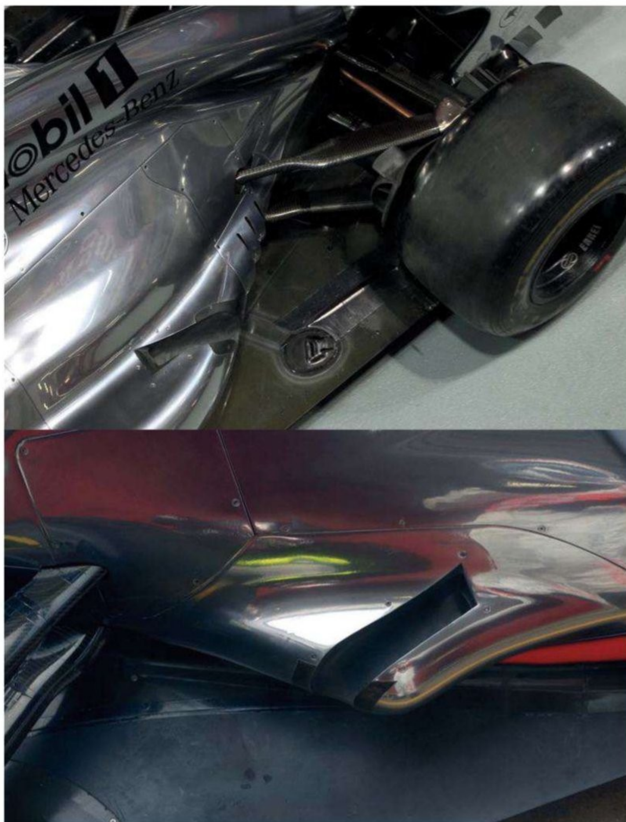
Key to the design and development of the MP4-27 is the 'Coanda' exhaust. It has been copied by most of the teams on the grid, and channels the exhaust plume to give the effect of a 'cold blown' diffuser
