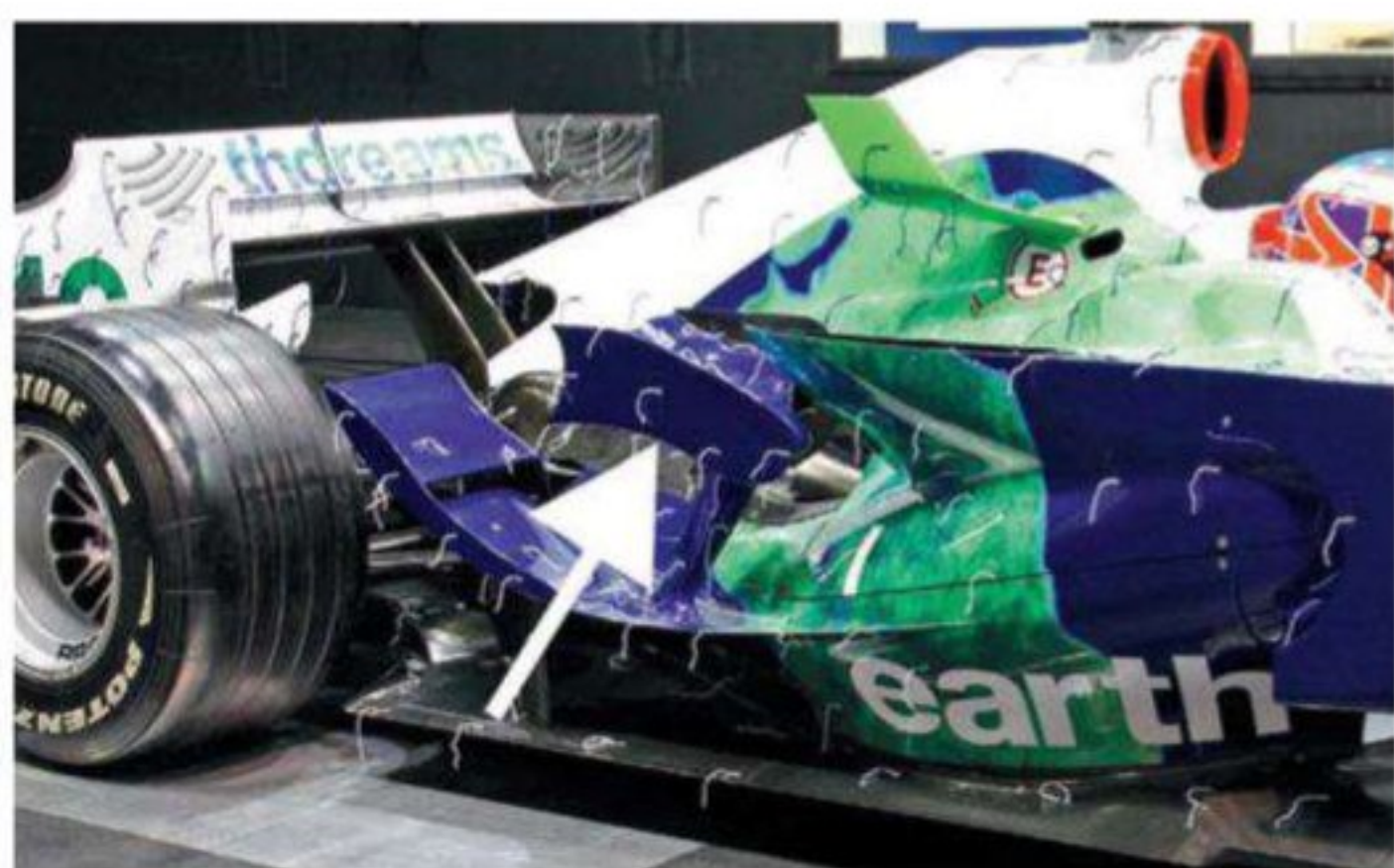
'Aero stalks' comprised a small single element wing section on a short pole
