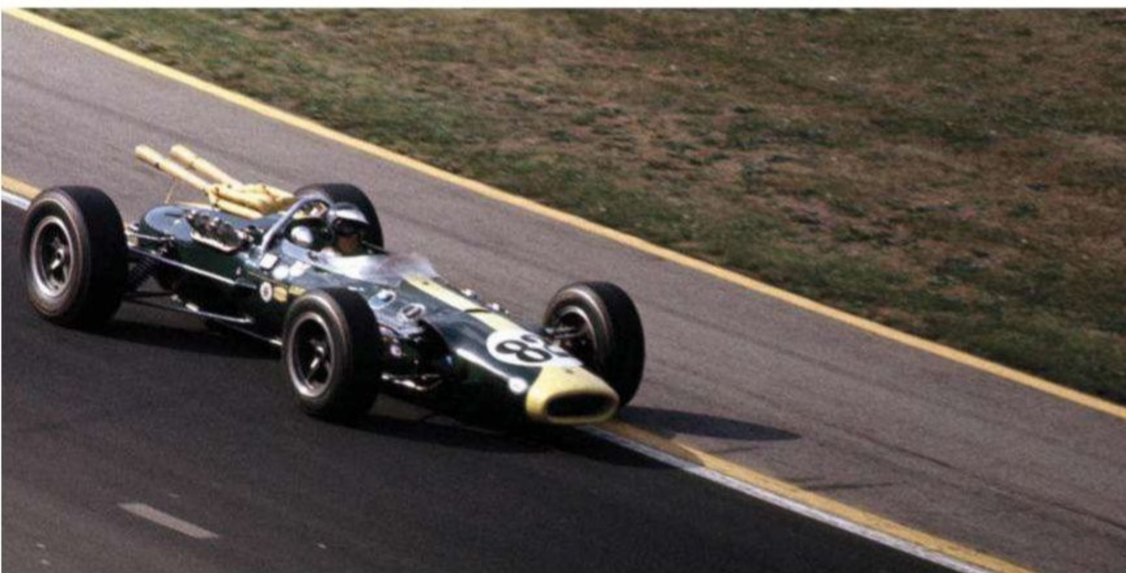
The 1965 Indianapolis 500 saw the Ford engine upgraded to run on methanol fuel for the first time, which produced more power and cooler engine temperatures, helping Jim Clark to win the event for Lotus having led 190 of the 200 laps
