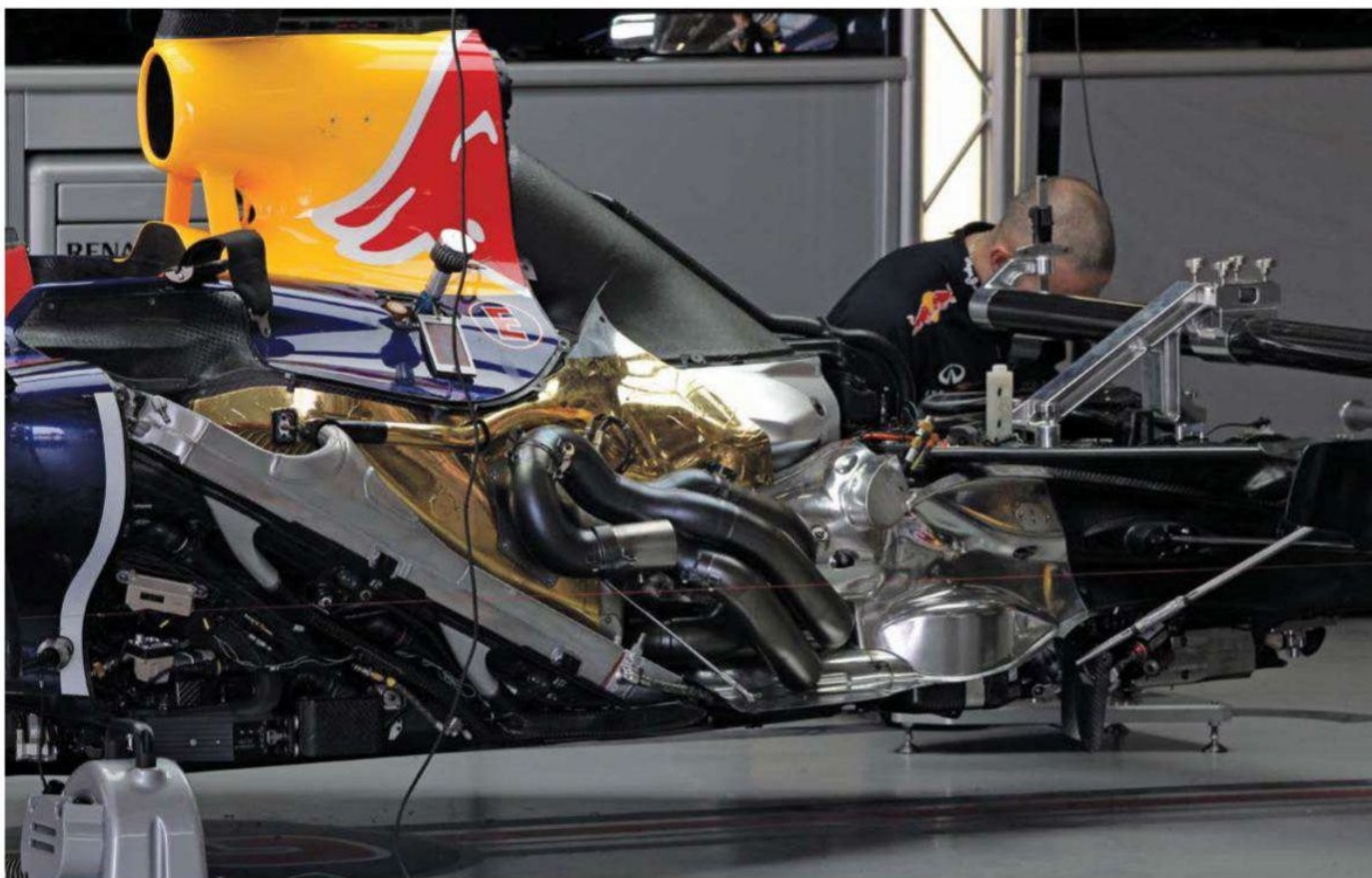
Exhaust layout was a strength of the Red Bulls until the regulation change for the 2012 season, which hurt the team more than most
