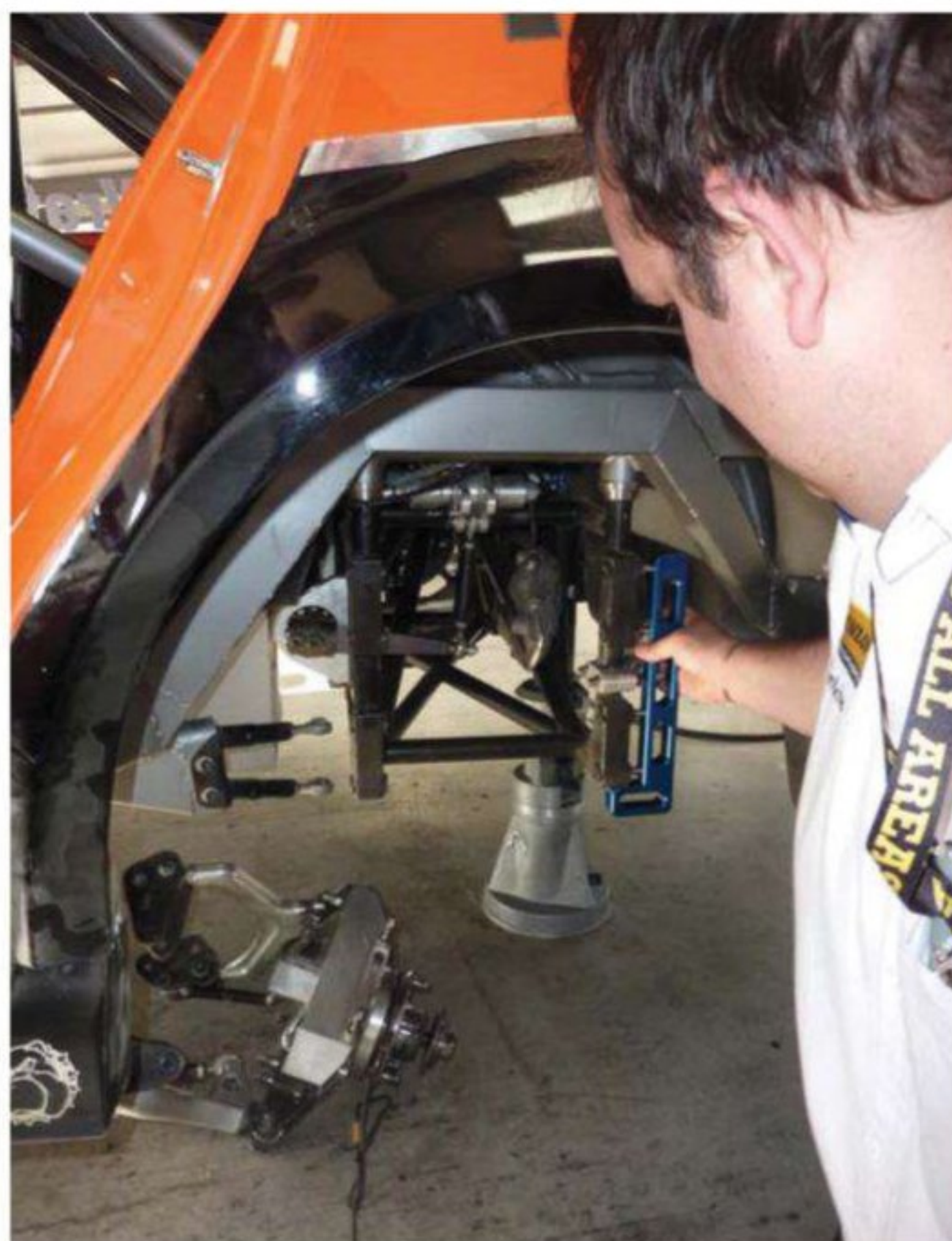
Inspections post qualifying and post race use specially made jigs that slot straight into a correctly manufactured suspension or chassis.
