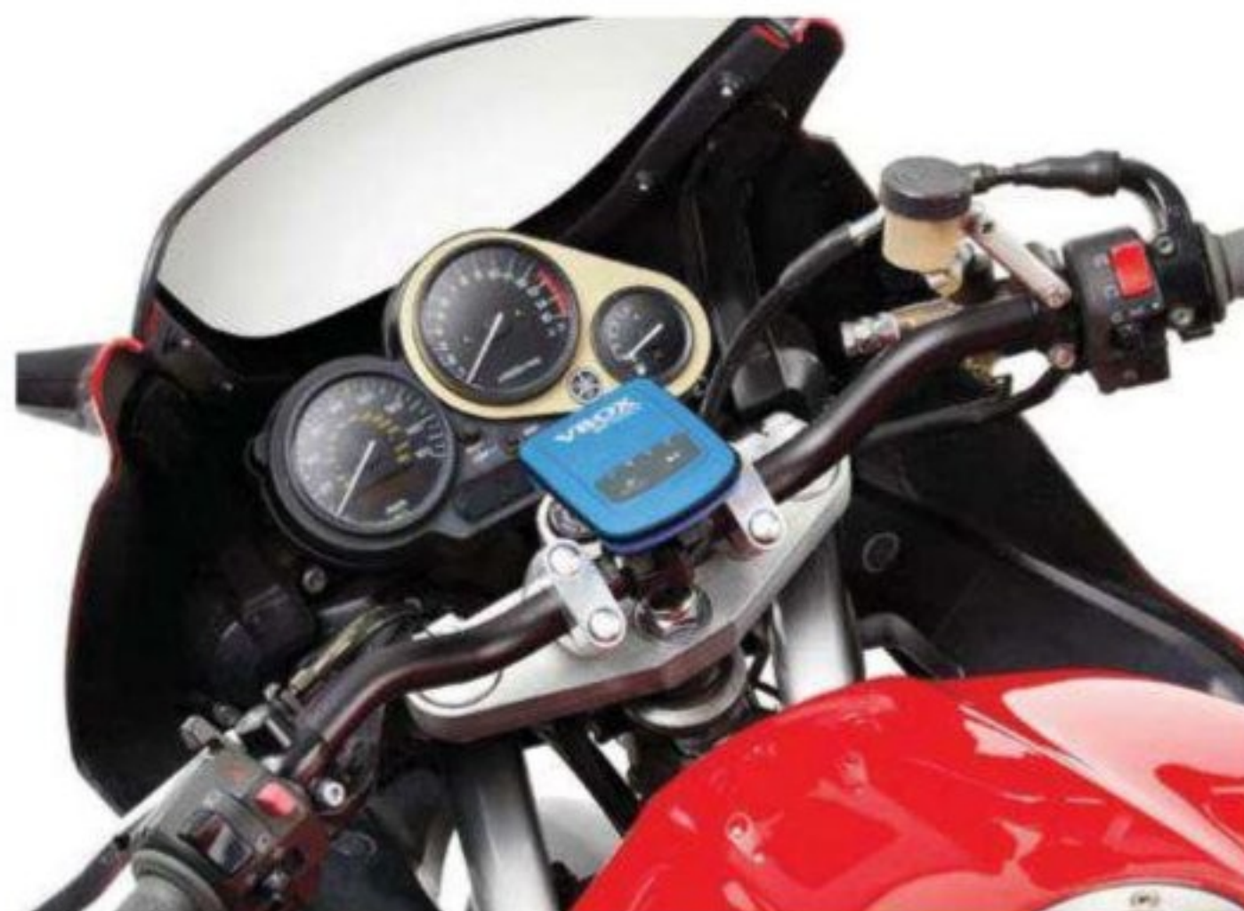
Racelogic's Video VBOX is small enough to be handlebar mounted
