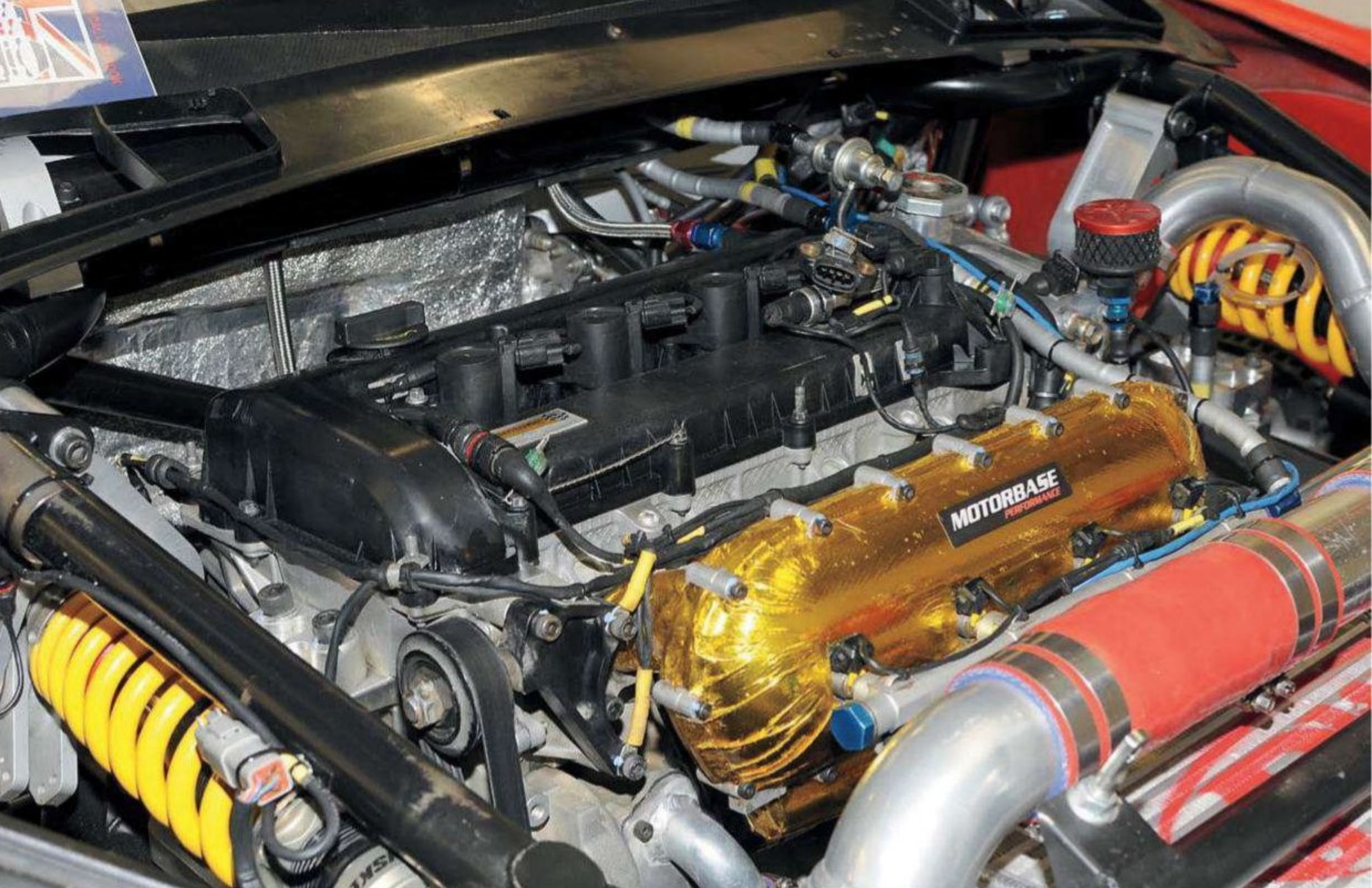
The Mountune engine is a direct carry over from the S2000 regulations, and was a natural fit for the new car given the experience of the British company
