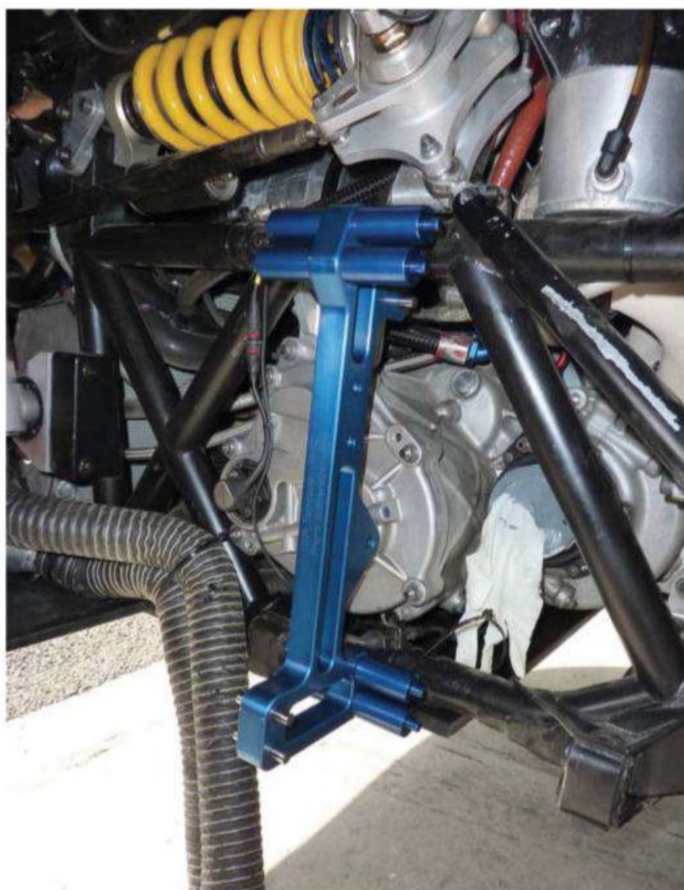
Inspections post qualifying and post race use specially made jigs that slot straight into a correctly manufactured suspension or chassis.
