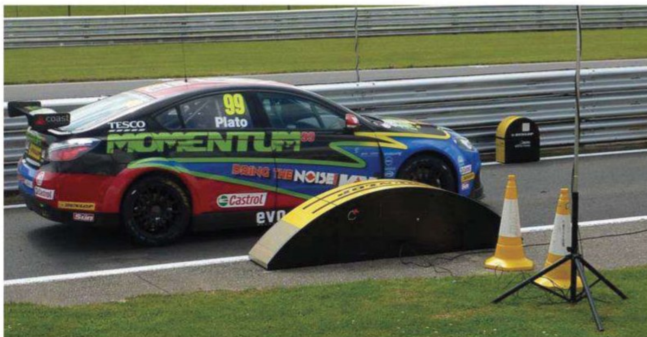
Electronic tagging on Dunlop's tyres means that the checks can be made electronically for each car
