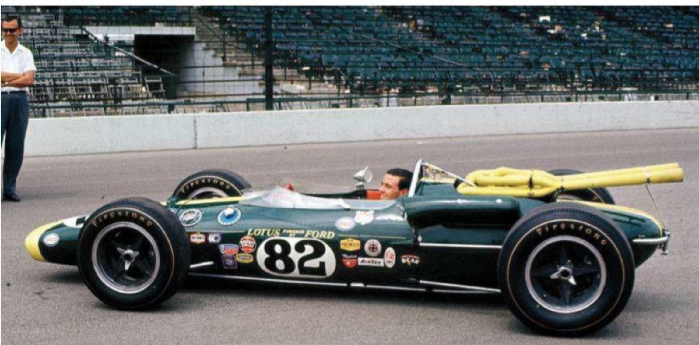
The 1965 Indianapolis 500 saw the Ford engine upgraded to run on methanol fuel for the first time, which produced more power and cooler engine temperatures, helping Jim Clark to win the event for Lotus having led 190 of the 200 laps
