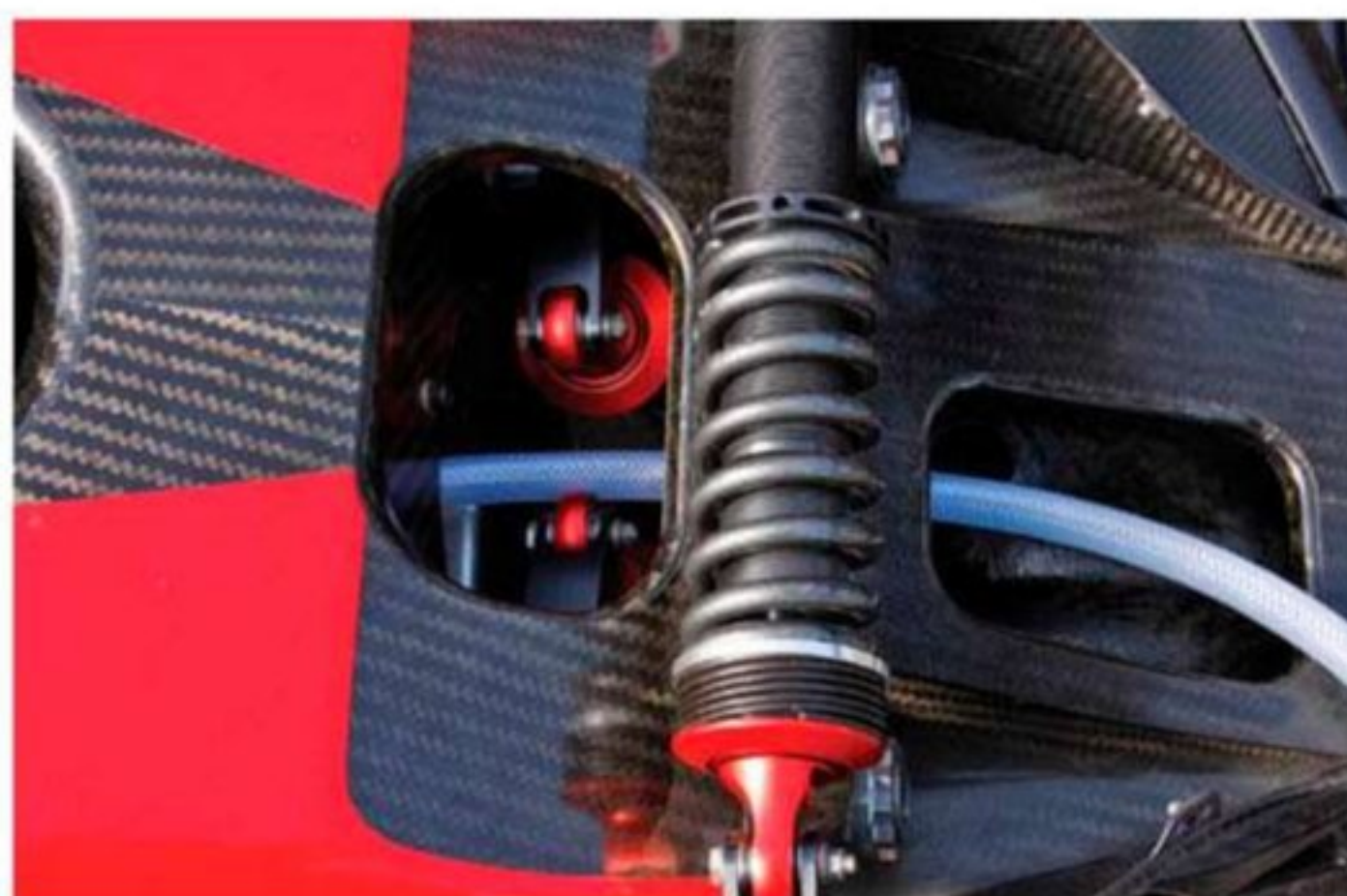
... while the twin roll springs can be seen tucked inside the rear chassis
