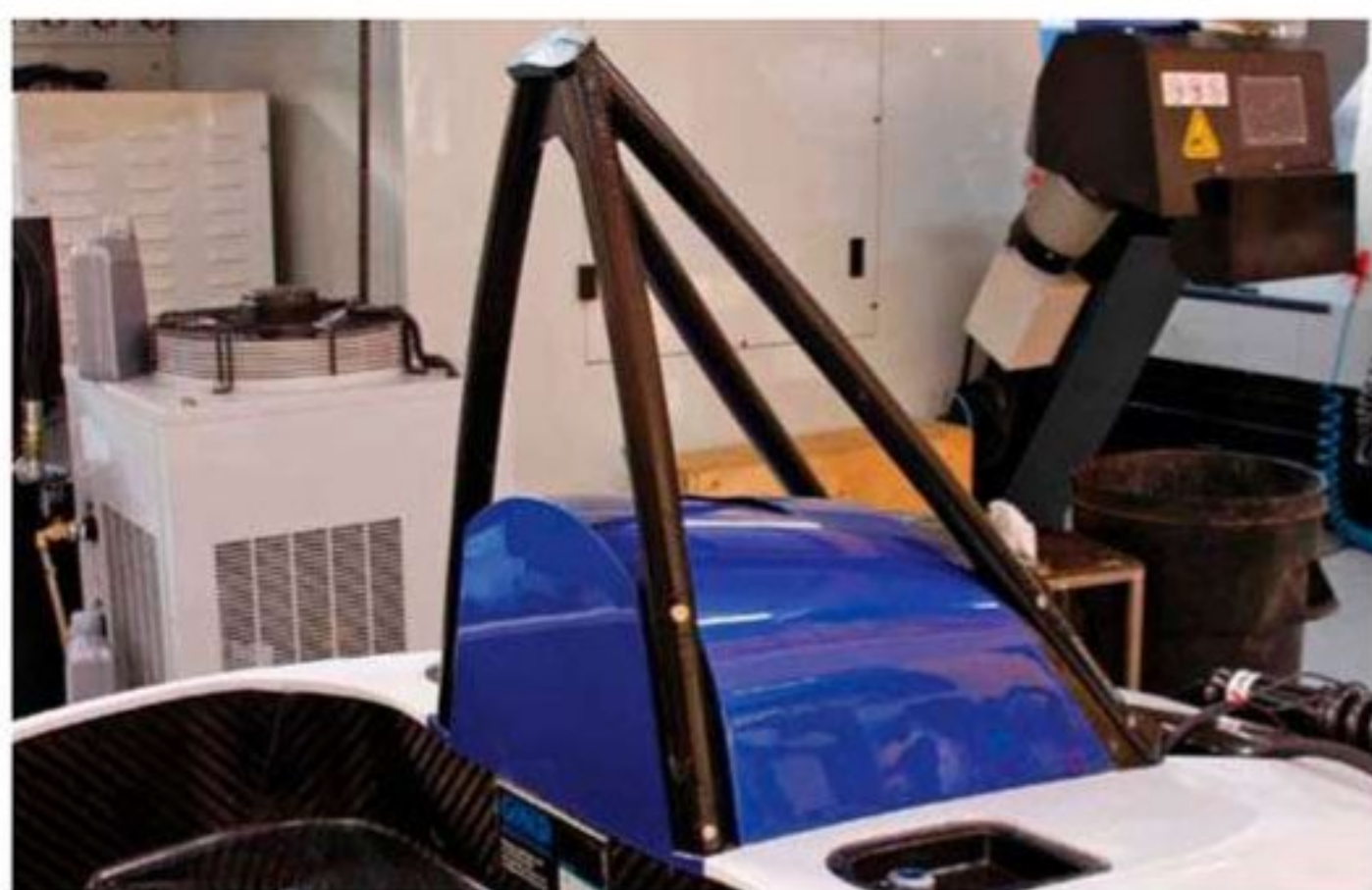
The roll hoop unofficially passed the F1-specification static load test
