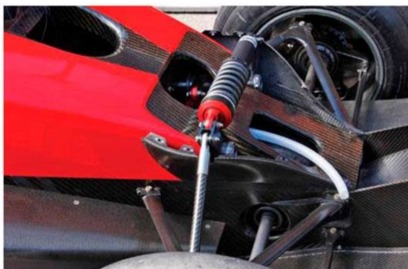
The triple spring/damper rear suspension sees the heave spring transversely mounted over the top of the rear chassis...
