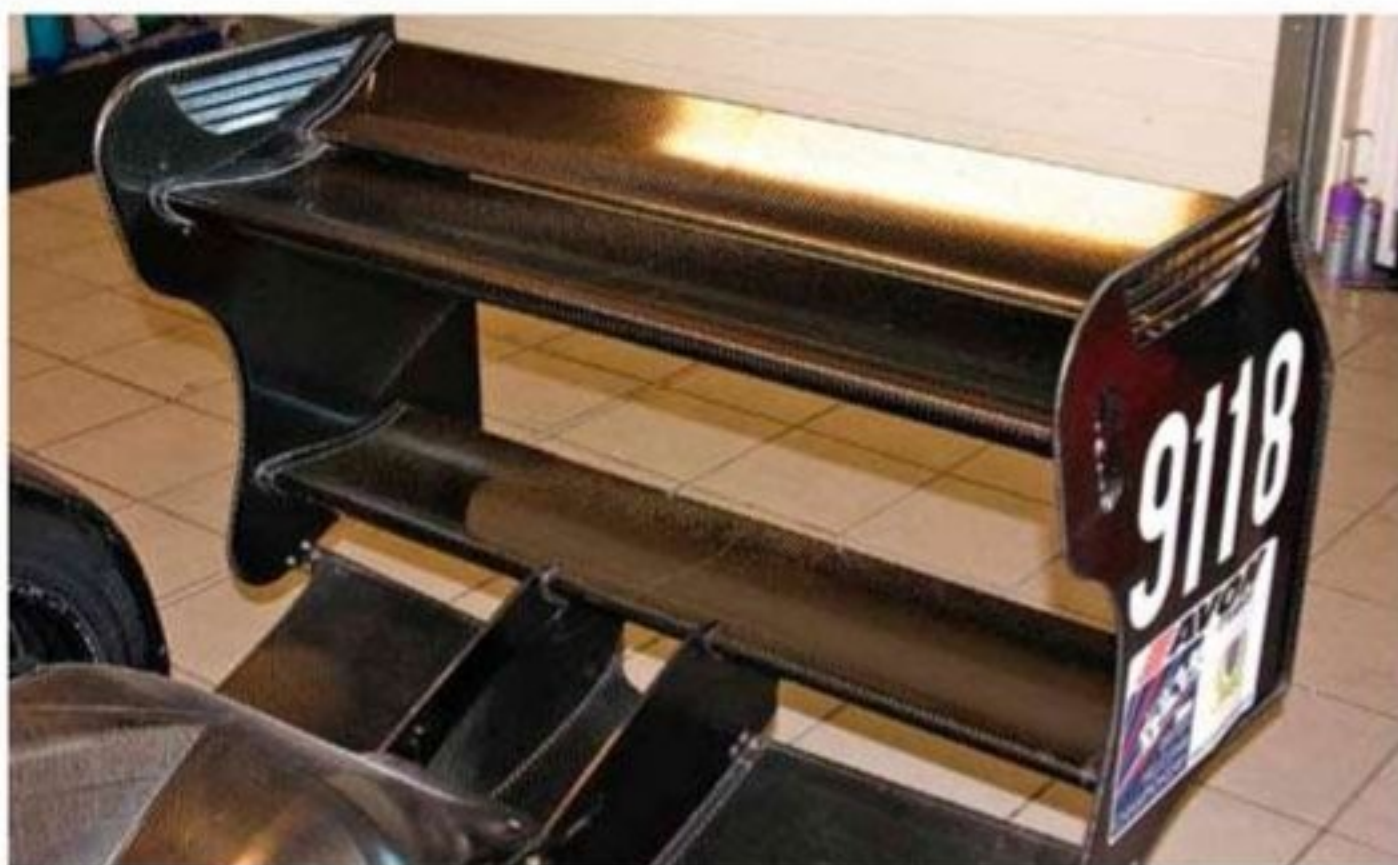
The rear wing features the same section profiles as the GR55 but at reduced span and with a single element lower tier
