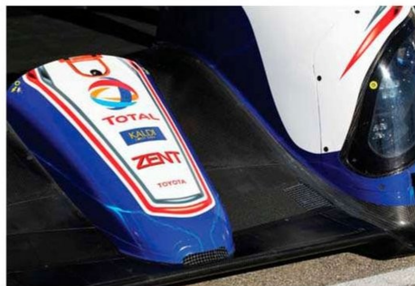
The new nose is lower than last year's model, meaning that Toyota will have to conduct new crash testing on the tub ahead of the first race in May
