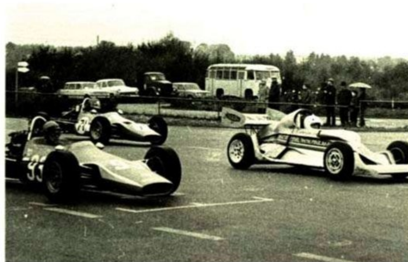
The 0113 was fitted with a 1.3-litre engine. Its wheels were from an aircraft
