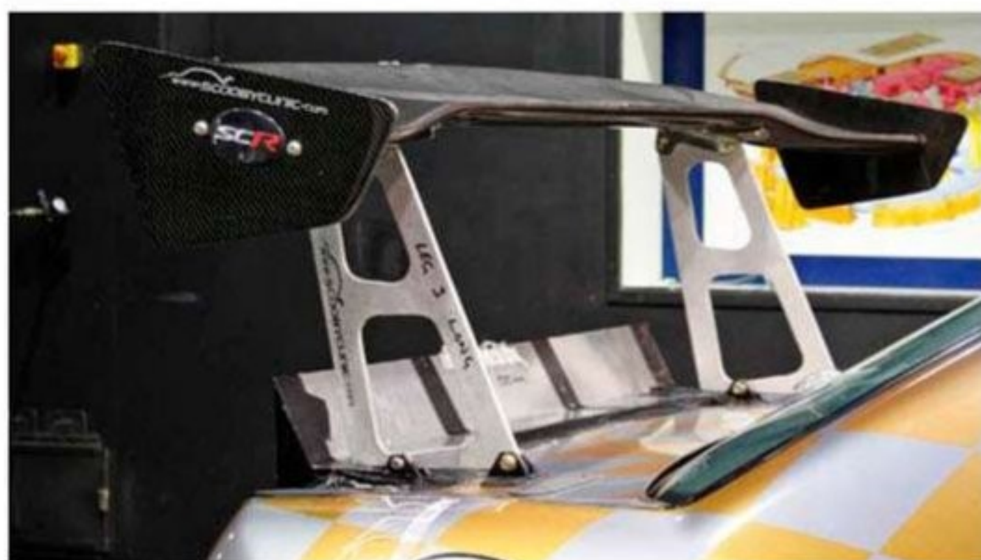
Wing plus 60-degree, 100mm spoiler
