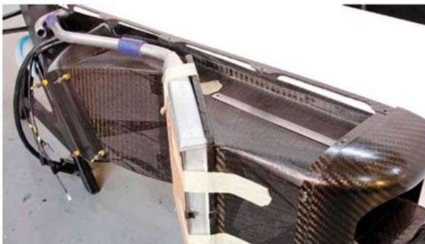
Close attention to internal aerodynamic detail reveals a split plenum featuring twin diffusers feeding the water radiator (centre) and intercooler (left) from a single inlet aperture
