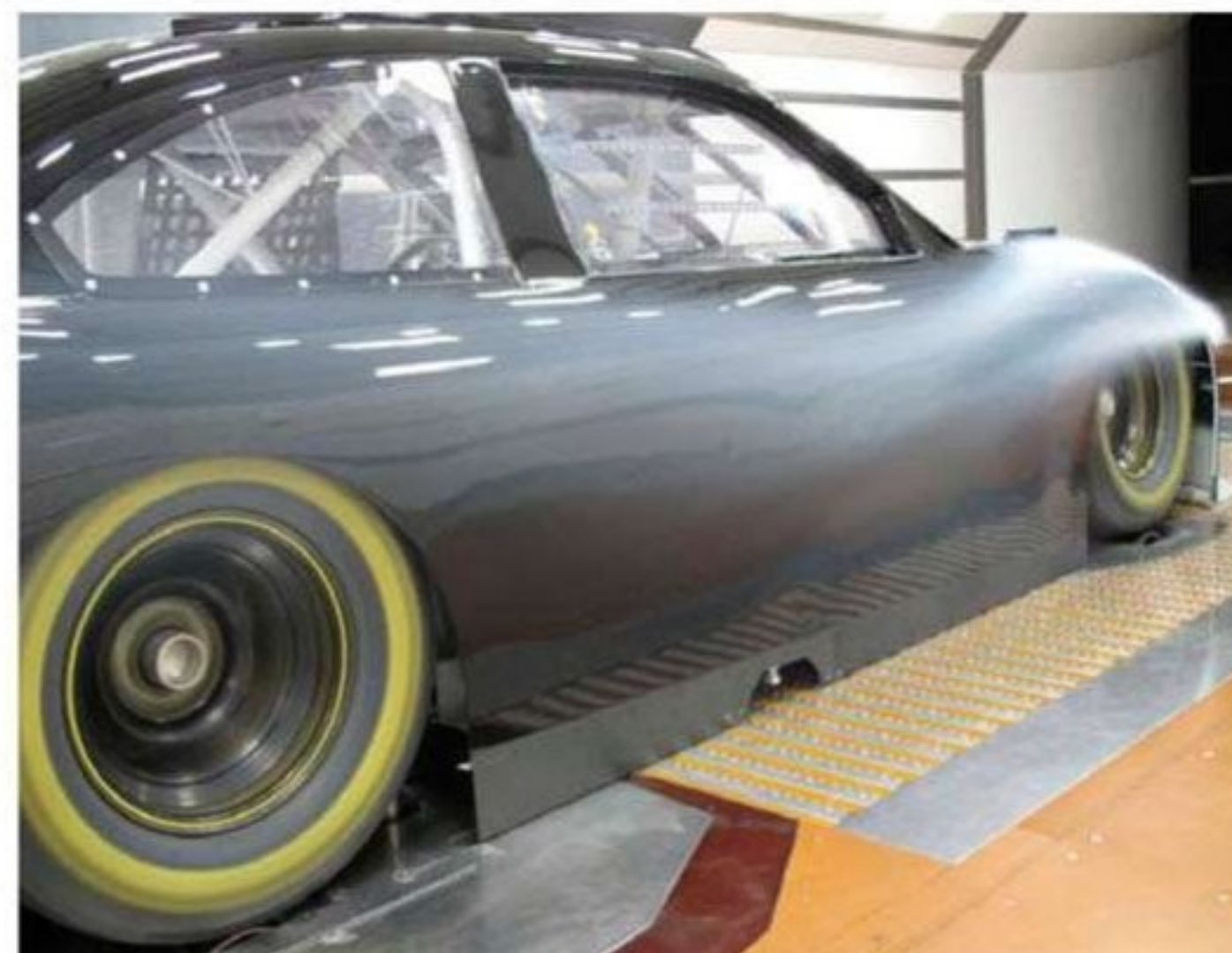
A last generation car on the move in the main AeroDyn tunnel
