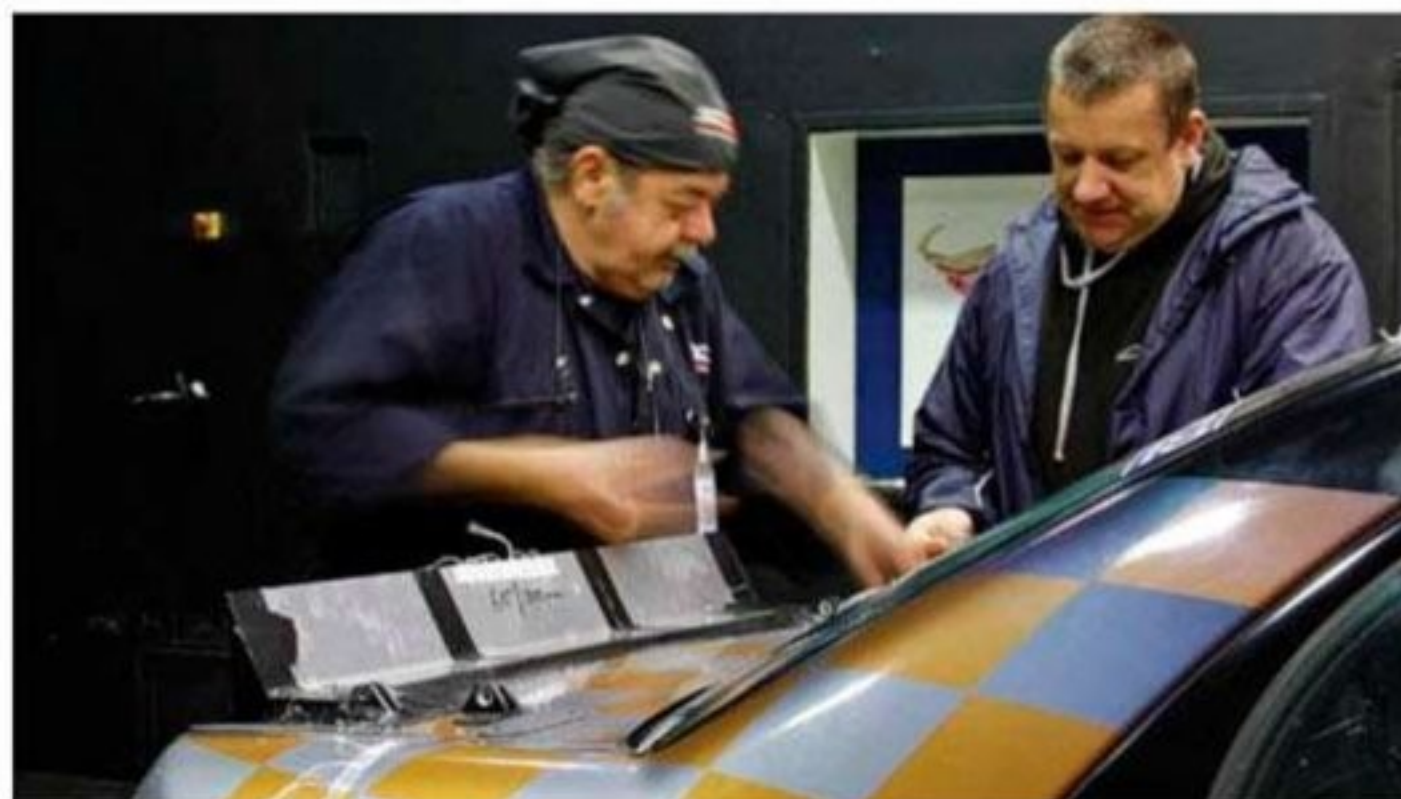
Prepping for a wingless run, with 60-degree, 100mm spoiler
