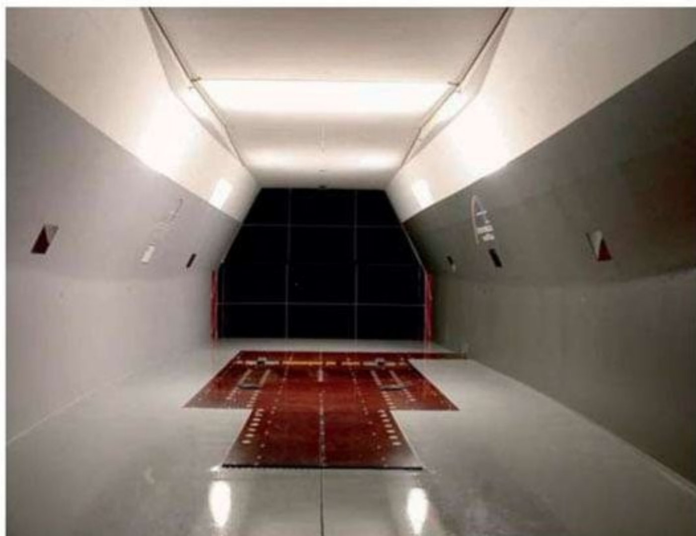
Wheels are not rotated in A2, the smaller alternative to the main tunnel
