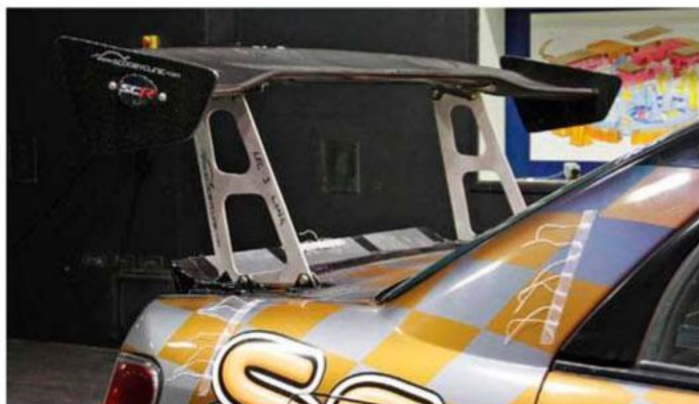
Wing in high location at 10 degrees plus 30-degree, 60mm spoiler
