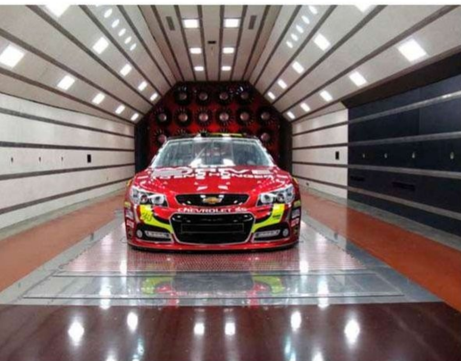
The test section floor was redesigned in 2008 to increase the performance of the floor boundary layer control
