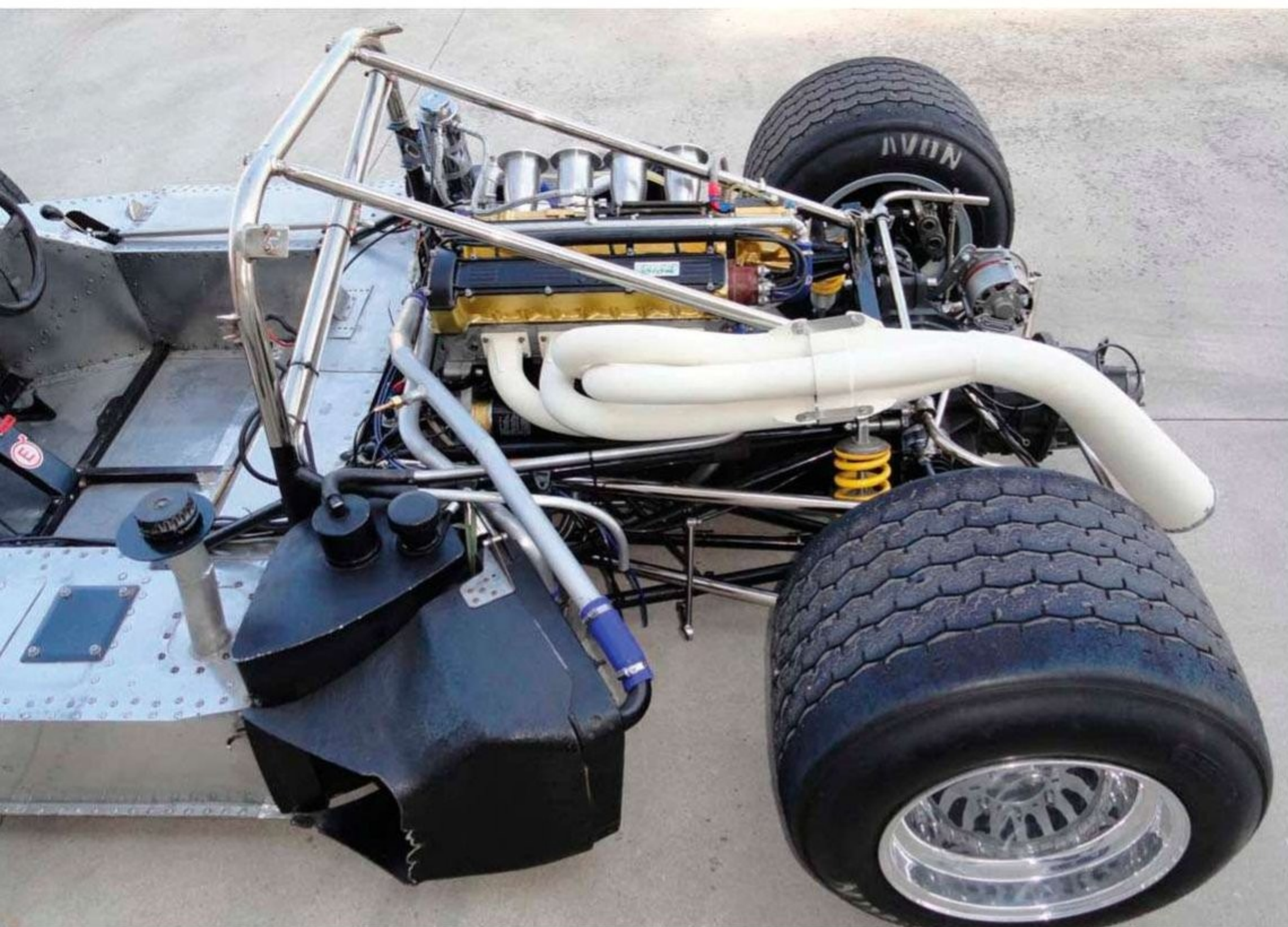
An example of a ceramic thermal coating on an exhaust system
