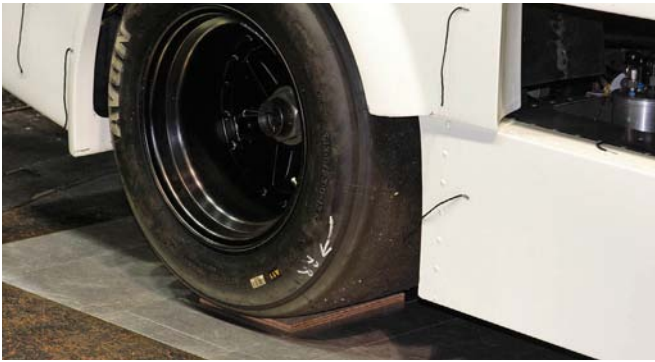
Rear ride height was raised with 'tyre shims'
