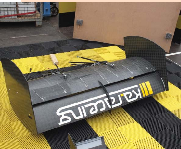
Karlsruhe's car was also bewinged. Note the wool tufts on the underside
