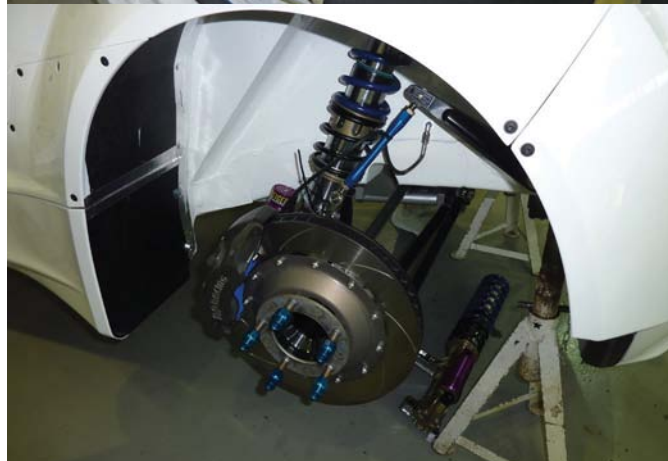
After the FIA rejected M-Sport's original WRC-style rollcage, a new design was created; the R5 features MacPherson struts with Reiger dampers
