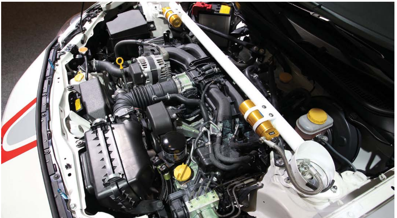
An example of a cross-brace, added to aid stiffness and stability. As a general rule, the stiffer the chassis, the more reliable the handling
