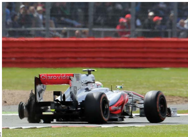
Sergio Perez's catastrophic tyre failure at the British GP in June
