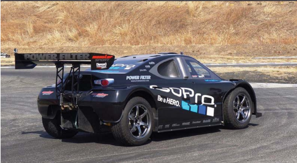
The 'Super 86' from Nobuhiro Tajima's Monster Sport company features a bespoke 3-litre twin turbo V6
