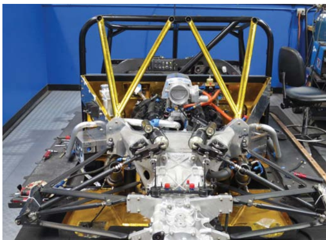
Rhys Millen's 2013 car was 2WD with a mid-engine configuration
