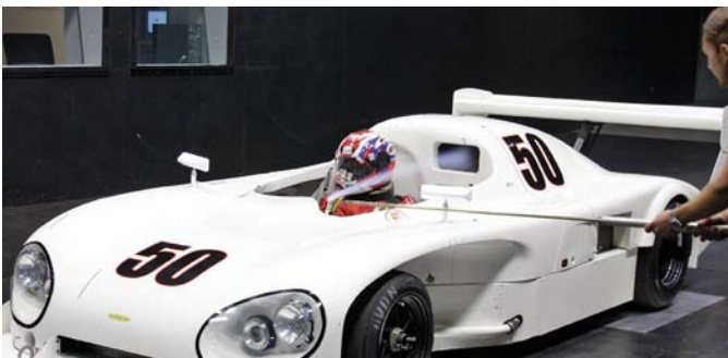
Air flowed into the rear compartment through the aperture next to the driver
