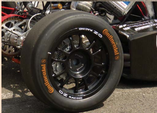
10-inch wheels offer a substantial weight saving, but there are disadvantages
