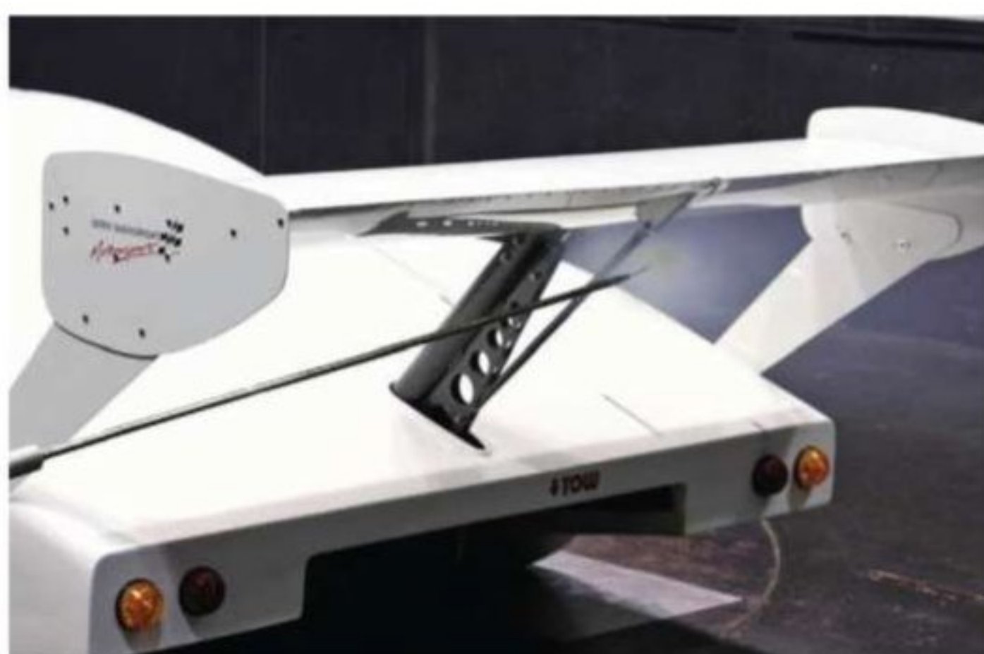
The smoke plume highlighted a stalled area behind the wing mounting post
