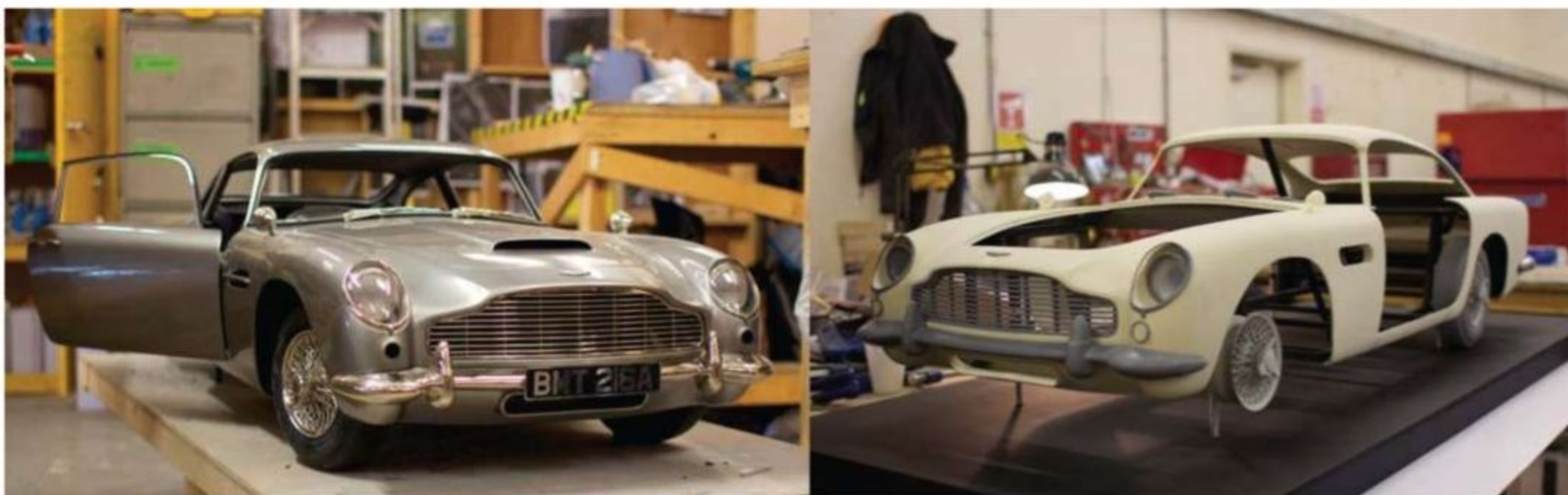
James Bond's iconic Aston Martin DB5 at 1/3 scale was constructed from 18 3D printed parts manufactured by Voxeljet
