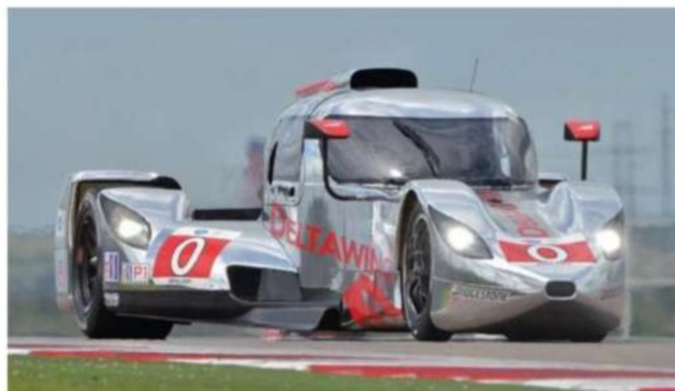
Development of the new DeltaWing's underbody continues, with the team acknowledging there are still aero improvements to be made
