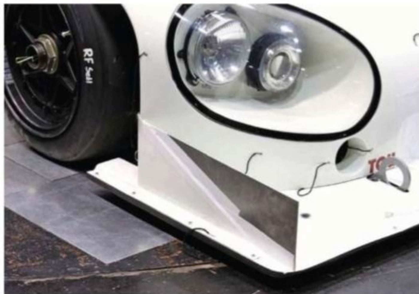
This configuration of splitter end fence produced the best front downforce
