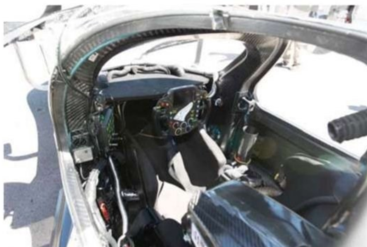
Seat and controls are affixed in the centre of the DWC13 - which is a marked change from the prototypes it will race against
