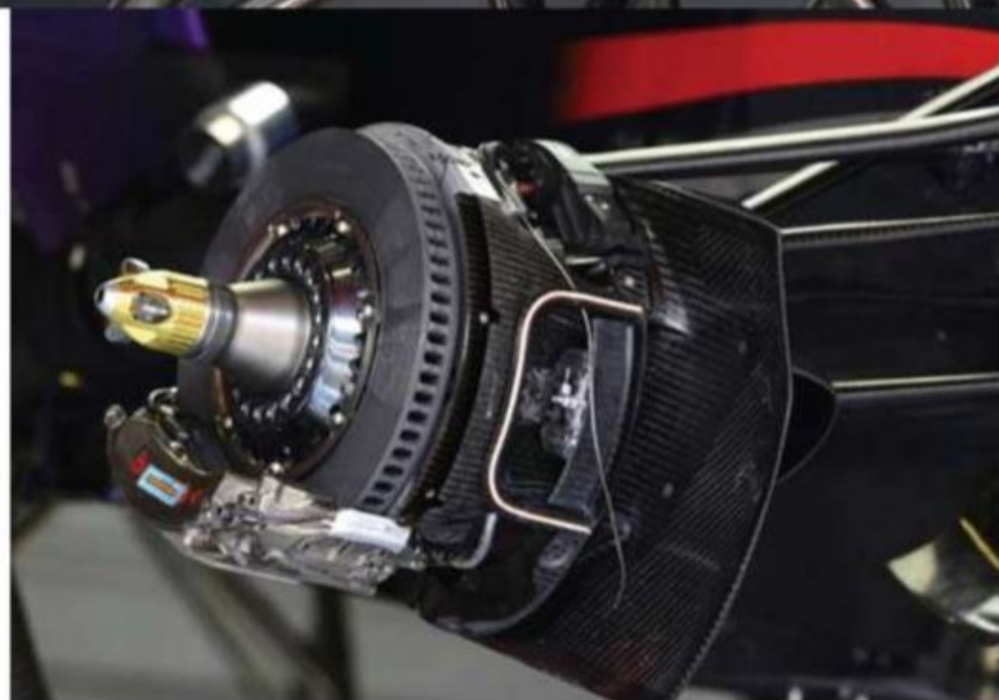
The front brake ducts on the 2013 Red Bull. The car's braking system features Brembo calipers and carbon discs and pads
