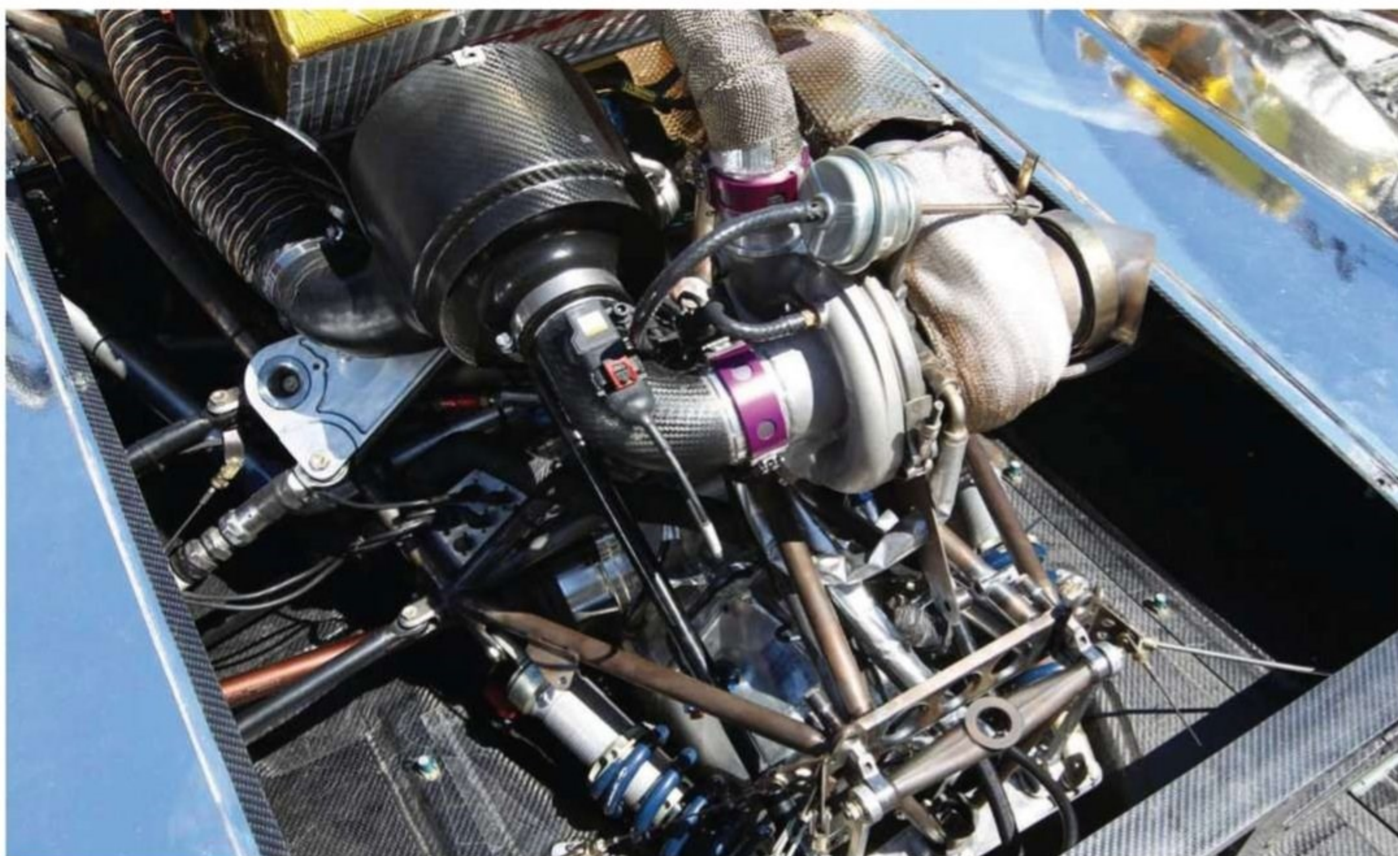
The Coupe has a Mazda-based engine from Élan Power Products, a change from the original's Nissan 1.6-litre
