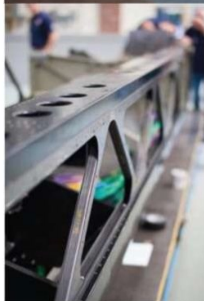
Top: the lower structural chassis of the Bloodhound has been built using steel and aluminium Above: the cockpit is made from composite material, but many of Bloodhound's structures will be metal
