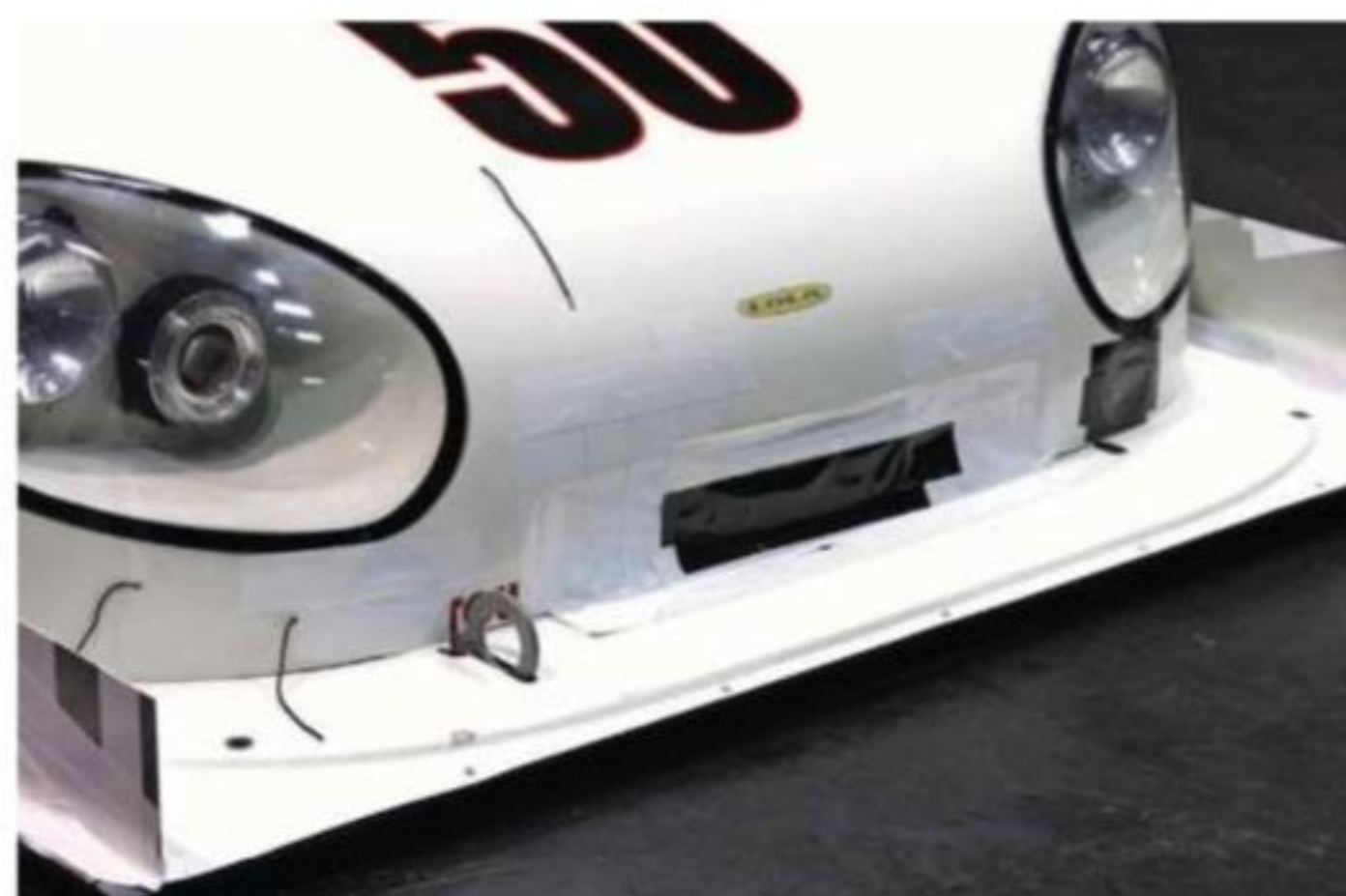
Taping up the front inlets showed potential for more front downforce
