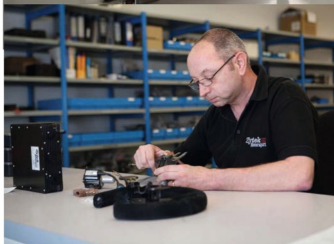
Zytek's third generation electric gearshift actuator works by drawing power from the battery to charge super capacitors, which store up the energy needed to change gear every two or three seconds
