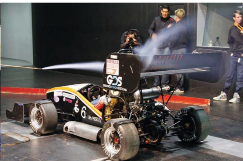
Wing flow attachment was visualised with smoke and wool tufts
