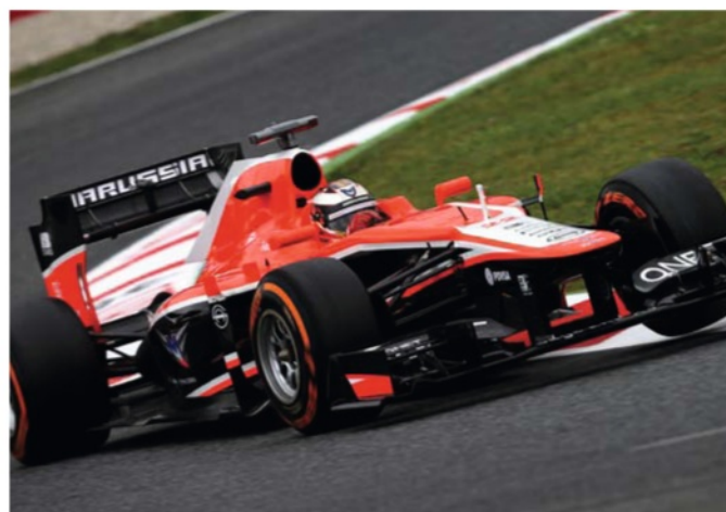
The Russian team has worked with Penske to develop an interlinked suspension, previously only the preserve of the very top teams
