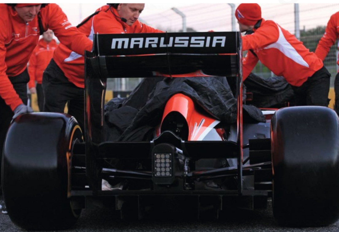
The Marussia MR02 used the same front and rear wings as the MR01 to speed up development, but all teams have worked on the use of exhaust gasses to increase downforce
