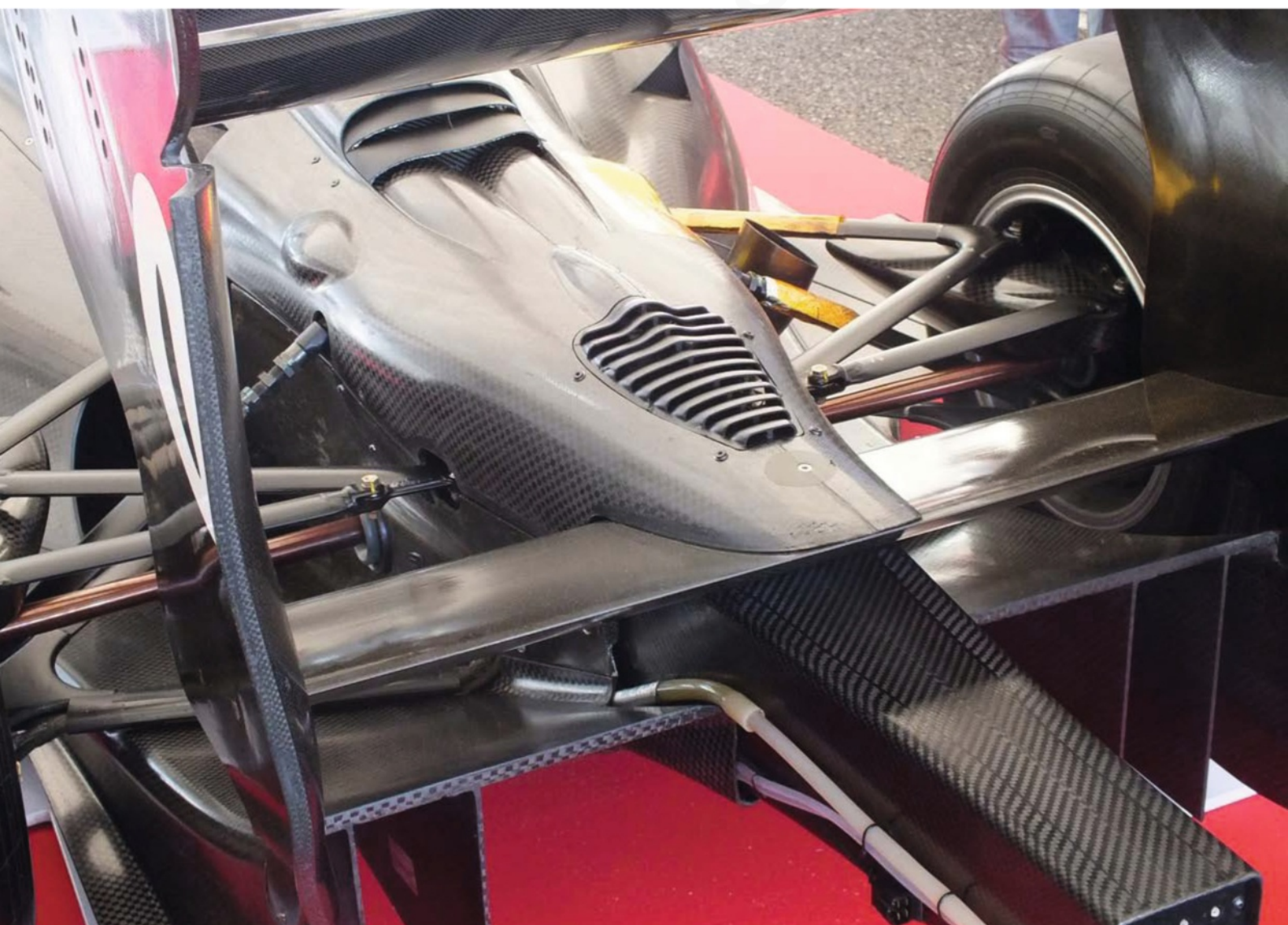
Rear packaging for a spec chassis designed to work with three different engines, although only Honda and Toyota have tested
