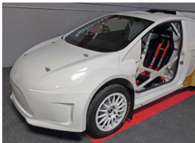
Steel doors for the Fiesta-based Supercar Lite are taken from the roadcar
