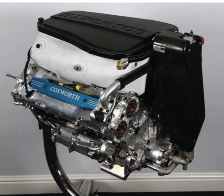
The Cosworth CA 2.4 litre V8 was Cosworth's first engine designed with the specific intention of reaching 20,000rpm
