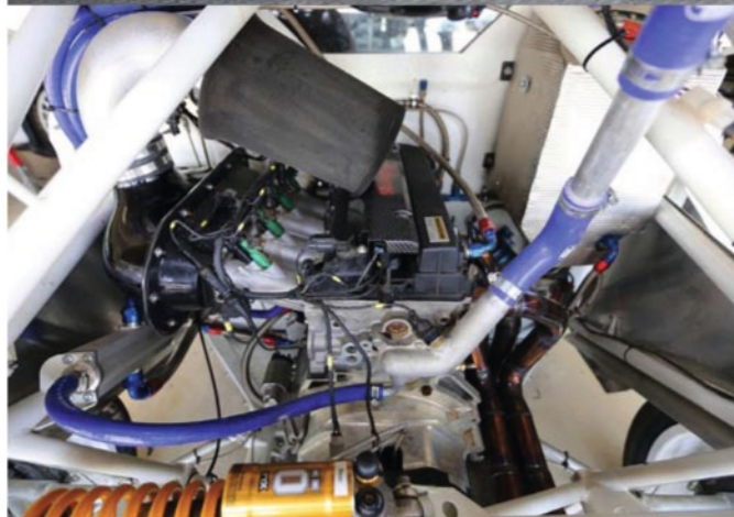
The Ford Duratec engine provides the base. OMSE, with Mountune, reduce capacity to 2.4 litres, with an 8,200rpm red line and it produces 310bhp
