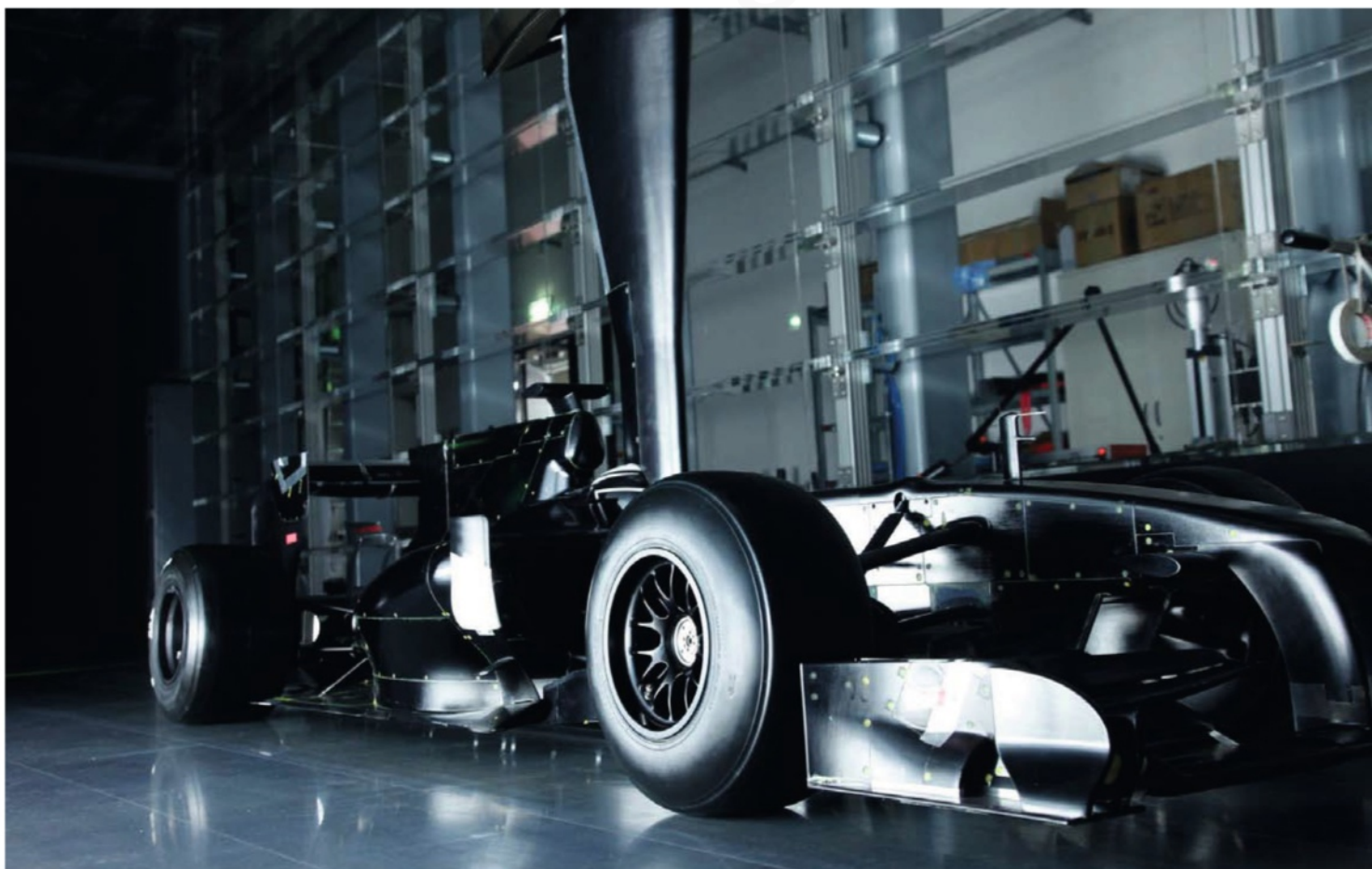
Next year's aero testing is heavily restricted, including a limitation of wind tunnel time and scale; 60 per cent models are the maximum allowed
