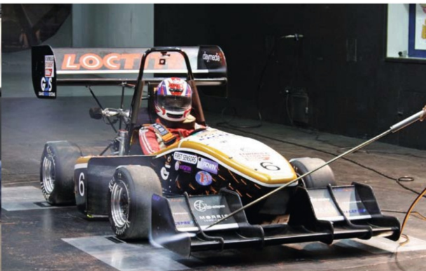
Flows around the front wing end plate came in for close examination
