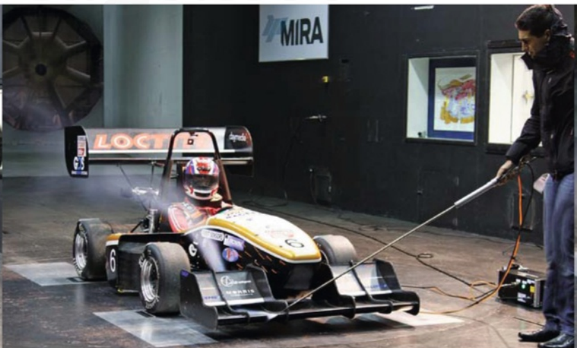
Setting up the split front wing flaps to maximum
