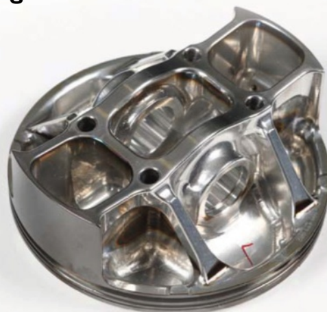
Above: Piston underside required extra cooling at higher revs
