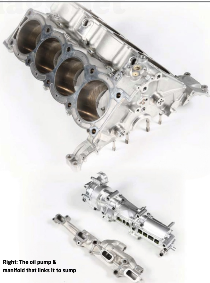
The Cosworth CA 2.4 litre V8 was Cosworth's first engine designed with the specific intention of reaching 20,000rpm
