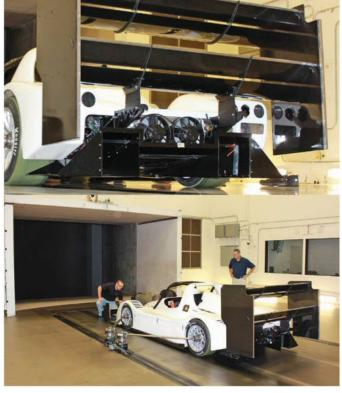
Top: the rear wing assembly, together with the extended diffuser. The fans draw cooling air through the 'airbox' inlet to cool the electric motors Above: getting ready to roll in the Windshear wind tunnel
