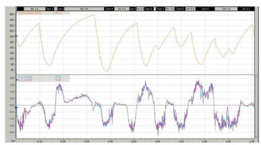
Figure 1: plot of lateral accelerometers and speed for a GT GT3 car
