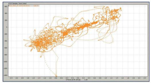
Figure 5: revised plot of lateral moment vs lateral acceleration with further filtering
