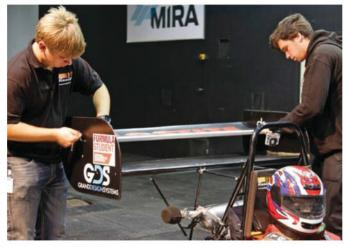
The rear flap in 'DRS' position significantly reduced drag - and downforce
