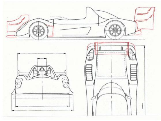
The first concept sketches illustrated a front wing in between the wheel arches and above a slightly extended splitter, and a dual tier rear wing above a slightly extended diffuser
