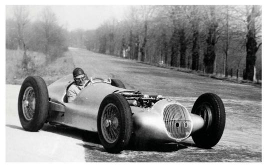
First track test of the Mercedes 154, featuring a 60-degree V12 3-litre supercharged engine
