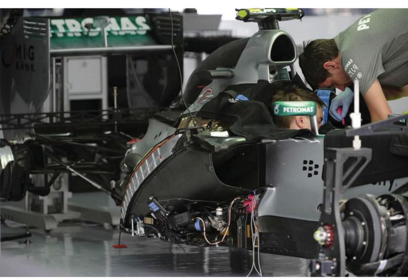
The car's sidepods have become increasingly compact and increasingly crowded with components, as can be seen here - a result of improvements in both design software and computer hardware. Note also the curved radiator
