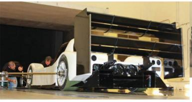
The first run of a wind tunnel programme on an untested configuration is always telling and tends to dictate the path for the rest of the session, despite any plans that might have been drawn up beforehand.
