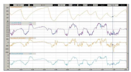
Figure 4: time plot of lateral moment and lateral acceleration
