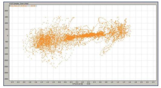
Figure 2: plot of lateral moment vs lateral acceleration for a GT GT3
