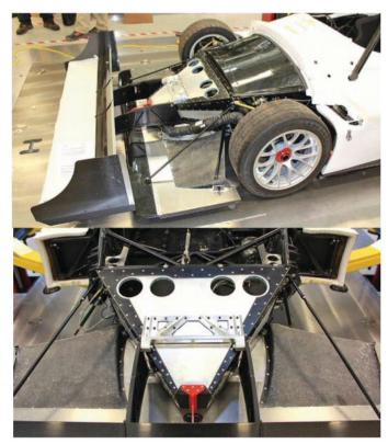
Top: the front wing was located forward of the original splitter lip Above: the front wing mounts cantilevered off a sturdy pair of brackets which were attached to the nose box
