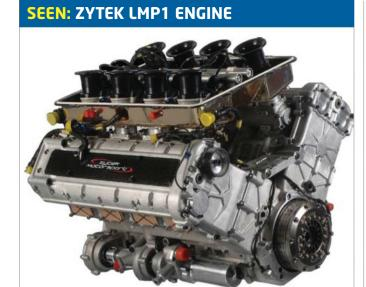
**Zytek has built** an LMP1 engine to the 2014 WEC fuel-flow regulations. The normally-aspirated unit incorporates technology from the company's V8 ZRS-03 engine – as used in Renault World Series FR3.5 – and it will also benefit from advanced control and drive-by-wire technology.
