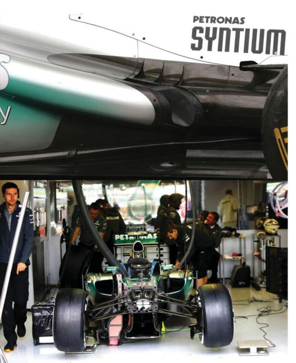
Top: the use of Coanda exhausts in F1 was something that Mercedes initially resisted, but eventually had to accept to keep up with their rivals. Various iterations were run on the W04 Above: the bulkhead of the Mercedes W04 reveals no obvious torsion bars. It is rumoured that the car has dropped the springs as part of its hydraulic suspension system
