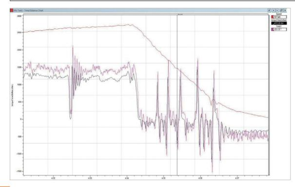
Torque and twist measurement shows the behaviour of the drivetrain during upshifts and downshifts. Note the large torque reversal during downshifts
