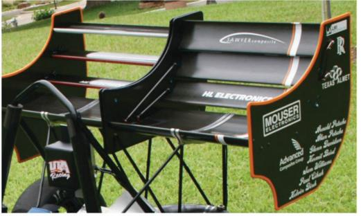
The UTA wing solution is a five-element configuration with a slat, main plane and three flaps
