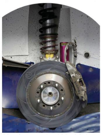
The i20 WRC features a 1.6 GDI Turbo, Brembo brakes and Reiger dampers
