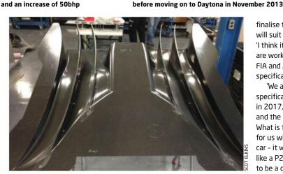
The chosen method of adding downforce was through the diffuser (pictured) and underbody aerodynamics. According to Scot Elkins, utilising the underbody aero helped to push the centre of pressure forwards 'rather than just piling downforce on to the rear'
