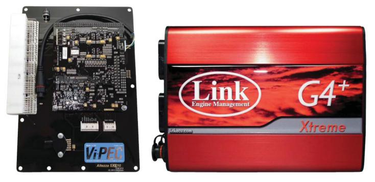
Left: Vi-PEC Altezza Plug-in ECU from New Zealand's Electronz; right: Link's top-of-the-range engine management system - G4+ Xtreme
