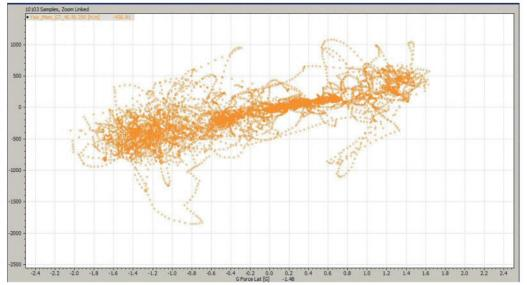
Figure 3: plot of lateral moment vs lateral acceleration filtered at 4Hz
