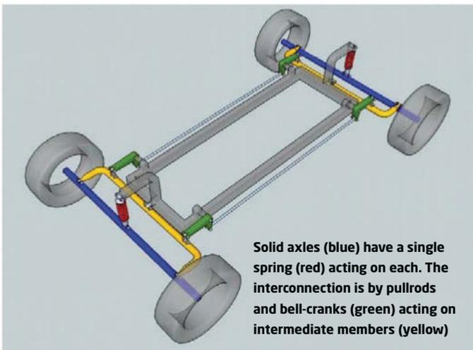
**Solid axles (blue) have a single spring (red) acting on each. The interconnection is by pullrods and bell-cranks (green) acting on intermediate members (yellow)**
