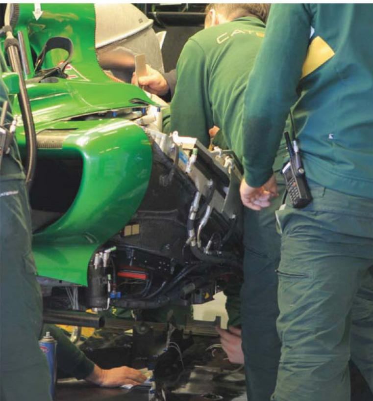
The cooling system on the cars is proving to be a major packaging issue. Here on the Caterham CT05, two heat exchangers are visible, as is the lower side impact structure
