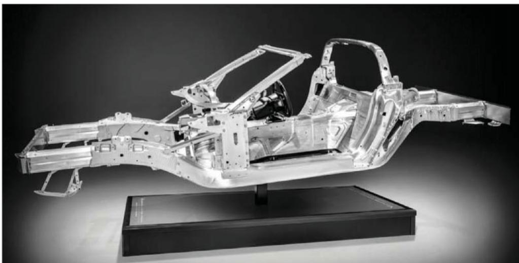
The aluminium frame structure of the Stingray, with 'greater torsional rigidity to improve ride and handling'
