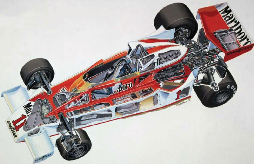
and had a semi-cured sandwich skin folded around machined aluminium bulkheads.'
