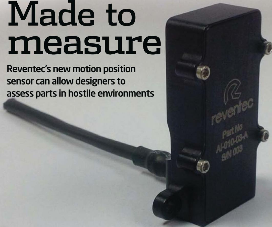
With the Reventec system, the electronics go outside the casing, while the 'target' - a magnet - can be embedded into confined areas
