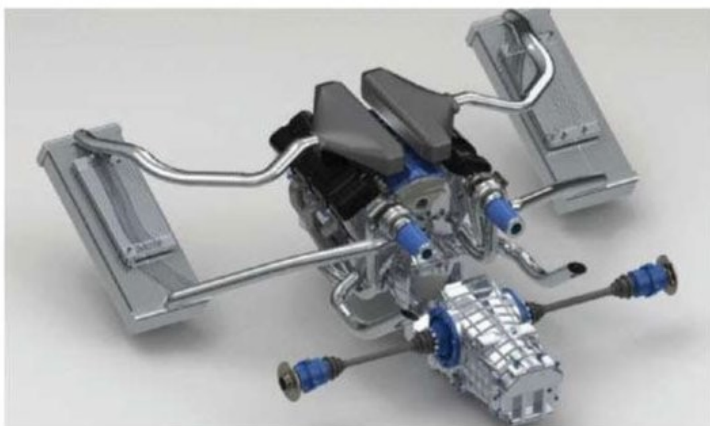
The revised Ford V6 engine with the additional coolers it would require, shown above in rendering form
