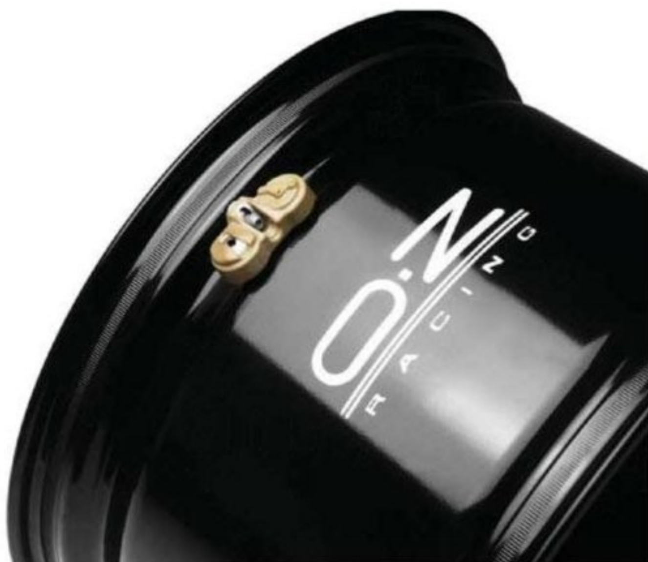
BF1 systems Infra Red Tyre Pressure and Temperature Monitoring System (IRTPTMS) wheel sensor mounted in the wheel rim
