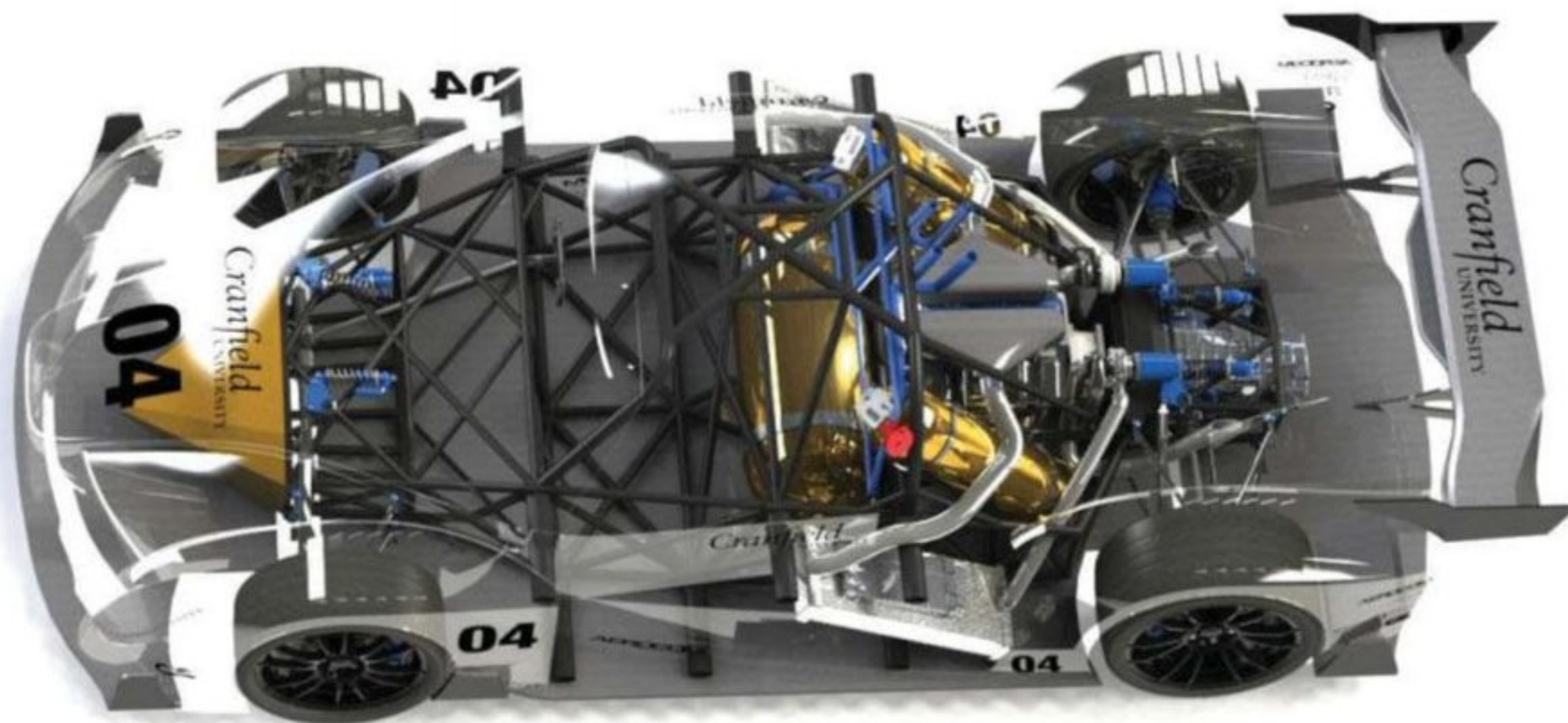
The students reworked the Radical RXC chassis into what is essentially an all-new design
