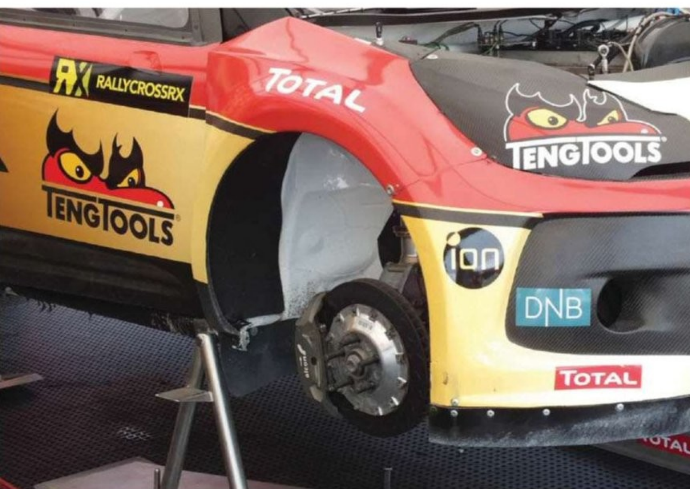
Alcon brakes are a common feature in both team's offerings. Pictured above is a Solberg car. LD, meanwhile, claims that it has 'something a little special in the discs that nobody else has'
