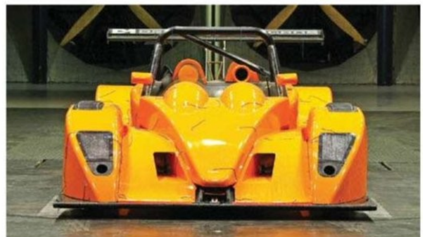
Picture 2: Tiga B presents is a more conventional CN car layout - note that the dummy driver was installed during testing!
