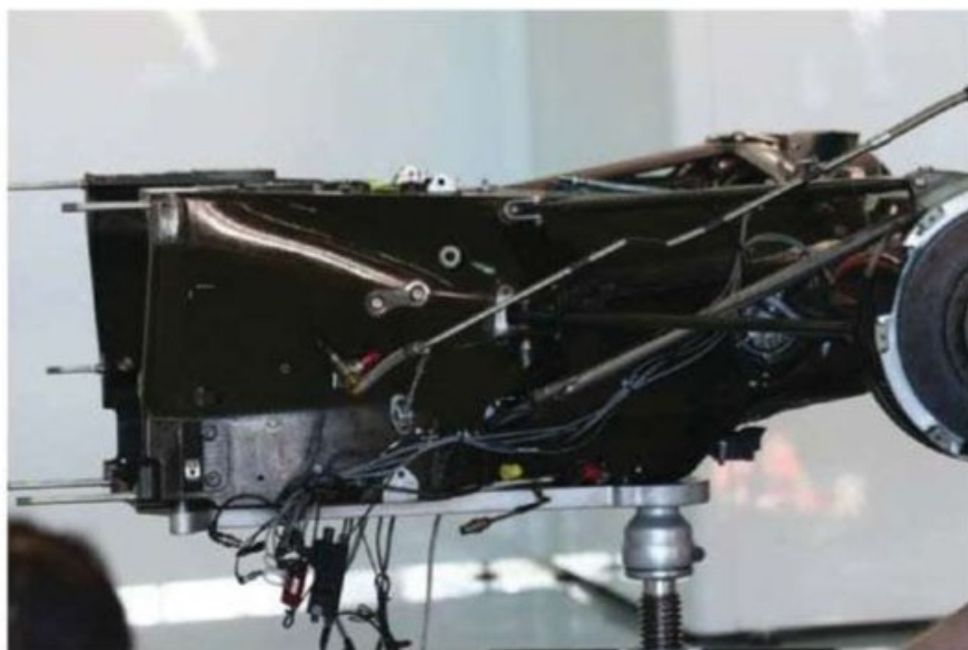
The Marussia shares its transmission with the Ferrari F14-T and the Sauber C33. The MR03 is the first car with which Marussia has used a composite main casing
