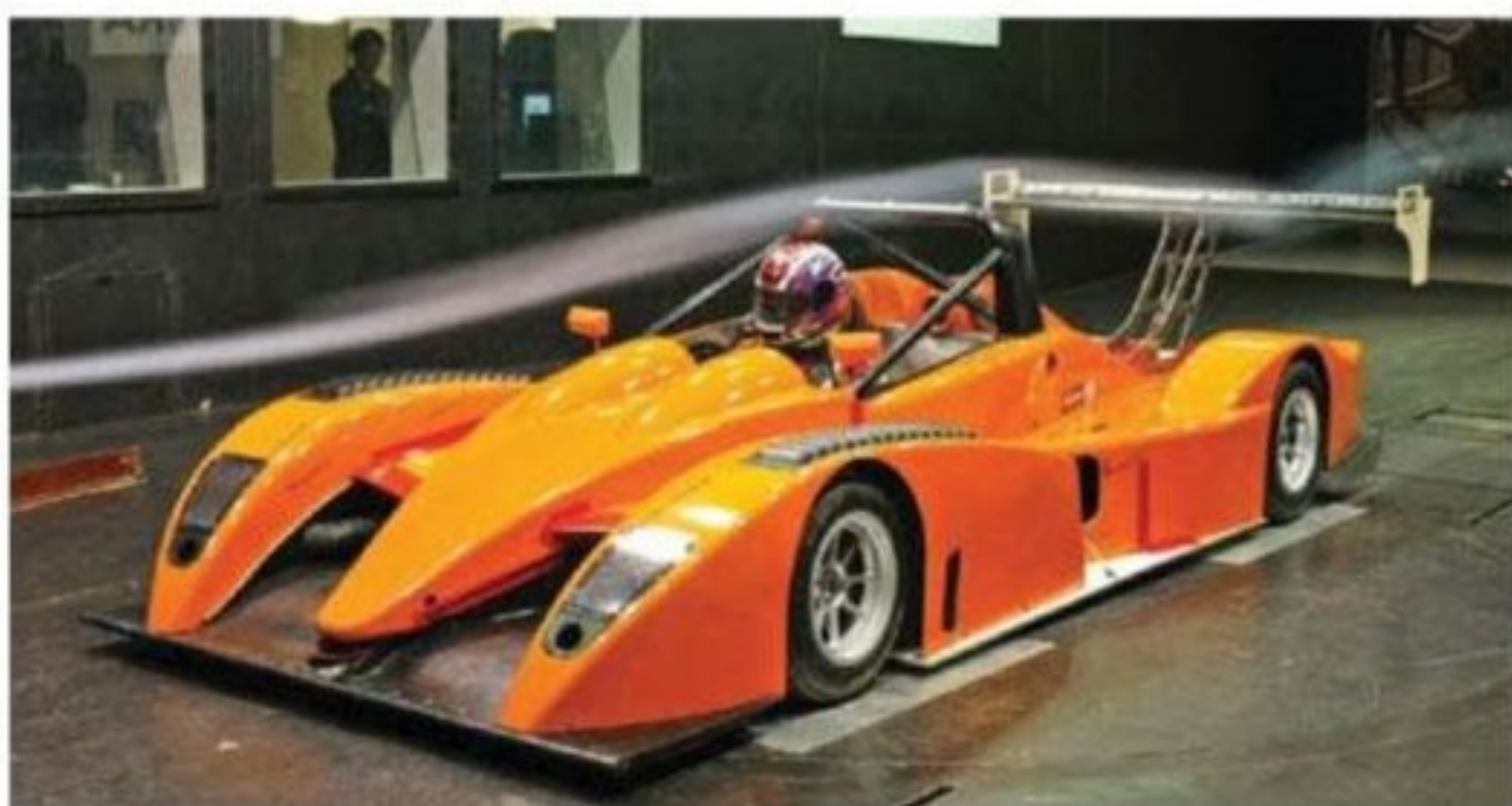
Picture 4: TIGA B's wing exploited the maximum permitted height
